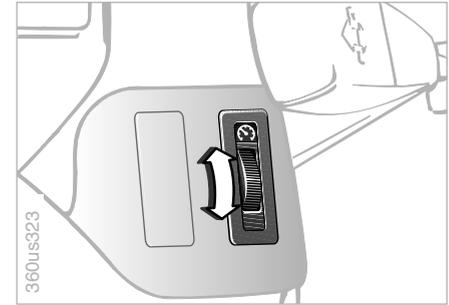
Adjust the illumination intensity by turning the rotary dial.
