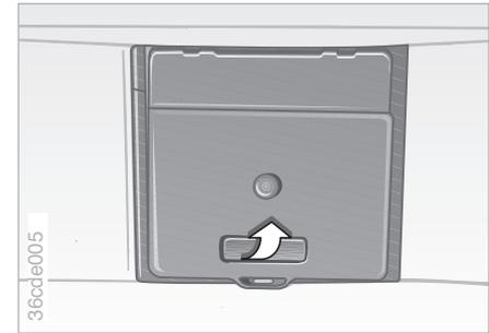
Open the cover panel from the luggage compartment and use the magnetic retainers to attach it to the lower side of the rear shelf within the luggage compartment.
