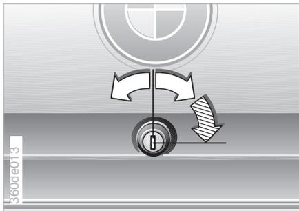
The lock actuation is only possible with a master key.
