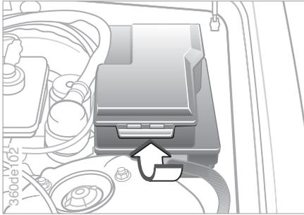
If an electrical device fails, switch it off and check the fuse.
