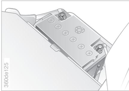
The battery is located behind the right-side trim panel in the luggage compartment. A separate positive terminal in the engine compartment is available for jump-starting (also refer to page 153). Only certain battery types may be used on the BMW convertible. Consult your BMW Retailer for details.
