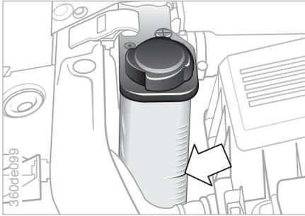
Coolant level with engine cold: up to the KALT/COLD mark on the transparent coolant expansion tank.
