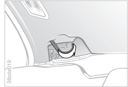
Before positioning the hardtop on the car, fold down the covers below the interior lamps at the left and right and open the locking levers outward.
