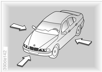
The airbags are triggered by impacts coming from the directions shown in the illustration. Note that the supplementary protection against lateral impact is available only on vehicles equipped with optional door-mounted airbags.
