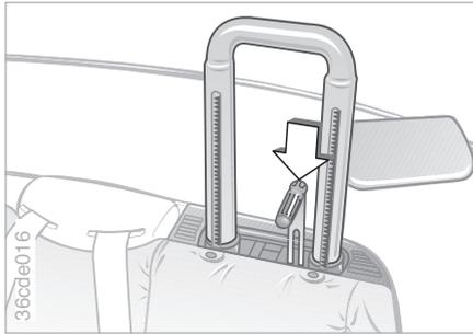
Following an unforeseen, automatic extension, the rollover protection system can be lowered again.
