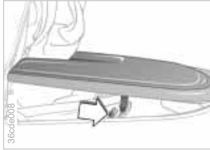
Position the rear convertible top bow vertically and hold in place. Raise the convertible top compartment lid somewhat and unlock the catch lock by pushing it to the right. Open the convertible top compartment lid completely.
