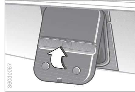
Use the magnetic retainers to attach the cover panel to the lower side of the rear shelf within the luggage compartment.
