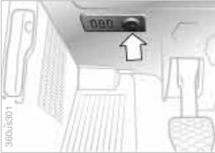
The OBD II interface (data link connector) is located beneath a cover panel (with the letters "OBD") near the foot support in the driver's side footwell (arrow).
