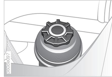
With the engine off, unscrew the reservoir cap, then reinsert it.
