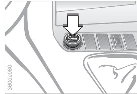
Press in. Remove as soon as the lighter jumps back out.
