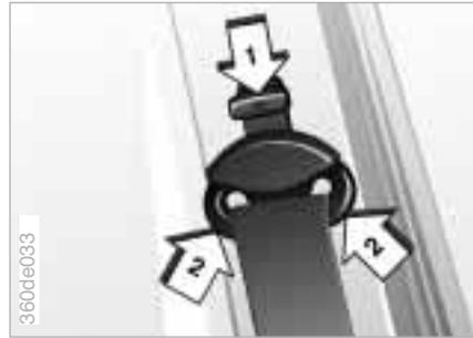
The safety belt can be adjusted individually to different body sizes with the belt height adjustment:
