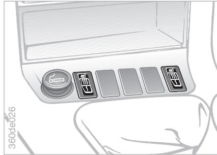
The seat cushion and backrest can be heated at ignition key position 2.
