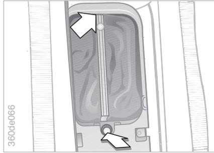
Press the round button to unlock the cover panel in the luggage compartment.
