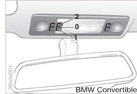
BMW Convertible: With the switch set to position 1, a safety circuit ensures that any lamps in the vehicle which may still be on are switched off automatically approx. 15 minutes after leaving the vehicle.
