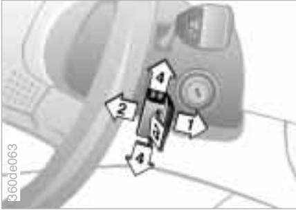
You can store and automatically maintain any desired vehicle speed above approx. 25 mph (40 km/h).
