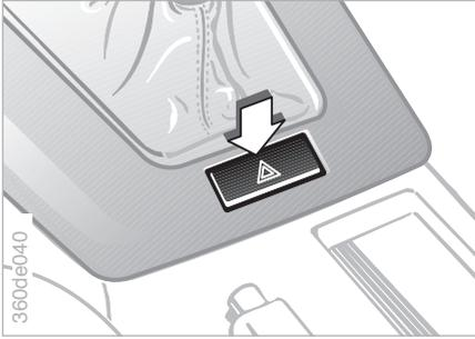
The button flashes intermittently when the hazard warning lamps are on.
