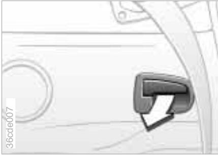
Unlock the convertible top storage compartment with the handle in the rear left side panel.
