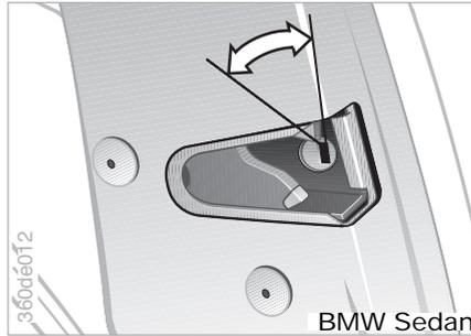
Insert the key in the slot in one of the rear door latch mechanisms and turn toward the outside: the door can now be opened from the outside only.
