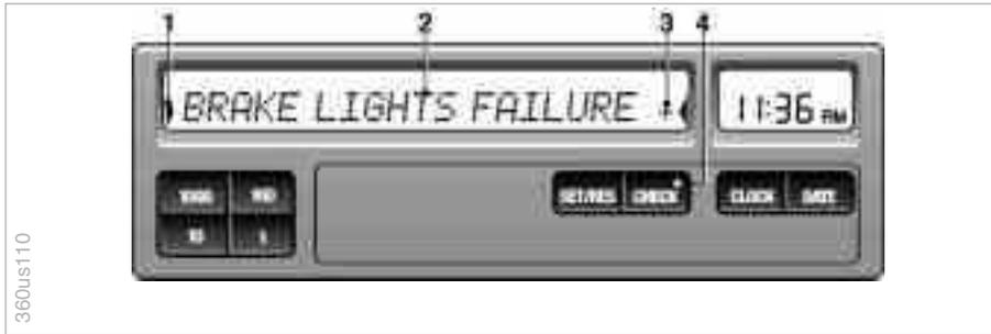
Texts with messages and warnings are used to alert the driver to defective systems. In addition, there is a warning lamp in the instrument panel.
