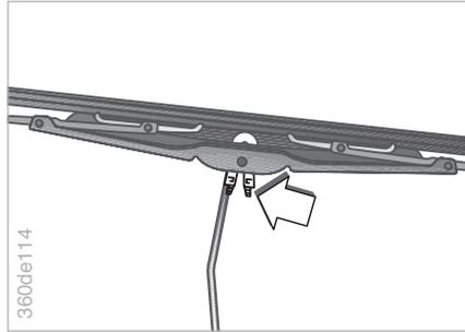
Lift the wiper arm, press the locking spring and pull off the wiper blade, pulling along the wiper arm.
