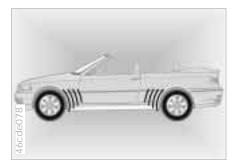
There is an antenna located right near every wheel in the vehicle body. Each antenna picks up signals from its respective wheel. A central electronics system evaluates all four signals and forwards any changes. The RDC provides an important contribution to driving safety.
