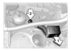
ing is identified by a "+" sign. Refer to the illustration. Remove by pulling the tab (arrow 1)
