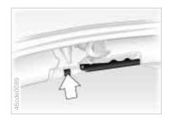
4 Open both front locking levers. To do this press the buttons. The levers will loosen somewhat. Flip the levers open until they hit the stop
