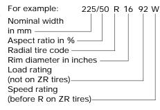
The speed rating indicates the approved maximum speed for the tire.
