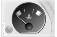
Coolant temperature gauge Service Interval Display
