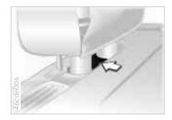
If this safety feature is no longer needed after it has been automatically deployed, then the rollover protection system can be lowered again. No special tools of any kind are needed to do this.
