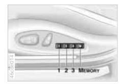
You can store and recall three different driver's seat and outside mirror positions. The illustration shows the buttons on the driver's seat, for making these position adjustments.
