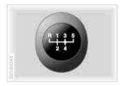
The shift lever's neutral plane (dot in the illustration) is located between 3rd and 4th gears.
