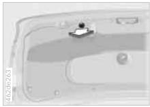
Bulbs in the luggage compartment lid: 1 Using a screwdriver, loosen the clip
