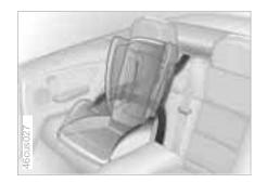
All of the rear belt retractors and the front passenger's safety belt can be locked for mounting and securing child restraint systems.
