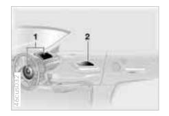
1 Front airbags for driver and passenger The illustration depicts schematically 2 Side airbags (front)
