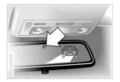
The semisolid reacts chemically to this electrical current, dimming the mirror through an infinitely-variable range (electrochromic technology).
