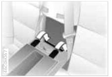
To re-attach the fill piece, guide the tabs into the strip of molding and snap the fill piece back into place. The safety belts can then be re-secured into their holders. ◀
