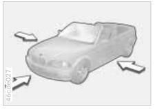
the primary directions of vehicle impact that initiate airbag deployment.
