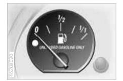
When you switch on the ignition, the indicator lamp lights up briefly as an operation check.
