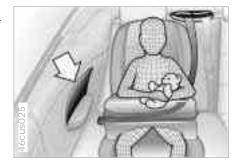
This is the right way a child should sit in a child restraint when rear side airbags (arrow) are provided.
