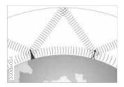
The AM frequency bands (medium-wave, long-wave and short-wave) make it possible to receive stations from a great distance, because the broadcast signals travel not only along the ground as surface waves, but also as atmospheric waves that are reflected from the ionosphere. Frequency-modulation (FM) provides substantially better sound quality than the other frequencies. However, because FM transmissions rely on line-of-sight broadcast waves, their effective reception range is limited.
