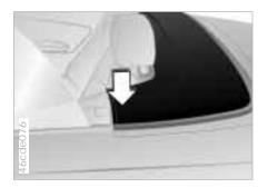
The central locking system unlocks automatically when the convertible top compartment lid is closed, i.e., the luggage compartment lid is no longer locked and can be opened again.
