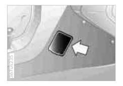
The connector for the Onboard Diagnostic system (OBD) is located in the center console under a cover on the passenger's side (arrow).
