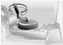
Using the wrench from the onboard tool kit (fastened to the jack with a Velcro<sup>®</sup> strip), turn the screw (arrow) two to three turns into the windshield frame on the right and left sides. Turn the right and left locking levers of the rear hardtop mounting fasteners in the direction of the arrow to the stop.
