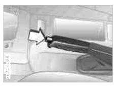
The parking brake is designed primarily to prevent the vehicle from rolling when parked. It operates against the rear wheels.
