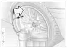
2 Remove the round cover and take out hose 4. Unscrew the valve stem cover from the defective wheel and screw the hose to the valve.
