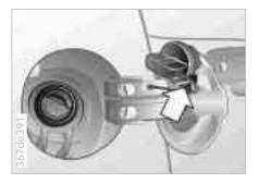
Before filling the tank, shut off the engine, as otherwise fuel cannot flow into the tank and the Service Engine Soon warning lamp may come on. Refer to page 22.
