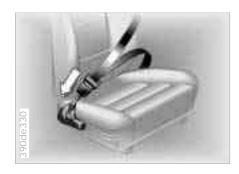
The safety belt tensioner responds to severe frontal impacts by tightening the belts to ensure that occupants remain firmly positioned in their seats. A gaspressure system retracts the buckle assembly to tension the shoulder and lap belts within fractions of a second. This tends to further reduce the tendency to slide under the lap belt. Overview
