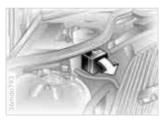
4 Start by connecting the jumper cable from the positive terminal of the support vehicle to the auxiliary terminal for jump-starting located in your BMW's engine compartment. The cover of the auxiliary terminal for jump-starting is indicated by a "+" sign. Refer to the illustration. Flip the cap forward to open.
