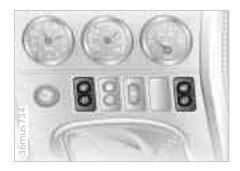
The seat cushion and backrest can be heated in ignition key position 2.
