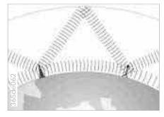
The AM frequency bands (mediumwave, long-wave and short-wave) make it possible to receive stations from a great distance, because the broadcast signals travel not only along the ground as surface waves, but also as atmospheric waves that are reflected from the ionosphere.
