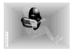
Deceleration sensors continuously monitor the physical forces acting upon the vehicle. In the event of a severe frontal impact, the gas generators of the driver- and passenger-side front airbags are ignited simultaneously. However, the passenger-side front airbag is only triggered if an additional sensor has recognized that the passenger seat is occupied.
