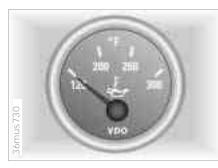
During normal operation the engine oil temperature is between 175 °F (80 °C) and 250 °F (120 °C). During performance-oriented driving, do not exceed the maximum temperature of 265 °F (130 °C).
