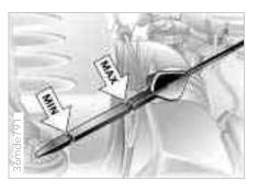
The space between the two marks on the dipstick corresponds to approx. 1.4 US quarts (1.3 liter). Do not fill beyond the upper mark on the dipstick. Excess oil will damage the engine.
