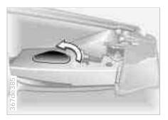
Rotate the cover panel which is located in the right and left trim panels behind the seats in the direction of the arrow until the opening for the hardtop mount is completely free.
