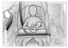
This is the right way a child should sit in a child restraint when side airbags (arrow) are provided.
