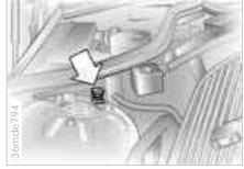
5 Then connect the negative terminals. First attach the cable to either the support vehicle's negative battery terminal "-", or to a suitable ground on its engine or body. Then connect the other terminal of the cable to a ground on the engine or on the body of the vehicle which is to be started. This is a special nut which is provided on the suspension strut dome of the BMW. Refer to the arrow in the illustration.
