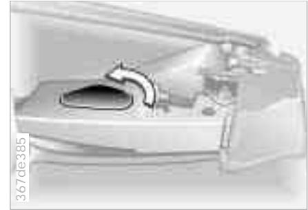
Rotate the cover panel which is located in the right and left trim panels behind the seats in the direction of the arrow until the opening for the hardtop mount is completely free.
