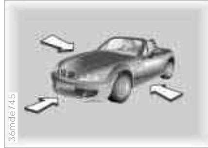
The illustration depicts schematically the primary directions of vehicle impact which initiate airbag deployment.
