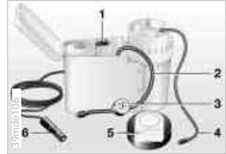
The M Mobility system is located in the luggage compartment at the rear right, on the M coupe also under a cover.
