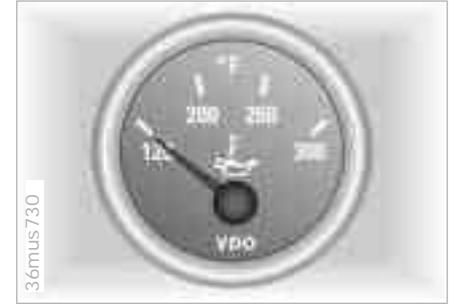
During normal operation the engine oil temperature is between 175 °F (80 °C) and 250 °F (120 °C). During performance-oriented driving, do not exceed the maximum temperature of 265 °F (130 °C).
