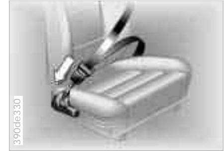
The safety belt tensioner responds to severe frontal impacts by tightening the belts to ensure that occupants remain firmly positioned in their seats. A gas-pressure system retracts the buckle assembly to tension the shoulder and lap belts within fractions of a second. This tends to further reduce the tendency to slide under the lap belt.
