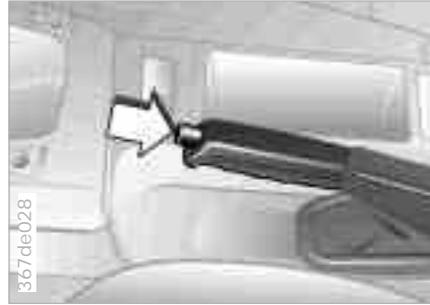
The parking brake is designed primarily to prevent the vehicle from rolling when parked. It operates against the rear wheels.
