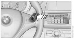
Insert the remote control all the way into the iqnition lock.
