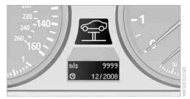
The remaining driving distance and the date of the next scheduled service are displayed briefly immediately after you start the engine or switch on the ignition.
