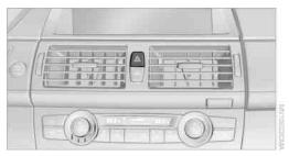
The button for the hazard warning system is located on the center console.
