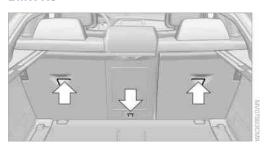
For child restraint fixing systems with tether strap, there are three additional mounting points
