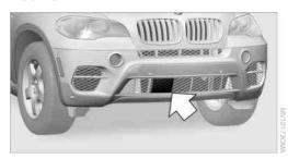
The radar sensor is integrated in the bumper.
