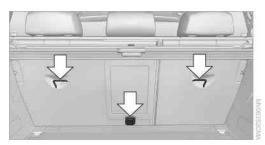
There are three additional mounting points for child restraint fixing systems with a tether strap on the 2nd row seats, refer to arrows. Fold out before using the center mounting point.
