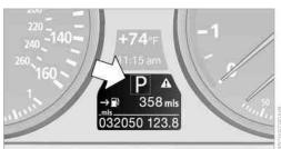
The gear position is displayed and the engaged gear, such as M4, is displayed in manual mode.
