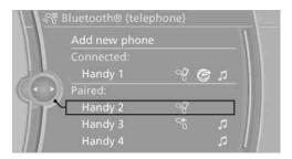
The functions that were assigned to the device before unpairing are assigned to the device when it is reconnected. If the device is already connected, these functions are deactivated.
