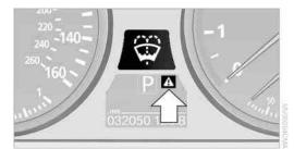
⚠ The symbol indicates that Check Control messages have been stored. The Check Control messages can be displayed later.
