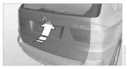
Press the button, see arrow, or the button of the remote control for approx. 1 second. The tailgate opens slightly. It can be swung upward.
