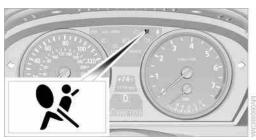
In the radio ready state and beyond, refer to page 61, the warning lamp comes on briefly to indicate that the entire airbag system and the belt tensioners are operational.
