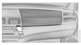
Press the button. The covers open upward and downward and the lighting in the glove compartment switches on.
