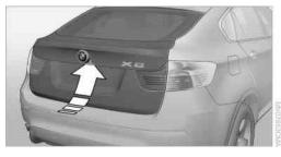
Press the button on the outside of the tailgate when the vehicle is unlocked.
