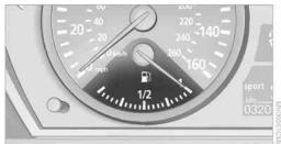
The vehicle inclination may cause the display to vary.
