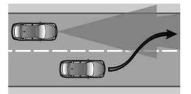
A vehicle driving in front of you is not detected until it is completely within the same lane as your vehicle.
