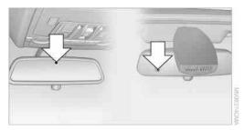
Two photocells are used for control:
