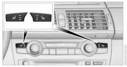
The temperature setting progresses one step through its control sequence each time you press the button. The maximum temperature is reached when three LEDs are lit.
