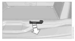
Pull the lever and swing the tailgate downward.
