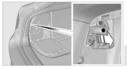
Apply gentle pressure to the bulb while turning it to the left for removal and replacement.
