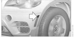
The two camera lenses are located on the sides of the bumper.
