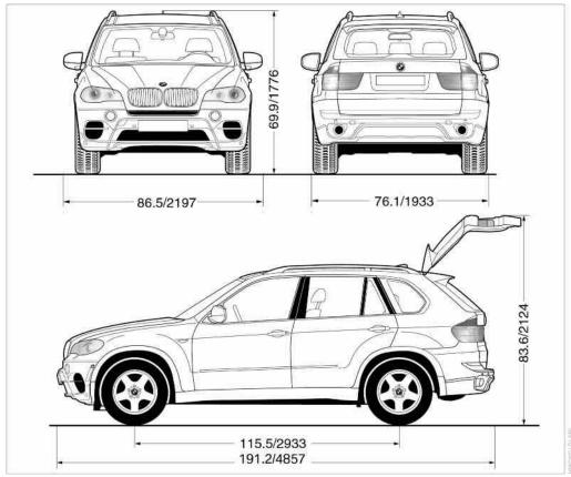
All dimensions given in inches/mm. Smallest turning circle dia.: 42.0 ft/12.8 m With mixed tires\* the vehicle width may exceed the specified dimension.
