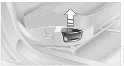
Pull the lever and slide the seat into the desired position. After releasing the lever, move the seat forward or back slightly to make sure it engages properly.
