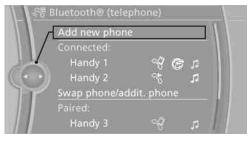
4. To perform additional steps on the mobile phone, refer to the mobile phone operating instructions: for instance, search for or connect the Bluetooth device or a new device.
