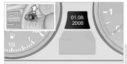
Press the button on turn signal lever upward; the date appears.
