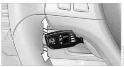
Press the lever up or down and additionally depress the brake if the vehicle is stationary. The mark in the speedometer changes color and the distance indicator goes out.
