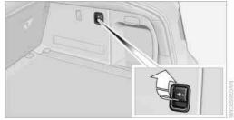
To access the socket: fold open the cover.
