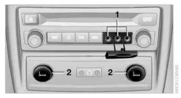
Connections for audio/video cables. Watch the colors of the sockets when connecting.
