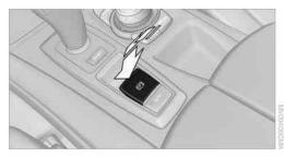
Press the button with the brake depressed.
