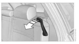
Pull the lever and fold the seat forward.
