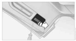
2. Push the catch on the bulb holder to the left, arrow, and remove it.
