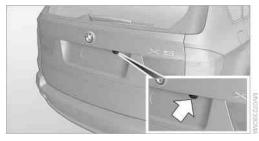
The lens of the rear view camera is under the grasping lip of the tailgate.
