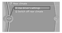
The rear automatic climate control cannot be operated if the front automatic climate control is switched off. With the defrost windows and eliminate condensation function activated, the rear automatic climate control is also not ready for operation.
