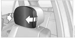
You can fold the side extensions on the head restraint forward for increased lateral support in the resting position.
