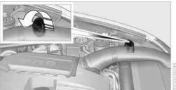
Left side of vehicle: rotate the bulb holder to the right, see arrow, and remove.
