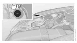
Rotate the bulb to the right along with the socket and replace.
