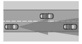
The detection capacity of the system and the automatic braking capacity are limited. Two-wheeled vehicles driving ahead of you for instance might not be detected.
