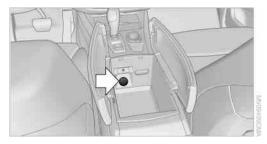
To access the socket\*: remove the cover.
