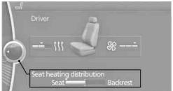
Turn the controller to adjust the distribution.The setting is applied.
