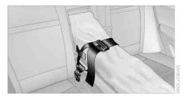
BMW X6: attach the hook of the ski bag retaining strap to the eyelet on the backrest.
