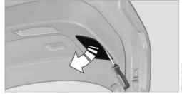
Rotate the bulb socket to the left and remove.
