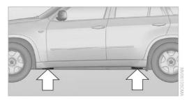
Guide the jack head into the rectangular recess of the jacking point when cranking up, refer to illustration detail.
