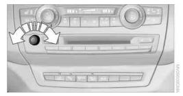
Turn the knob until the desired volume is selected. The setting is stored for the remote control currently in use.
