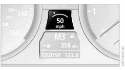
The system stores the current vehicle speed. It is indicated on the speedometer and briefly in the instrument panel.
