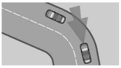
If the desired speed is too high for a curve, the speed is reduced slightly in the curve, although curves cannot be anticipated in advance. Therefore, drive into a curve at an appropriate speed. In tight curves, situations may result due to the restricted detection range of the system in which a vehicle driving ahead of you may not be detected at all, or not until after a considerable delay.
