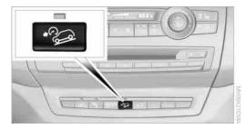
Press the button; the LED above the button lights up.
