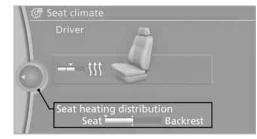
Turn the controller to adjust the distribution. The setting is applied.
