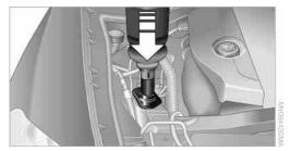
3. The reservoir is full when the fill level in the bottle stops changing. It is not possible to
