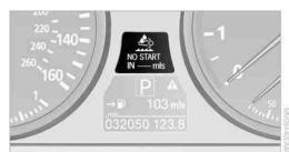
Even with a display of -- mls, the engine will continue to run, provided that it is not switched off, and all other operating requirements are met, e.g. sufficient fuel.
