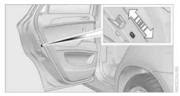
Push the locking lever on the rear doors down. The door can now be opened from the outside only.
