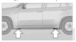
The jacking points for the vehicle jack are located in the positions shown.
