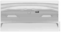
The tailgate closes automatically when the button on the inside of the tailgate is pressed.
