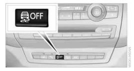
Press and hold the button, but not longer than approx. 10 seconds, until the indicator lamp for DSC lights up in the instrument cluster and DSC OFF is displayed. DTC Dynamic Traction Control and DSC are deactivated together.
