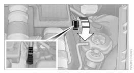
The so-called starting aid terminal in the engine compartment acts as the battery's positive terminal. Fold open the cover. To do so, pull the tab.
