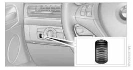
Adjust the brightness using the thumbwheel.
