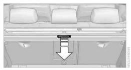
Pull out the luggage compartment roller cover and hook it into the brackets.
