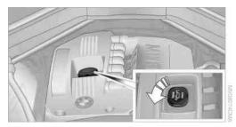
Add a maximum quantity of 1 US quart/1 liter of oil only after the corresponding message appears on the Control Display.
