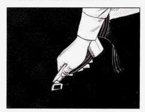
Put the belt's special latch plate into the vehicle's safety belt buckle.
