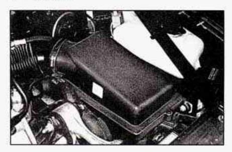
The air cleaner is in the right front area of the engine compartment.
