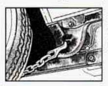
Attach "T" hook chains into slots in the bottom of the floor pan just ahead of the rear wheels on both sides.
