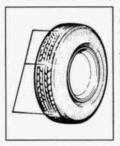
One way to tell when it's time for new tires is to check the treadwear indicators, which will appear when your tires have only 2/32 inch (1.6 mm) or less of tread remaining.
