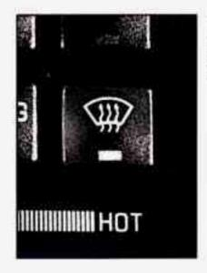
When fog or ice is on the windshield, this setting directs the maximum air flow toward the windshield.
