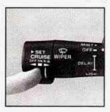
Move the Cruise switch from "ON" to "Resume/Accelerate," Hold it there until you get up to the speed you want, and then release the switch.  To increase your speed in very small amounts, move the switch to "Resume/Accelerate" for less than half a second and then release it. Each time you do this, your vehicle will go about 1 mph (1.6 km/h) faster.
