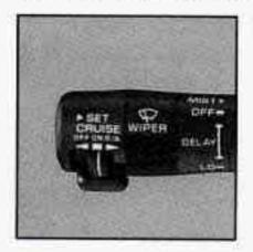
Move the Cruise Control switch to "ON."
