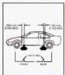
Position the jack under the vehicle. Your Buick has a notch on the frame near each of the wheels. Fit the lift head into the notch nearest the wheel with the flat tire.
