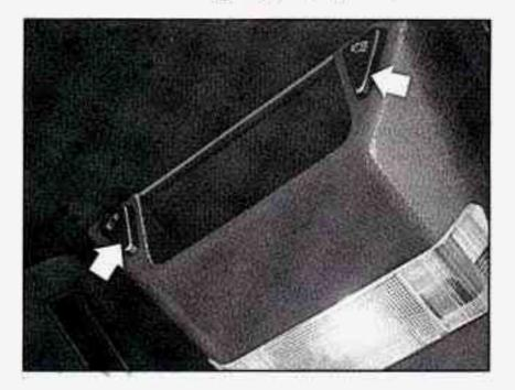
The front seat reading lights are turned on by pressing the switches.
