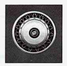
If there is a wheel cover, remove it by using the flat end of the wheel wrench. Pry along the edge of the wheel cover until it comes off. Be careful, the rim edges may be sharp. Don't try to remove it with your bare hands.
