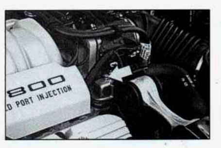
3.8L V6 (VIN Code L27): There is one bleed valve. It is located on the thermostat housing.
