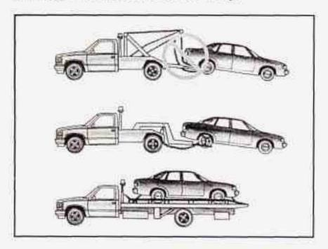
Use wheel lift or car carrier equipment. Additional ramping may be required for car carrier equipment. Use safety chain and wheel straps.
