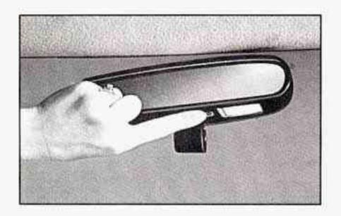
The reading lights on the inside rearview mirror are turned on by pressing the switch.
