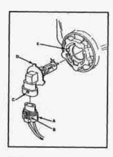
Remove the electrical connector (A) from the bulb by raising the lock tab (B) and pulling the connector down and away from the bulb's plastic base (C).
