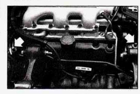
3.1L V6 (VIN Code T or M): There are two bleed valves. One is located on the thermostat housing. The other is located on the thermostat bypass tube.
