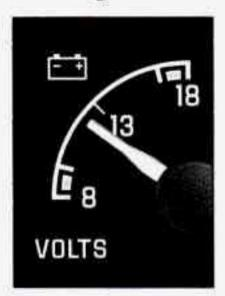
The "Volts" gage shows voltage in the electrical system. The normal range is 11 to 15 volts. If the gage reading stays in either red range, have your Buick dealer check the electrical system.
