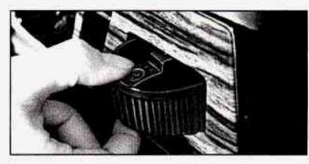
To remove the rear ashtray for cleaning, press down on the snuffer as you pull the ashtray down and out.
