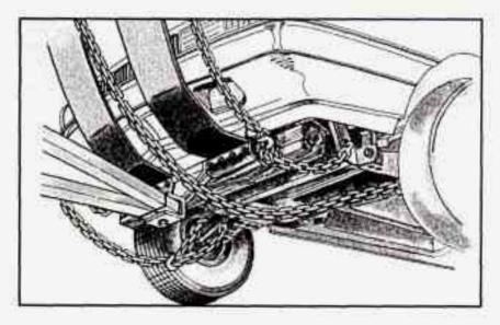
Position a 4" x 4" wood beam across the sling chains against the bottom of the cradle horns. Position the lower sling crossbar against the front of the 4" x 4" wood beam.
