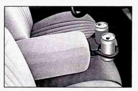
The armrest between the front seats opens into a storage area. To open it, press the lever at the front edge and lift the cover. To use the cupholder which is stored inside, pull it up and rotate it forward. You may have an adjustable cup holder.
