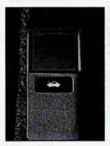
To open the hood, first pull the handle inside the vehicle. It is located on the floor next to the driver's seat.
