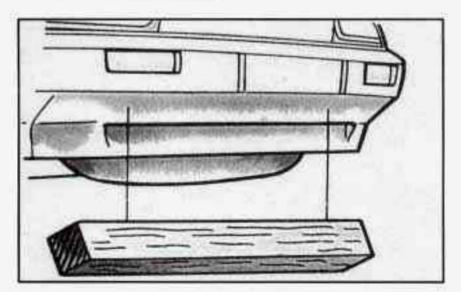
Position a 4" x 4" wood beam across the sling chains and center in the middle of the lower facia.
