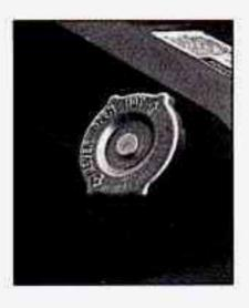
10. Then replace the pressure cap. At any time during this procedure if coolant begins to flow out of the filler neck, reinstall the pressure cap. Be sure the arrows on pressure cap line up like this.
