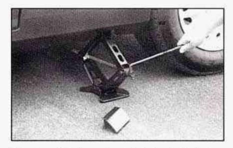
Raise the vehicle by rotating the jack handle clockwise. Raise the vehicle far enough off the ground so there is enough room for the spare tire to fit.
