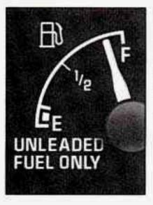
Your fuel gage shows about how much fuel is in your tank. It works only when the engine is on. When the indicator nears "E," you still have a little fuel left. You need to get more right away. Here are some concerns owners have had about the fuel gage. All these situations are normal and indicate nothing wrong with the fuel gage.
