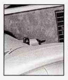
Press down on the switch to make your front and rear turn signal lights flash on and off.
