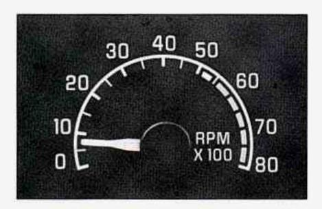
The tachometer tells you how fast the engine is running. It shows speed in revolutions per minute (RPM). Do not operate your engine in the red line range. If you do you can cause severe engine damage.
