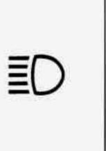
To change the headlights from low beam to high or high to low, pull the turn signal lever all the way toward you. Then release it. When the high beams are on, this blue light on the instrument panel also will be on.
