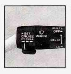
Push the button at the end of the lever, then release the button and the accelerator pedal. You'll now cruise at the higher speed.
