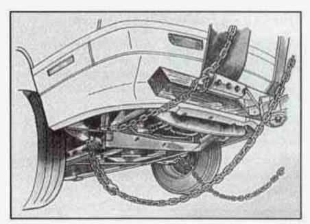
Position the lower sling crossbar against the front of the 4" x 4" wood beam.
