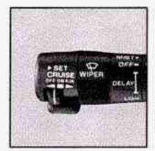
With Cruise Control, you can maintain a speed of about 25 mph (40 km/h) or more without keeping your foot on the accelerator. This can really help on long trips. Cruise Control does not work at speeds below about 25 mph (40 km/h).
