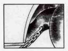
Attach "T" hook chains in front of the wheel into the side slots in the cradle on both sides.
