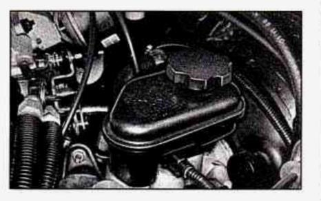
There are only two reasons why the brake fluid level in your master cylinder might go down. The first is that the brake fluid goes down to an acceptable level during normal brake lining wear. When new linings are put in, the fluid level goes back up. The other reason is that fluid is leaking out of the brake system. If it is, you should have your brake system fixed, since a leak means
