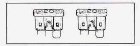
Look at the silver-colored band inside the fuse. If the band is broken or melted, replace the fuse. Be sure to replace the bad fuse with a new one of the identical size and rating.
