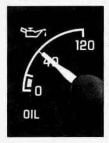
You can read your engine oil pressure directly from the gage on your instrument panel.
