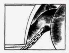
Attach "T" hook chains in front of the wheels into the side slots of the cradle on both sides.
