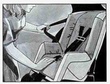
To tighten the belt, feed the shoulder belt into the retractor while you push down on the child restraint.
