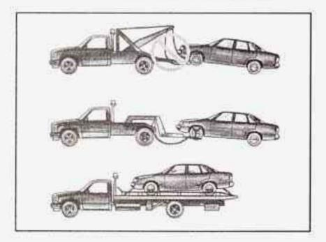
Use wheel lift or car carrier equipment. Additional ramping may be required for car carrier equipment. Use safety chain and wheel straps.
