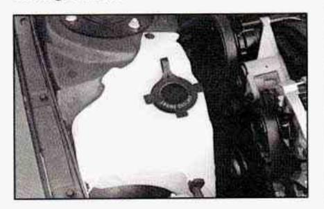
The coolant recovery tank is located at the left of the engine compartment.
