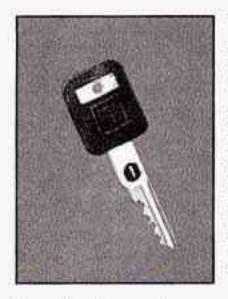
Your vehicle is equipped with the PASS-Key<sup>®</sup>II (Personalized Automotive Security System) theft deterrent system. PASS-Key<sup>®</sup>II is a passive theft deterrent system. This means you don't have to do anything different to arm or disarm the system.
