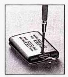
If your transmitter has a screw, remove the screw from the back cover. If there is no screw, carefully pry off the cover by inserting a dime (or similar object) in the slot between the covers and twist.
