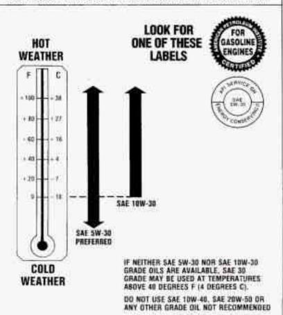
If your vehicle has the 3.1L engine, as shown in the chart, SAE 5W-30 is best for your vehicle. However, you can use SAE 10W-30 if it's going to be 0°F (-18°C) or above. These numbers on an oil container show its viscosity, or thickness. Do not use other viscosity oils, such as SAE 10W-40 or SAE 20W-50.
