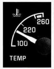
This gage shows the engine coolant temperature. If the gage pointer moves into the red area, your engine is too hot!
