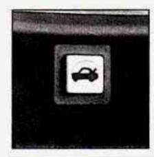
The remote trunk release button is in the glovebox. It works only when the transaxle is in Park.
