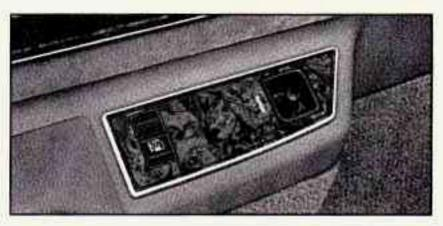
To adjust your left outside mirror move the control located on the driver's door.
