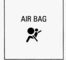
You will see this light flash for a few seconds when you turn your ignition to "Run" or "Start." Then the light should go out, which means the system is ready.
