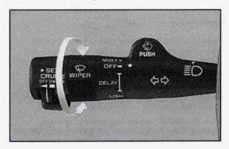
You control the windshield wipers by turning the band marked "WIPER". For a single wiping cycle, turn the band to "MIST." Hold it there until the wipers start, then let go. The wipers will stop after one cycle. If you want more cycles, hold the band on "MIST" longer.
