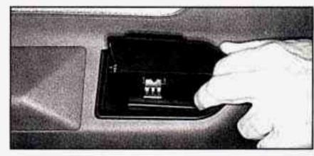
This ashtray can be removed for cleaning by lifting it out of the armrest.
