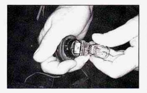
Pull the bulb straight out to remove it from its socket. The new bulb must be aligned properly, then push it in the socket. Reinstall the socket, taillight, and rear trunk trim.
