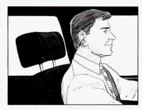
Slide the head restraint up or down so that the top of the restraint is closest to the top of your ears.
