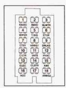
This fuse panel is inside the glove box. Pull the cover down to access the fuses. Some spare fuses and a fuse puller are included.
