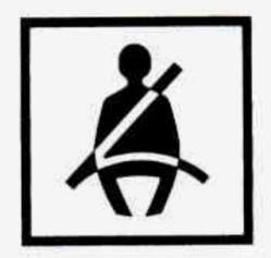
This figure lights up as a reminder to buckle up. (See "Safety Belt Warning Light" in the Index.)
