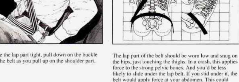
3. To make the lap part tight, pull down on the buckle end of the belt as you pull up on the shoulder part.
