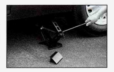
Lower the vehicle by rotating the jack handle counterclockwise. Lower the jack completely.
