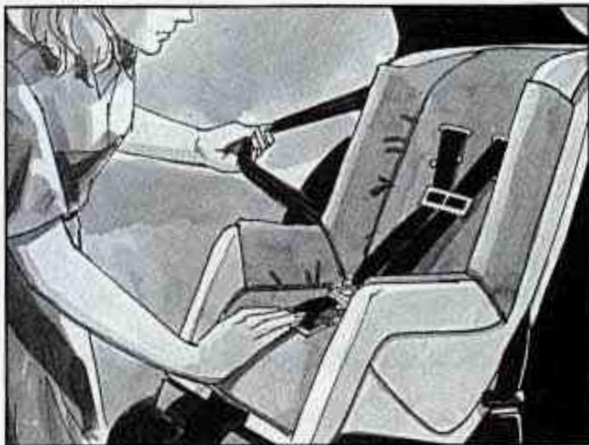
6. To tighten the belt, feed the shoulder belt into the retractor while you push down on the child restraint.
