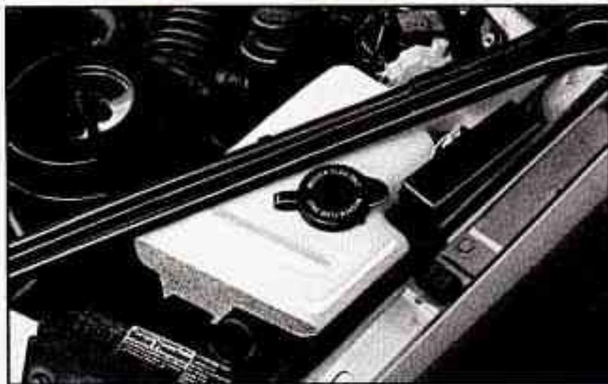
Open the cap labeled "WASHER FLUID ONLY." Add washer fluid until the bottle is full.
