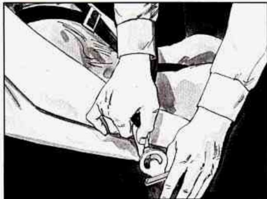
9. To make it tight, pull the belt while you push down on the child restraint. If the belt won't stay tight, switch it end for end.
