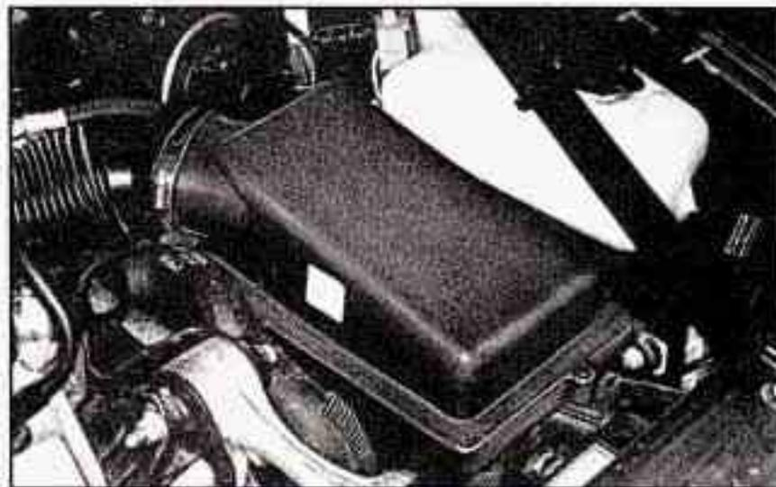
The air cleaner is in the right front area of the engine compartment.
