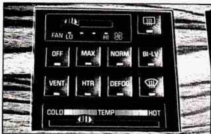
Fresh air from outside your vehicle flows through your Buick when the car is moving. When the vehicle is not moving, you can get outside air to flow through by selecting any air choice (except the rear window defogger) and the HI fan speed.
