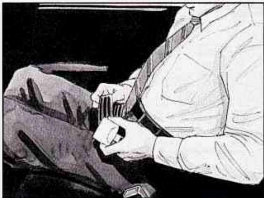
When you sit in a center seating position, you have a lap safety belt, which has no retractor. To make the belt longer, tilt the latch plate and pull it along the belt.
