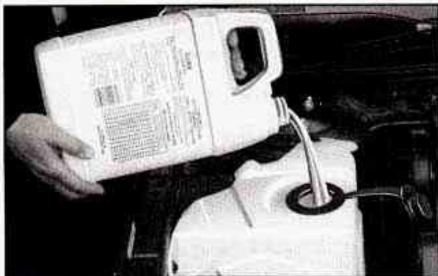
6. Then fill the coolant recovery tank to "COLD."
