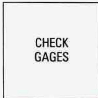
The "CHECK GAGES" light indicates that there is an engine or electrical problem. If the "TEMP," "OIL" or "VOLTS" gages read properly, there may still be an electrical problem which should be checked by your Buick dealer.
