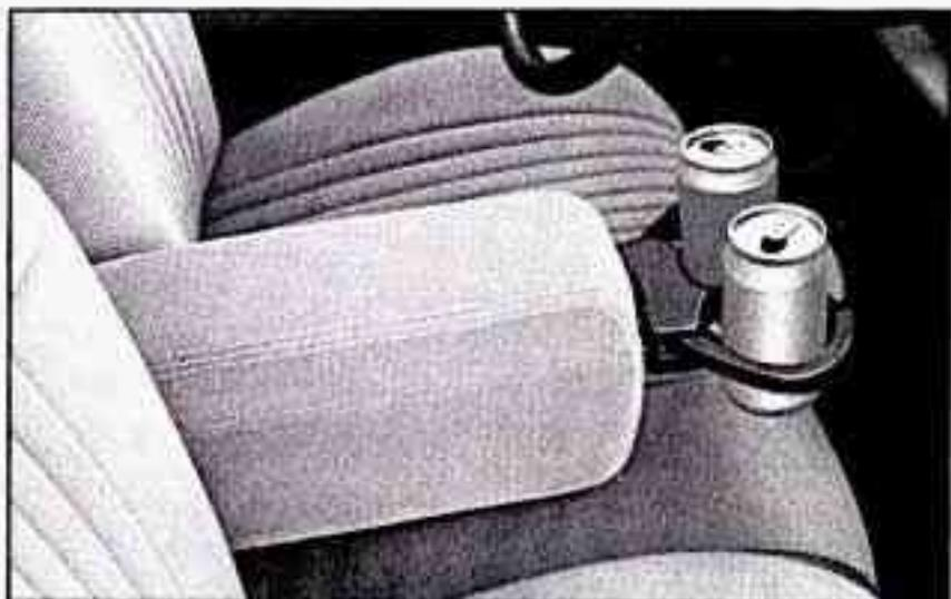
The armrest between the front seats opens into a storage area. To open it, press the lever at the front edge and lift the cover. To use the cupholder which is stored inside, pull it up and rotate it forward. You may have an adjustable cup holder.
