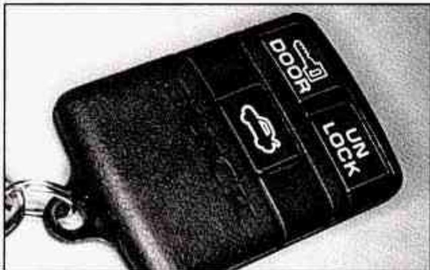
If your Buick has this option, you can lock and unlock your doors or unlock your trunk from up to 30 feet (9 m) away using the key chain transmitter supplied with your vehicle.
