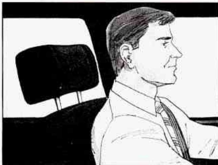
Slide the head restraint up or down so that the top of the restraint is closest to the top of your ears.
