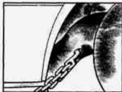
Attach "T" hook chains in front of the wheels into the side slots of the cradle on both sides.
