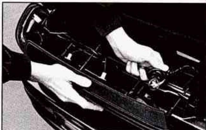
3. Squeeze the bulb socket and turn it 1/4 turn to detach it from the light.
