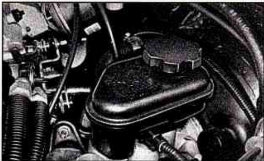
There are only two reasons why the brake fluid level in your master cylinder might go down. The first is that the brake fluid goes down to an acceptable level during normal brake lining wear. When new linings are put in, the fluid level goes back up. The other reason is that fluid is leaking out of the brake system. If it is, you should have your brake system fixed, since a leak means
