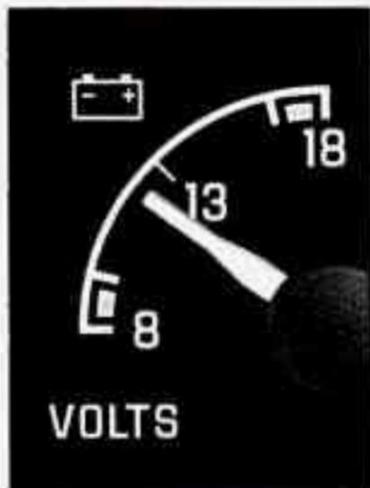
The "Volts" gage shows voltage in the electrical system. The normal range is 11 to 15 volts. If the gage reading stays in either red range, have your Buick dealer check the electrical system.
