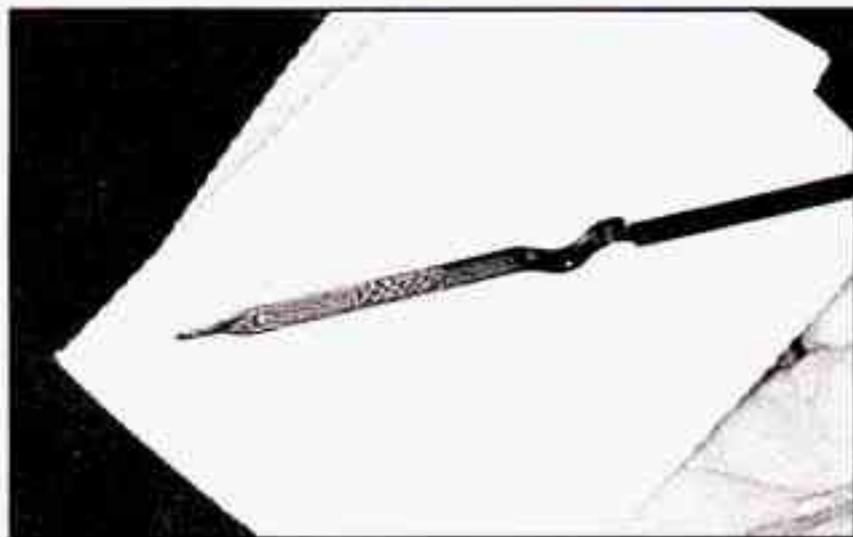
3. Check both sides of the dipstick, and read the lower level. The fluid level must be in the cross-hatched area.
