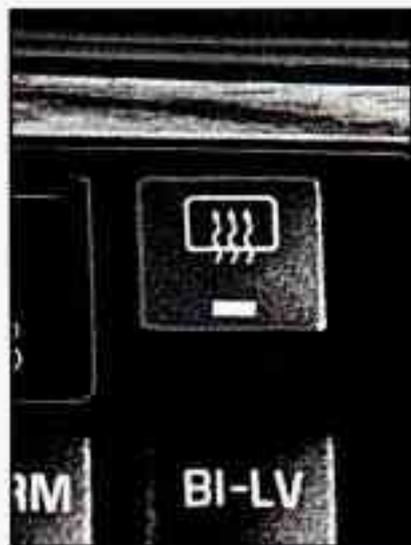
The lines you see on the rear window warm the glass. Press the button to start warming your window. After 10 minutes, it will go off by itself or pressing the button again during the heating cycle will shut it off. If you need additional warming time, push the button again, the defogger will go off after 5 minutes.
