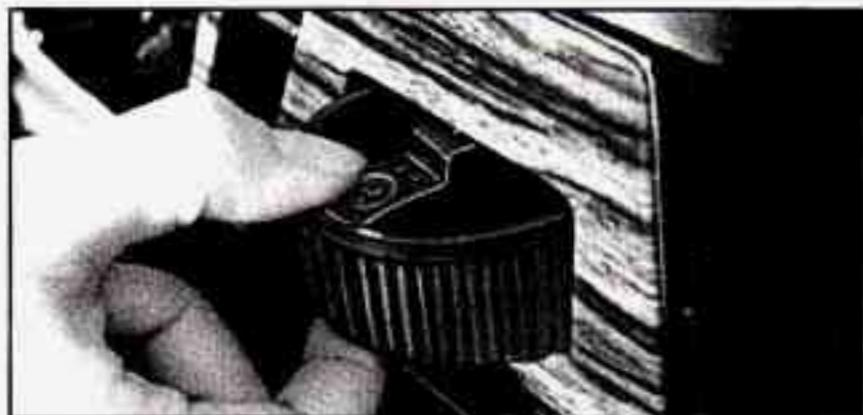
To remove the rear ashtray for cleaning, press down on the snuffer as you pull the ashtray down and out.
