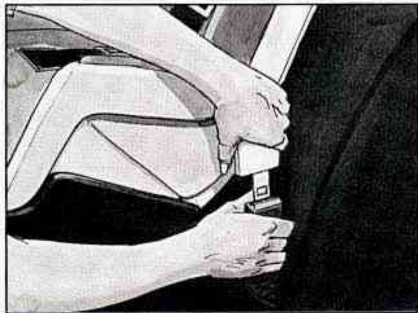
5. To tighten the belt, pull up on the shoulder belt while you push down on the child restraint.
