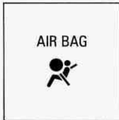
You will see this light flash for a few seconds when you turn your ignition to "Run" or "Start." Then the light should go out, which means the system is ready.
