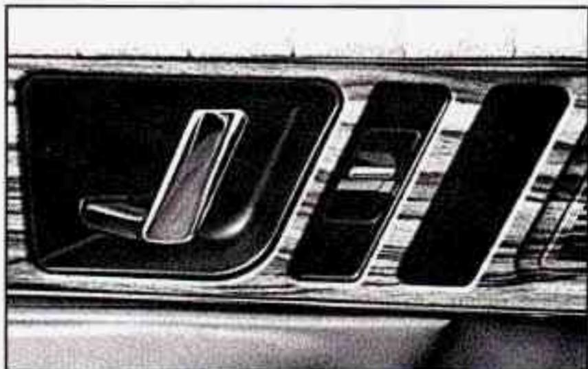
From the inside: To lock the door, move the lock control down.
