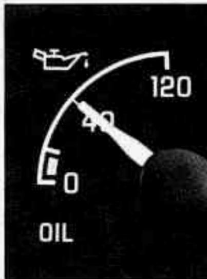
You can read your engine oil pressure directly from the gage on your instrument panel.
