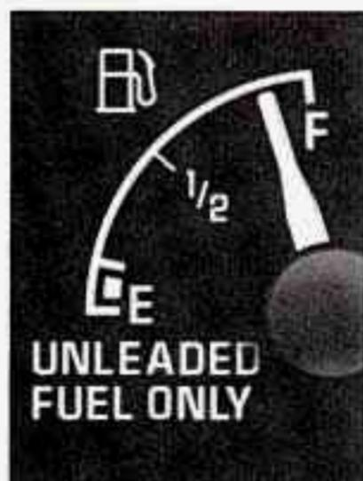
Your fuel gage shows about how much fuel is in your tank. It works only when the engine is on. When the indicator nears "E," you still have a little fuel left. You need to get more right away.
