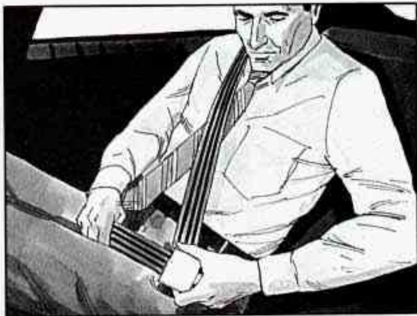
If the belt stops before it reaches the buckle, tilt the latch plate and keep pulling until you can buckle it.
