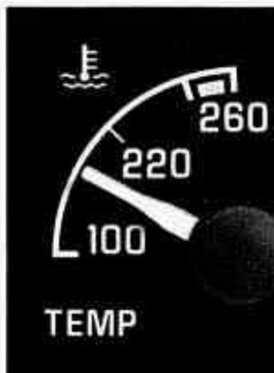
This gage shows the engine coolant temperature. If the gage pointer moves into the red area, your engine is too hot!
