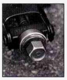
The jack has a bolt at the end. Attach the wheel wrench to the bolt to create a jack handle.
