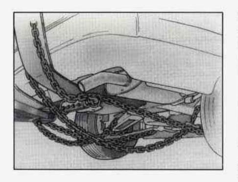
Position the lower sling crossbar directly under the rear bumper.
