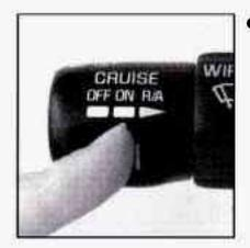
Move the cruise switch from ON to R/A. Hold it there until you reach a desired speed and then release the switch. To increase your speed in very small amounts, move the switch to R/A for less than half a second and then release it.
