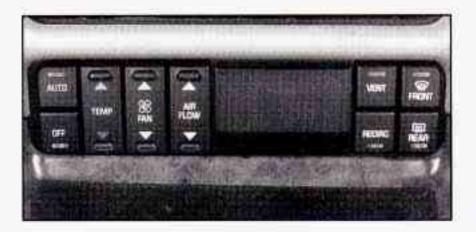
Sun and temperature sensors automatically adjust the air temperature, the airflow direction and the fan speed to maintain your comfort setting. The system may supply cooler air to the side toward the sun. Be careful not to put anything over the sensors on top of the dash.
