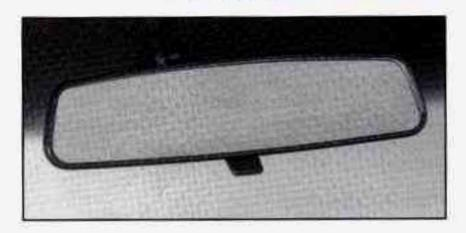
When you are sitting in a comfortable driving position, adjust the mirror so you can see clearly behind your vehicle. Grip the mirror in the center to move it up or down and side to side. The day/night adjustment allows you to adjust the mirror to avoid glare from the lamps behind you. Pull the tab forward for daytime use; push it back for night use.
