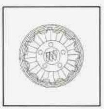
If your vehicle has this aluminum wheel, you may have plastic wheel nut caps. Use the wheel nut wrench to remove the wheel nut caps and to loosen the wheel nuts.
