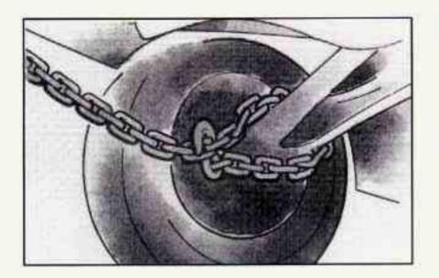
Attach a separate safety chain around the outboard end of each lower control arm.
