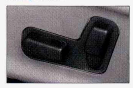
The front seatbacks can be adjusted by pressing the vertical control located on the side of the seat. Push it forward to bring the seat to a more upright position. Push it rearward to recline the seatback.
