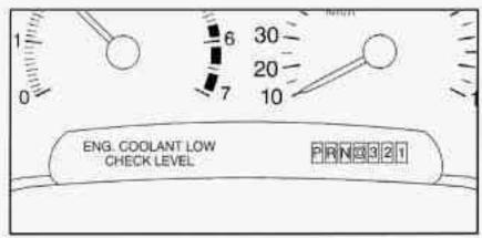
If this ENG. COOLANT LOW-CHECK LEVEL message comes on, it means you're low on engine coolant.
