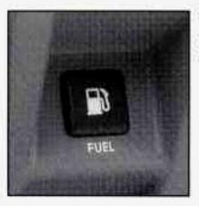
The release button for the fuel door is to the left of the steering column.
