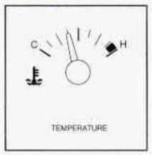
This gage measures the temperature of your engine. If the pointer moves into the red area, your engine is too hot. A temperature indicator light will turn on and a chime will sound.
