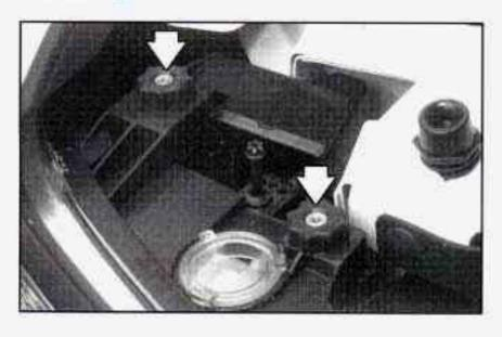
Each headlamp is attached by thumb screws.
