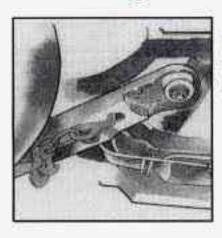
Attach T-hook chains behind the front wheels into the bottom slots of the cradle rails on both sides.
