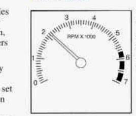
The tachometer tells you how fast the engine is running. It displays engine speed in thousands of revolutions per minute (rpm).
