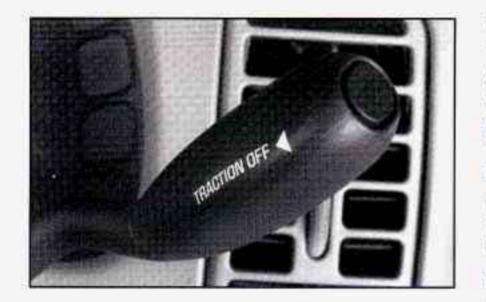
To turn the system off, press the button located at the end of the shift lever.
