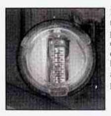
It is recommended that the upper limit not exceed plus 0.4 degrees from the center of the bubble. Other drivers may flash their high beams at you if your adjustment is much above plus 0.4 degrees.
