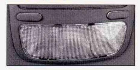
Turn on the front seat reading lamps by pressing the switch on the overhead console. Press the switch again to turn them off. The driver's switch controls the driver and center lamps. The passenger switch controls the passenger side lamp.
