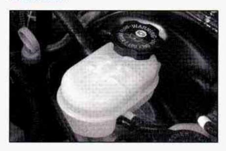
Your brake master cylinder reservoir is here. It is filled with DOT-3 brake fluid.
