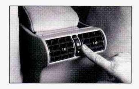
You have rear passenger comfortemp outlets that you can use to adjust the direction of the airflow to the rear seating area. The temperature is controlled by the front passenger setting.
