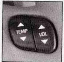
If your vehicle has this feature, you can control the temperature function by using the button on your steering wheel. Press the TEMP up arrow to increase the temperature and the TEMP down arrow to decrease the temperature.
