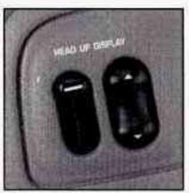
The HUD controls are located in the overhead console.
