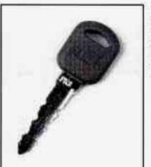
The valet key is used for the ignition and the two side doors only. It will not open the trunk or glove box. This is a theft-deterrent feature.
