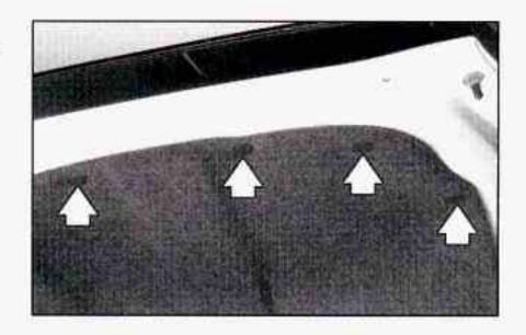
There are eight fasteners along the top of the trunk lid (four on each side), holding the trunk trim in place. Remove these fasteners.
