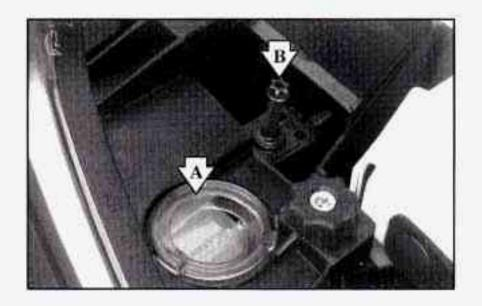
The headlamp aiming device is under the hood, directly behind the headlamps.
