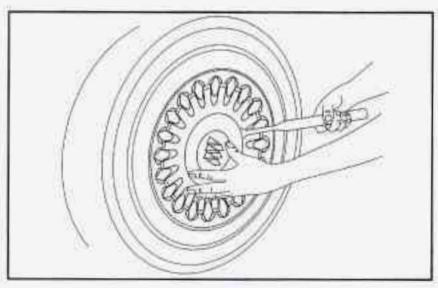
Insert the flat end of the wheel wrench in the notch and pry off the center cover. Do not drop the cover or lay it face down, as it could be scratched or damaged.
