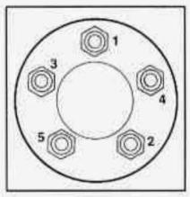
Using the wheel wrench, tighten the wheel nuts firmly in a crisscross sequence.
