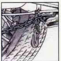
Attach T-hook chains on both sides in the slotted holes in the floor pan support rails just ahead of the rear wheels.
