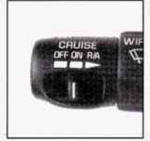
Move the cruise control. switch to ON.
