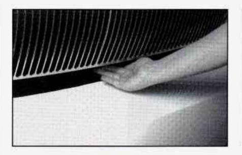
Then go to the front of the vehicle and locate the secondary hood release. It is under the front edge of the grille.
