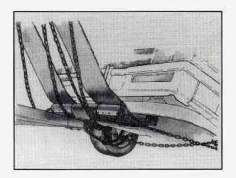
Position a 4" x 4" wood beam across the sling chains contacting the bottom of the radiator support. Position the lower sling crossbar just behind the rear edge of the front bumper.
