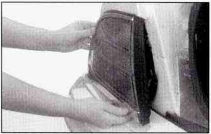
Beneath the trim panel are three nuts that secure the taillamp assembly. Remove these nuts with a 10 mm wrench. Remove the nuts from only the side you want to access. The turn signal and a stoplamp can now be accessed.
