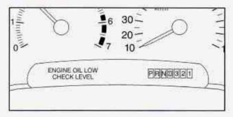
If you have the Driver Information Center, an ENGINE OIL LOW-CHECK LEVEL message will appear when the engine oil is approximately 1 quart (1L) low. If the message is displayed, check the dipstick level and add oil as needed.
