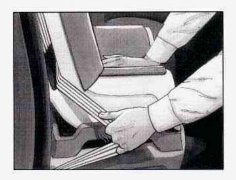
Pull the rest of the lap belt all the way out of the retractor to set the lock.
