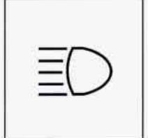
When the high beams are on, a light on the instrument panel will also be on. If your vehicle is equipped with HUD, this light will also appear in the display area.
