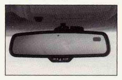
This mirror automatically changes to reduce glare when set in the M (Mirror) or C/M (Compass/Mirror) position.
