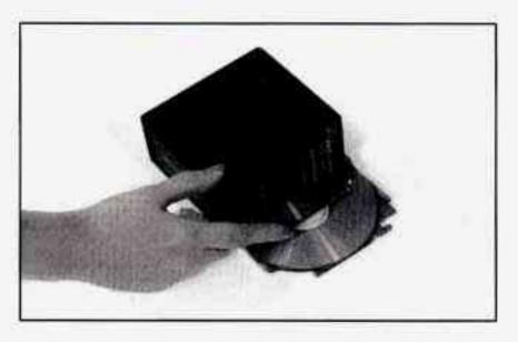
You must first load the magazine with discs before you can play a compact disc. Each of the 12 trays holds one disc. Press the button on the back of the magazine and pull gently on one of the trays. Load the trays from bottom to top, placing a disc on the tray label side down. If you load a disc with the label side up, the disc will not play and an error will occur. Gently push the tray back into the magazine slot. Repeat this procedure for loading up to 12 discs in the magazine.
