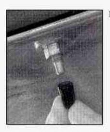
There are four studs located at the edge of the trunk lid. Remove the protective vinyl caps from the studs.
