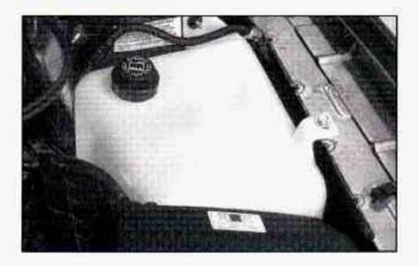
The coolant recovery tank is located on the driver's side of the engine compartment.
