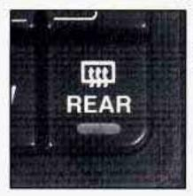
The lines you see on the rear window warm the glass. Press this button to start warming your window. At speeds above 30 mph (48 km/h), the rear defogger will stay on until you press the REAR button again. After 10 minutes of driving below 30 mph (48 km/h), the defogger will turn off automatically. If you need additional warming time, push the button again. The system will then operate for five minutes before going off by itself.
