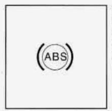
With the anti-lock brake system, the light(s) will come on when you start your engine and may stay on for several seconds. That's normal.
