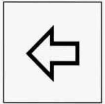
An arrow on the instrument panel will flash in the direction of the turn or lane change. If your vehicle is equipped with the Head-Up Display (HUD), an arrow will also appear in the display area to indicate the direction of the turn or lane change.
