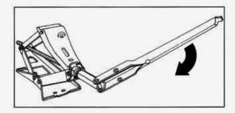
Rotate the wheel wrench clockwise (to the right) to lower the jack head a few inches.
