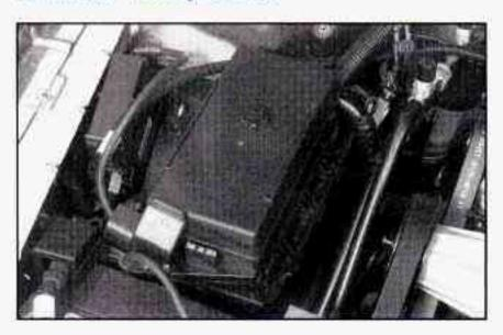
To check the fuses in this underhood fuse center, turn the knob counterclockwise and remove the cover. There is a chart inside the cover that explains the features and controls governed by each fuse and relay.
