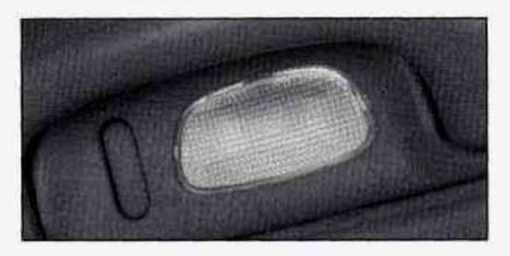
To turn on the rear seat reading lamp, press the switch above that rear door. To turn off the lamp, press the switch again.
