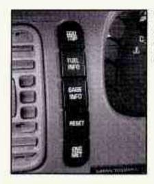
The following buttons are on the DIC control panel which is located to the left of the steering column:
