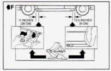
4. Near each wheel well is a notch in the plastic trim panel to position the jack head. You'll find the word JACK and an arrow stamped into the plastic near each notch. Position the jack under the vehicle and raise the jack head until it fits firmly against the sheet metal next to the word JACK. Do not raise the vehicle yet. Put the compact spare tire near you.
