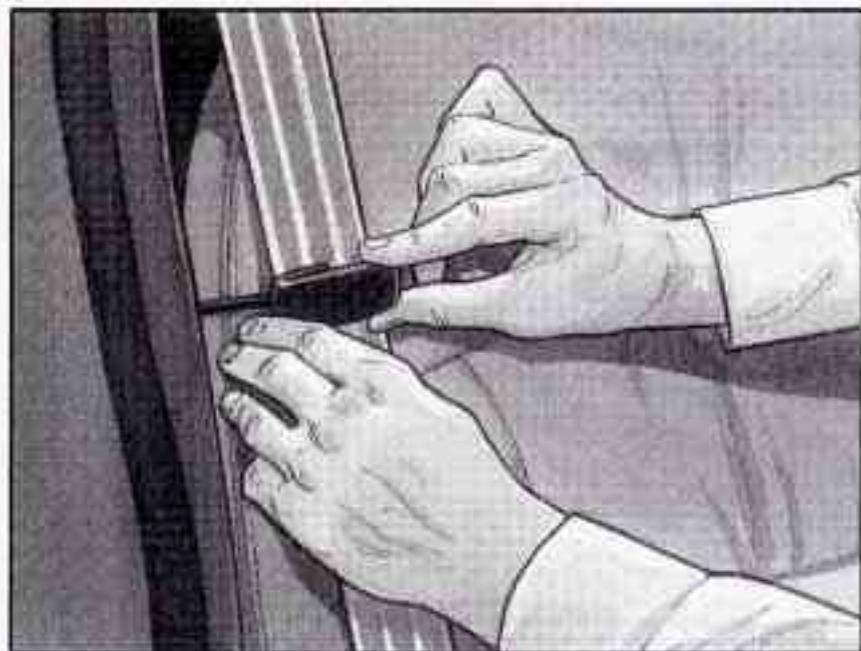
2. Slide the guide under and past the belt. The elastic cord must be under the belt. Then, place the guide over the belt, and insert the two edges of the belt into the slots of the guide.
