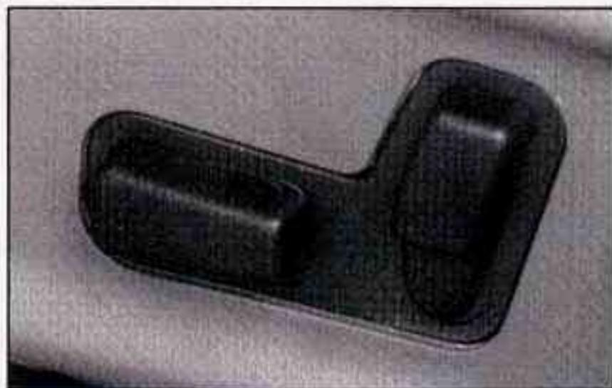
The front seatbacks can be adjusted by pressing the vertical control located on the side of the seat. Push it forward to bring the seat to a more upright position. Push it rearward to recline the seatback.
