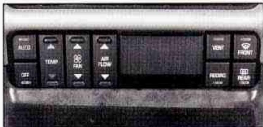
Sun and temperature sensors automatically adjust the air temperature, the airflow direction and the fan speed to maintain your comfort setting. The system may supply cooler air to the side toward the sun. Be careful not to put anything over the sensors on top of the dash.
