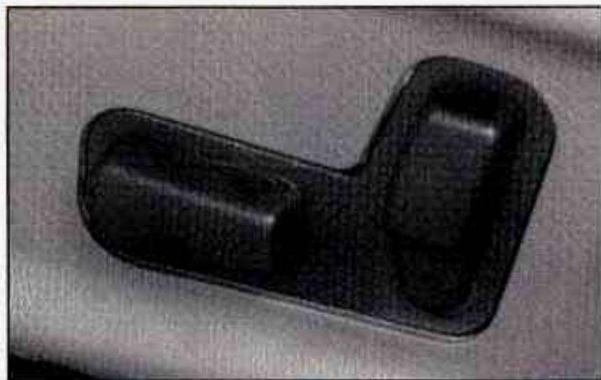
Use the vertical switch to move a front head restraint up or down. Lift up on the switch to move the head restraint up. Press down on the switch to move the head restraint down. The top of the head restraint should be closest to the top of your ears. This position helps reduce the chance of a neck injury in a crash. When you move a front seat head restraint up or down, the shoulder belt height changes. On some models, the head restraints tilt forward and rearward also.
