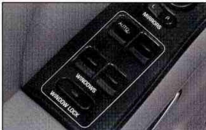
Switches on the driver's armrest control each of the windows while the ignition is on or retained accessory power is active. In addition, each passenger door has a switch for its own window:
