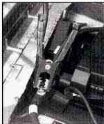
9. Now connect the black negative (-) cable to the good battery's negative (-) terminal. Don't let the other end touch anything until the next step. The other end of the negative cable *doesn't* go to the dead battery. It goes to a heavy unpainted metal part on the engine of the vehicle with the dead battery.
