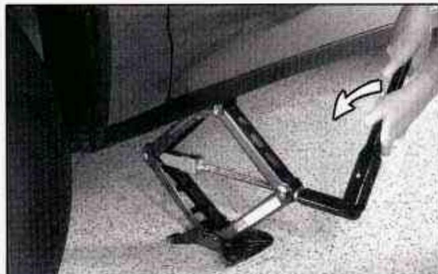
9. Lower the vehicle by rotating the wheel wrench counterclockwise. Lower the jack completely.
