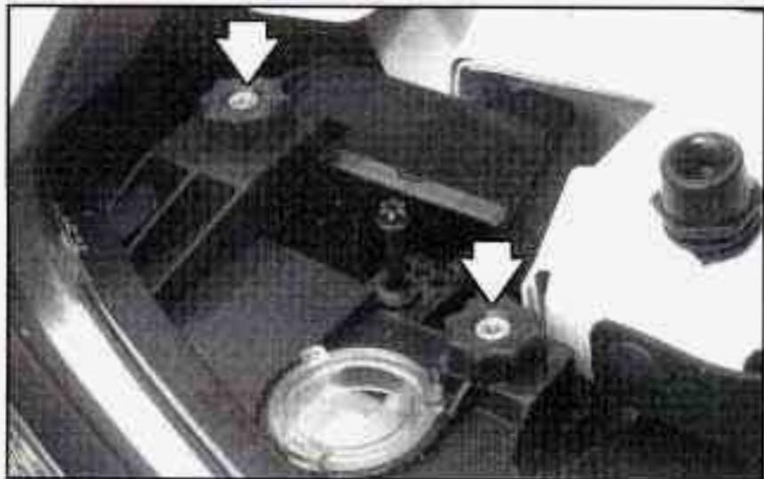
Each headlamp is attached by thumb screws.
