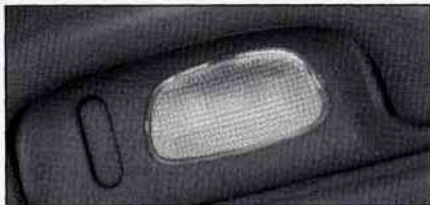
To turn on the rear seat reading lamp, press the switch above that rear door. To turn off the lamp, press the switch again.
