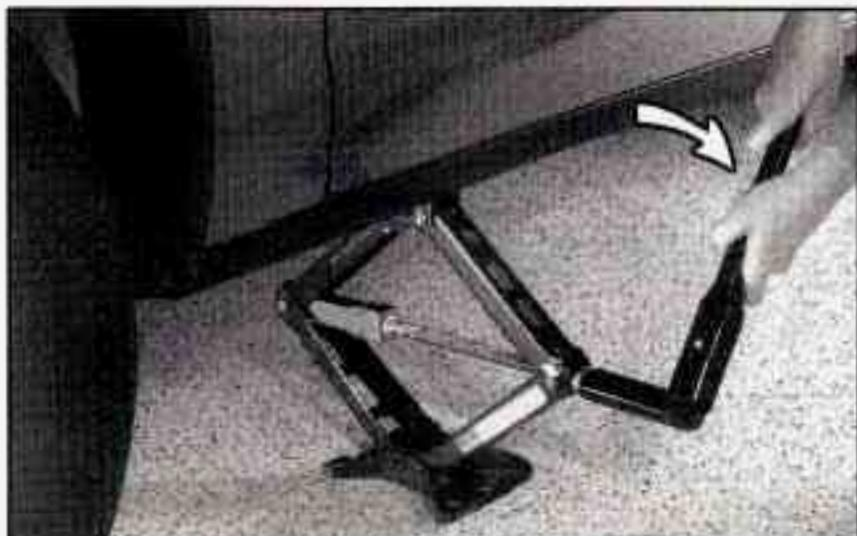
5. Raise the vehicle by rotating the wheel wrench clockwise in the jack. Raise the vehicle far enough off the ground so there is enough room for the spare tire to fit.
