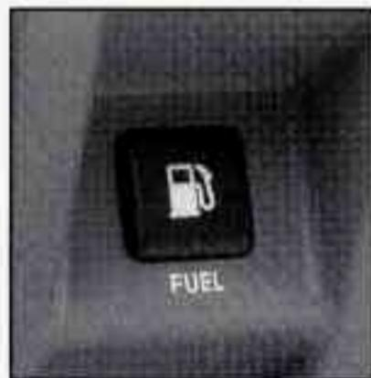
The release button for the fuel door is to the left of the steering column.
