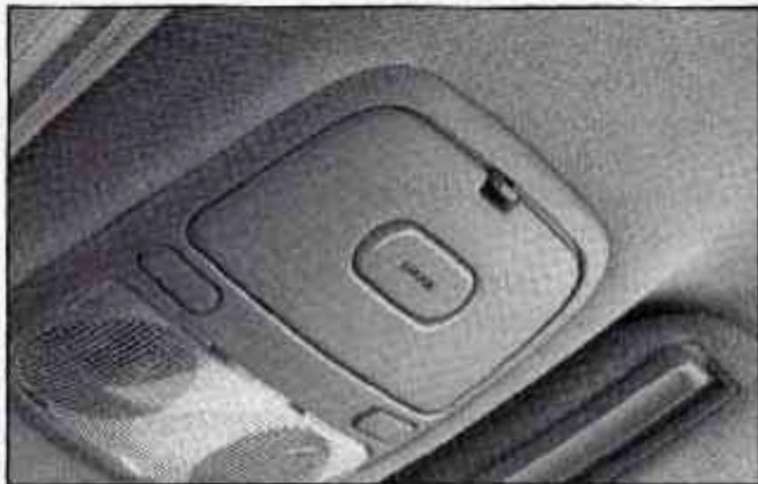
The garage door opener storage area is located in the headliner near the reading lamps. The following chart and instructions will help you install your garage door opener in the overhead storage area.
