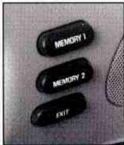
You can use this memory function to save your seat cushion (minus the head restraint), optional lumbar, mirror adjustment, HVAC and radio settings by using the following procedure:
