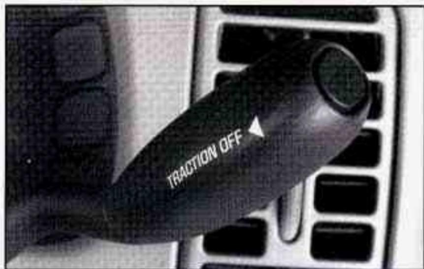
To turn the system off, press the button located at the end of the shift lever.
