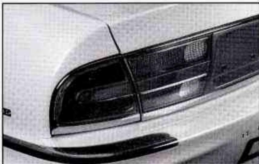
Turn lamps, stoplamps, and back-up bulbs are located behind the taillamp assembly along the trunk lid.
