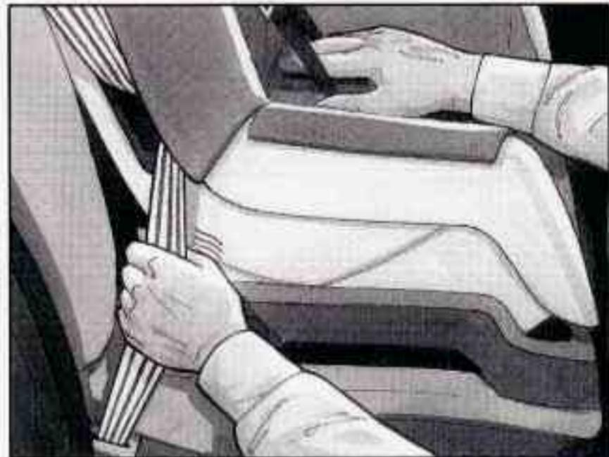
7. To tighten the belt, feed the lap belt back into the retractor while you push down on the child restraint.
