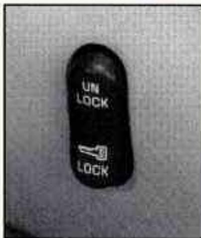
With power door locks, you can lock or unlock all doors of your vehicle by using either the driver or front passenger power door lock switch.
