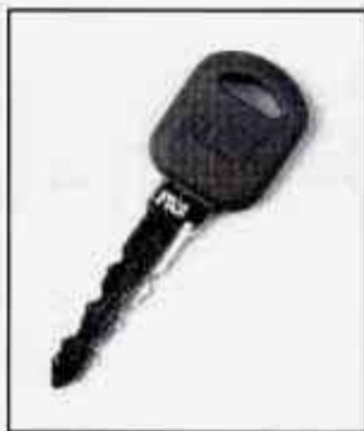
The valet key is used for the ignition and the two side doors only. It will not open the trunk or glove box. This is a theft-deterrent feature.
