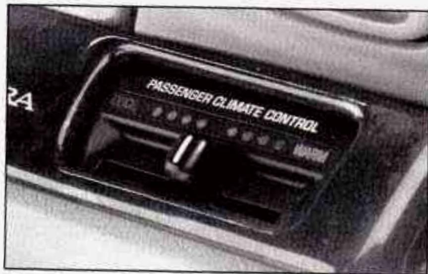
The front seat passenger can control the air temperature in their seating area. This can be set up to 5° F (-15°C) cooler or warmer than the primary setting. You can activate this feature by sliding the lever located on the instrument panel toward warm or cool.
