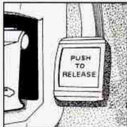
Your Park Avenue has a **PUSH TO RELEASE** parking brake pedal. To set the parking brake, hold the regular brake pedal down with your right foot. Push down the parking brake pedal with your left foot.
