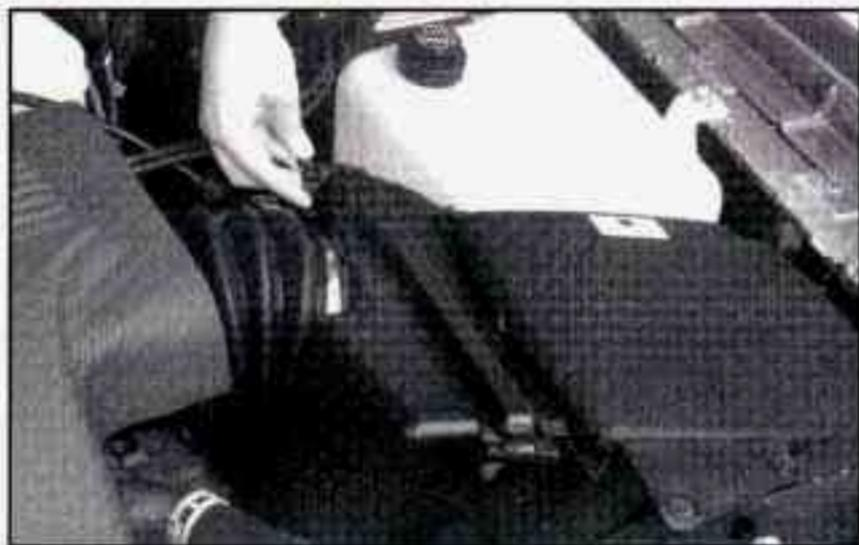
1. Remove the wing nuts on the air cleaner housing cover.
