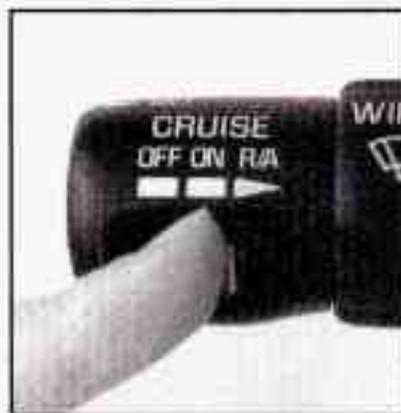
Once you're going about 25 mph (40 km/h) or more, you can move the cruise control switch from ON to R/A (Resume/Accelerate) for about half a second to reset. This returns you to your desired preset speed.
