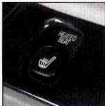
The heated seat controls are located next to the climate controls on the instrument panel. Press this button to turn on the heating element in the seat.
