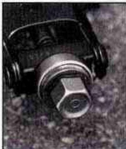
2. The jack has a bolt at the end. Attach the wheel wrench to the bolt to create a jack handle.
