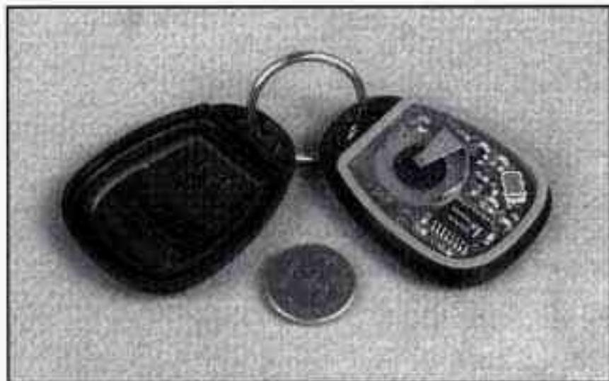
For battery replacement, use a Duracell<sup>®</sup> battery, type DL-2032, or a similar type.
