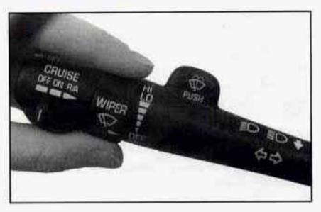
You control the windshield wipers by turning the band marked WIPER. For a single wiping cycle, turn the band to MIST. Hold it there until the wipers start, then let go. The wipers will stop after one cycle. If you want more cycles, hold the band on MIST longer. For steady wiping at low speed, turn the band to LO. For high-speed wiping, turn the band further, to HI. To stop the wipers, turn the band to OFF.
