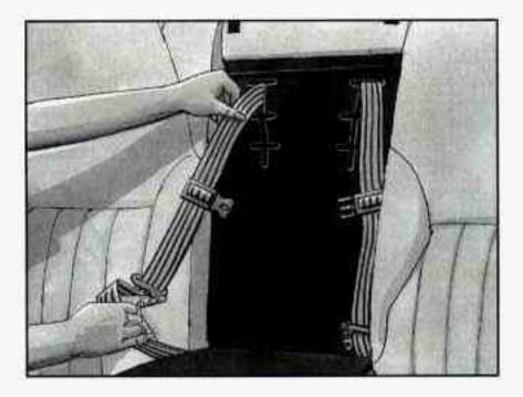
Move the harness up or down to the correct slot. The correct slot is the one that will be at or just above the top of the child's shoulder.
