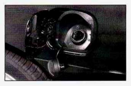
While refueling, let the cap hang by the tether below the fuel fill opening.
