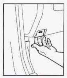
To open the hood, first pull the handle inside the vehicle, located just below the instrument panel and to the left of the steering column.
