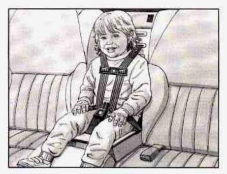
10. Adjust the position of the harness on the child's shoulders by moving the clip up or down along the harness. On each side of the harness, the shoulder part should be centered on the child's shoulder. The harness should be away from the child's face and neck, but not falling off the child's shoulders. Removing the Child from the Built-in Child Restraint
