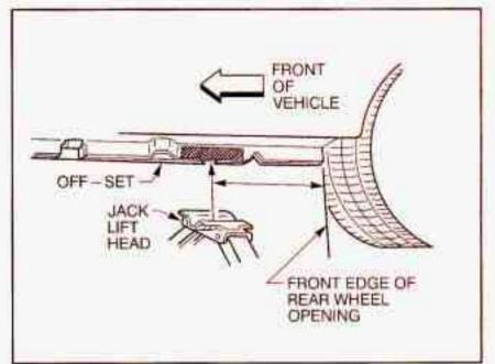
For jacking at the vehicle's rear location, put the jack lift head about 5 inches (13 cm) from the front edge of the rear wheel opening or just behind the off-set as shown.
