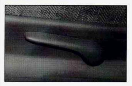
Lift the lever to release the seatback, then move the seatback to where you want it. Release the lever to lock the seatback into place. Pull up on the lever without pushing on the seatback and the seatback will move forward.
