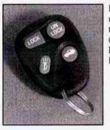
Press UNLOCK once to unlock the driver's door and to turn on the interior lamps (see "Illumination on Remote Activation" in the Index for more details).
