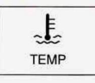
This light tells you that your engine coolant has overheated or your radiator cooling fan is not working.
