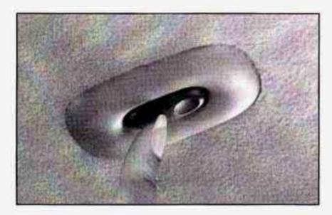
To open the astroroof, push the rear of the switch once and the astroroof will open to the vent position only. You will need to open the sunshade by hand.
