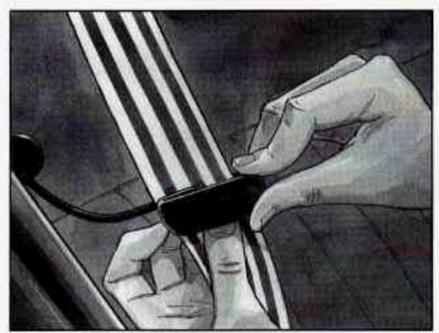
Slide the guide under and past the belt. The elastic cord must be under the belt. Then, place the guide over the belt, and insert the two edges of the belt into the slots of the guide.
