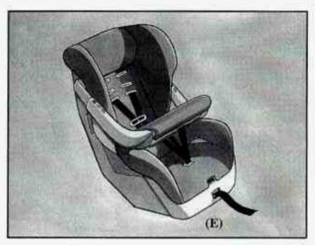
A forward-facing child restraint (C-E) positions a child upright to face forward in the vehicle. These forward-facing restraints are designed to help protect children who are from 20 to 40 lbs. (9 to 18 kg) and about 26 to 40 inches (66 to 102 cm) in height, or up to around four years of age. One type, a convertible restraint, is designed to be used either as a rear-facing infant seat or a forward-facing child seat.
