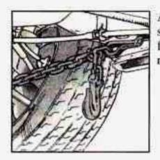
Attach T-hook chains into slots in the bottom of the floor pan, just ahead of the rear wheels, on both sides.
