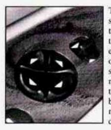
The power mirror control switches are located near the driver's side window, on the armrest. To choose either the left or right outside mirror, move the top switch from left through neutral to right. Press any of the four buttons located below the top switch to move the mirrors in the desired direction.
