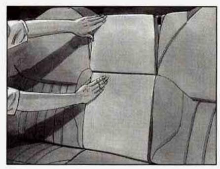
Then press the leg rest firmly into the seatback, and secure it by pressing the upper corners against the fastener strips on the seatback.
