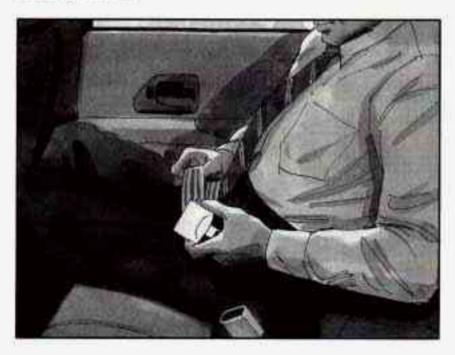
When you sit in a center seating position, you have a lap safety belt, which has no retractor. To make the belt longer, tilt the latch plate and pull it along the belt.
