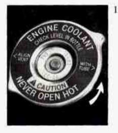
You can remove the radiator pressure cap when the cooling system, including the radiator pressure cap and upper radiator hose, is no longer hot. Turn the pressure cap slowly counterclockwise until it first stops. (Don't press down while turning the pressure cap.)
