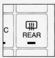
The rear window defogger uses a warming grid to remove fog from the rear window. Press the button to turn the rear defogger on. It will turn itself off after about 10 minutes. The picture above on the left refers to the defogger button that is found on a Manual Single Zone Climate Control System or Dual ComforTemp Climate Control System; the button on the right is found on the Dual Automatic ComforTemp System.
