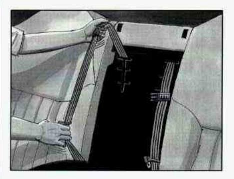
Select one side of the harness. Add some slack to the shoulder part by pulling up on the lap part. You'll keep most of this slack until you finish Step 9.
