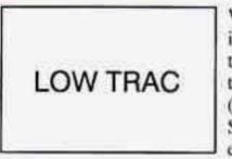
When your anti-lock system is adjusting brake pressure to help avoid a braking skid, this light will come on. (Also see "Anti-Lock Brake System Active Light" earlier in this section.)
