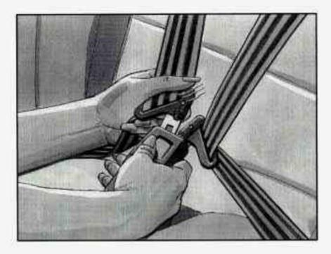
If the lap-shoulder harness is buckled, unlatch it by pushing the button on the buckle.
