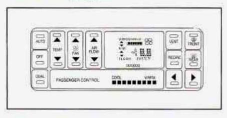
With this system, you set a temperature. You can then either let the system automatically control airflow direction and force to maintain the temperature, or you can manually adjust it. The system works best if you keep your windows closed while using it.
