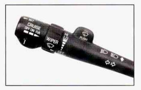
With cruise control, you can maintain a speed of about 25 mph (40 km/h) or more without keeping your foot on the accelerator. This can really help on long trips. Cruise control does not work at speeds below about 25 mph (40 km/h).
