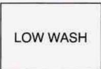
The LOW WASH light on your instrument panel cluster will glow when the fluid level is low.
