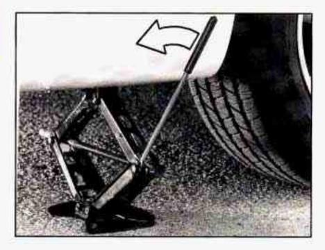
Lower the vehicle by turning the jack handle to the left. Lower the jack completely.
