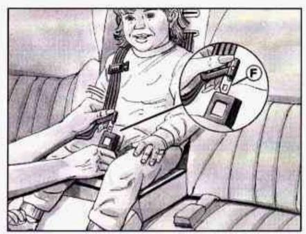
Select only one side of the harness. Pull the lap part of the harness out, and place the harness over the child's shoulder.
