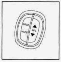
**SRCE:** Press this button to change to the cassette tape, compact disc function or return to playing the radio.
