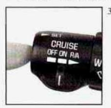
Push in the SET/COAST button at the end of the lever and release it. The CRUISE light on the instrument panel will come on.
