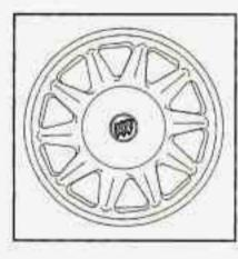
To remove a center cap, use the wrench to pry gently at the notch. Don't use a tool that is narrower than the wrench to pry at this notch. Then pry off the cap. They won't come off. You will only be able to loosen them. Once you have loosened the plastic nut caps with the wheel wrench, if needed, you can finish loosening them with your fingers.
