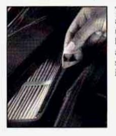
The passenger compartment air filter is located underneath your hood just below the windshield wiper arm on the car's passenger side (underneath the air inlet grille).
