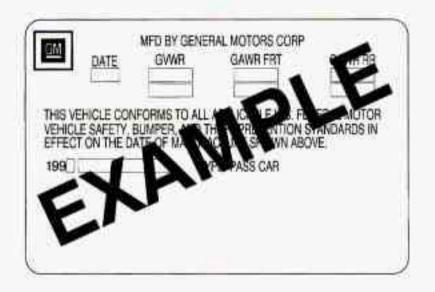
The other label is the Certification label, found on the rear edge of the driver's door. It tells you the gross weight capacity of your vehicle, called the Gross Vehicle Weight Rating (GVWR). The GVWR includes the weight of the vehicle, all occupants, fuel and cargo. Never exceed the GVWR for your vehicle or the Gross Axle Weight Rating (GAWR) for either the front or rear axle.
