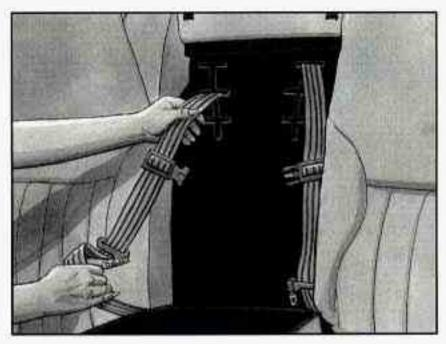
Twist the harness slightly to route it through the correct slot.
