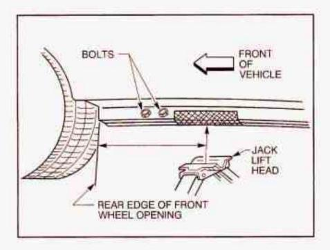
For jacking at the vehicle's front location, put the jack lift head about 6 inches (15 cm) from the rear edge of the front wheel opening or just behind the two bolts as shown.
