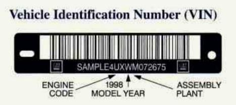
This is the legal identifier for your vehicle. It appears on a plate in the front corner of the instrument panel, on the driver's side. You can see it if you look through the windshield from outside your vehicle. The VIN also appears on the Vehicle Certification and Service Parts labels and the certificates of title and registration.
