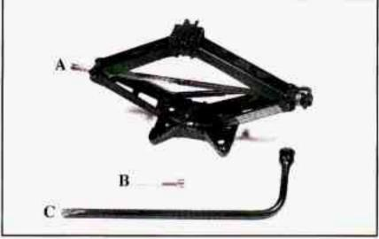
Turn the nut holding the jack to the left and remove it. Then remove the jack and wrench. The tools you'll be using include the jack (A), extension and protection guide (B) and wheel wrench (C).
