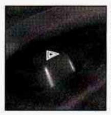
Press the switch on top of the steering column to make your front and rear turn signal lamps flash on and off. Your hazard warning flashers work no matter what position your key is in; they even work if the key isn't in the ignition.
