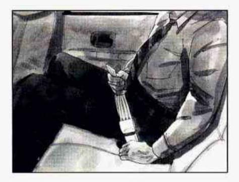
To make the belt shorter, pull its free end as shown until the belt is snug. Buckle, position and release it the same way as the lap part of a lap-shoulder belt. If the belt isn't long enough, see "Safety Belt Extender" at the end of this section.
