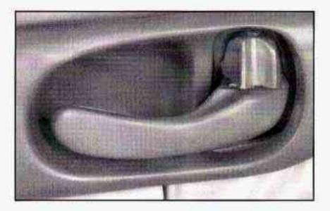
From the inside, to lock or unlock the door manually, push the lever forward to lock the door. To unlock, push the lever rearward.
