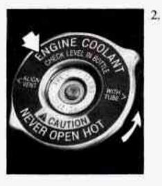
Then keep turning the pressure cap, but now push down as you turn it. Remove the pressure cap.
