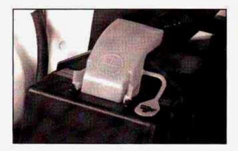
5. Find the positive (+) and negative (-) terminals on each battery. Your vehicle has a remote positive (+) jump starting terminal. The terminal is on the same side of the engine compartment as your battery. To uncover the remote positive (+) terminal, squeeze the sides of the red plastic cap and pull the cap upward. You should always use the remote positive (+) terminal instead of the positive (+) terminal on your battery.
