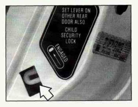
Your vehicle is equipped with rear-door child security locks that help prevent passengers from opening the rear doors of your vehicle from the inside. To use one of these locks:
