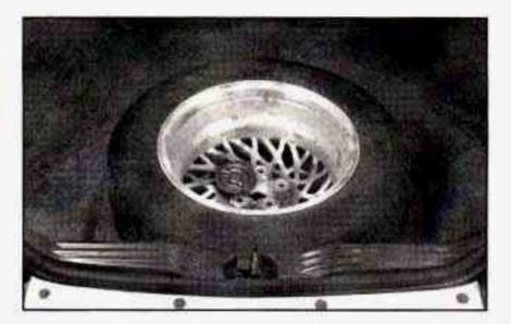
When reinstalling a compact spare tire, put the protector/guide back in the foam holder. Store the cover as far forward as possible.
