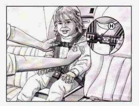
8. Now fasten the left and right halves of the shoulder harness clip together. The indicator window (H) on the clip will show green when the two halves are fastened together. The purpose of this clip is to help keep the harness positioned on the child's shoulders.
