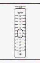
It is recommended that the upper limit not exceed plus 0.4 degrees from the center of the bubble. Other drivers may flash their high beams at you if your adjustment is much above plus 0.4 degrees. If you find that the headlamp aiming needs adjustment, follow these steps:
