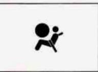
This light will come on when you start your engine, and it will flash for a few seconds. Then the light should go out. This means the system is ready.
