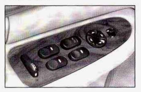
Switches on the driver's door armrest control each of the windows when the ignition is on. In addition, each passenger's door has a switch for its own window. The driver's window switch has an express-down feature. This switch is labeled AUTO. Tap the rear of the switch, and the driver's window will open a small amount. If the rear of the switch is pressed all the way down, the window will go all the way down.
