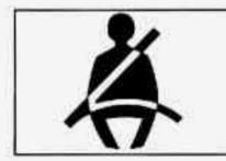
The safety belt light will also come on and stay on for about 20 seconds, then it will flash for about 55 seconds. If the driver's belt is already buckled, neither the chime nor the light will come on.
