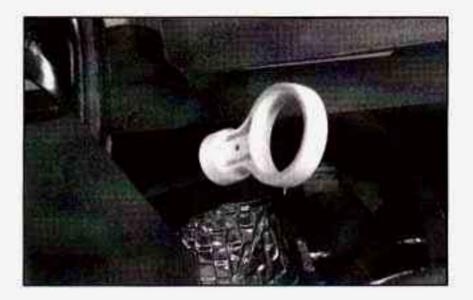
The engine oil dipstick handle is the yellow loop near the front of the engine.
