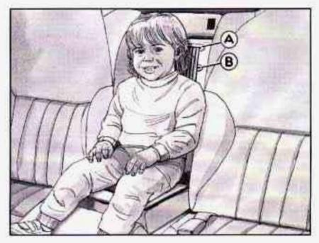
For the child shown here, the harness should go through the middle pair of slots (B).
