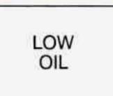
Your engine is equipped with an oil level monitoring system. When the ignition key is turned on, the LOW OIL light will come on briefly.
