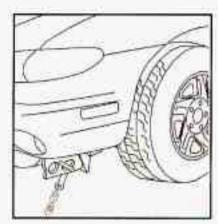
Attach T-hook chains in front of the wheels, into the slots of the front shipping brackets on the cradle (both sides). Insert the hook from the inward side of the slot and not the outward side.
