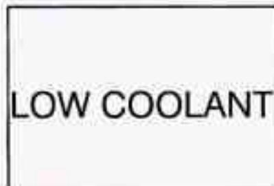
If this light comes on, your system is low on coolant and the engine may overheat. See "Engine Coolant" in the Index and have your vehicle serviced as soon as you can.
