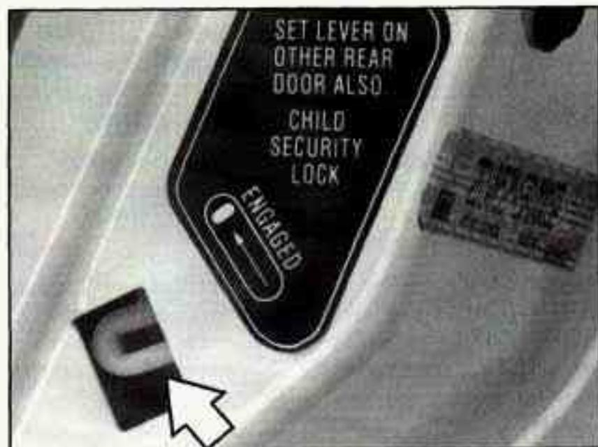
Your vehicle is equipped with rear-door child security locks that help prevent passengers from opening the rear doors of your vehicle from the inside. To use one of these locks:
