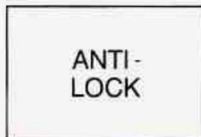
If there's a problem with the anti-lock brake system, this warning light will stay on or flash. See "Anti-Lock Brake System Warning Light" in the Index.
