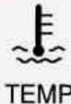
This light tells you that your engine coolant has overheated or your radiator cooling fan is not working.
