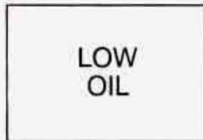
Your engine is equipped with an oil level monitoring system. When the ignition key is turned on, the LOW OIL light will come on briefly.
