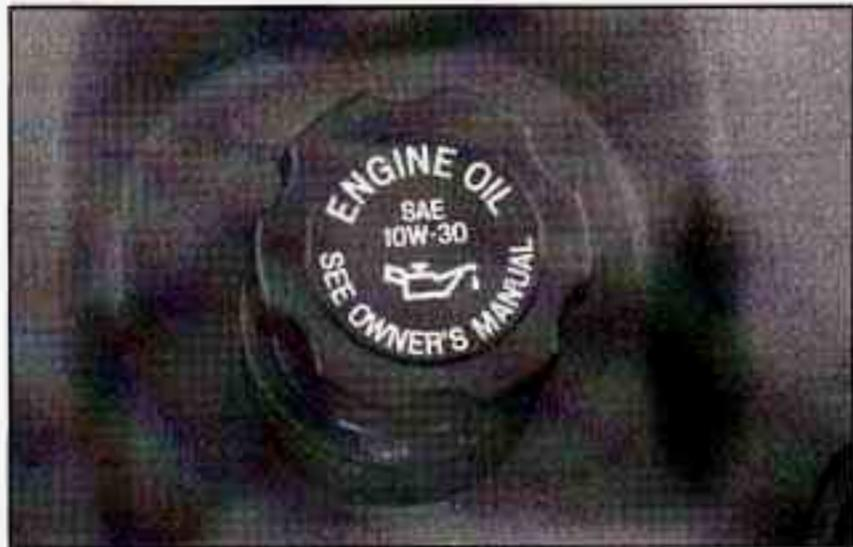
The engine oil fill cap is located toward the front of the engine near the yellow-looped engine oil dipstick handle.
