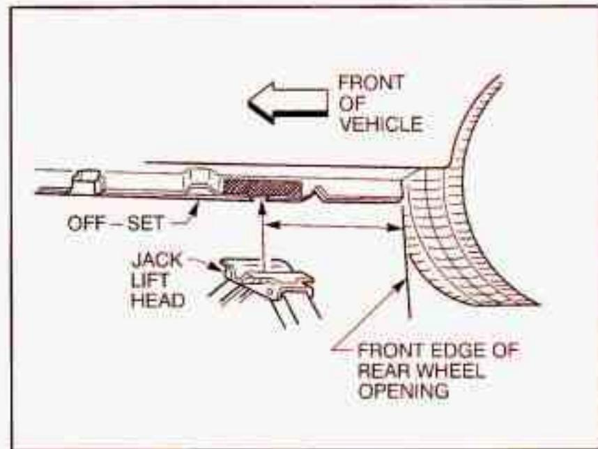
4. For jacking at the vehicle's rear location, put the jack lift head about 5 inches (13 cm) from the front edge of the rear wheel opening or just behind the off-set as shown.
