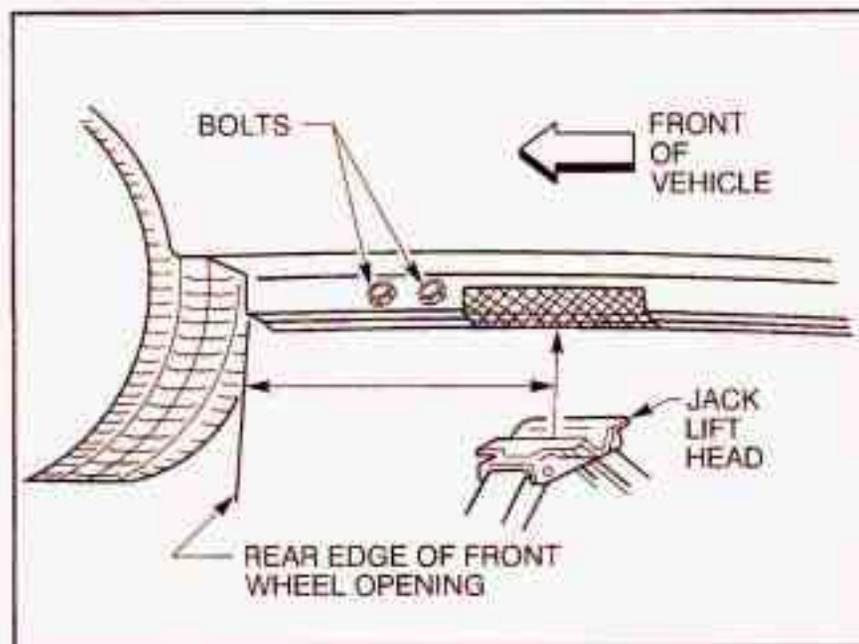
3. For jacking at the vehicle's front location, put the jack lift head about 6 inches (15 cm) from the rear edge of the front wheel opening or just behind the two bolts as shown.
