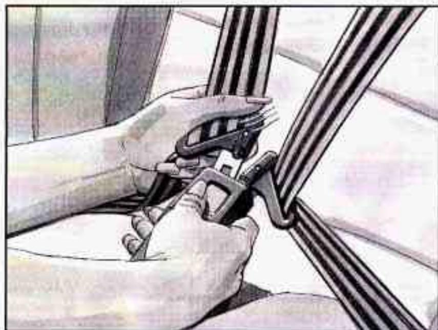
2. If the lap-shoulder harness is buckled, unlatch it by pushing the button on the buckle.
