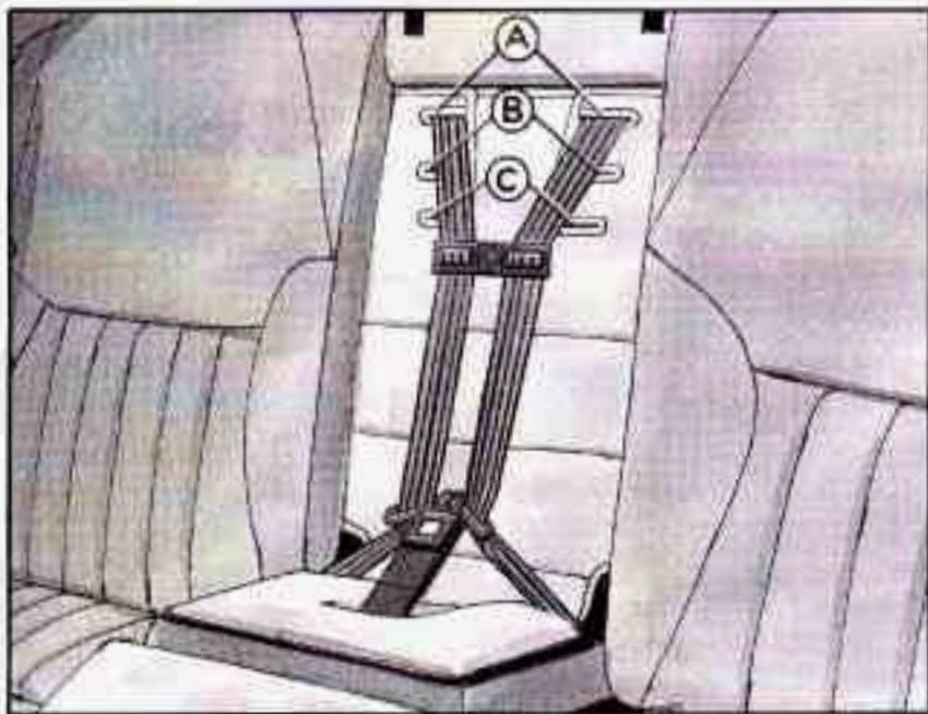
With this built-in child restraint, you can adjust the height of the harness. Depending on the seated height of the child, you can route it through the upper pair of slots (A), the middle pair of slots (B) or the lower pair of slots (C).
