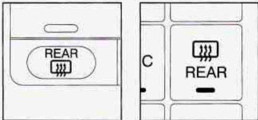
The rear window defogger uses a warming grid to remove fog from the rear window. Press the button to turn the rear defogger on. It will turn itself off after about 10 minutes. The picture above on the left refers to the defogger button that is found on a Manual Single Zone Climate Control System or Dual ComfortTemp Climate Control System; the button on the right is found on the Dual Automatic ComfortTemp System.
