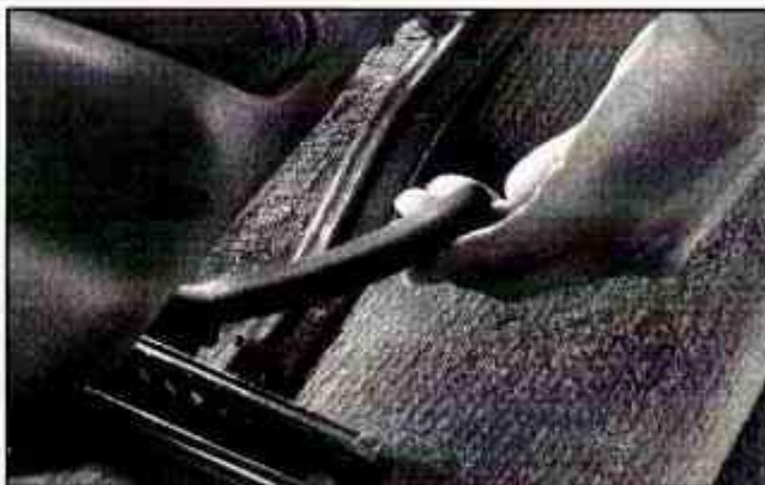
Lift the bar under the front of the seat using an upward motion. This will unlock the seat. Slide the seat to where you want it and release the bar. Try to move the seat with your body to be sure the seat is locked into place.
