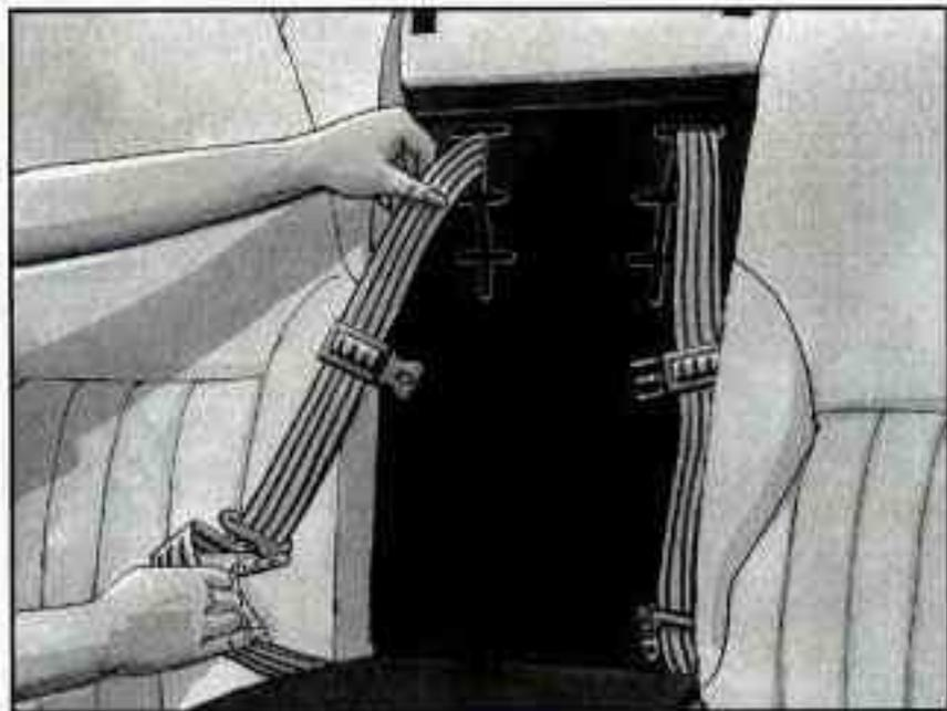
8. Move the harness up or down to the correct slot. The correct slot is the one that will be at or just above the top of the child's shoulder.
