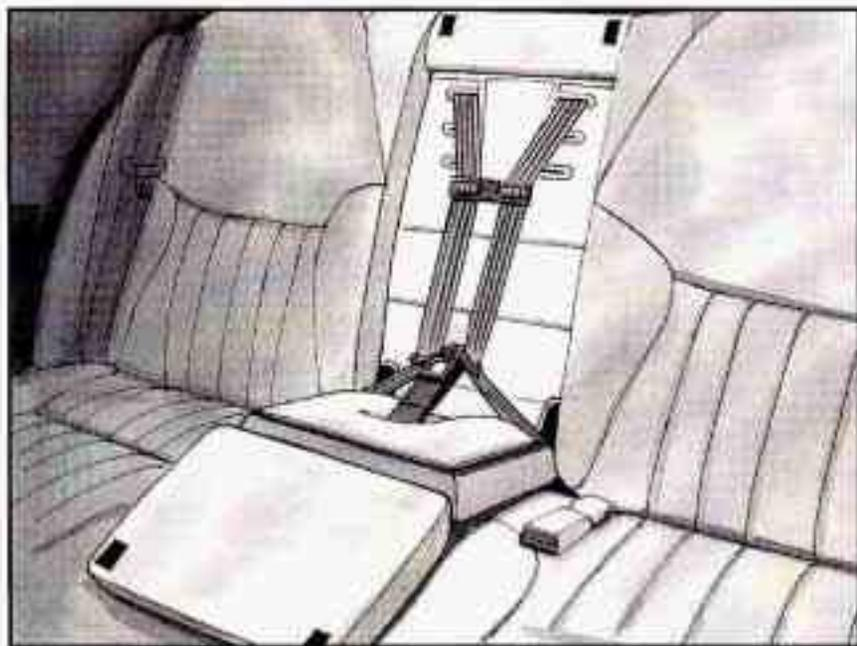
If your vehicle has this option, there's a built-in child restraint in the center rear seat position. This child restraint system conforms to all applicable Federal Motor Vehicle Safety Standards.
