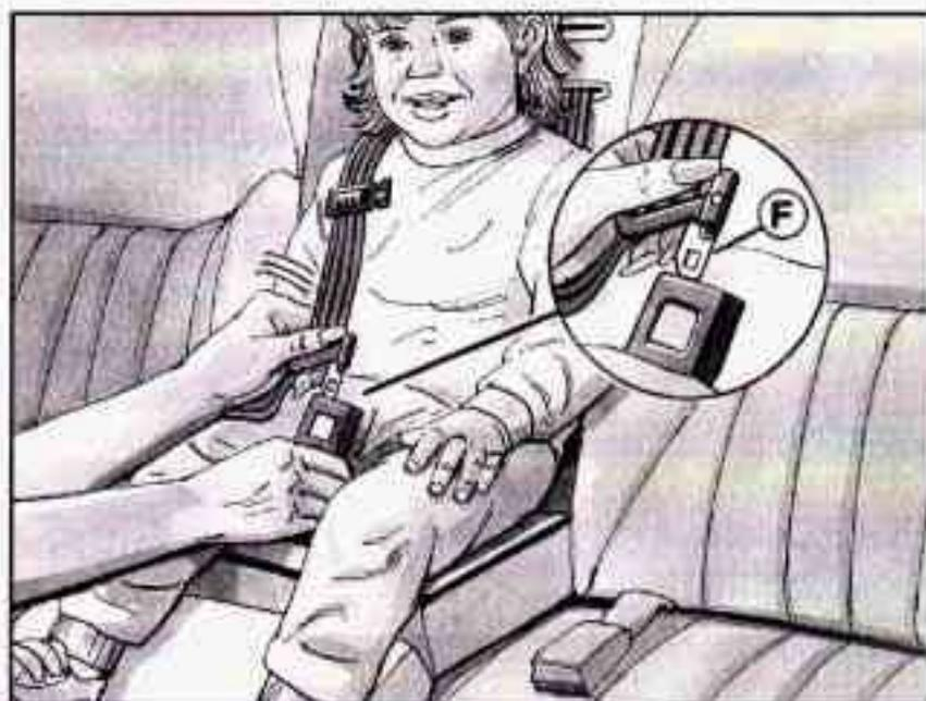
4. Select only one side of the harness. Pull the lap part of the harness out, and place the harness over the child's shoulder.
