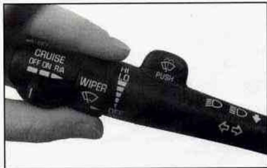
You control the windshield wipers by turning the band marked WIPER. For a single wiping cycle, turn the band to MIST. Hold it there until the wipers start, then let go. The wipers will stop after one cycle. If you want more cycles, hold the band on MIST longer.
