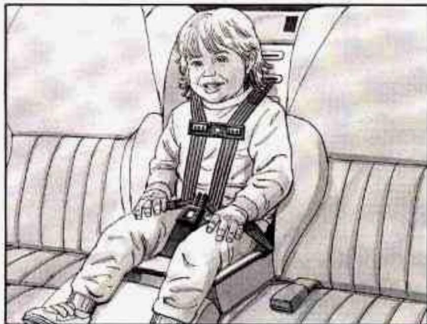
10. Adjust the position of the harness on the child's shoulders by moving the clip up or down along the harness. On each side of the harness, the shoulder part should be centered on the child's shoulder. The harness should be away from the child's face and neck, but not falling off the child's shoulders.
