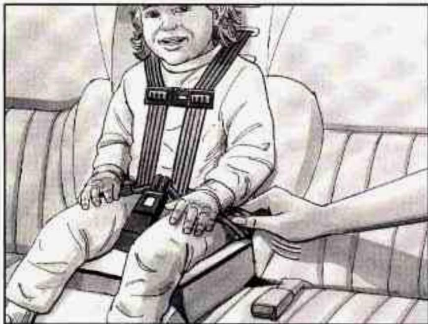
9. On both sides of the harness, pull up on the lap part a little to be sure it's locked.
