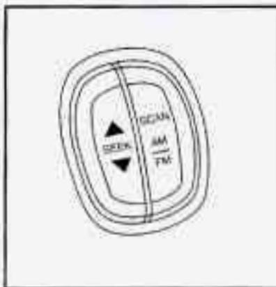
**SEEK:** Press the up or down arrow to tune to the next or previous radio station.
