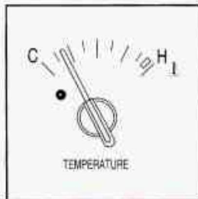
You have a gage that shows the engine coolant temperature. If the gage pointer moves into the red area, your engine is too hot!
