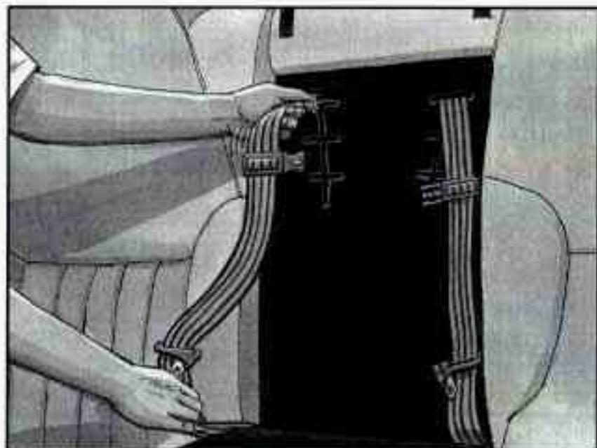
6. Feed a small amount of harness slack back into the slot.
