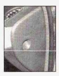
Some fuses are located in a fuse block on the passenger's side of the vehicle. Pull off the cover labeled FUSES to expose the fuses.
