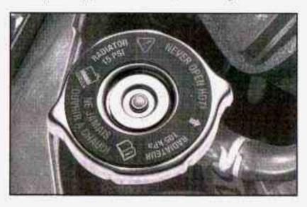
Turn the pressure cap slowly counterclockwise until it first stops. (Don't press down while turning the pressure cap.)
