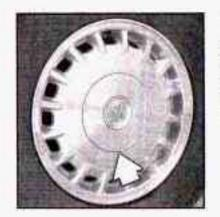
To remove a center cap, use the wrench to pry gently at the notch. Don't use a tool that is narrower than the wrench to pry at this notch. Then pry off the cap.
