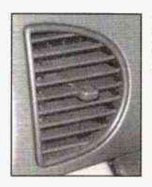
Open and close the air outlets, or adjust the direction of the airflow by moving the levers in the center of each outlet.
