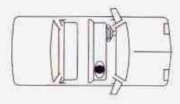
If your child restraint is equipped with the LATCH system, see Lower Anchorages and Top Tethers for Children (LATCH System) on page 1-42. Your vehicle has a right front passenger air bag. Never put a rear-facing child restraint in this seat. Here's why:
