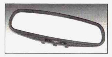
Your vehicle may have an automatic dimming rearview mirror. Push the button in the center of the mirror to turn this feature on. The mirror will darken gradually to reduce glare from headlamps behind you.
