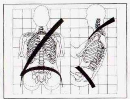
The lap part of the belt should be worn low and snug on the hips, just touching the thighs. In a crash this applies force to the strong pelvic bones. And you'd be less likely to slide under the lap belt. It you slid under it, the belt would apply force at your abdomen. This could cause serious or even fatal injuries. The shoulder belt should go over the shoulder and across the chest. These parts of the body are best able to take belt restraining forces.
