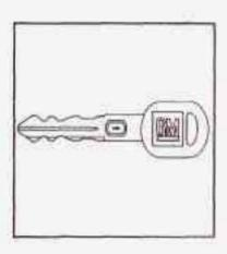
Your vehicle is equipped with the PASS-Key II (Personalized Automotive Security System) theft-deterrent system. PASS-Key II is a passive theft-deterrent system. It works when you insert or remove the key from the ignition.
