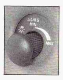
This control, located to the left of the instrument panel, operates the exterior lamps.
