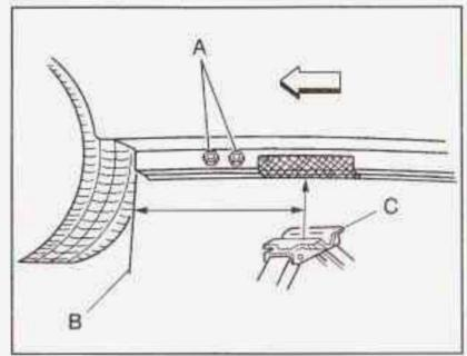
For jacking at the vehicle's front location, put the jack lift head (C) about 6 inches (15 cm) from the rear edge of the front wheel opening (B) or just behind the two bolts (A) as shown.
