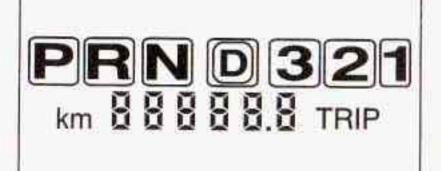
The graphic shown above is displayed on your instrument panel cluster and will indicate the gear your vehicle is in when you move.
