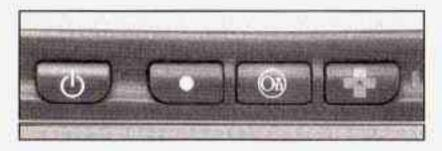
There are also three OnStar<sup>III</sup> buttons located at the bottom of the mirror. See your dealer for more information on the system and how to subscribe to OnStar<sup>III</sup>. See OnStar<sup>III</sup> System on page 2-35 for more information about the services OnStar<sup>IIII</sup> provides.
