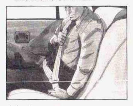
To make the lap part tight, pull down on the buckle end of the beit as you pull up on the shoulder part.
