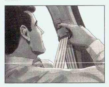
To move it down, squeeze the release lever and the shoulder belt guide as shown and move the height adjuster to the desired position. You can move the adjuster up just by pushing up on the shoulder belt guide. After you move the adjuster to where you want it, try to move it down without squeezing the release lever to make sure it has locked into position.
