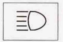
When the high beams are on this light, located on the instrument panel cluster, will also be on.
