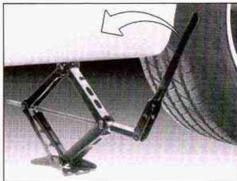
10. Lower the vehicle by turning the jack handle counterclockwise. Lower the jack completely.
