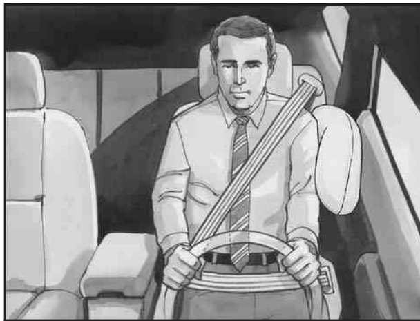
The driver's side impact air bag is in the side of the driver's seatback closest to the door.
