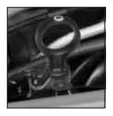
The automatic transaxle fluid dipstick handle is the black loop located toward the rear of the engine. See Engine Compartment Overview on page 5-12 for more information on location.
