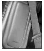
If your vehicle has a side impact airbag for the driver it will say AIR BAG on the airbag covering on the side of the driver's seatback closest to the door.
