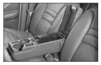
To use the storage area, fold down the armrest located in the center front seat. Press the latch on the front edge and pull up to access the storage area.
