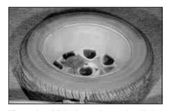
When storing a full-size tire, use the extension with the protector, located in the foam holder, to help avoid wheel surface damage. To store a full-size tire, place the tire valve stem facing down, and then remove the protector and attach the retainer securely. Store the cover as far forward as possible.
