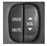
If your vehicle has this feature, some audio functions can be adjusted at the steering wheel. They include the following:
