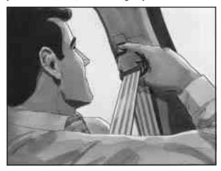
To move it down, squeeze the release lever and the shoulder belt guide as shown and move the height adjuster to the desired position. You can move the adjuster up just by pushing up on the shoulder belt guide.
