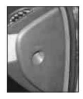
Some fuses are located in a fuse block on the passenger's side of the instrument panel. Pull off the cover labeled FUSES to expose the fuse block.
