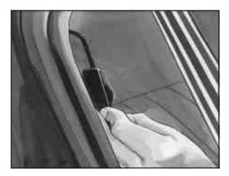
Pull the elastic cord out from between the edge of the seatback and the interior body to remove the guide from its storage clip.
