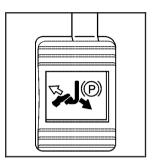
To set the parking brake, hold the regular brake pedal down with your right foot. Push down the parking brake pedal with your left foot.
