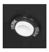
Press the remote trunk release button located behind the glove box door to release the trunk lid from inside the vehicle
