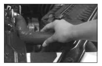
Start the engine and let it run until you can feel the upper radiator hose getting hot. Watch out for the engine cooling fans.
