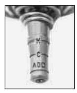
When the engine compartment is hot, the level should be at the H (hot) mark. When it is cold, the level should be at the C (cold) mark. If the fluid is at the ADD mark, fluid should be added.
