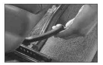
Lift the bar located under the front of the passenger's seat to unlock the seat. Slide the seat to the desired position and release the bar. Try to move the seat to be sure it is locked into place.
