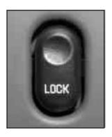
The vehicle has front power door lock switches. Press the top portion of a door lock switch to unlock or the bottom portion to lock all doors.
