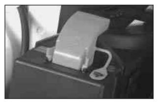
You will not need to access your battery for jump starting. Your vehicle has a remote positive (+) jump starting terminal for that purpose. The terminal is located on the same side of the engine compartment as your battery. See *Engine Compartment Overview on page 5-12* for more information on location
