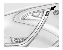
(Unlock): Press to unlock the doors.
