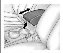
The armrest is adjustable. Lift the lever to move it forward or rearward.
