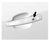
If equipped, use the Keyless Access system to lock and unlock the door. When the doors are locked and the Remote Keyless Entry (RKE) transmitter is within 1 m (3 ft) of the driver door handle, press the lock/ unlock button. When unlocking from the driver door, the first press unlocks that door; press again within five seconds to unlock all passenger doors.
