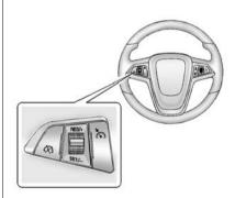
n (On/Off): Press to turn the cruise control system on or off. A white indicator comes in the instrument cluster when cruise is turned on
