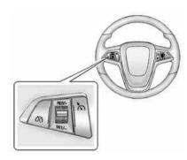
ৈ: Press to turn the cruise control system on or off. A white indicator comes in the instrument cluster when cruise is turned on.
