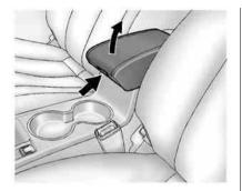
The armrest must be in the rearward position to open it. Lift the lever and then lift up on the armrest to access the storage area.
