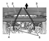
3. Place a 1.2 m (4 ft) X 102 mm (4 in) X 102 mm (4 in) wood beam (4) under the front cradle crossmember (3), and on top of both tow chains (5) to ensure the tow chains do not come into contact with the front fascia (1).
