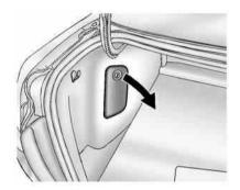
The rear compartment fuse block, if equipped, is on the left side of the trunk behind a cover.
