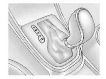
Move the shift lever from D (Drive) to the left into the (+) or (-) manual position.
