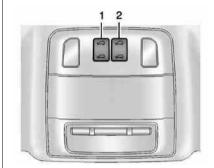
For vehicles with a sunroof, the sunroof only operates when the ignition is in ON/RUN or ACC/ACCESSORY, or in Retained Accessory Power (RAP). See Retained Accessory Power (RAP) on page 9-21.
