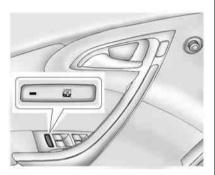
This feature prevents the rear passenger windows from operating, except from the driver position. This feature only works when the ignition is in ACC/ACCESSORY or ON/RUN, or in RAP.
