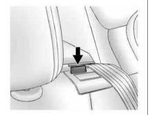
A tab near the seatback lever raises when the seatback is unlocked.
