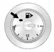
This light comes on for a few seconds when the ignition is turned on as a check to indicate it is working. If it does not come on, have it fixed.
