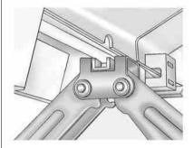
Make sure the jack lift head notch is placed in the flange notch.
