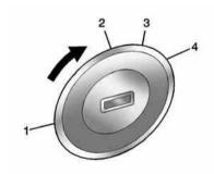
The ignition switch has four different positions.
