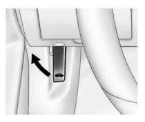
Pull up on the hood release handle. It is located inside the vehicle to the left of the steering column.
