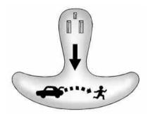
There is an emergency trunk release handle inside the trunk on the trunk lid. The release handle
