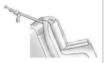
If you are using a single tether in the rear center seating position, route the single tether over the headrest
