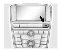
To open the trunk, press on the center stack or press and hold HOLD on the Remote Keyless Entry (RKE) transmitter.
