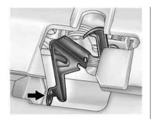
Go to the front of the vehicle and with hand palm side down, slide the secondary hood release handle toward the driver side of the vehicle.
