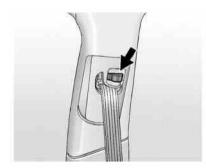
Press the release button and move the height adjuster to the desired position. The adjuster can be moved up by pushing the slide/trim up. After the adjuster is set to the desired position, try to move it down without pushing the release button to make sure it has locked into position.
