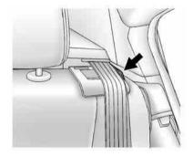
3. Make sure the safety belt is in the guide on top of the seatback.
