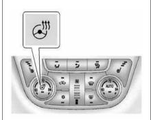
(Heated Steering Wheel): For vehicles with a heated steering wheel, press to turn it on or off. A light on the button displays when the feature is turned on.
