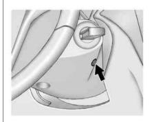
Vehicles with an automatic transmission and a key start system, are equipped with an electronic key lock release. The key lock release is designed to prevent ignition key removal unless the shift lever is in P (Park).
