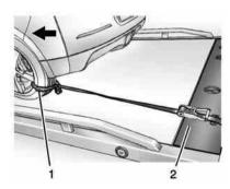
7. Secure the vehicle to the flatbed (2) using nonabrasive straps (1) through all four wheel openings and secure the straps to the flatbed (2).
