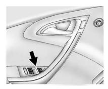
The power window switches on the driver door control all four windows. Each passenger door has a switch that controls only that window.
