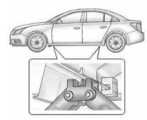
Position the jack lift head at the jack location nearest the flat tire. The location is indicated by a notch in the flange. The jack must not be used in any other position.
