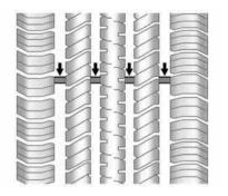
Treadwear indicators are one way to tell when it is time for new tires. Treadwear indicators appear when the tires have only 1.6 mm (1/16 in) or less of tread remaining. See *Tire Inspection on page 10-52* and *Tire Rotation on page 10-52*.
