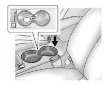
Place the new transmitter into the transmitter pocket with the buttons facing up. The transmitter pocket is inside the center console cupholder. The cupholder liner will need to be removed to access the transmitter pocket. Use a finger or a tool in the notch at the rear of the cupholders to remove the liner. See Cupholders on page 4-2.
