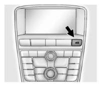
Use one of the following methods to open the trunk. The vehicle must be off, or stopped with the parking brake applied (manual transmission), or the shift lever must be in P (Park) (automatic transmission), in order for the trunk to be opened.
