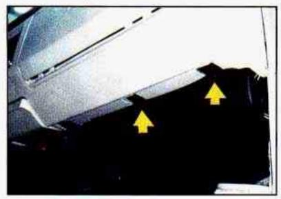
You'll find the interior relay center under the right side of the instrument panel. To gain access, remove two screws from the black hush panel.
