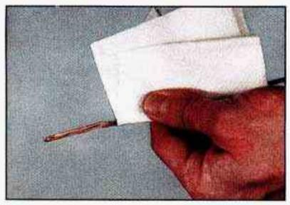
When to Add Oil: If the oil is at or below the ADD line, then you'll need to add some oil. But you must use the right kind. This section explains what kind of oil to use. For crankcase capacity, see "Capacities and Specifications" in the Index
