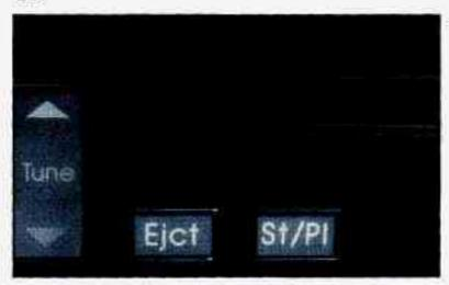
Press St/Pl (Stop/Play). The disc will stop and the radio will play. Press St/Pl to restart the disc. It will resume playing at the point where it stopped.
