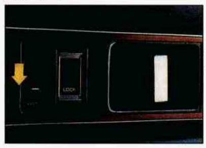
From the inside: To lock the door, slide the lock lever down to the "LOCK" position.
