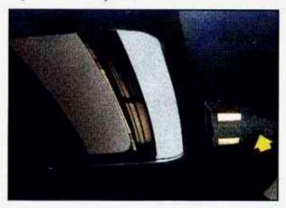
The astroroof includes a sliding glass panel and a sliding sunshade. The control switch only works with the ignition on or in Retained Accessory Power (RAP) mode.
