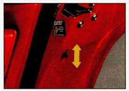
Move the lever on the door all the way down.
