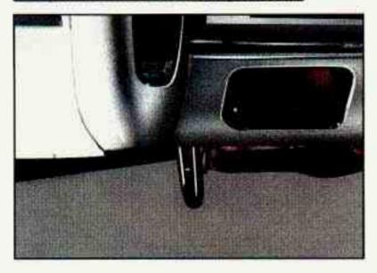
If you ever get stuck in sand, mud, ice or snow, your vehicle may be equipped with a retrieval hook. The retrieval hook is provided at the left rear of your vehicle. You may need to use it if you're stuck off-road and need to be pulled to some place where you can continue driving.
