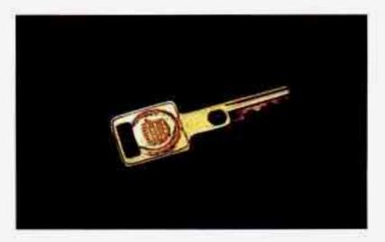
Your vehicle is equipped with the PASS-Key II <sup>™</sup> (Personalized Automotive Security System) theft deterrent system. PASS-Key II <sup>™</sup> is a passive theft deterrent system. This means you don't have to do anything different to arm or disarm the system. It works when you insert or remove
