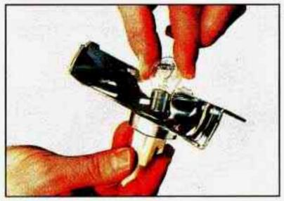
To remove the bulb, push it in and rotate it counterclockwise.
