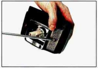
Remove the two housing screws.
