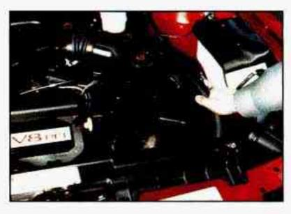
Start the engine and let it run until you can feel the upper radiator hose getting hot. Watch out for the engine fans.
