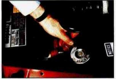
Start by removing the red positive (+) terminal cover.
