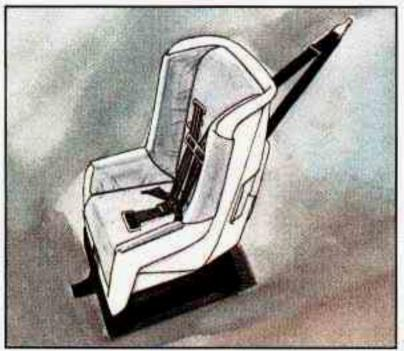
If your child restraint has a top strap, it should be anchored.
