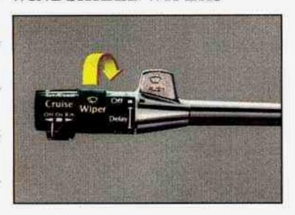
You control the windshield wipers by turning the band marked "WIPER."
