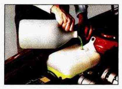
4. Then fill the coolant recovery tank to "FULL COLD."
