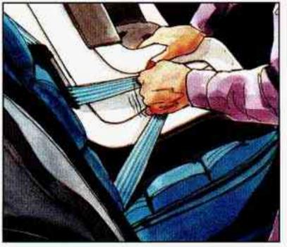
Pull the rest of the lap belt all the way out of the retractor to set the lock.
