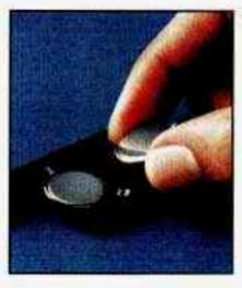
Replace the batteries. Put them in with the printed side down.
