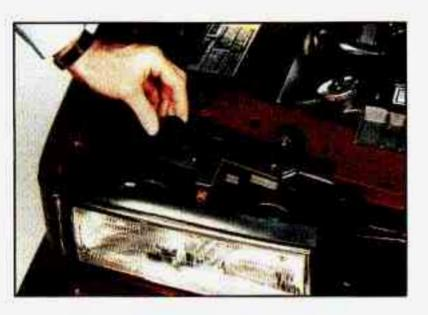
Domestic or Export - Remove the two headlamp housing assembly fasteners.
