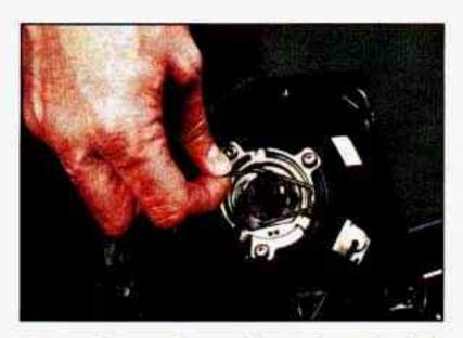
Export - Remove the retaining spring and raise it up, out of the way.
