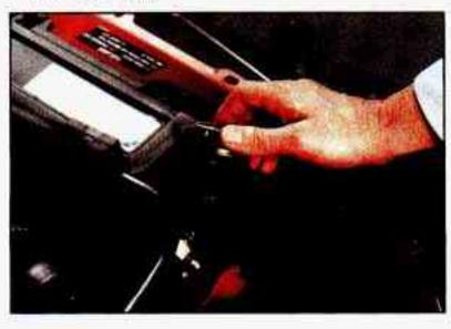
Then keep turning the pressure cap, but now push down as you turn it. Remove the pressure cap.
