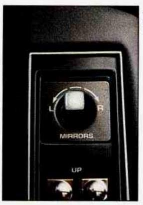
Just rotate the knob to choose the left or right mirror. Then move it to adjust the mirror.
