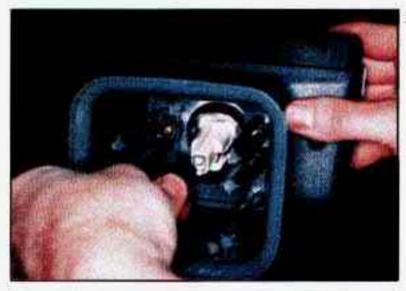
Disconnect the wiring harness connector from the socket.
