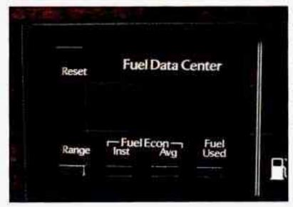
This shows how far the computer thinks you can go with the fuel that's in your tank. When you get down to 40 miles to go (or, in metric, 64 km) it just says "L," which means "LOW." You should then get fuel right away.
