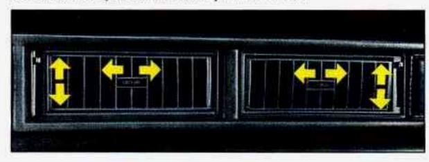
Move the center lever to direct air flow from side to side.
