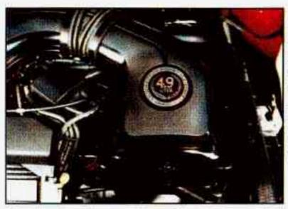
To gain access to the air cleaner element. loosen the four screws and lift the top half of the air cleaner assembly.
