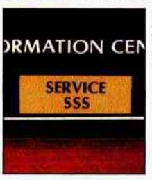
When you first start your car, the "SERVICE SSS" light will come on as a bulb check and a system self-check for a few seconds.
