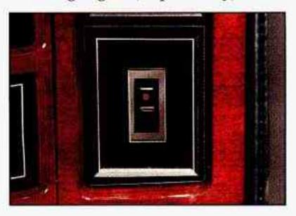
To turn them on, push the switch located on the right lower side of your instrument panel. A small indicator light will glow to tell you they are on.
