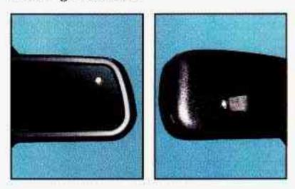
Use a cotton swab and glass cleaner to clean the front and rear photocells that make the mirror work.
