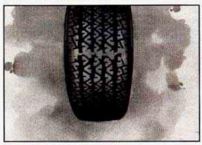
One way to tell when it's time for new tires is to check the treadwear indicators, which will appear when your tires have only 2/32 inch (1.6 mm) or less of tread remaining.
