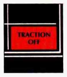
The "TRACTION OFF" warning light lets you know if your traction control system is not working. See "Traction Control System Warning Light" in the Index.
