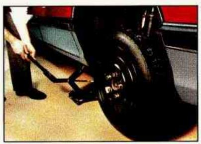
Lower the vehicle completely by rotating the wheel wrench counterclockwise. Tighten the wheel nuts firmly in a criss-cross sequence as shown.
