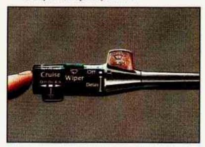
Push in the button at the end of the lever and release it.
