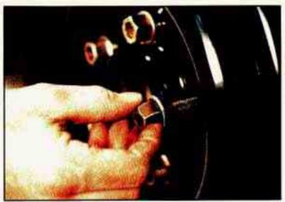
Replace the wheel nuts with the rounded end of the nuts toward the wheel. Tighten each nut by hand until the wheel is held against the hub.
