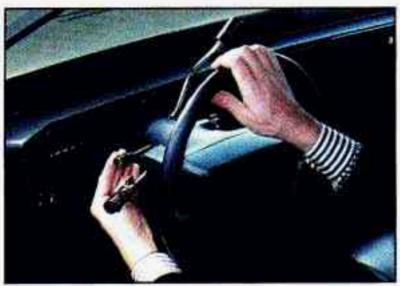
To tilt the wheel, hold the steering wheel and pull the lever. Move the steering wheel to a comfortable level, then release the lever to lock the wheel in place.
