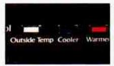
To choose the temperature you want inside the car, push the cooler or warmer button. You can choose from 65°F (18°C) to 85°F (29°C). And, at each end, you may choose 60°F (16°C), for maximum cooling, and 90° F (33°C), for maximum heating.
