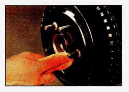
Remove any rust or dirt from the wheel bolts, mounting surfaces or spare wheel. Place the spare on the wheel mounting surface.
