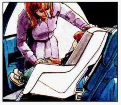
Push and pull the child restraint in different directions to be sure it is secure.
