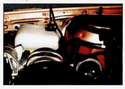
10. Attach the cable at least 18 inches (45cm) away from the dead battery, but not near engine parts that move. The electrical connection is just as good there, but the chance of sparks getting back to the battery is much less.
