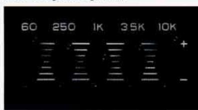
Your equalizer lets you set the bass, midrange and treble to sound just the way you want. The 60 and 250 controls work the bass side. Midrange is the 1K. The 3.5K and 10K are treble sound controls.
