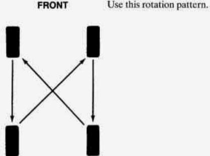
After the tires have been rotated, adjust the front and rear inflation pressure as shown on the Tire-Loading Information label. Make certain that all wheel nuts are properly tightened. See "Wheel Nut Torque" in the Index.
