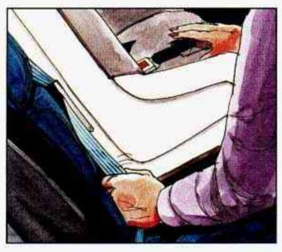
To tighten the belt, feed the lap belt into the retractor while you push down on the child restraint.
