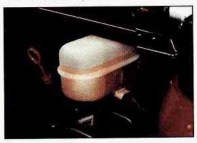
There are only two reasons why the brake fluid level in your master cylinder might go down. The first is that the brake fluid goes down to an acceptable level during normal brake lining wear. When new linings are
