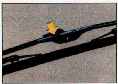
Using a small screwdriver or your finger, gently lift the release lever up while at the same time pulling the blade assembly from the wiper arm.
