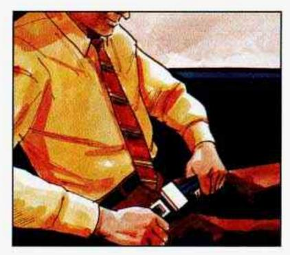
To make the belt shorter, pull its free end as shown until the belt is snug.
