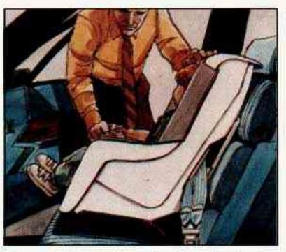
Push and pull the child restraint in different directions to be sure it is secure.
