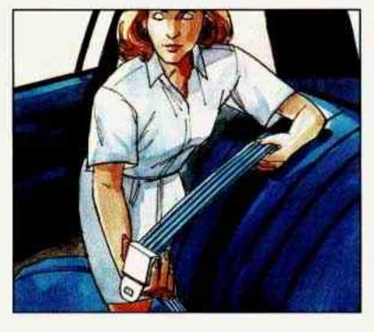
Make the belt as long as possible by tilting the latch plate and pulling it along the belt.
