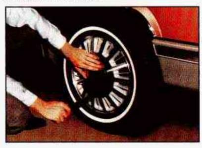
Use the flat end of the wheel wrench. Insert into the small slot on the wheel and gently remove the center cover. Be careful not to drop the cover on the ground, you could scratch it.
