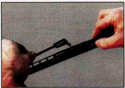
To install the wiper blade, align the wiper arm pin with the hole on the wiper blade assembly and snap it into place. If you only want to replace the wiper inserts follow these steps:
