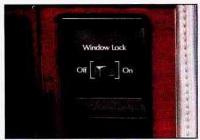
When the switch is in the "On" position, an amber indicator light will illuminate. Only the driver's window control switches will operate the power windows. This feature is useful when you're transporting small children and you don't want them using the power windows.
