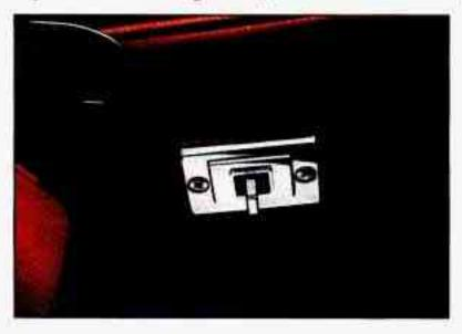
Move the switch forward to raise the seat back and rearward to recline the seat back.
