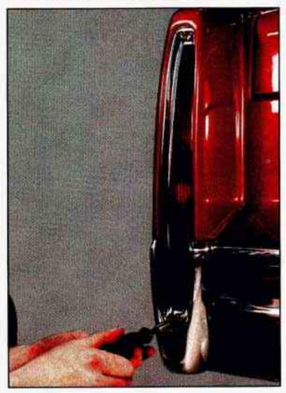
Remove the upper and lower torx screws and remove the bezel.
