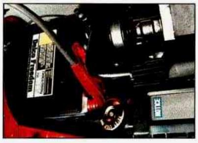
Connect the red positive (+) cable to the positive (+) terminal of the vehicle with the dead battery.
