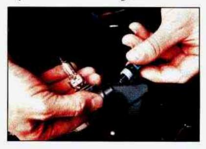
**Domestic** - Remove the wiring harness from the bulb socket. Connect the wiring harness to the new bulb socket and install into headlamp assembly.
