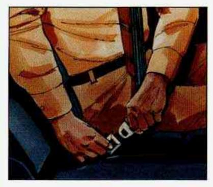
To unlatch the belt, just push the button on the buckle. The belt should go back out of the way.
