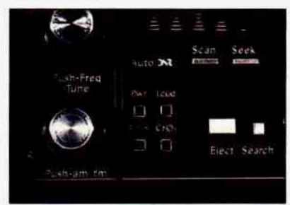
The power (or PWR) button turns your system on and off unless you have a Bose system. If you do, rotate the upper knob to turn it on and off.
