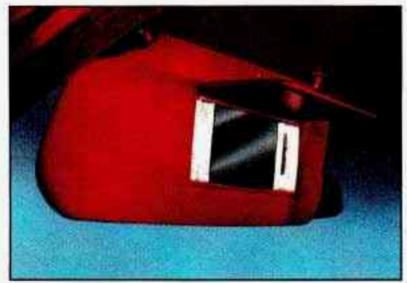
To use one, turn the sunshade down. Then lift the cover up to see the mirror. The switch makes the light brighter.
