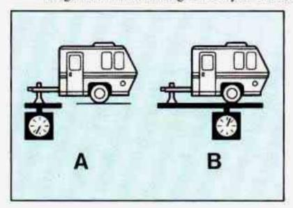
The trailer tongue (A) should weigh 10% of the total loaded trailer weight (B). After you've loaded your trailer, weigh the trailer and then the tongue, separately, to see if the weights are proper. If they aren't, you may be able to get them right simply by moving some items around in the trailer.
