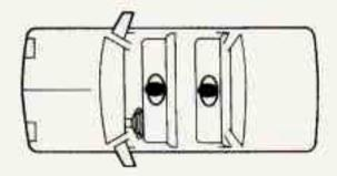
When you secure a child restraint in a center seating position, you'll be using the lap belt.
