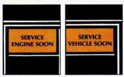
A computer monitors operation of your fuel, ignition and emission control systems. This light should come on when the ignition is on, but the engine is not running, as a check to show you it is working. If it does not come on at all, have it fixed right away. If it stays on, or it comes on while you are driving, the computer is indicating that you have a problem. You should take your vehicle in for service soon.
