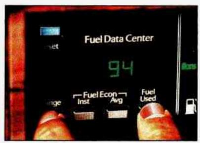
Press and hold the Range and Fuel Used buttons to display the oil life percentage.
