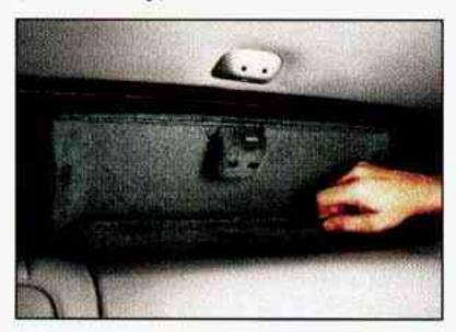
To gain assess to the bulbs, gently pull the back panel located inside the rear storage compartment.
