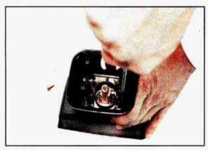
Remove the two screws, and then remove the pedestal.
