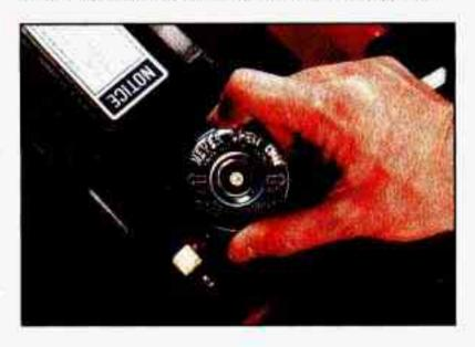
You can remove the radiator pressure cap when the cooling system, including the radiator pressure cap and upper radiator hose, is no longer hot. Turn the pressure cap slowly to the left until it first stops. (Don't press down while turning the pressure cap.)
