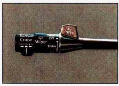
Move the Cruise Control switch to "ON."
