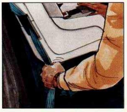
To tighten the belt, feed the lap belt back into the retractor while you push down on the child restraint.
