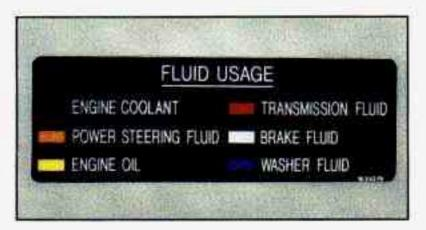
Use the fluid usage label to identify the correct fluid you want to check.
