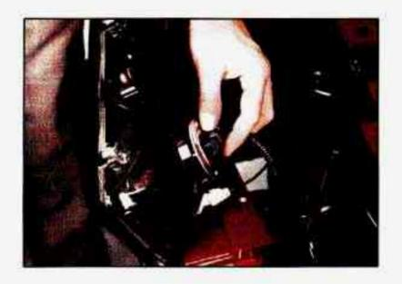
**Domestic -** Turn the housing socket 1/4 turn counterclockwise and remove it from the headlamp housing.
