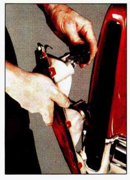
Press the bulb housing lever, rotate the housing counterclockwise 1/6 turn and remove it.
