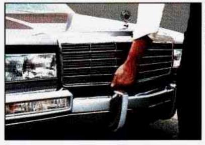
Then go to the front of the vehicle and push the secondary hood release upward to release it.
