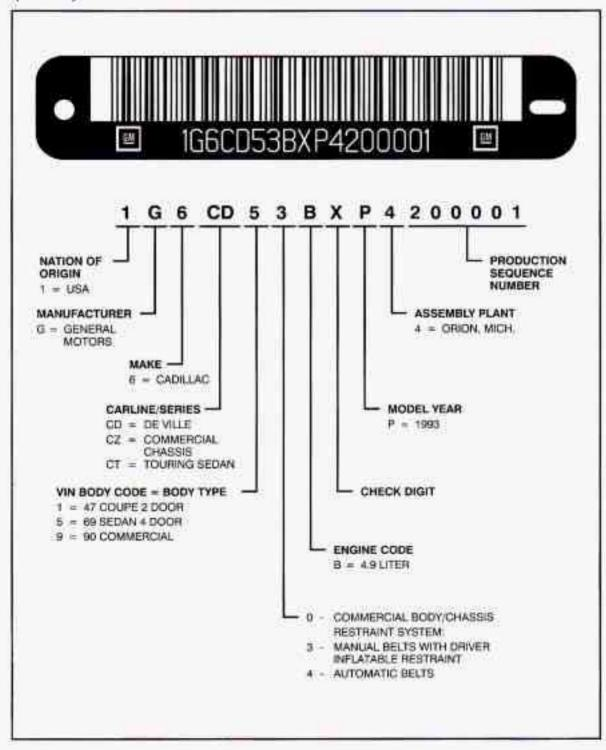
This is the legal identifier for your Cadillac. It appears on a plate in the front corner of the instrument panel, on the driver's side. You can see it if you look through the windshield from outside your vehicle. The VIN also appears on the Vehicle Certification and Service Parts labels and the certificates of title and registration.
