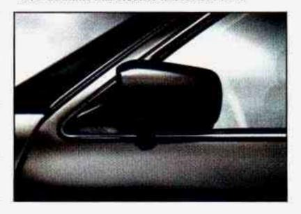
If you have the Touring Sedan or an Export vehicle, you have collapsible outside mirrors. These mirrors can pivot to accommodate tight situations. Just pivot the mirror inward. To return the mirror to its normal position, rotate the mirror until it locks into place.
