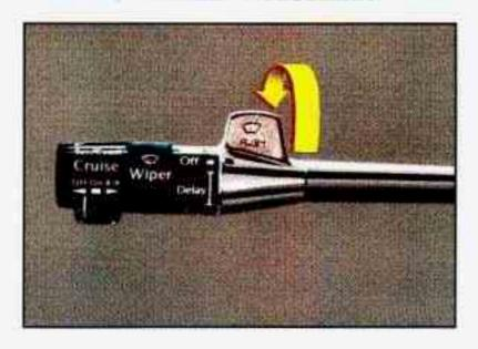
At the top of the multifunction lever there's a paddle with the word "PUSH" on it. To spray washer fluid on the windshield, push and release the paddle. The wipers will clear the window and then either stop or return to your preset speed. For continued wash operation, press and hold the paddle down.
