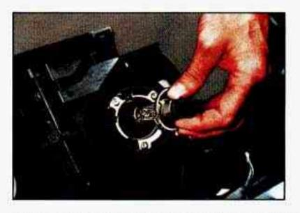
Export - Reinstall new bulb into headlamp housing assembly, reinstall rubber grommet and wiring harness.
