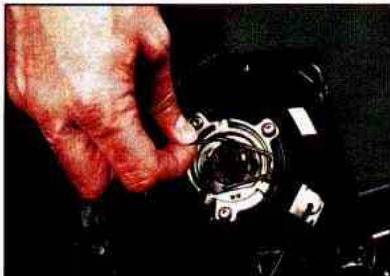
**Export - Remove the retaining spring and raise it up, out of the way.**
