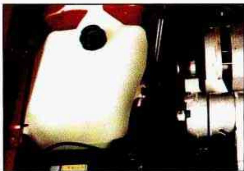
5. Put the cap back on the coolant recovery tank, but leave the radiator pressure cap off.
