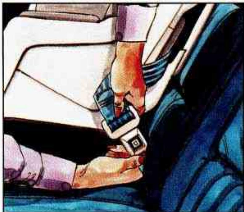
4. Buckle the belt. Make sure the release button faces upward or outward, so you'll be able to unbuckle it quickly if you ever need to.
