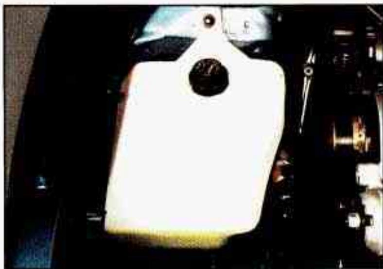
The coolant level should be at or above near “FULL COLD.” If it isn’t, you may have a leak in the radiator hoses, heater hoses, radiator, water pump or somewhere else in the cooling system.
