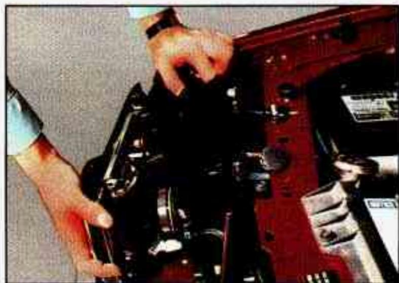
**Domestic or Export** - Gently lift the headlamp housing assembly and pull it forward to gain access to the bulb and socket housing.
