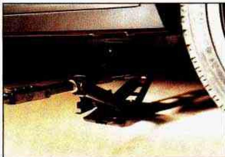
Your Cadillac has a notch on the frame near each of the wheels. Fit the lift head into the notch nearest the wheel with the flat tire.
