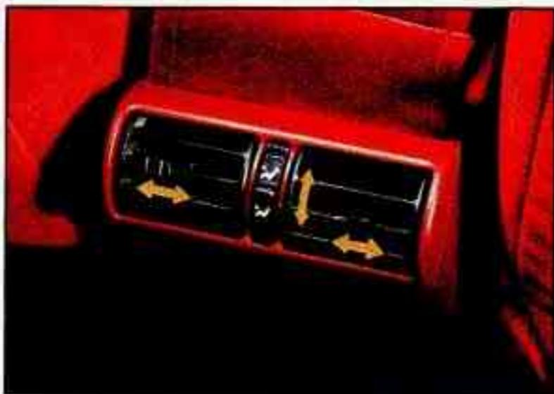
Turn the center dial to direct the air flow through the vents or at the floor.
