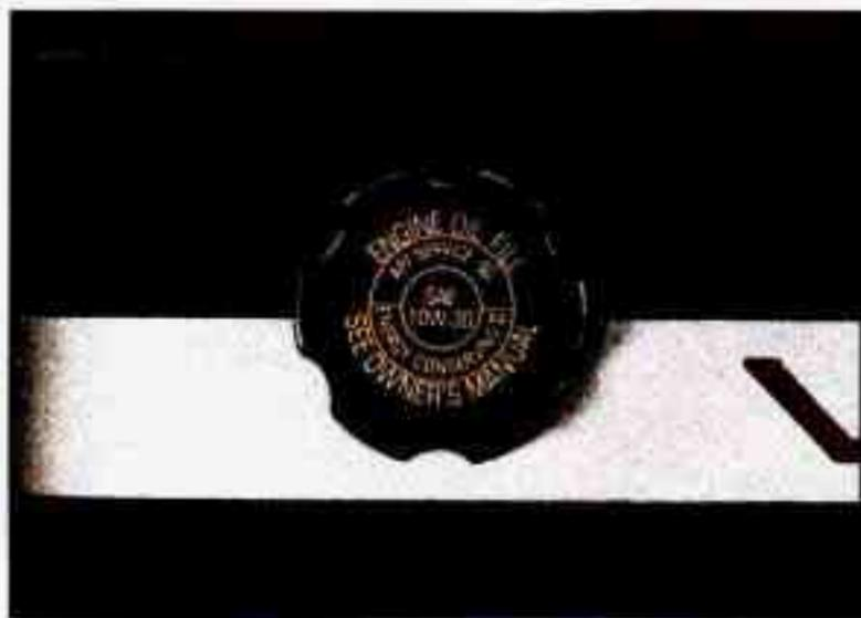
To remove, turn the oil fill cap to the left.
