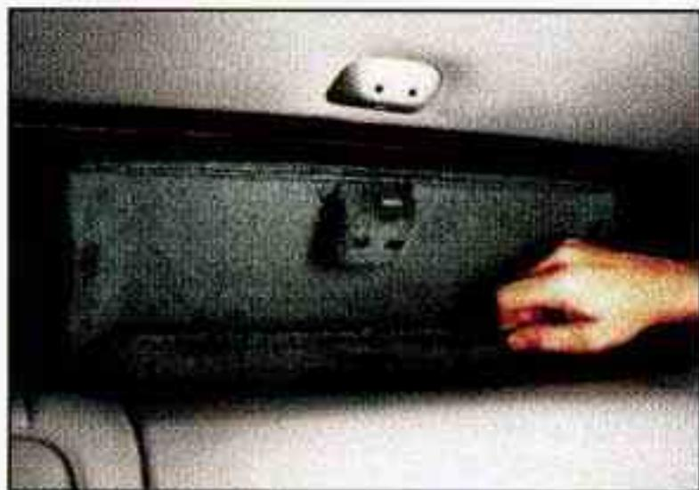
To gain access to the bulbs, gently pull the back panel located inside the rear storage compartment.
