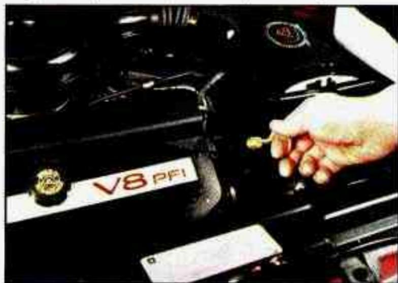
**To Check Engine Oil:** Pull out the dipstick and clean it with a paper towel or cloth, then push it back in all the way. Remove it again, keeping the tip lower.
