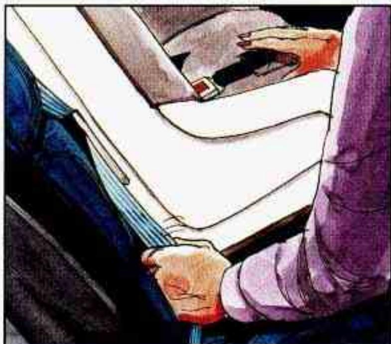
6. To tighten the belt, feed the lap belt into the retractor while you push down on the child restraint.
