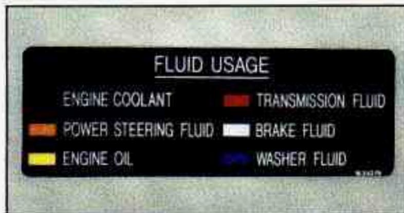
Use the fluid usage label to identify the correct fluid you want to check.
