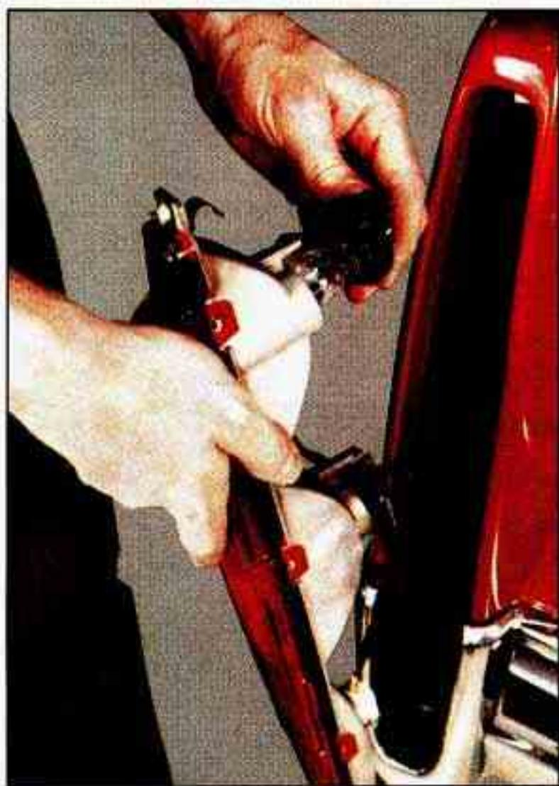
3. Press the bulb housing lever, rotate the housing counterclockwise  $1/6$  turn and remove it.
