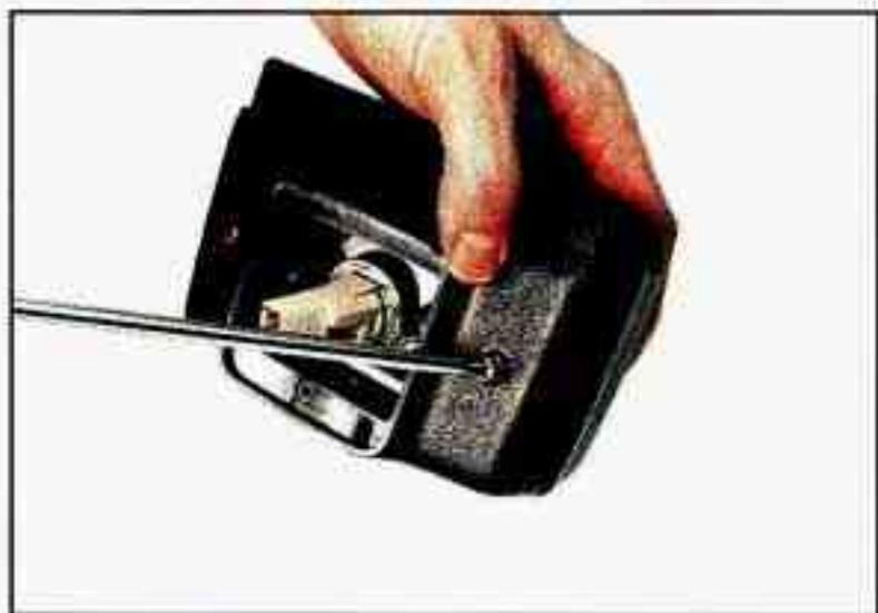
4. Remove the two housing screws.
