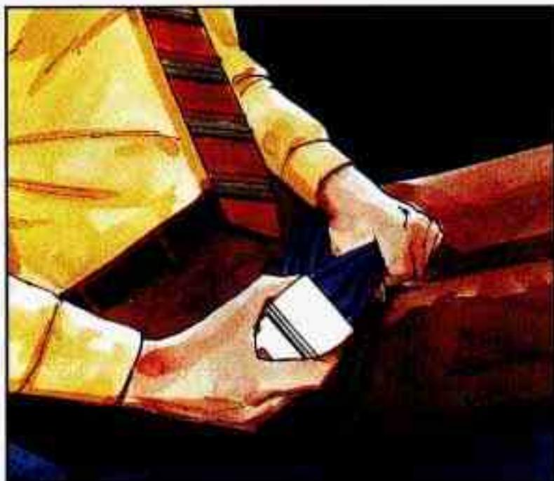
When you sit in a center seating position, you have a lap safety belt, which has no retractor. To make the belt longer, tilt the latch plate and pull it along the belt.
