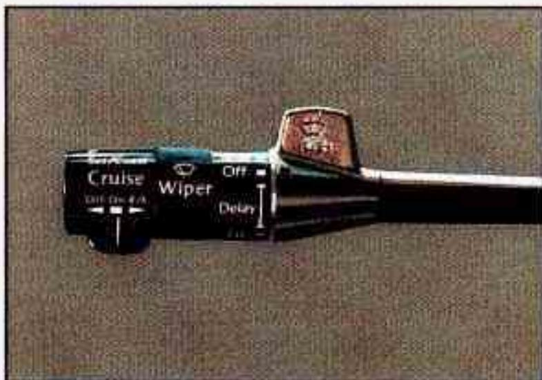
Move the Cruise Control switch to "ON."
