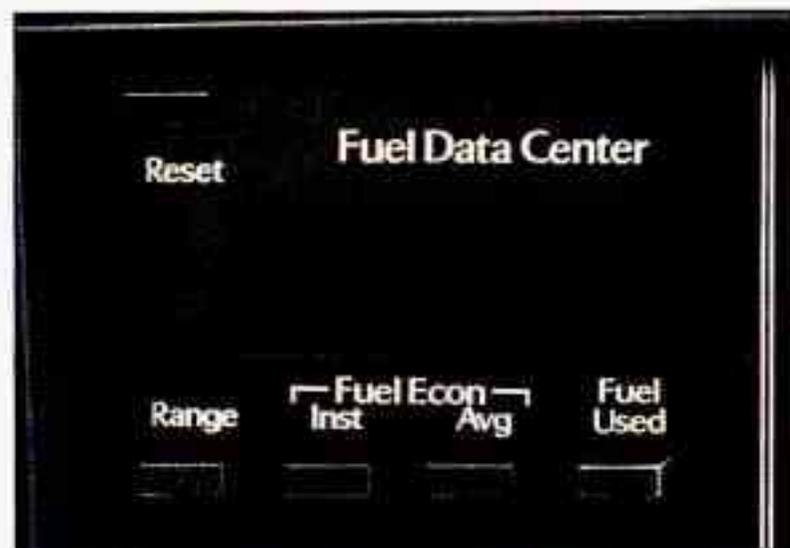
This reading shows how much fuel you've used since you last reset the system. It returns to zero after 99.9 gallons (or, in metric, 379 liters).
