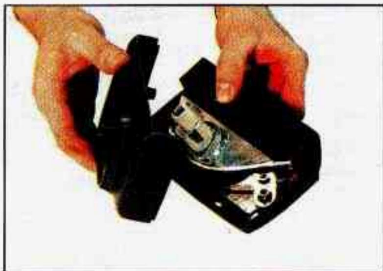
5. Disassemble the housing assembly like this.
