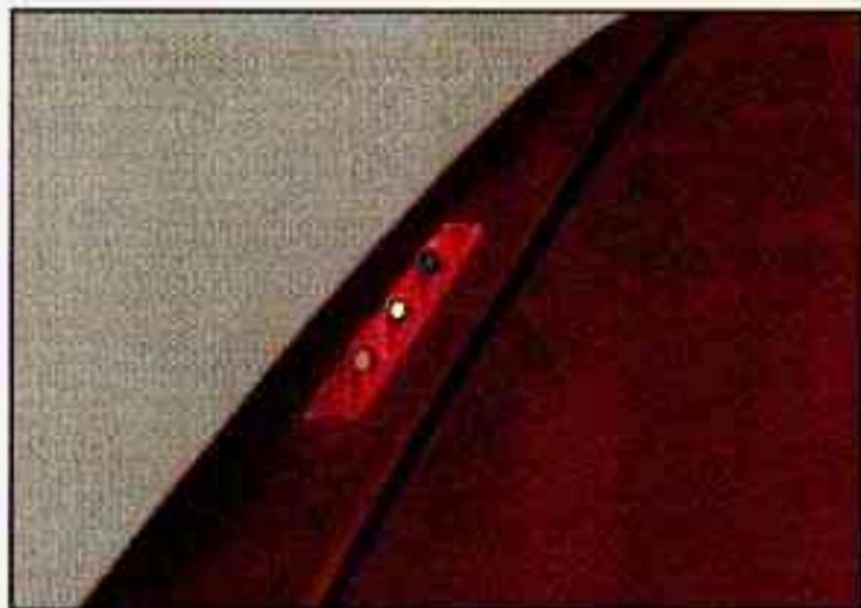
The front lamp monitors show that your headlamps, high beam and turn signals are working.
