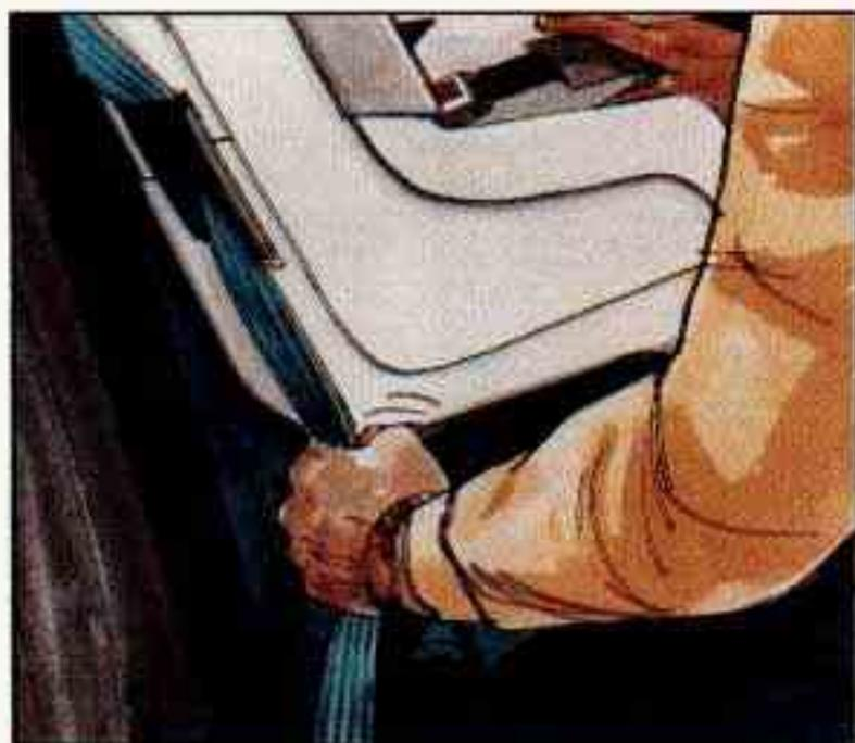
6. To tighten the belt, feed the lap belt back into the retractor while you push down on the child restraint.
