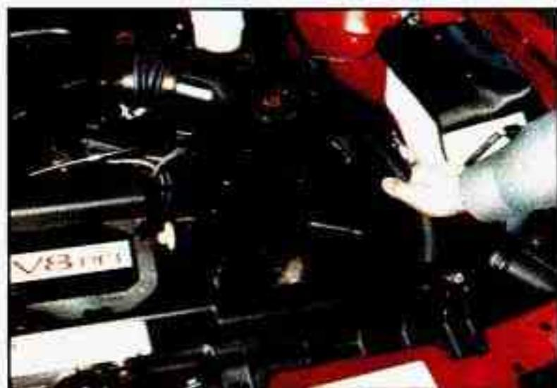
6. Start the engine and let it run until you can feel the upper radiator hose getting hot. Watch out for the engine fans.
