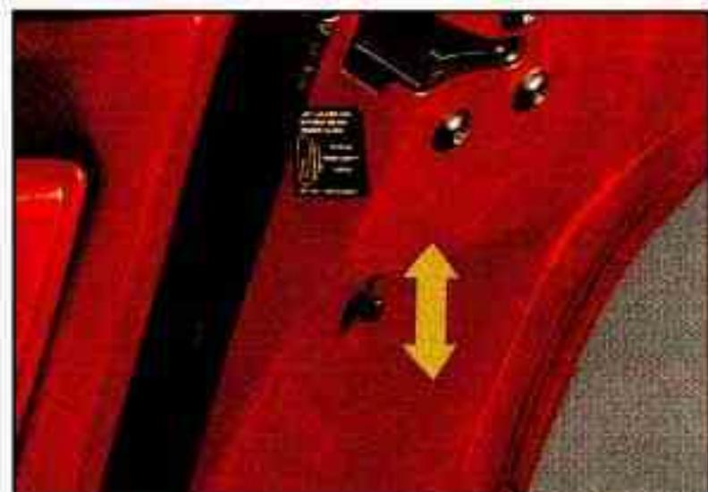
1. Move the lever on the door all the way down.
