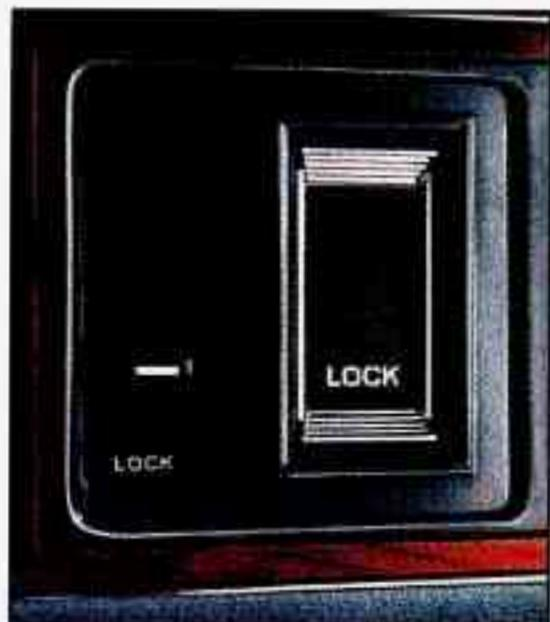
Push the lower part of the switch marked "LOCK" to lock all the doors at once. Push the upper part of the switch to unlock all the doors.
