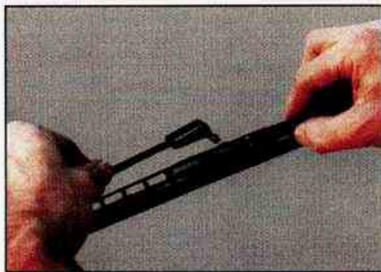
To install the wiper blade, align the wiper arm pin with the hole on the wiper blade assembly and snap it into place.
