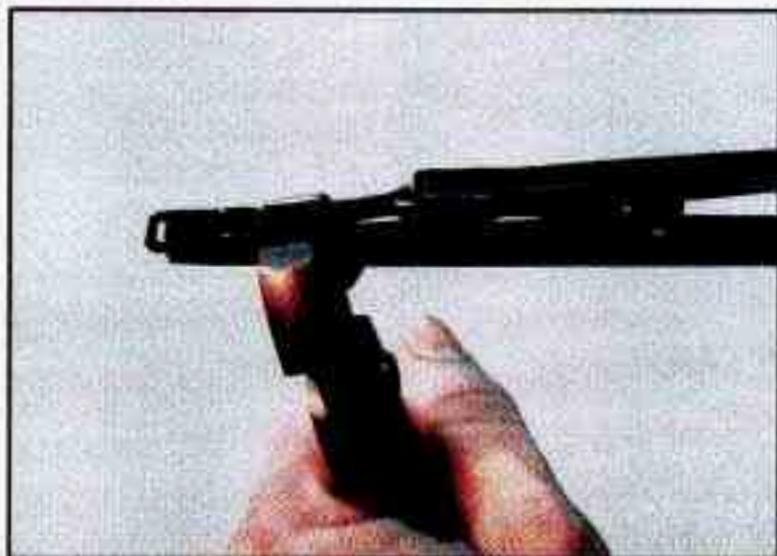
1. Disconnect the wiper insert by bending the end of the insert gently using pliers. Then pull it from the housing retaining tab.
