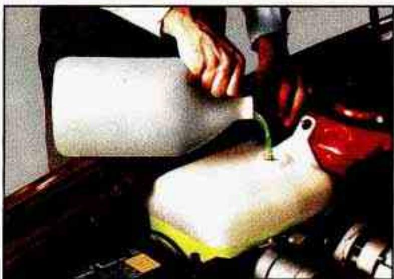
4. Then fill the coolant recovery tank to "FULL COLD."
