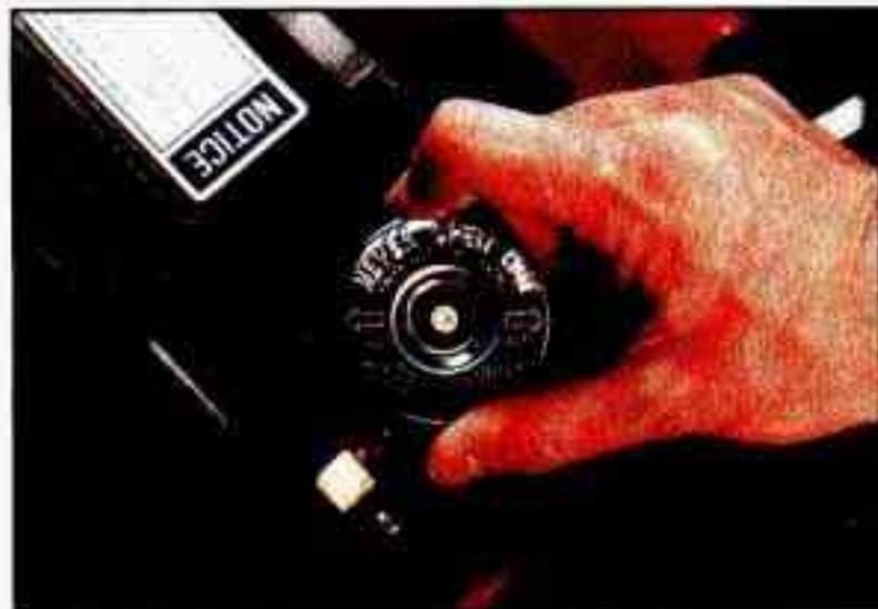
1. You can remove the radiator pressure cap when the cooling system, including the radiator pressure cap and upper radiator hose, is no longer hot. Turn the pressure cap slowly to the left until it first stops. (Don't press down while turning the pressure cap.)
