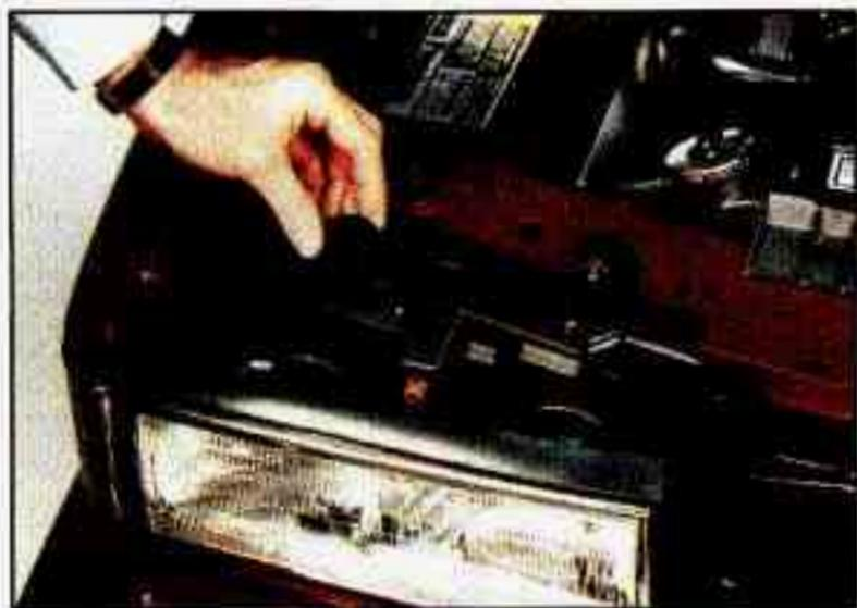
**Domestic or Export** - Remove the two headlamp housing assembly fasteners.
