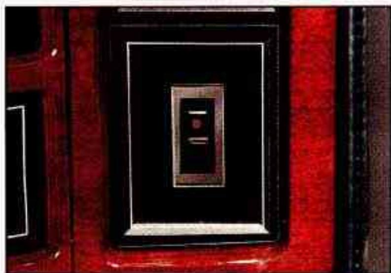
To turn them on, push the switch located on the right lower side of your instrument panel. A small indicator light will glow to tell you they are on.
