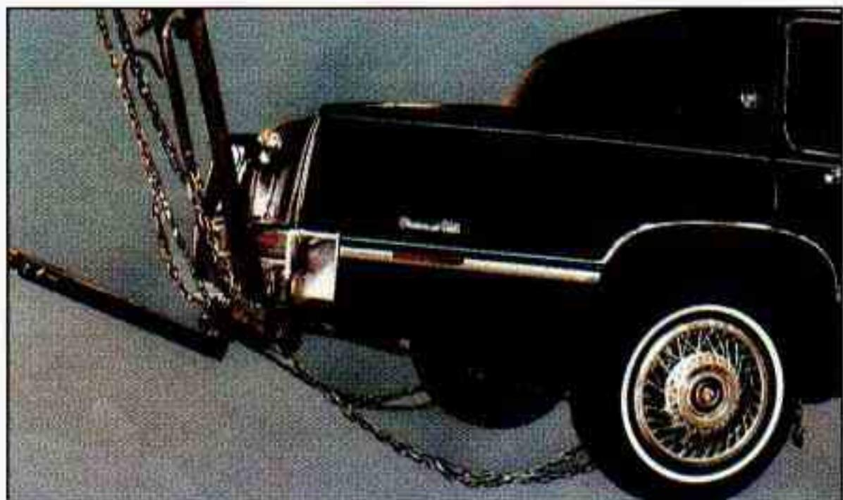
No 4x4 wood beam required. Position lower sling cross bar directly under the rear bumper.
