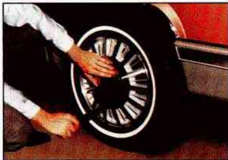
Use the flat end of the wheel wrench. Insert into the small slot on the wheel and gently remove the center cover. Be careful not to drop the cover on the ground, you could scratch it.
