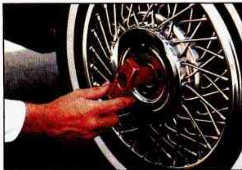
Use the other end of the wire wheel wrench like this. Remove the special anti-theft wheel nut by turning it counterclockwise.
