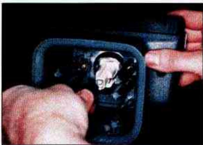
2. Disconnect the wiring harness connector from the socket.
