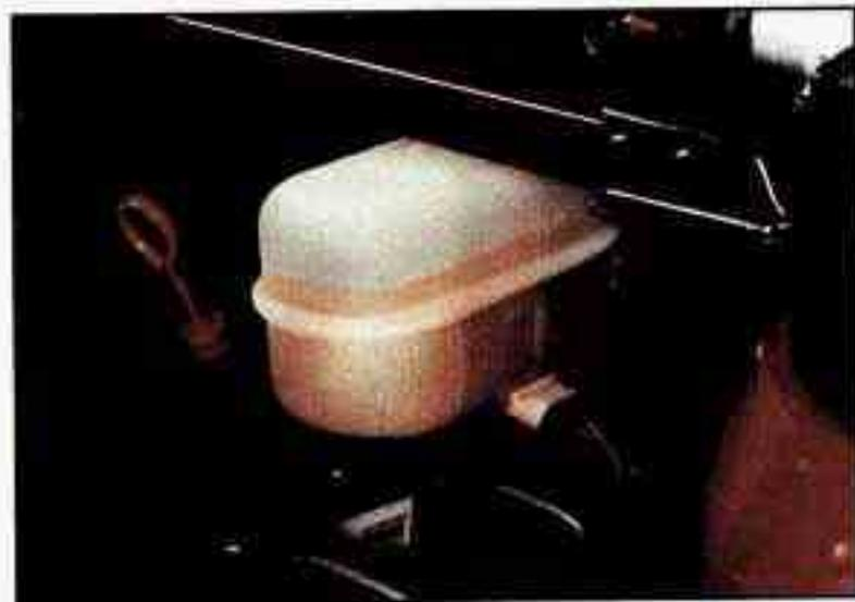
There are only two reasons why the brake fluid level in your master cylinder might go down. The first is that the brake fluid goes down to an acceptable level during normal brake lining wear. When new linings are
