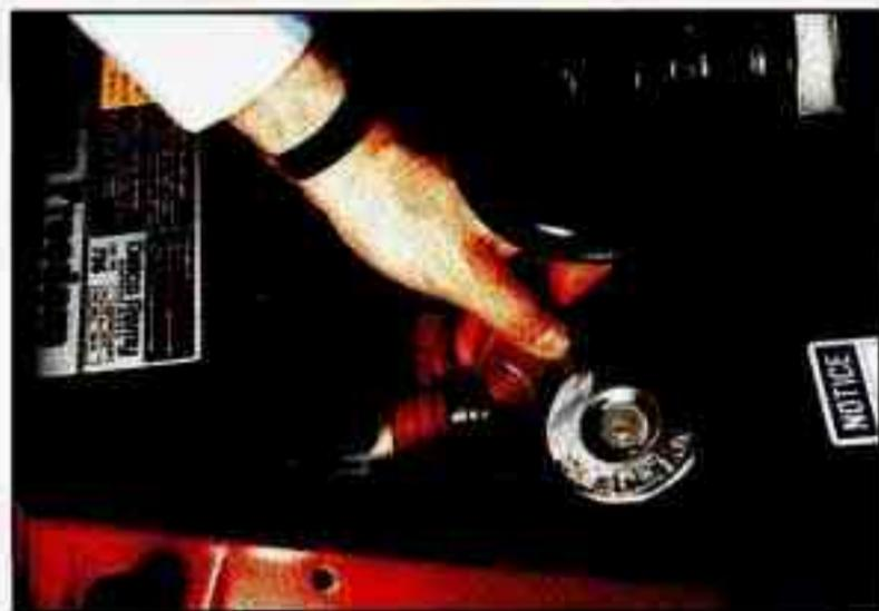
6. Start by removing the red positive (+) terminal cover.
