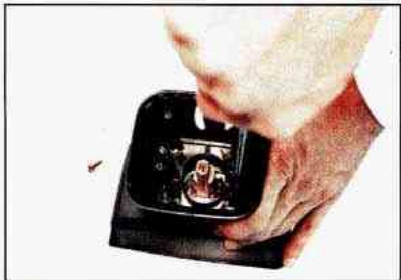
3. Remove the two screws, and then remove the pedestal.
