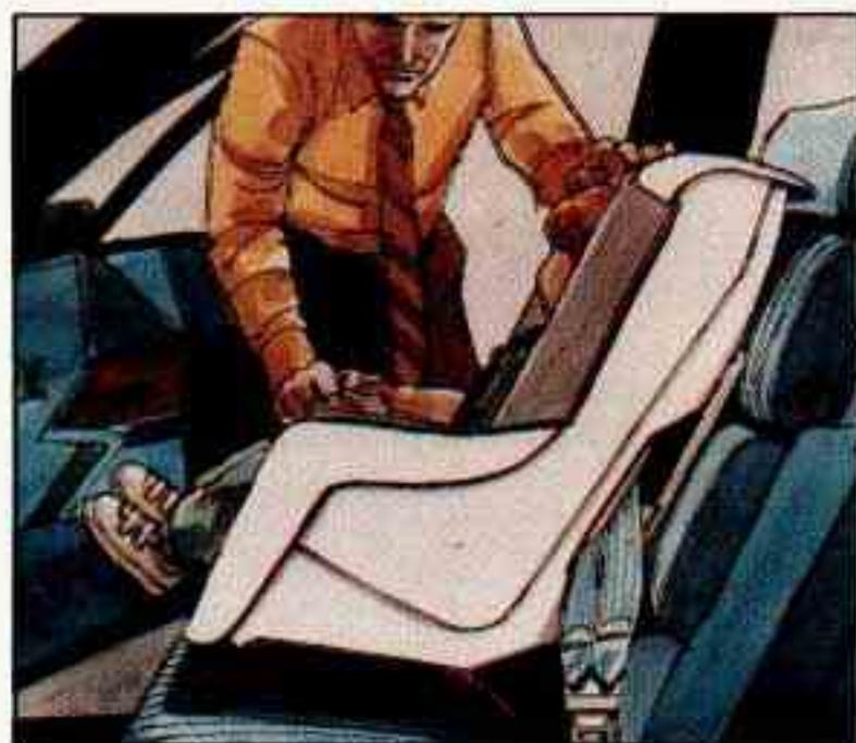
7. Push and pull the child restraint in different directions to be sure it is secure.
