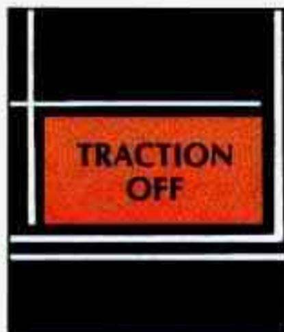
The "TRACTION OFF" warning light means that the system is not working. This warning light may come on for the following reasons:
