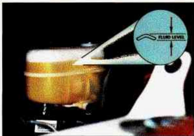
You can check the brake fluid without taking off the cap. If it's low, fill it to the maximum "FLUID LEVEL" indicator.
