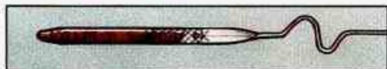
3. Check both sides of the dipstick, and read the lower level. The fluid level must be in the cross-hatched area.
