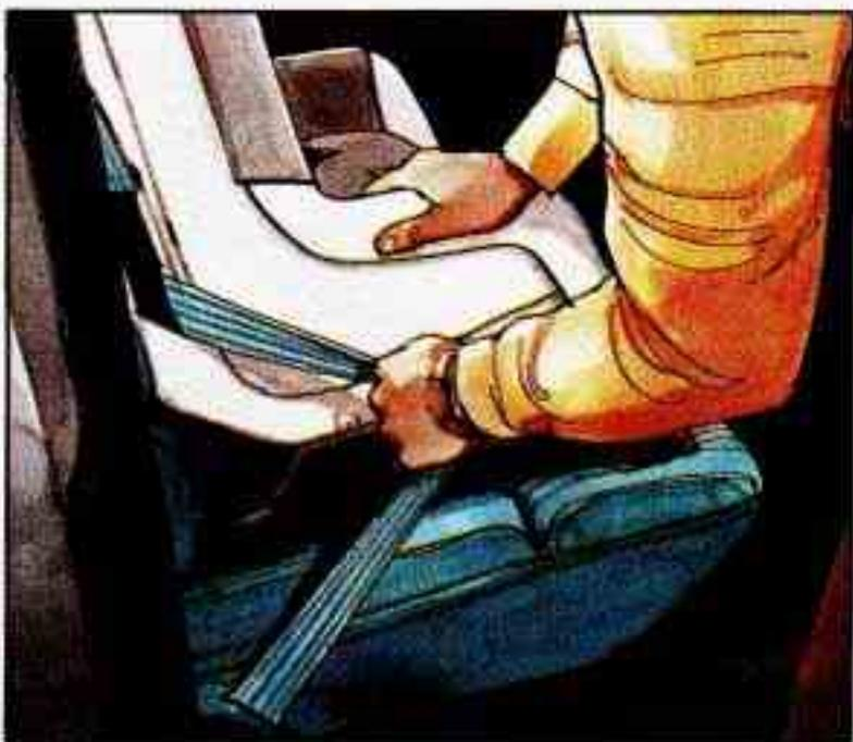
5. Pull the rest of the lap belt all the way out of the retractor to set the lock.
