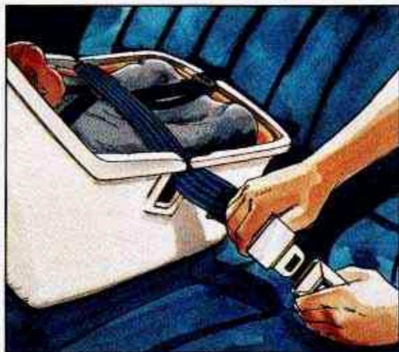
5. Buckle the belt. Make sure the release button faces upward or outward, so you'll be able to unbuckle it quickly if you ever need to.
