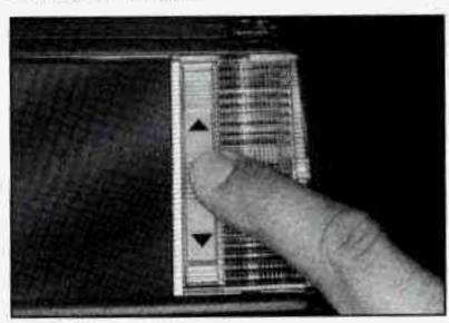
To use one, turn the sunshade down. Then lift the cover up to see the mirror. The slide switch controls the lamp intensity.
