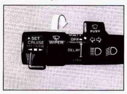
WIPER: To control the wipers turn the band on the multifunction lever.
