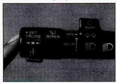
Press the button at the end of the lever and release it.
