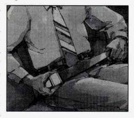
When you sit in the center seating position, you have a lap safety belt, which has no retractor. To make the belt longer, tilt the latch plate and pull it along the belt.
