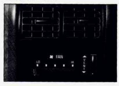
Move the FAN switch to adjust the blower speed from LO to HI.
