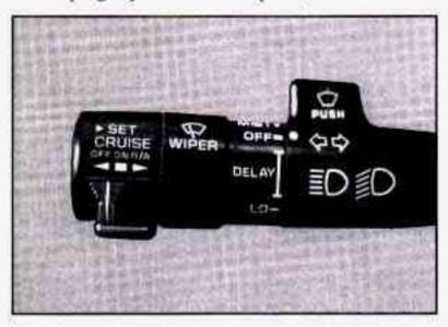
2. Move the CRUISE switch to OFF. (The CRUISE light will go out.)
