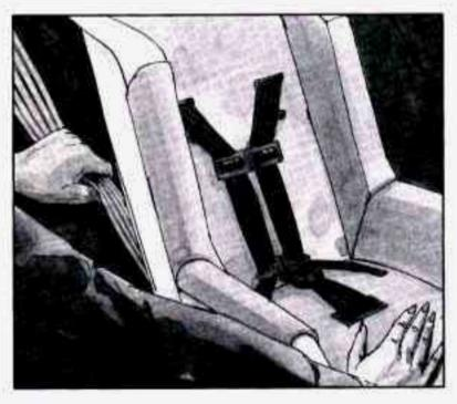
To tighten the belt, pull up on the shoulder belt while you push down on the child restraint.
