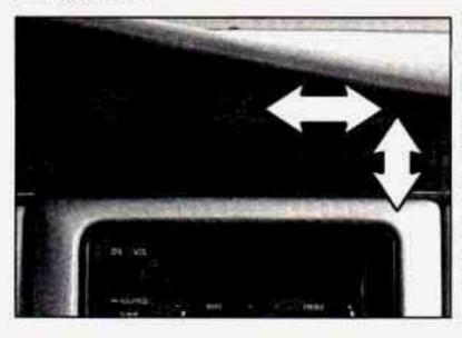
Air outlets are located in the center and at each side of the instrument panel. You can adjust the direction of airflow by moving the center control levers or you can stop the airflow by moving the lever located on each side of the outlets downward.
