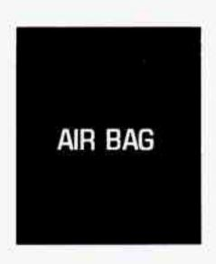
There is an air bag readiness light on the instrument panel, which shows AIR BAG. The system checks the air bag's electrical system for malfunctions. The light tells you if there is an electrical problem. See "Air Bag Readiness Light" in the Index for more information.
