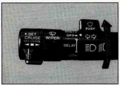
To wash your windshield, press and hold the paddle labeled PUSH. Once you feel you have enough washer fluid on the windshield, release the paddle. The wipers will continue to clear the windshield, then either stop or return to your preset speed.
