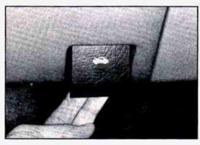
To open the hood, first pull the lever inside the vehicle, located at the lower left side of the instrument panel.
