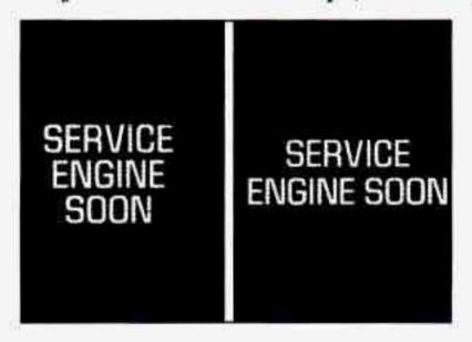
A computer monitors operation of your fuel, ignition and emission control systems. One of these lights should come on when the ignition is on, but the engine is not running, as a check to show you it is working. If the light doesn't come on, have it fixed right away. If it stays on or it comes on while you are driving, the computer is indicating that you have a problem. You should take your vehicle in soon for service.
