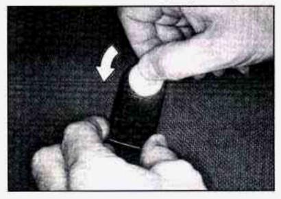
Use the round end of the door key, or a coin, to rotate the cover counterclockwise 1/16 of a turn.
