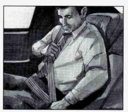
To make the lap part tight, pull down on the buckle end of the belt as you pull up on the shoulder part.
