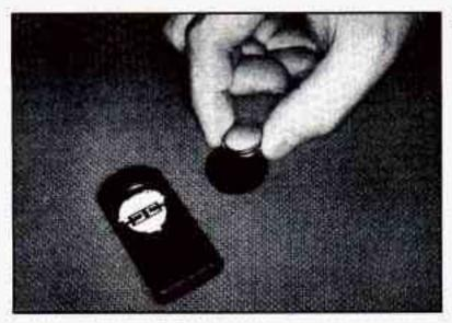
Remove the battery and replace with CR2025 or an equivalent. Using the wrong size battery can damage the transmitter.
