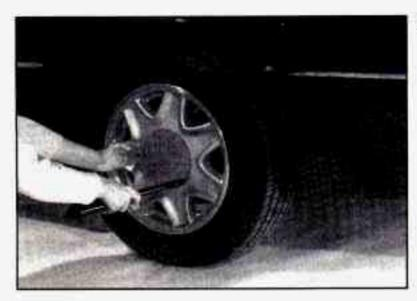
4. There is a center wheel cover on your aluminum wheel. Use the flat end of the wheel wrench, prying along the edge of this cover until it comes off. Be careful not to scratch the aluminum wheel edge. Don't try to remove it with your hands.
