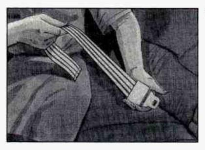
Make the belt as long as possible by tilting the latch plate and pulling it along the belt.
