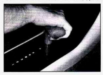
Hold in the button on the lever and push the lever all the way toward the front of your vehicle.
