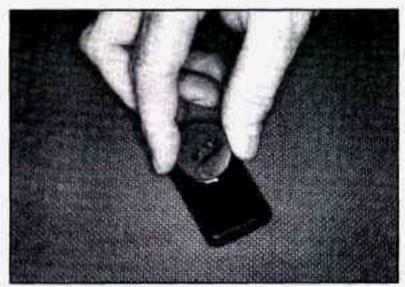
Align the notches on the cover and the transmitter. Rotate the cover clockwise to reinstall.
