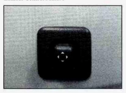
If you have this feature, you can change the shape of the driver and passenger seats. It works independently of the other seat controls. Use the power seat control first to get the proper position. Then proceed with the lumbar adjustment.
