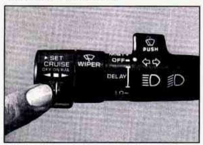
Move the cruise control switch to ON.
