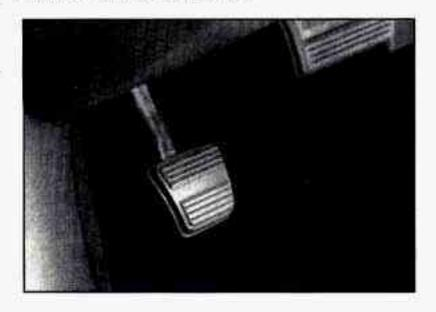
To set the parking brake, hold the regular brake pedal down with your right foot and push down the parking brake pedal with your left foot. If the ignition is on, the brake system warning light will come on.
