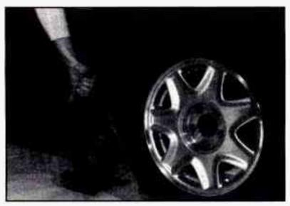
Raise the vehicle by rotating the wheel wrench clockwise.
