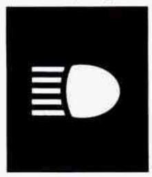
To change the headlamps from low beam to high or high to low, pull the turn signal lever all the way toward you. Then release it. When the high beams are on, this blue light on the instrument panel will also be on.
