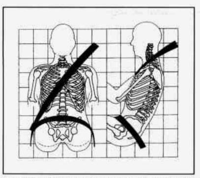
The lap part of the belt should be worn low and snug on the hips, just touching the thighs.
