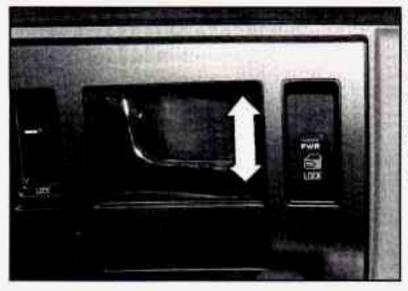
Press the power door lock switch to lock or unlock all the doors at once. The rear power door lock switches only provide a lock function as a safety feature. They will not unlock the doors.
