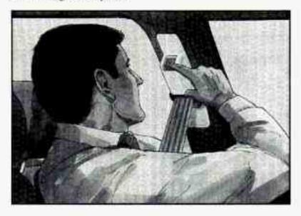
To move it down, squeeze the release handle and move the height adjuster to the desired position. You can move the adjuster up just by pushing up on the bottom of the release handle. After you move the adjuster to where you want it, try to move it down without squeezing the release handle to make sure it has locked into position.
