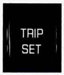
By using this button, you can tell how far you've gone since you last set the TRIP SET back to zero. To reset, press and hold the button until zeros appear.
