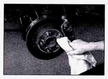
Remove any rust or dirt from the wheel bolts. mounting surfaces and spare wheel. Place the spare on the wheel mounting surface.
