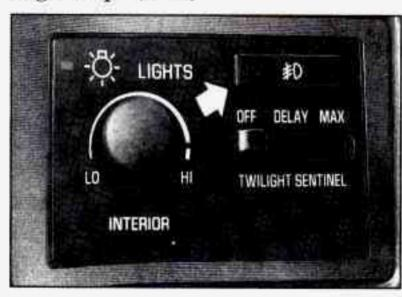
Use your fog lamps for better vision in foggy or misty conditions. When you press the upper fog lamp switch, a small indicator light will glow to tell you the fog lamps are on. To turn them off press the switch again.
