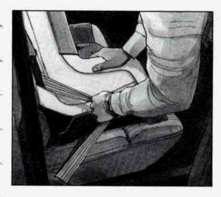
Pull the rest of the lap belt all the way out of the retractor to set the lock.
