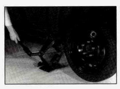
Lower the vehicle by rotating the wheel wrench counterclockwise.
