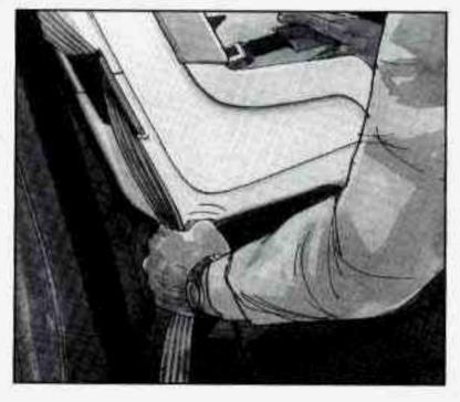
To tighten the belt, feed the lap belt back into the retractor while you push down on the child restraint.
