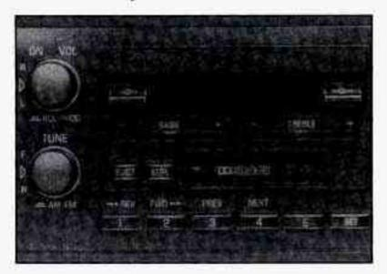
This standard music system is the Delco<sup>®</sup> Bose Music System with dual playback. The system includes an AM and FM stereo electronically tuned radio receiver with an integral cassette, and six Delco<sup>®</sup> custom designed speakers with very specific frequency ranges. A digital clock is also included.
