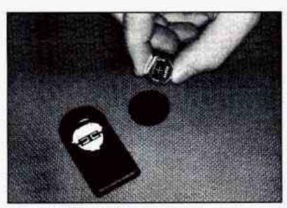
Make sure the battery is positioned with the "plus" (+) sign facing the cover.
