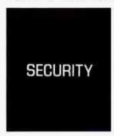
If your Cadillac has this option, it has a Theft Deterrent Alarm System, With this system, the SECURITY light will flash as you open the door (if your ignition is off).
