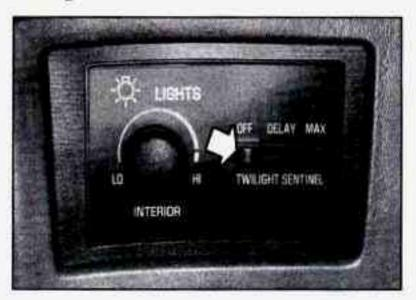
The control is next to the headlamp switch. It automatically switches your lamps on and off by sensing how dark it is outside. To operate the twilight sentinel, leave the lamp switch off and move the control to any position but OFF.
