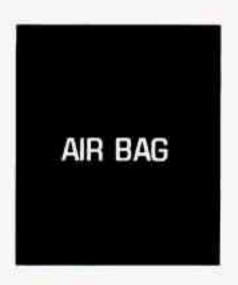
You will see this light flash for a few seconds when you turn your ignition to RUN or START. Then the light should go out. This means the system is ready.
