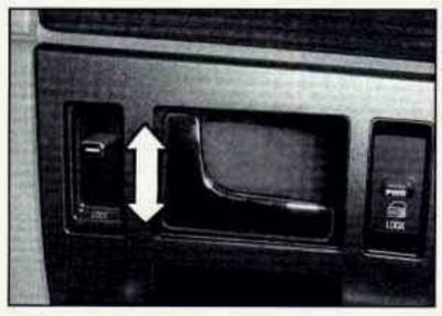
From the inside, slide the lock lever down to manually lock the door. To unlock the door, slide the lock lever up.
