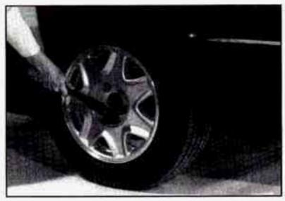
Using the wheel wrench, loosen all the wheel nuts. Do not remove them yet.
