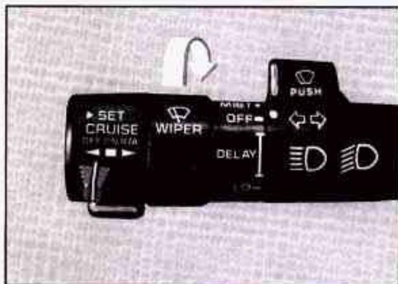
**WIPER:** To control the wipers turn the band on the multifunction lever.
