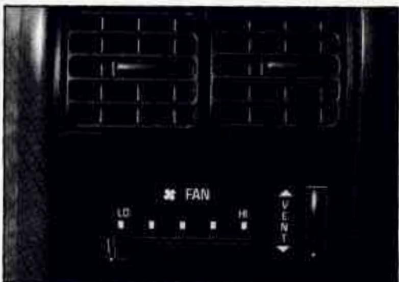
Move the FAN switch to adjust the blower speed from LO to HI.
