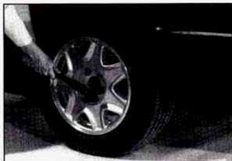
5. Using the wheel wrench, loosen all the wheel nuts. Do not remove them yet.
