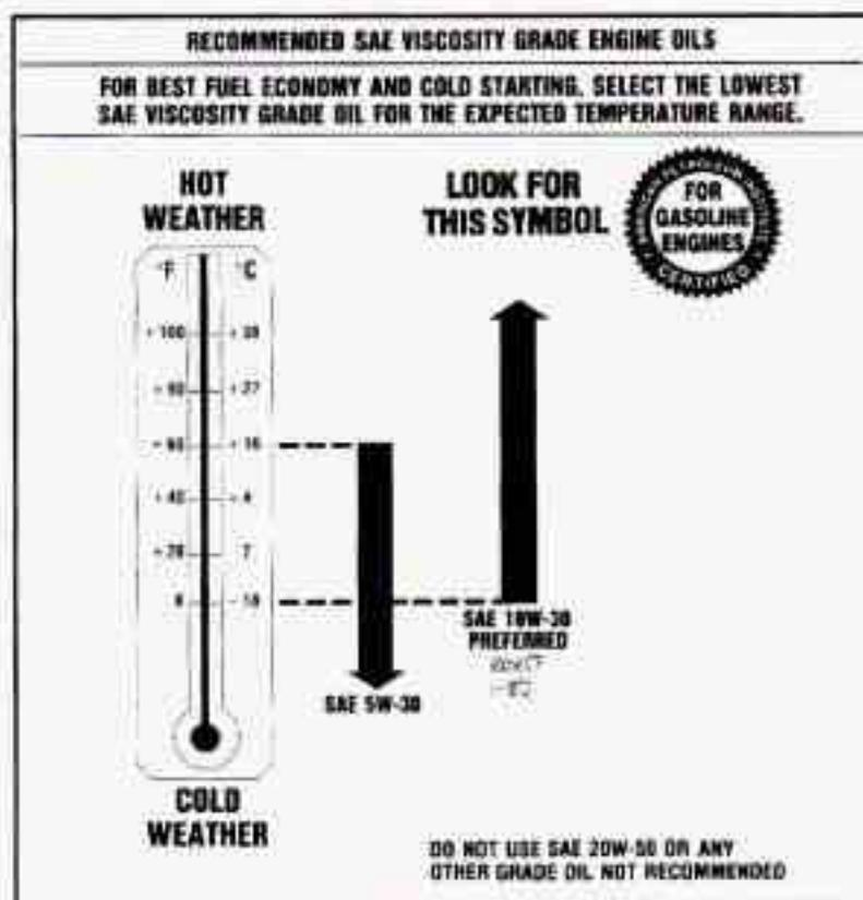
As shown in the chart, SAE 10W-30 is best for your vehicle. However, you can use SAE 5W-30 if it's going to be colder than 60°F (16°C) before your next oil change. When it's very cold, you should use SAE 5W-30. These numbers on an oil container show its viscosity, or thickness. Do not use other viscosity oils, such as SAE 20W-50.
