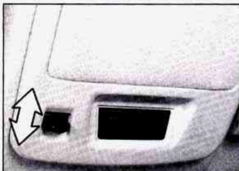
The astroroof includes an express open feature, a sliding glass panel and a sliding sunshade. The control switch only works with the ignition on or in the Retained Accessory Power (RAP) mode.
