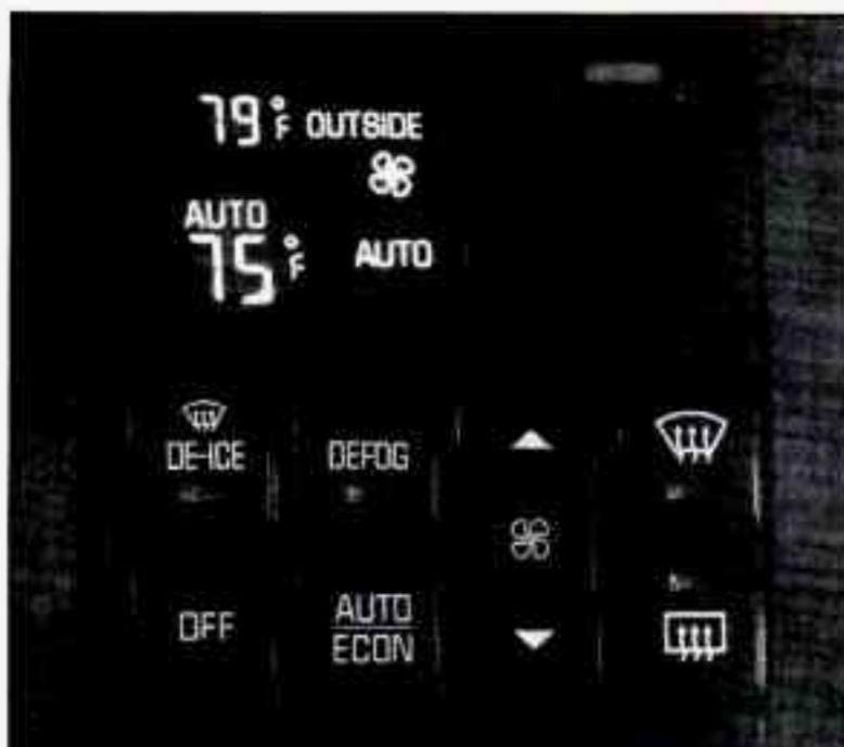
Your vehicle has strategically placed electronic sensors that provide information to the vehicle's computer systems. Your vehicle can control the ventilation, heating and air conditioning automatically year round. The outside temperature, inside temperature setting, fan speeds and the ECC selection are displayed on a digital screen.
