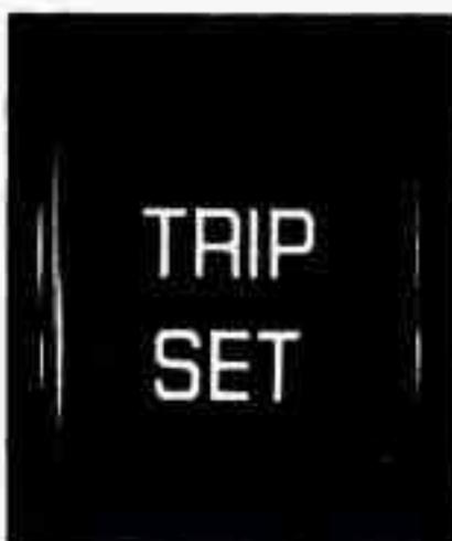
By using this button, you can tell how far you've gone since you last set the TRIP SET back to zero. To reset, press and hold the button until zeros appear.
