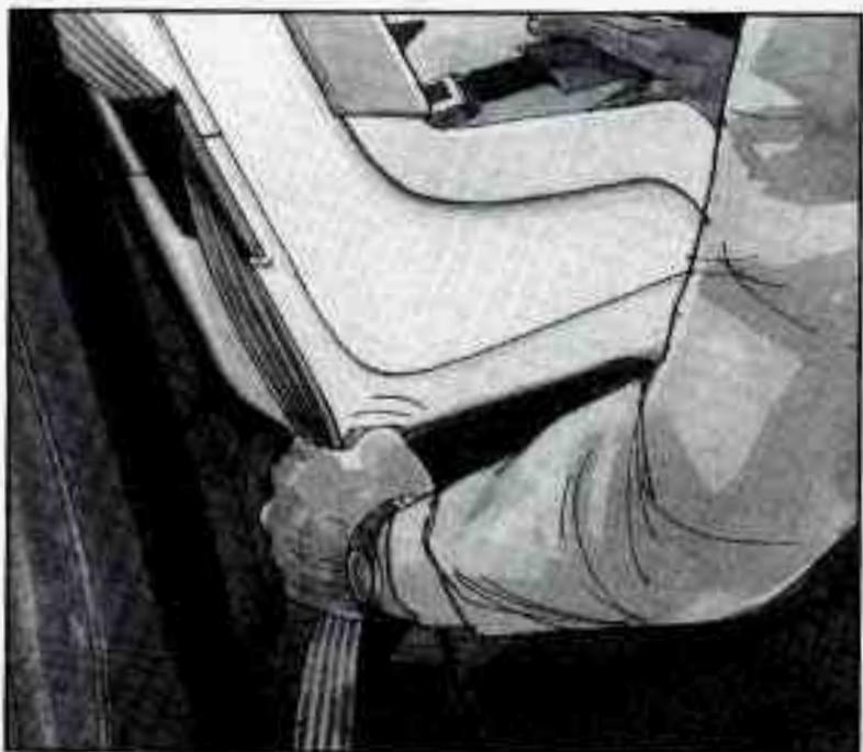
7. To tighten the belt, feed the lap belt back into the retractor while you push down on the child restraint.
