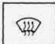
Press this button to remove fog or frost from the windshield.
