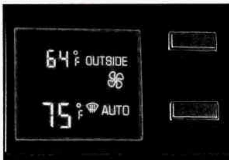
To select the temperature you want, press the blue button for a cooler setting or the red button for a warmer setting. The temperature setting will be displayed on the digital screen.
