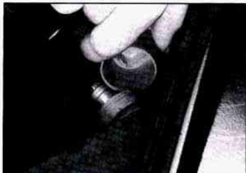
5. Start by removing the red positive (+) terminal cover.
