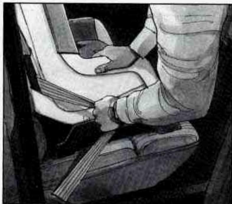
6. Pull the rest of the lap belt all the way out of the retractor to set the lock.
