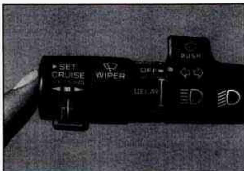
3. Press the button at the end of the lever and release it.
