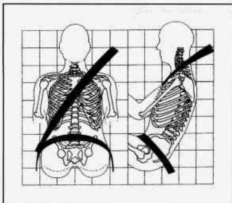
The lap part of the belt should be worn low and snug on the hips, just touching the thighs.
