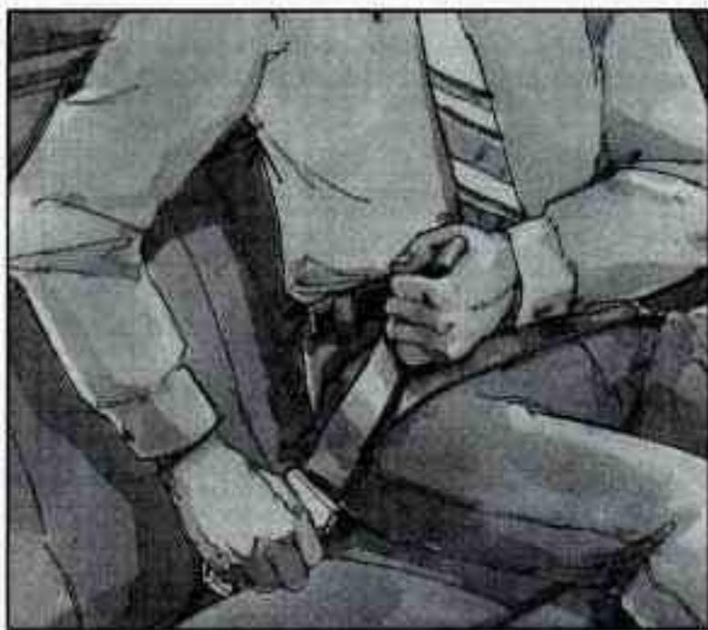
To make the belt shorter, pull its free end as shown until the belt is snug.
