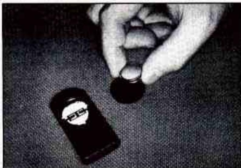
2. Remove the battery and replace with CR2025 or an equivalent. Using the wrong size battery can damage the transmitter.
