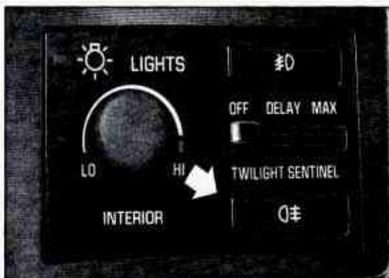
To operate the rear fog lamps, first turn on the front fog lamps, then press the lower switch. A small indicator light will glow to tell you they are on. To turn them off press the switch again.
