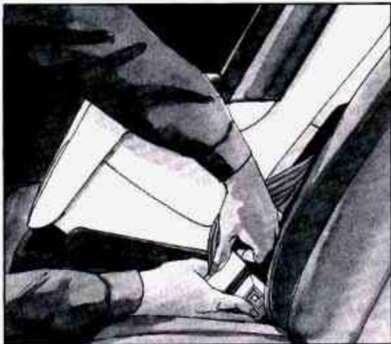
4. Buckle the belt. Make sure the release button is positioned so you would be able to unbuckle the safety belt quickly if you ever had to.
