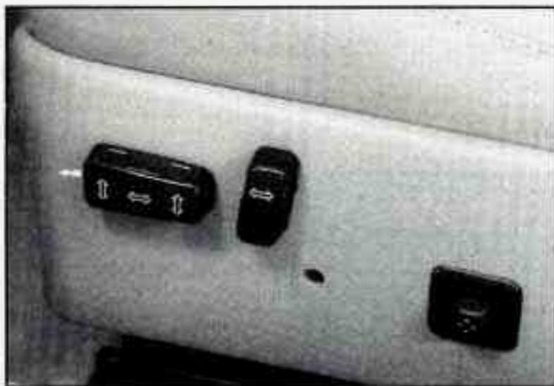
The power seat control switches are located on the outboard side of the front seat cushion.
