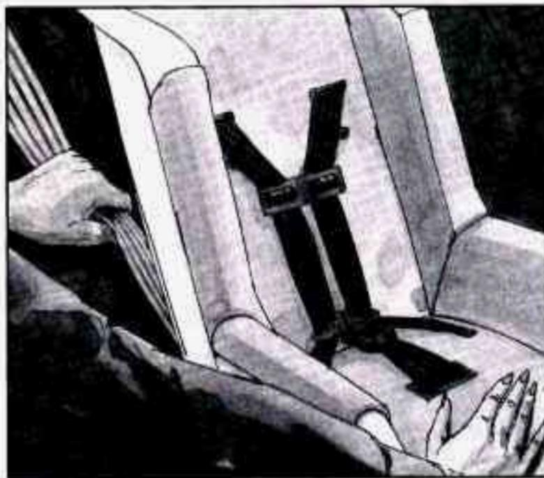
5. To tighten the belt, pull up on the shoulder belt while you push down on the child restraint.
