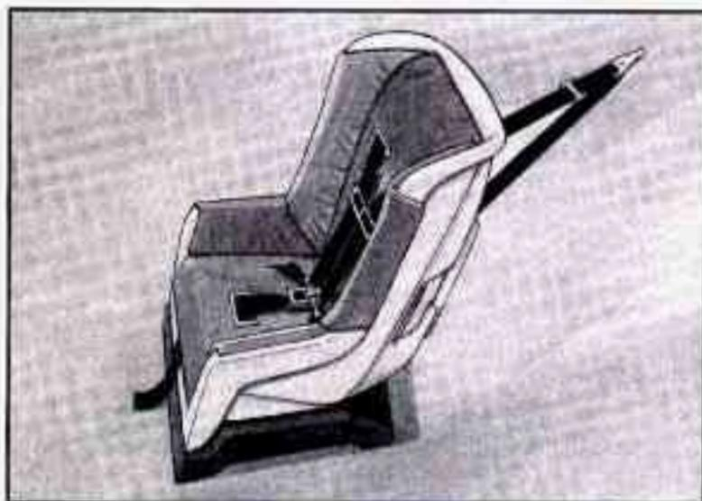
If your child restraint has a top strap, it should be anchored.
