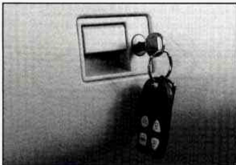
The glove box is directly in front of the front passenger seat. To lock the glove box door, insert the oval key into the lock cylinder and turn it clockwise a quarter turn and remove the key. To unlock the door, turn the key counterclockwise and remove the key.
