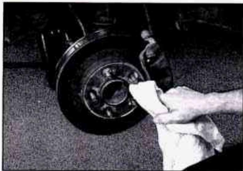
9. Remove any rust or dirt from the wheel bolts, mounting surfaces and spare wheel. Place the spare on the wheel mounting surface.
