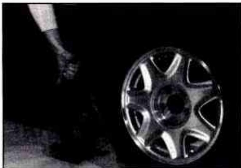
7. Raise the vehicle by rotating the wheel wrench clockwise. Raise the vehicle high enough off the ground so the tire can be removed.
