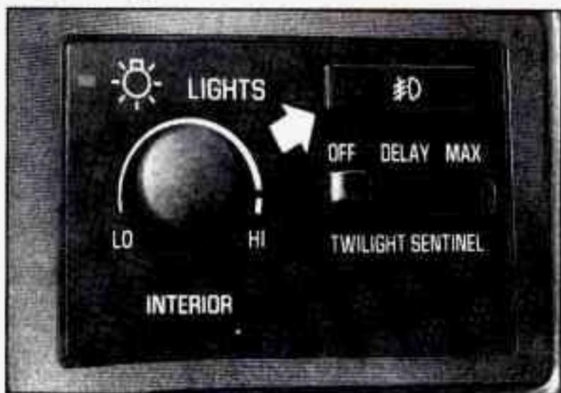
Use your fog lamps for better vision in foggy or misty conditions. When you press the upper fog lamp switch, a small indicator light will glow to tell you the fog lamps are on. To turn them off press the switch again.
