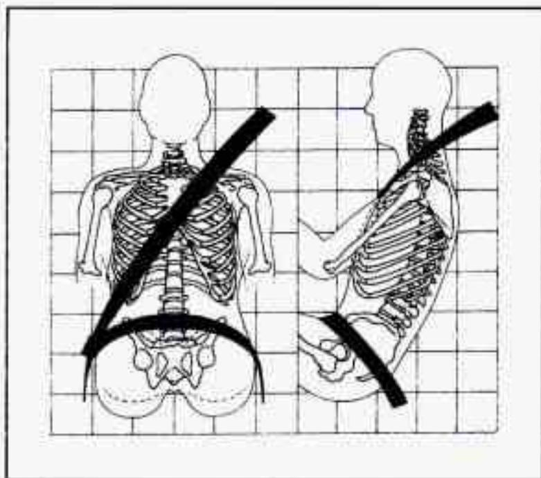
The lap part of the belt should be worn low and snug on the hips, just touching the thighs. In a crash, this applies force to the strong pelvic bones. And you'd be less likely to slide under the lap belt. If you slid under it, the belt would apply force at your abdomen. This could cause serious or even fatal injuries. The shoulder belt should go over the shoulder and across the chest. These parts of the body are best able to take belt restraining forces.
