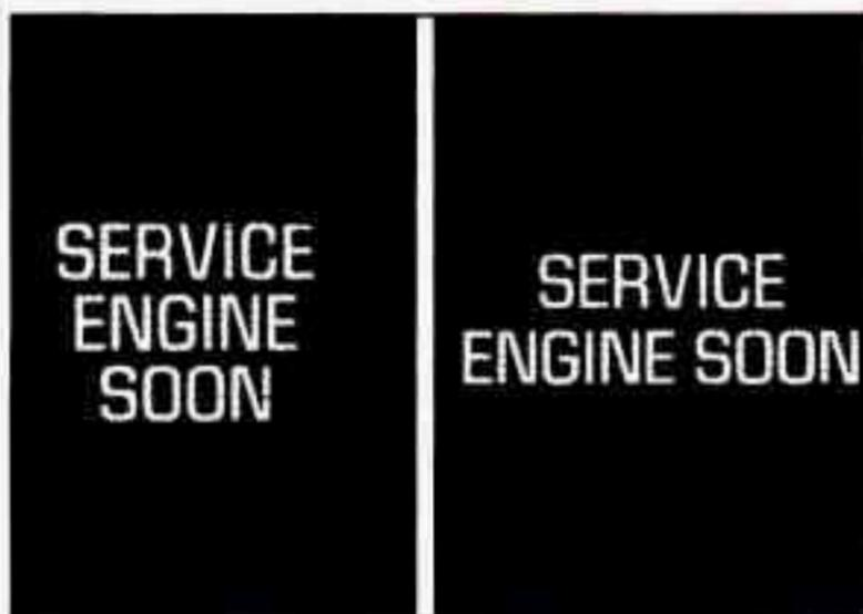
A computer monitors operation of your fuel, ignition and emission control systems. One of these lights should come on when the ignition is on, but the engine is not running, as a check to show you it is working. If the light doesn't come on, have it fixed right away. If it stays on or it comes on while you are driving, the computer is indicating that you have a problem. You should take your vehicle in soon for service.
