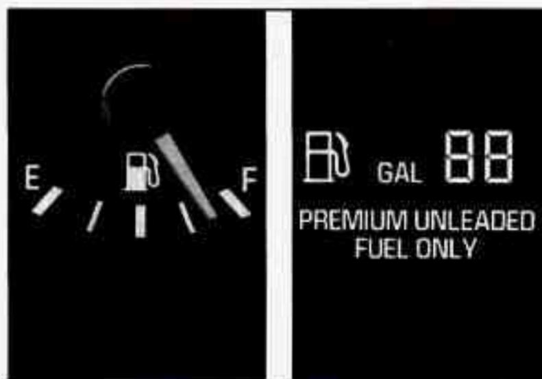
Your fuel gage shows approximately how much fuel is in your tank. It works only when the ignition is in the RUN position.
