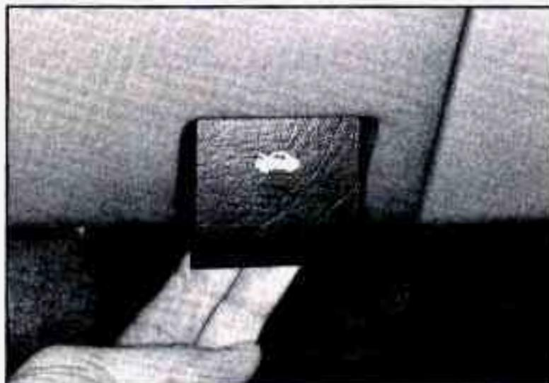
To open the hood, first pull the lever inside the vehicle, located at the lower left side of the instrument panel.
