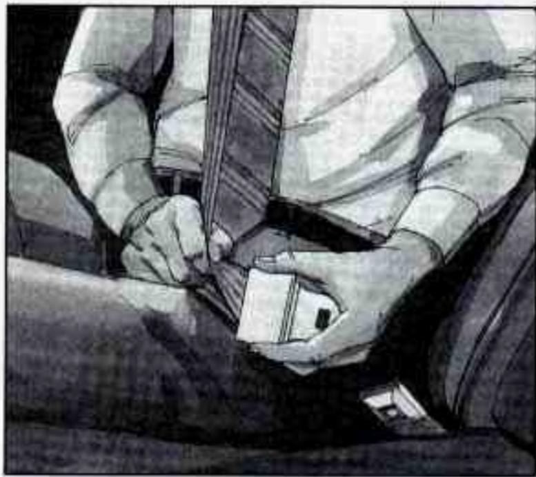
If the belt stops before it reaches the buckle, tilt the latch plate and keep pulling until you can buckle it.
