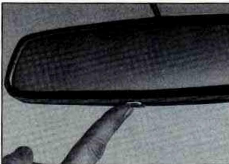
To turn the auto-dimming feature on press the switch located at the base of the mirror.
