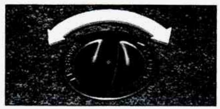
The equipment you'll need is in the trunk. Pull the carpeting from the floor of the trunk. Turn the center dial on the compact spare cover counterclockwise to remove it. Lift and remove the cover. (See "Compact Spare Tire" later in this section for more information about the compact spare.)
