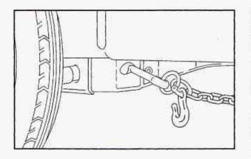
Attach T-hook chains on both sides, in the slotted holes in the bottom of the frame rails, behind the front wheels.
