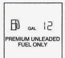
The fuel gage shows approximately how much fuel is in the tank. It works only when the ignition is in the RUN position.
