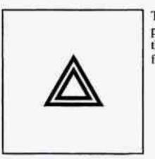
This light on the instrument panel will flash indicating that the hazard warning flashers are on.
