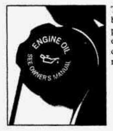
The oil fill cap is located behind the radiator on the passenger's side of the engine. Turn the cap counterclockwise to remove.
