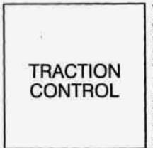
This warning light will come on to let you know if there's a problem with your traction control system. See "Traction Control System Warning Light" in the Index. When this warning light is on, the system will not limit wheel spin. Adjust your driving accordingly.
