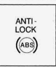
If there's a problem with the anti-lock brake system, this warning light will stay on. See "Anti-Lock Brake System Warning Light" in the Index.
