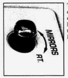
The control on the driver's door armrest operates both outside rearview mirrors. Rotate the control knob to choose the right or left mirror.
