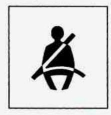
The safety belt light will also come on and stay on for about 20 seconds, then it will flash for about 70 seconds. If the driver's belt is already buckled, neither the chime nor the light will come on.
