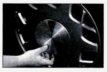
There is a center wheel cover on the aluminum wheel. Using the flat end of the wheel wrench, gently pry the wheel cover off. Be careful not to scratch the aluminum wheel edge and don't try to remove it with your hands.
