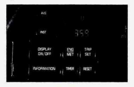
DISPLAY ON/OFF: Pressing this button will turn off the DIC, Electronic Climate Control, fuel data center, the fuel gage, trip odometer and odometer. While the displays are off, pressing the INFORMATION button will only turn on the DIC. If the TRIP SET button is pressed or the fuel level falls below four gallons (15.2 L), all the displays will come back on.
