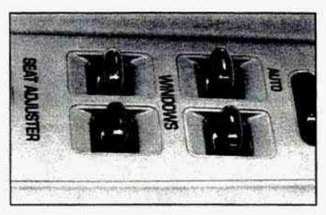
The controls are located near each window. Press the control forward to raise the window and press rearward to lower. Your vehicle has RAP. When you stop your vehicle and turn the ignition key to OFF, you can still use your power windows. The electrical power to operate the windows will not shut off until you open a door or 10 minutes have passed. If you want this power for another 10 minutes, turn the key to RUN and back to OFF.
