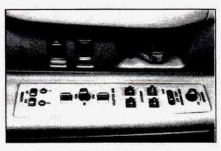
The power seat controls move and adjust the angle of the seat and they are located on the front doors.
