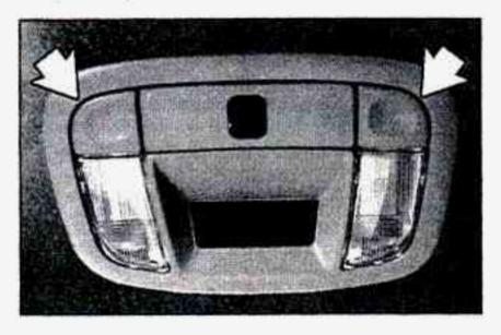
These lamps are located in the overhead panel. Press the button to turn them on. Press it again to turn them off.
