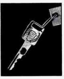
Your vehicle is equipped with the PASS-Key II theft-deterrent system. PASS-Key II is a passive system. The system is armed when the key is removed from the ignition.
