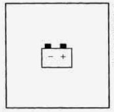
When you turn the key to RUN, this red light will come on briefly to show that the alternator and battery charging systems are working.
