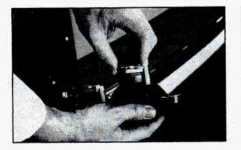
Press the bulb socket housing lever and rotate the socket counterclockwise to remove it.
