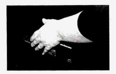
Close the door by sliding it all the way to the left. If the door is left partially open, the changer will not operate and an error will occur. When the door is closed, the changer will begin checking for discs in the magazine. This will continue for up to one and a half minutes depending on the number of discs loaded.
