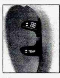
Some heating and cooling controls can be adjusted at the steering wheel. Other touch controls operate some audio controls. See "Steering Wheel Controls for Audio System" later in this section.
