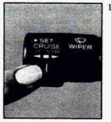
Move the cruise control switch to ON. 2. Accelerate to the speed you want.
