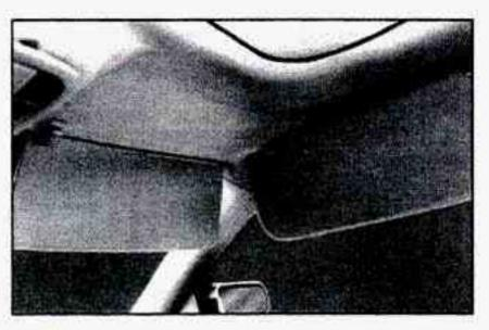
Swing down the visor to block out glare. It can also be detached from the center mount and moved to the side while the auxiliary sunshade remains to block glare from the front. Pull the front shade from the headliner and position it to your preference.
