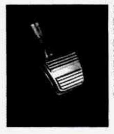
Hold the regular brake pedal down with your right foot and push down the parking brake pedal with your left foot to set the parking brake. If the ignition is on, the PARK BRAKE indicator light will come on.
