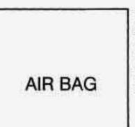
You will see this light flash for a few seconds when you turn your ignition to RUN or START. Then the light should go out. This means the system is ready.
