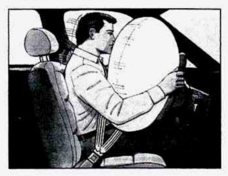
Where is the air bag? The driver's air bag is in the middle of the steering wheel.
