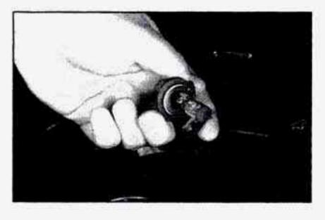
Disconnect the socket from the harness by separating the locking clip.
