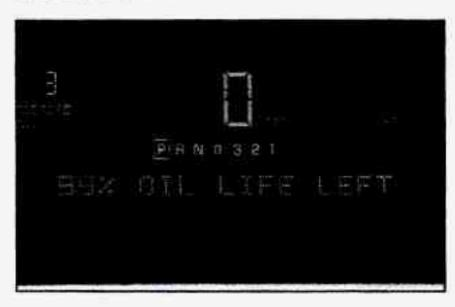
This feature lets you know when to change the engine oil. It's based on the engine oil temperatures and your driving patterns. To see the display, press the INFORMATION button several times until XX OIL LIFE LEFT appears. If you see 99% OIL LIFE LEFT, 99% of your current oil life remains.
