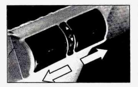
The direction of airflow to the rear seats can also be adjusted. Move the center lever to direct airflow toward the upper or floor outlets. To direct airflow from side to side, move the lever located in the center of each vent to the right or left.
