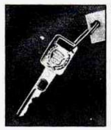
The square key is for the ignition only. It has a resistor pellet which is part of the vehicle's PASS-Key<sup>®</sup>II system.
