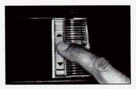
Turn the sunshade down and lift the cover to see the mirror. Move the slide switch up or down to brighten or dim the lamp.
