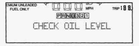
A CHECK OIL LEVEL message will appear when the engine oil is approximately a quart low. If the message is displayed, check the dipstick level and add oil as needed.
