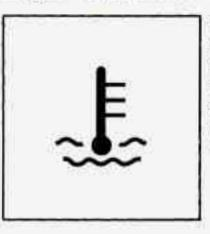
This red light tells you that your engine has overheated. You should stop the car and turn the engine off as soon as possible. A warning chime should also sound if this light comes on.
