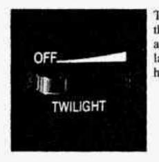
The control is next to the headlamp knob. It automatically switches the lamps on and off by sensing how dark it is outside.
