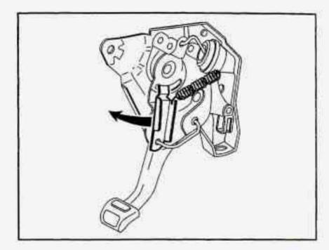
Reach under the driver's side of the instrument panel and pull on the manual release lever, which is located above the parking brake pedal. If the parking brake does not release, you will have to have your vehicle serviced.
