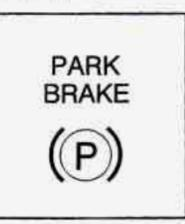
This light comes on when the parking brake is set, and it will stay on if the parking brake does not fully release. If you try to drive off with the parking brake set, this light will remain on.
