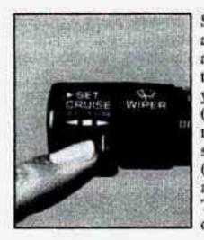
Setting the cruise control at a desired speed and then applying the brake will end the cruise function. Once you're going about 25 mph (40 km/h) or more, you can move the cruise control switch from ON to R/A (Resume/Accelerate) for about half a second to reset. This returns you to your desired preset speed.
