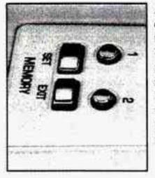
Adjust the driver's seat to a comfortable position and then press the SET button. Within five seconds, press the MEMORY button "1." A second seating position may be programmed by repeating the above steps and pressing the MEMORY button "2" instead of button 1.
