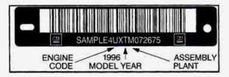
This is the legal identifier for your Cadillac. It appears on a plate in the front corner of the instrument panel, on the driver's side. You can see it if you look through the windshield from outside your vehicle. The VIN also appears on the Vehicle Certification and Service Parts labels and the certificates of title and registration.
