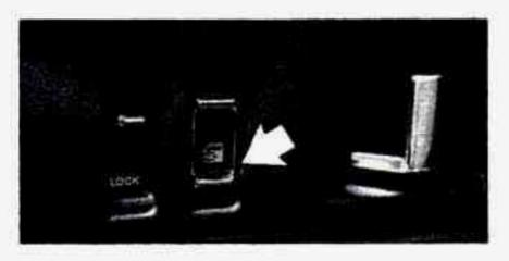
Press the power door lock to lock or unlock all the doors at once. The rear power door locks only provide a lock function as a safety feature. They will not unlock the doors.
