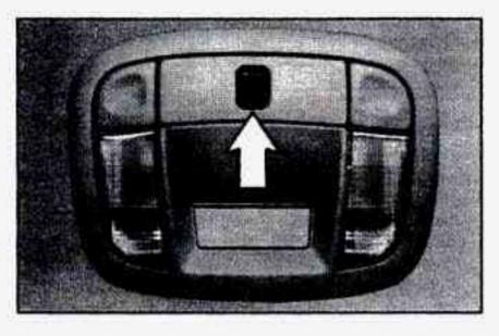
The express-open astroroof provides an airy, spacious feel to your vehicle's interior and can also increase ventilation. It includes a sliding glass panel and a sliding sunshade. The control switch only works when the ignition is on or when the Retained Accessory Power (RAP) is active.
