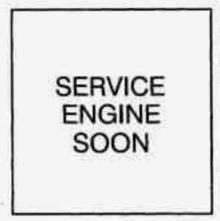
Your Cadillac is equipped with a computer which monitors operation of the fuel, ignition and emission control systems.
