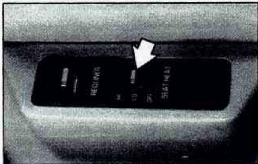
The control is located on the outboard side of each front seat. Move the SEAT HEAT control to either LO or HI to turn on the heating elements in the seat. The LO setting warms the seatback and cushion until the seat approximates body temperature. The HI setting heats the seat to a slightly higher temperature. A telltale light in the control reminds you that the heating system is in use. The heated seats can only be used when the ignition is turned on.
