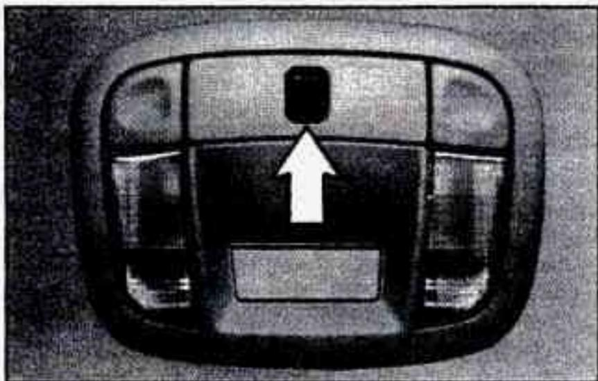
The express-open astrorooft provides an airy, spacious feel to your vehicle's interior and can also increase ventilation. It includes a sliding glass panel and a sliding sunshade. The control switch only works when the ignition is on or when the Retained Accessory Power (RAP) is active.
