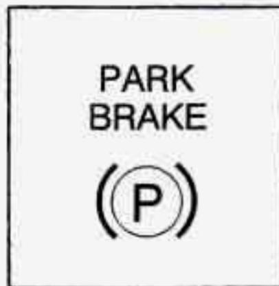
This light comes on when the parking brake is set, and it will stay on if the parking brake does not fully release. If you try to drive off with the parking brake set, this light will remain on.
