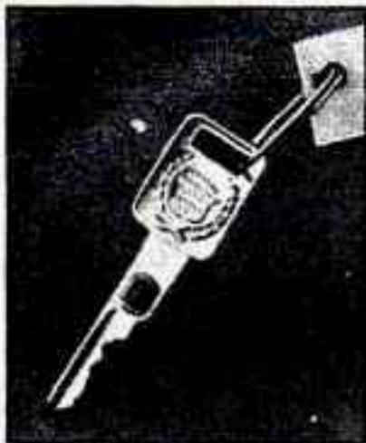
The square key is for the ignition only. It has a resistor pellet which is part of the vehicle's PASS-Key<sup>®</sup> II system.
