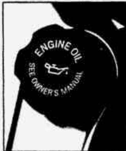
The oil fill cap is located behind the radiator on the passenger's side of the engine. Turn the cap counterclockwise to remove.
