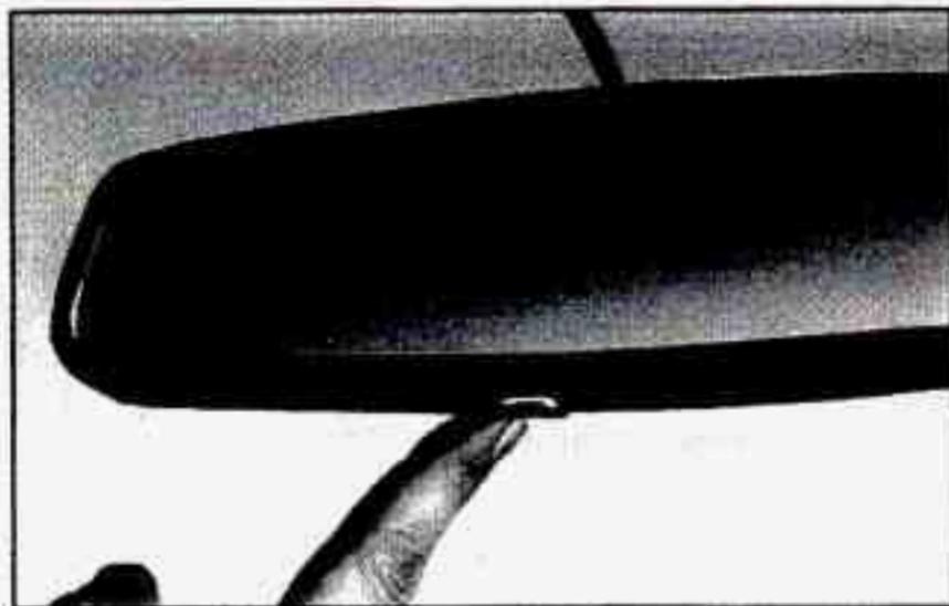
Press the button at the base of the mirror to turn on the automatic feature. The button has an indicator light to show it is on. Press the button to turn the automatic feature off.
