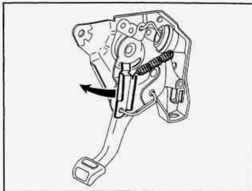
Reach under the driver's side of the instrument panel and pull on the manual release lever, which is located above the parking brake pedal. If the parking brake does not release, you will have to have your vehicle serviced.
