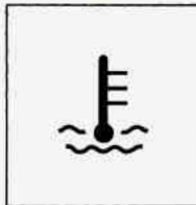
This red light tells you that your engine has overheated. You should stop the car and turn the engine off as soon as possible. A warning chime should also sound if this light comes on.
