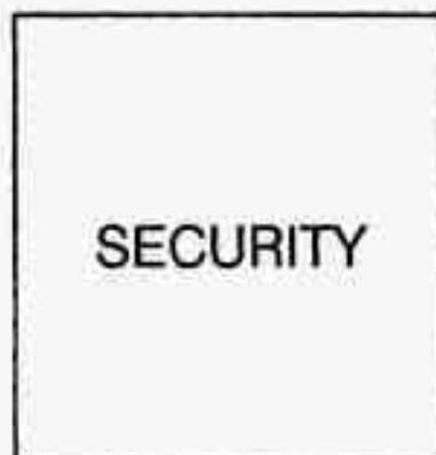
If your ignition is off and any door is open, the SECURITY light will flash reminding you to activate the system (the light will also flash if the battery has been disconnected or reconnected).
