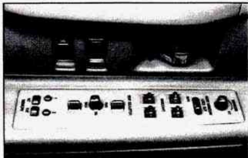
The power seat controls move and adjust the angle of the seat and they are located on the front doors.
