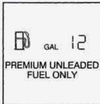
The fuel gage shows approximately how much fuel is in the tank. It works only when the ignition is in the RUN position.
