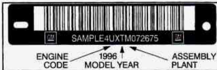
This is the legal identifier for your Cadillac. It appears on a plate in the front corner of the instrument panel, on the driver's side. You can see it if you look through the windshield from outside your vehicle. The VIN also appears on the Vehicle Certification and Service Parts labels and the certificates of title and registration.
