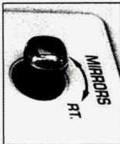
The control on the driver's door armrest operates both outside rearview mirrors. Rotate the control knob to choose the right or left mirror.
