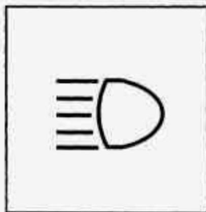
Pull the turn signal lever all the way toward you and then release it to change the headlamps from low beam to high or from high beam to low. The blue light on the instrument panel will be on indicating high beam usage.
