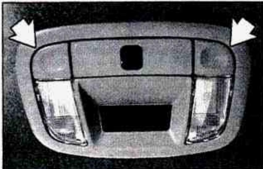
These lamps are located in the overhead panel. Press the button to turn them on. Press it again to turn them off.
