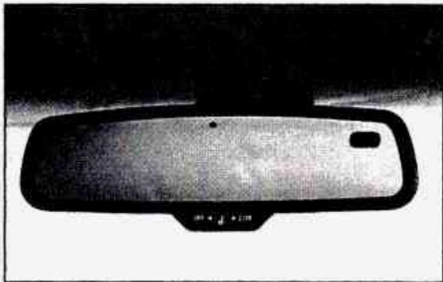
This mirror automatically changes to reduce glare when set in the **M** (Mirror) or **C/M** (Compass/Mirror) positions. One photocell on the back of the mirror senses when it is becoming dark outside. Another photocell is built into the mirror surface to sense headlamps behind you.
