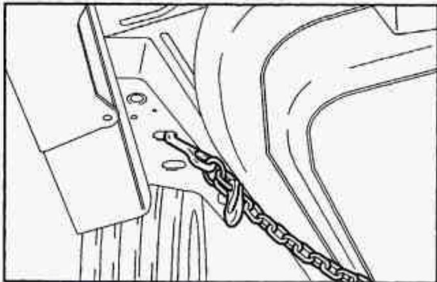
Attach R-hook chains to the R-hook slots in the frame rails just ahead of the rear wheels on both sides.
