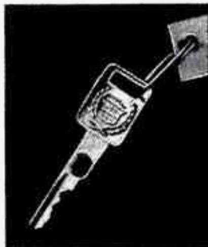
Your vehicle is equipped with the PASS-Key II theft-deterrent system. PASS-Key II is a passive system. The system is armed when the key is removed from the ignition.
