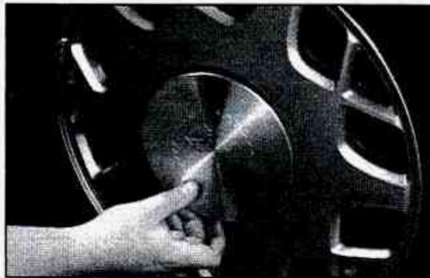
There is a center wheel cover on the aluminum wheel. Using the flat end of the wheel wrench, gently pry the wheel cover off. Be careful not to scratch the aluminum wheel edge and don't try to remove it with your hands.
