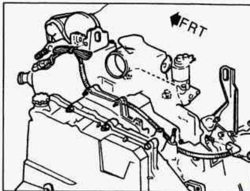
In very cold weather, 0°F (-18°C) or colder, the engine coolant heater can help. You'll get easier starting and better fuel economy during engine warm-up. Usually, the coolant heater should be plugged in a minimum of four hours prior to starting your vehicle.
