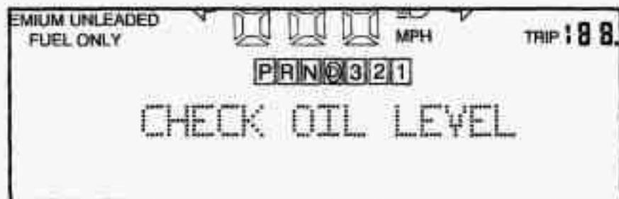
A CHECK OIL LEVEL message will appear when the engine oil is approximately a quart low. If the message is displayed, check the dipstick level and add oil as needed.
