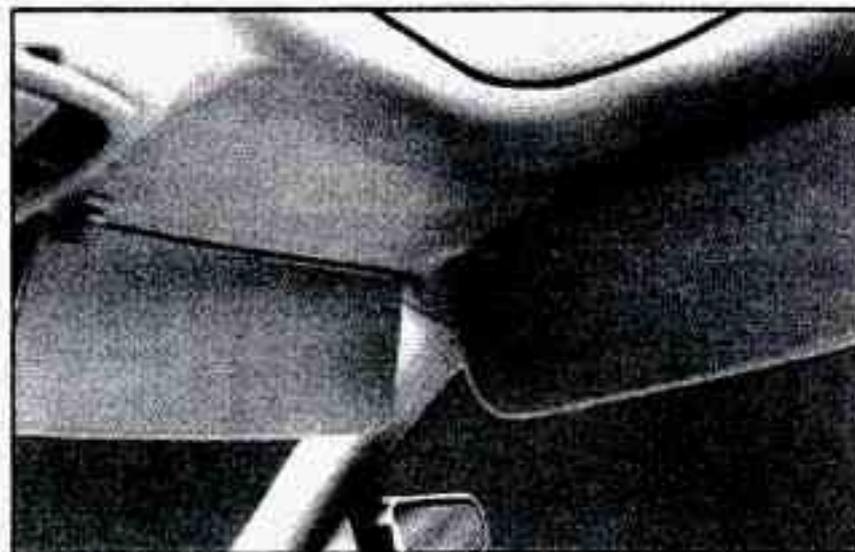
Swing down the visor to block out glare. It can also be detached from the center mount and moved to the side while the auxiliary sunshade remains to block glare from the front. Pull the front shade from the headliner and position it to your preference.
