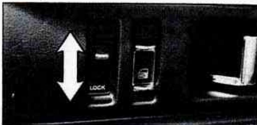
Slide the lock lever down to lock the door from the inside. To unlock the door, slide the lock lever up.
