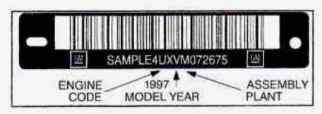
This is the legal identifier for your Cadillac. It appears on a plate in the front corner of the instrument panel, on the driver's side. You can see it if you look through the windshield from outside your vehicle. The VIN also appears on the Vehicle Certification and Service Parts labels and the certificates of title and registration.
