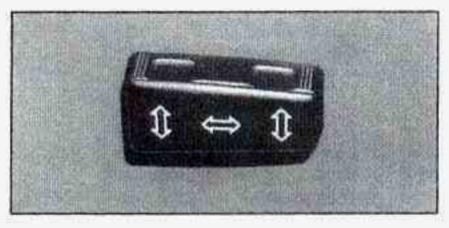
The power seat controls are located on the outboard side of the front seat cushion.
