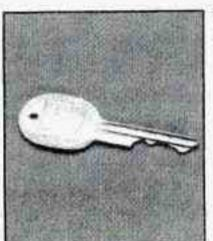
The oval key is for the doors and all other locks. When a new Cadillac is delivered, the dealer removes the plug from the door key. The plug has a code on it that tells the dealer or a qualified locksmith how to make extra keys. The ignition key has a bar code tag attached to it rather than a knock out plug. Your dealer or qualified locksmith can make extra ignition keys by reading the bar code tag.
