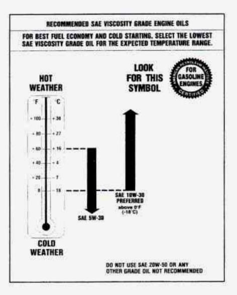
As shown in the chart, SAE 10W-30 is best for your vehicle. However, you can use SAE 5W-30 if it's going to be colder than 60°F (16°C) before your next oil change. When it's very cold, you should use SAE 5W-30. These numbers on an oil container show its viscosity, or thickness. Do not use other viscosity oils, such as SAE 20W-50.
