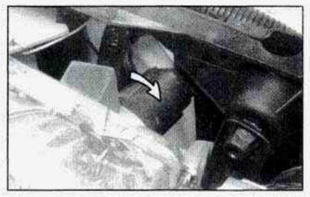
Turn the housing socket clockwise to unlock the socket from the lamp housing.
