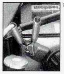
Don't let the other end of the positive cable touch metal. Connect it to the positive (+) terminal of the good battery.
