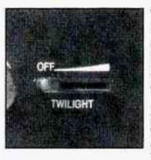
The control is next to the headlamp knob. It automatically switches the lamps on and off by sensing how dark it is outside.
