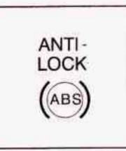
If there's a problem with the anti-lock brake system, this warning light will stay on. See "Anti-Lock Brake System Warning Light" in the Index.
