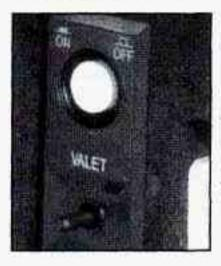
Pressing the VALET button located inside the glove box will disable the use of the trunk, fuel door and garage door opener. Pressing this button again will make these features reusable. Locking the glove box with the door key will also help to secure your vehicle.
