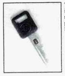
The square key is for the ignition only. It has a resistor pellet which is part of the vehicle's PASS-Key®II system.
