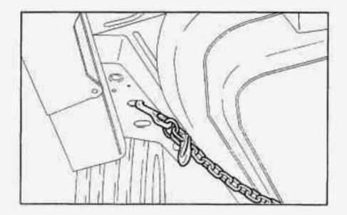
Attach R-hook chains to the R-hook slots in the frame rails just ahead of the rear wheels on both sides. These slots are to be used when loading and securing to car-carrier equipment.
