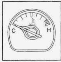
This gage shows the engine coolant temperature. If the gage pointer moves into the red area, the engine is too hot.
