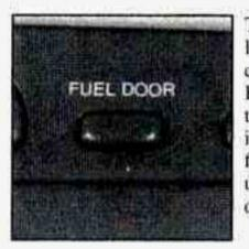
The fuel door release is located on the optional full console and on the Remote Keyless Entry (RKE) transmitter. If your vehicle is not equipped with the full console, then you must use the RKE transmitter to open the fuel door.
