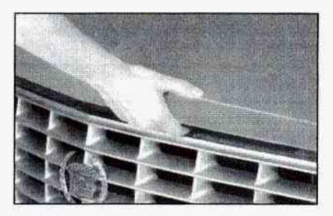
Then go to the front of the vehicle and find the secondary hood release which is located above the front grille. Lift up on the release lever as you raise the hood. When you open the hood, you'll see:
