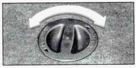
The equipment you'll need is in the trunk. Pull the carpeting from the floor of the trunk. Turn the retainer (center dial) on the compact spare cover counterclockwise to remove it. Lift and remove the cover. (See "Compact Spare Tire" later in this section for more information about the compact spare.)
