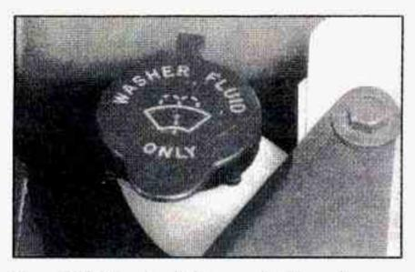
The windshield washer fluid reservoir is located next to the air cleaner on the driver's side of the engine. Open the cap labeled WASHER FLUID ONLY. Add washer fluid until the tank is full.
