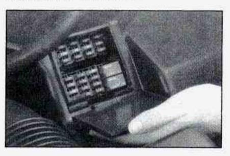
The fuse block is located next to the air cleaner on the driver's side of the engine. Lift the cover to gain access,
