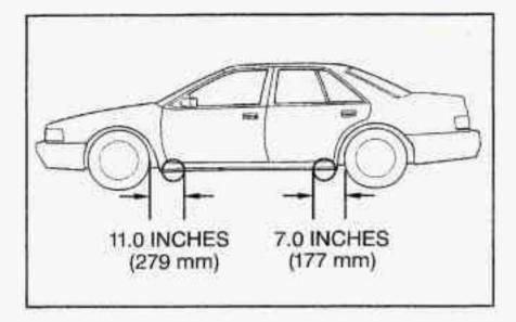
Position the jack under the vehicle and raise the jack lift head until it fits firmly into the notch in the vehicle's frame nearest the flat tire.
