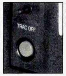
To turn the system off, press the TRAC OFF button located inside of the glove box.
