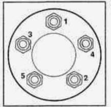
Tighten the wheel nuts firmly in a criss-cross sequence as shown.
