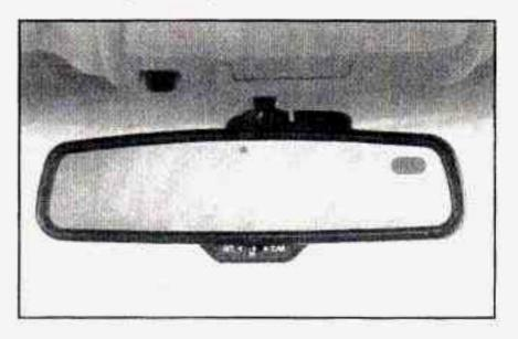
This mirror automatically changes to reduce glare when set in the M (Mirror) or C/M (Compass/Mirror) positions. One photocell on the back of the mirror senses when it is becoming dark outside. Another photocell is built into the mirror surface to sense headlamps behind you.
