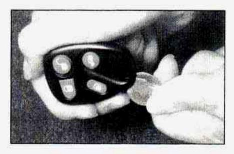
Use the round end of the door key or a coin to pry open the transmitter.
