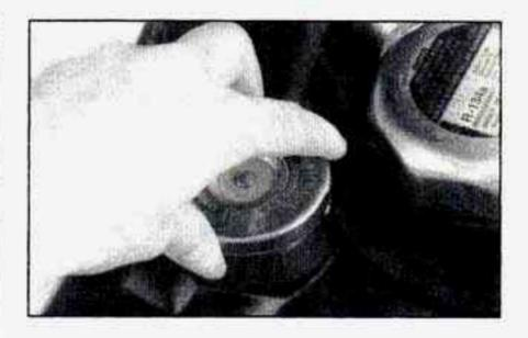
You can remove the coolant surge tank pressure cap when the cooling system, including the coolant surge tank pressure cap and upper radiator hose, is no longer hot. Turn the pressure cap slowly counterclockwise until it first stops. (Don't press down while turning the pressure cap.)
