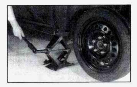
Lower the vehicle by turning the jack handle counterclockwise. Lower the jack completely.
