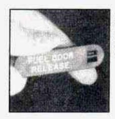
An alternate fuel door release is located inside of the trunk on the left hand side. Pull it to release the fuel door.
