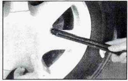
There is a center wheel cover on the aluminum wheel. Using the flat end of the wheel wrench, gently pry the wheel cover off. Be careful not to scratch the aluminum wheel edge and don't try to remove it with your bands. Removing the Flat Tire and Installing the Spare Tire
