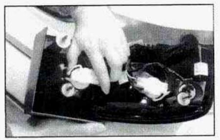
Press the bulb housing lever and rotate the housing counterclockwise to remove it. To remove the bulb, push and rotate it counterclockwise.
