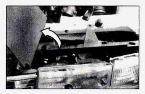
1. To access the headlamps, lift the cover off as shown.
