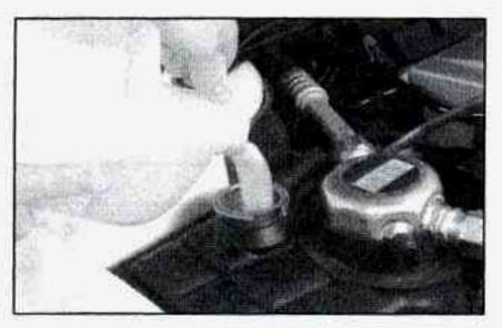
Then fill the coolant surge tank with the proper mix, up to the base of the filler neck.
