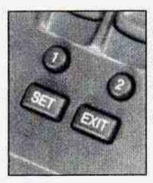
Adjust the driver's seat (including lumbar adjustments) and both outside mirrors to a comfortable position and then press the SET button. Within five seconds, press button "1."
