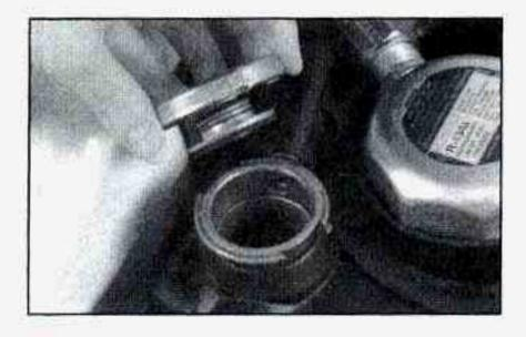
Then keep turning the cap, but now push down as you turn it. Remove the pressure cap.
