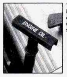
The engine oil dipstick is located behind the radiator on the driver's side of the engine. The black handle says ENGINE OIL on it.
