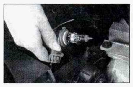
3. Remove the headlamp housing socket.
