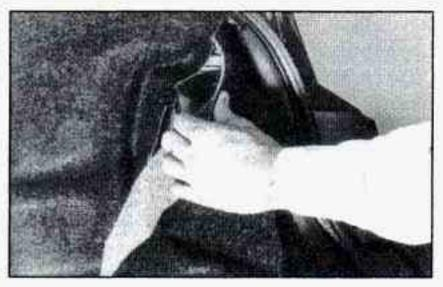
Remove the convenience net and pull trim away to access the wing nuts.
