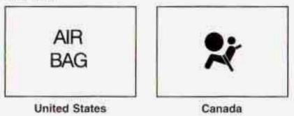
This light will come on when you start your vehicle, and it will flash for a few seconds. Then the light should go out. This means the system is ready. If the air bag readiness light stays on after you start the vehicle or comes on when you are driving, your air bag system may not work properly. Have your vehicle serviced right away.
