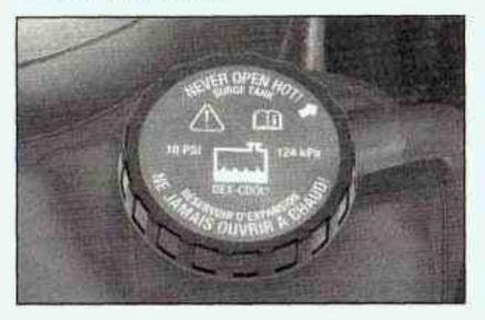
The engine coolant surge tank is located toward the rear of the engine compartment on the passenger's side of the vehicle. For more information on location, see *Engine Compartment Overview on page 5-12.*
