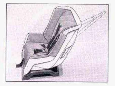
In Canada, the law requires that forward-facing child restraints have a top strap, and that the strap be anchored. In the United States, some child restraints also have a top strap. If your child restraint has a top strap, it should be anchored. Anchor the top strap to one of the following anchor points. Be sure to use an anchor point located on the same side of the vehicle as the seating position where the child restraint will be placed.
