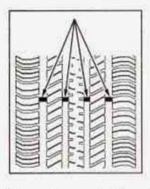
One way to tell when it's time for new tires is to check the treadwear indicators, which will appear when your tires have only 1/16 Inch (1.6 mm) or less of tread remaining.
