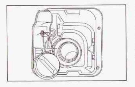
While refueling, hang the fuel cap by the tether from the hook on the filler door.
