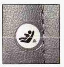
To assist you in locating the lower anchors for this child restraint system, each seating position with the LATCH system will have the LATCH system symbol on the seatback directly above the anchors. In order to use the system, you need either a forward-facing child restraint that has attaching points (B) at its base and a top tether anchor (C), or a rear-facing child restraint that has attaching points (B), as shown here.
