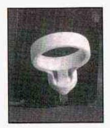
The engine oil dipstick is located behind the radiator on the driver's side of the vehicle. The handle is a yellow loop. For more information on location see Engine Compartment Overview on page 5-12. Turn off the engine and give the oil several minutes to drain back into the oil pan. If you don't, the oil dipstick might not show the actual level.
