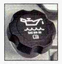
The engine oil fill cap is located behind the radiator on the passenger's side of the vehicle. For more information on location, see Engine Compartment Overview on page 5-12.
