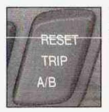
The trip odometer button is located to the left of the steering wheel on the instrument panel. The two trip modes are indicated by Trip A and Trip B. In order to change from one mode to the other, press the A/B portion of the TRIP button.
