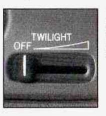
This lever is located next to the exterior lamp control. It automatically turns the lamps on and off by sensing how dark it is outside.
