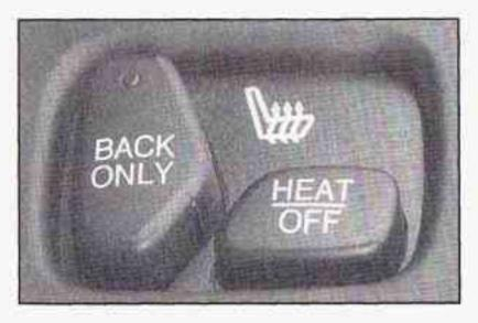
The buttons are located on the armrests. Press the buttons to turn the feature on. Press them again to turn off the heated seats. The feature will also shut off when the ignition is turned to OFF.
