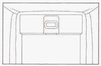
Your vehicle may be equipped with a small door in the rear seat. The door allows you to access the trunk from inside the vehicle.
