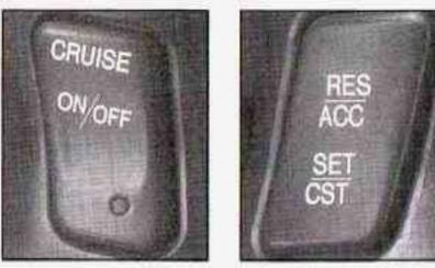
The buttons to operate cruise control are located on the steering wheel.
