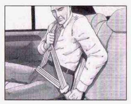
To make the lap part tight, pull down on the buckle end of the beit as you pull up on the shoulder part.
