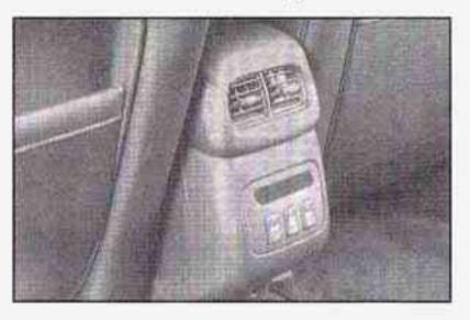
Your vehicle has a rear climate-control system that allows the rear-seat passengers to adjust the direction of the airflow, the fan speed and the temperature for the rear-seating area. This system also works with the main climate-control system in your vehicle.
