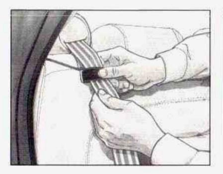
Slide the guide under and past the belt. The elastic cord must be under the belt. Then, place the guide over the belt, and insert the two edges of the beit into the slots of the guide.
