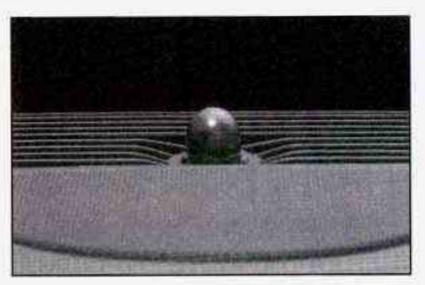
The light sensor for the DRL and the Twilight Sentinel<sup>®</sup> is located in the center of the front defogger grille. If you cover the sensor, it will read "dark" and the exterior lamps or the HEADLAMPS SUGGESTED message will be displayed whenever the ignition is on.
