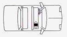
If your child restraint is equipped with the LATCH system, see Lower Anchorages and Top Tethers for Children (LATCH System) on page 1-41. Your vehicle has a right front passenger air bag. Never put a rear facing child restraint in this seat. Here's why:
