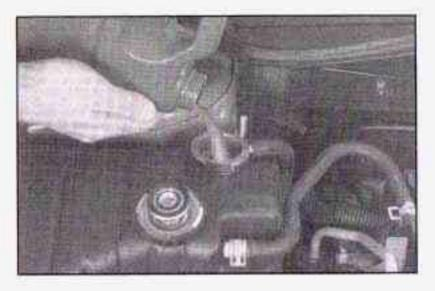
Then fill the coolant surge tank with the proper mixture to the full cold fill mark on the side of the coolant surge tank.
