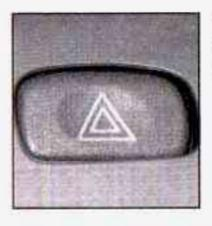
The hazard warning button is located on the center of the instrument panel between the two air vents.
