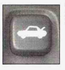
The trunk lock release button is located to the left of the steering wheel on the instrument panel.
