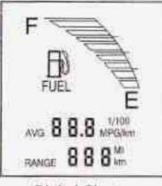
The fuel gage shows approximately how much fuel is in the tank. It works only when the ignition is in ON.
