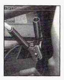
Now connect the black negative (-) cable to the negative (-) terminal location of the vehicle with the good battery. Use a remote negative (-) terminal if the vehicle has one.
