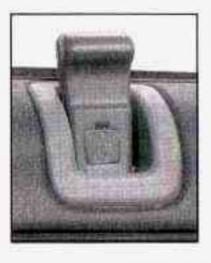
From the inside, use the manual lock levers located at the top of the door panel near the window.
