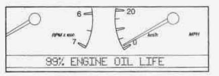
This feature lets you know when to change the engine oil. It's based on the engine oil temperatures and your driving patterns. To see the display, press the INFO button several times until ENGINE OIL LIFE appears. If you see 99% ENGINE OIL LIFE, 99 percent of your current oil life remains.
