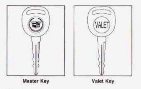
There is a master key that works all of the lock cylinders (driver's door, trunk, ignition and glove box).
