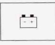
When you turn the key to ON or START, this light will come on briefly to show that the generator and battery charging systems are working properly.
