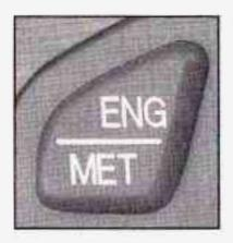
By pressing this button located to the left of the steering wheel on the instrument panel, you can go back and forth from English (miles) to metric (kilometers).
