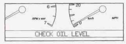
If the CHECK OIL LEVEL message appears on the instrument cluster, it means you need to check your engine oil level right away. For more information, see "CHECK OIL LEVEL" under *DIC Warnings and Messages on page 3-60.*
