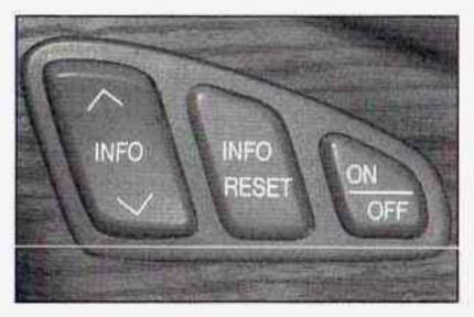
The Driver Information Center (DIC) buttons are located to the right of the steering wheel on the instrument panel, near the air outlets. ∧ INFO ∨ (Information): Pressing this button up or down will display the MILES RANGE (Analog Cluster), MPG AVG, MPG INST, GAL FUEL USED, AVG MPH, TIMER, BATTERY VOLTS, LF-RF-LR-RR TIRE (If Equipped), RPM TACHOMETER (Digital Cluster), ENGINE OIL LIFE, TRANS FLUID LIFE, PHONE (If Equipped), FEATURE PROGRAMMING and Blank Display.
