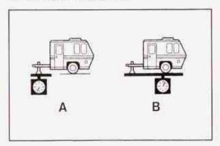
If you're using a weight-carrying hitch or a weight-distributing hitch, the trailer tongue (A) should weigh 10 – 15 percent of the total loaded trailer weight (B).
