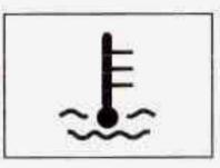
This light tells you that your engine has overheated. As a check, the light should come on for a few seconds when you start your engine.
