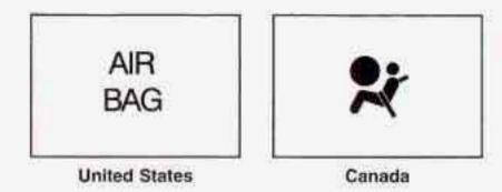
There is an air bag readiness light on the instrument panel, which shows the words AIR BAG or an air bag symbol.
