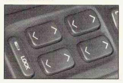
The power window switches are located on the armrest near each window. Press the up or down arrows on the switches to raise or lower the windows. Your vehicle has Retained Accessory Power (RAP) that allows you to use the power windows once the ignition has been turned off. For more information, see "Retained Accessory Power" under *Ignition Positions* on page 2-23.
