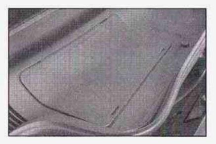
The access panel for the passenger compartment air filter is located under the hood near the windshield, on the passenger's side of the vehicle.
