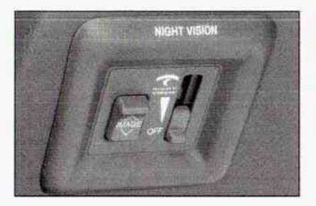
The controls for this feature are located to the left of and below the steering wheel. They are used to adjust the brightness and location of the image. Adjust the IMAGE control so the image is as low as possible while remaining visible.
