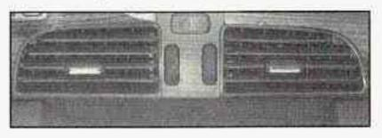
Use the levers located in the center of each outlet to change the direction of the airflow. Use the thumbwheels to open or close the outlets.
