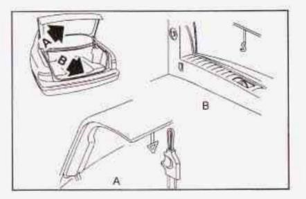
Your vehicle may be equipped with a trunk-lid tie down. This feature is used to secure the trunk lid if it will not close completely, such as when carrying large packages in the trunk. Use the following steps to secure the trunk lid:
