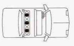
Your vehicle has the LATCH system. You'll find anchors (A) in all three rear seating positions.
