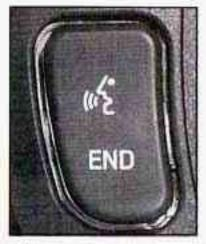
The controls are located on the left side of the steering wheel. Press the top part of the control to access OnStar<sup>®</sup>. You will hear a ready prompt from the system, and then you can begin your OnStar<sup>®</sup> session or begin making calls.
