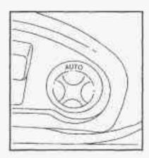
If your vehicle has this feature, the control is located on the outboard side of each front seat. It is marked AUTO.
