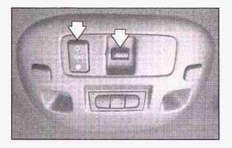
Your vehicle may have a sunroof. The two switches that operate the sunroof are located on the overhead console and include VENT, ROOF, open and close.
