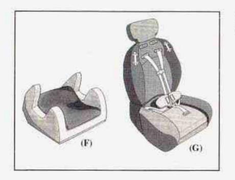
A booster seat (F-G) is a child restraint designed to improve the fit of the vehicle's safety belt system. Some booster seats have a shoulder belt positioner, and some nigh-back booster seats have a five-point namess. A booster seat can also help a child to see out the window.
