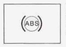
If there's a problem with the anti-lock brake system, this warning light will stay on. See Anti-Lock Brake System Warning Light on page 3-48.
