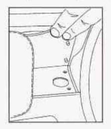
The console shift lock release is located on the front of the center console.
