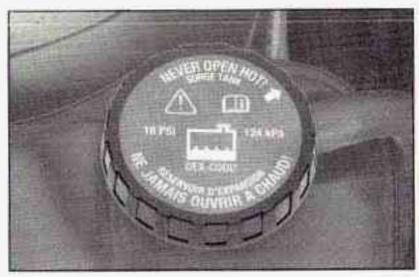
Then replace the pressure cap. Be sure the arrow on the pressure cap lines up like this.
