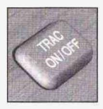
To turn the system off, press the TRAC ON/OFF button located on the center console. (For vehicles with a column shift lever, the button is located at the end of the shift lever.)
