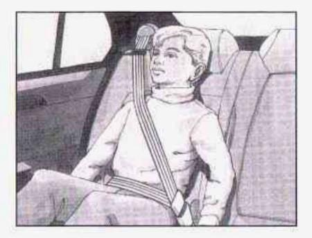
Buckle, position and release the safety belt as described in *Rear Seat Passengers on page 1-22*. Make sure that the shoulder belt crosses the shoulder.
