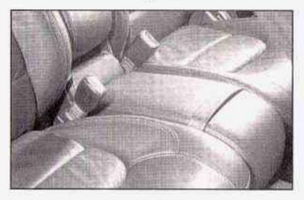
Your vehicle may be equipped with a center flex storage unit that includes a front center seat with a lap belt and an underseat storage compartment. The center seatback can also be used as a fold down armrest with extra space for CDs or tapes. An optional cellular telephone may be located in the underseat storage compartment. Cupholders are also located at the front edge of the storage unit and can be accessed by pulling the strap and folding the compartment forward.
