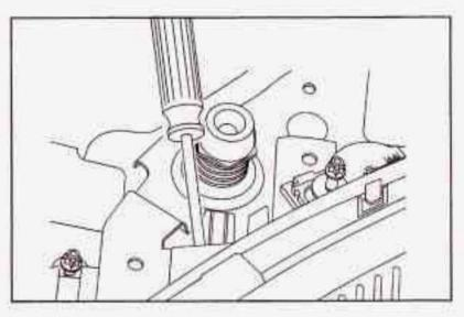
Use a tool to help pry the headlamp assembly away from the vehicle.
