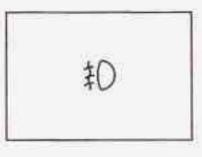
This light will come on when the fog lamps are in use. It will go out when the fog lamps are turned off.
