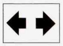
An arrow on the instrument panel cluster and in the outside rearview mirror will flash in the direction of the turn or lane change.
