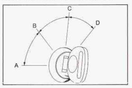
Notice: If your key seems stuck in OFF and you can't turn it, be sure you are using the correct key; if so, is it all the way in? If it is, then turn the steering wheel left and right while you turn the key hard. Turn the key only with your hand. Using a tool to force it could break the key or the ignition switch. If none of these works, then your vehicle needs service.
