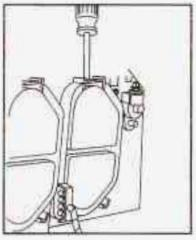
Remove the bulb socket dust cover.
