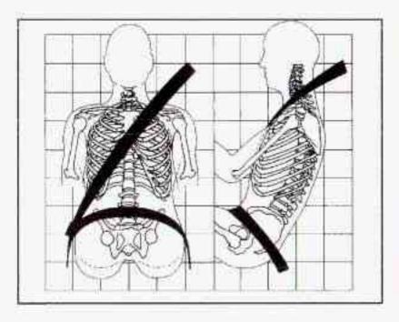
The lap part of the belt should be worn low and snug on the hips, just touching the thighs. In a crash, this applies force to the pelvic bones. And you'd be less likely to slide under the lap belt. If you slid under it, the belt would apply force at your abdomen. This could cause serious or even fatal injuries. The shoulder belt should go over the shoulder and across the chest. These parts of the body are best able to take belt restraining forces.
