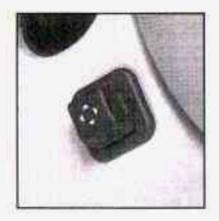
If your vehicle has this feature, the power tilt wheel control is located on the outboard side of the steering column.
