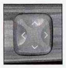
The rear lumbar support controls are located on the rear door trim panels. To activate the rear lumbar support feature, push forward on the control to increase support or rearward to decrease support. The lumbar control can also be moved up and down to adjust the location of the support.
