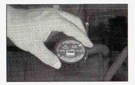
Park the vehicle on a level surface. You can remove the coolant surge tank pressure cap when the cooling system, including the coolant surge tank pressure cap and upper radiator hose, is no longer hot. Turn the pressure cap slowly counterclockwise (left) until it first stops. (Don't press down while turning the pressure cap.)
