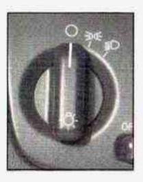
The exterior lamp control is located to the left of the steering wheel on the instrument panel.
