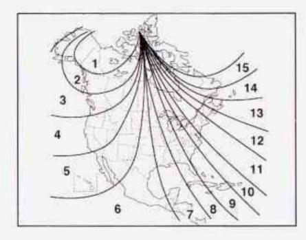
Once the zone number appears in the display, press the on/off button quickly until the correct zone number appears in the display. Stop pressing the button and the mirror will return to normal operation. If C appears in the compass window, the compass may need calibration. See Compass Calibration listed previously.
