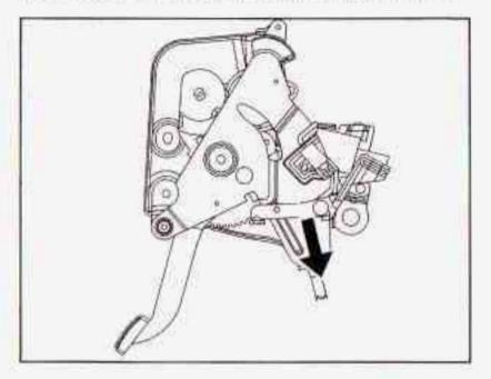
Reach under the driver's side of the instrument panel and pull down on the manual release lever, which is located behind the parking brake pedal. Pull down on the yellow tab as shown by the arrow in the illustration. If the parking brake does not release, you should have your vehicle towed to your dealer for service. Notice: Driving with the parking brake on can cause your rear brakes to overheat. You may have to replace them, and you could also damage other parts of your vehicle.
