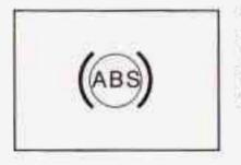
With the anti-lock brake system, the light(s) will come on when your engine is started and may stay on for several seconds. That's normal.
