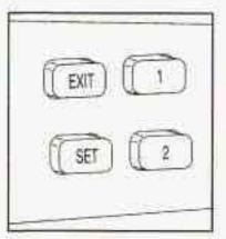
Your vehicle may be equipped with the memory package. The controls for these features are located on the driver's door panel, and are used to program and recall memory settings for the driver's seating positions.
