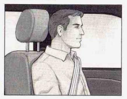
Adjust your head restraint so that the top of the restraint is closest to the top of your head. This position reduces the chance of a neck injury in a crash. The front head restraints are adjustable. Lift up or push down on the head restraint to raise or lower it. Pull forward or push rearward on the head restraint to tilt it forward or rearward.
