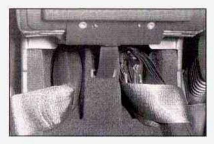
When not being used, the center seat iap belt can be stored in the underseat storage compartment as shown.
