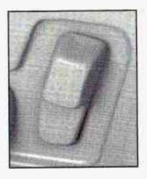
The recliner controls are located on the outboard sides of the front seats.
