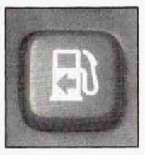
The fuel door release button is located to the left of the steering wheel next to the exterior lamp control
