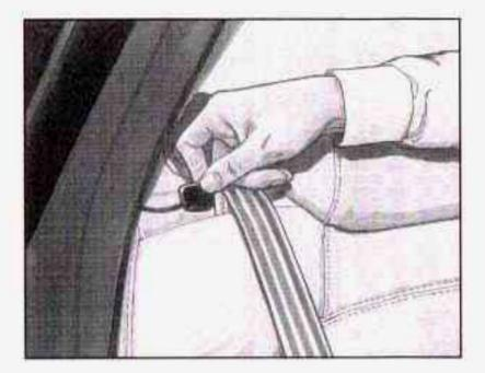
Remove the guide from its storage pocket on the top of the seatback.
