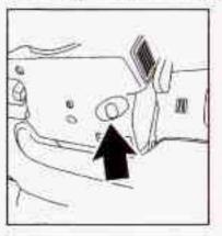
Locate the override access slot underneath the steering column below the lock cylinder. The following procedure applies only to vehicles equipped with the console shift lever and is used to shift the transaxie out of PARK (P) in case of a dead battery or low voltage battery.
