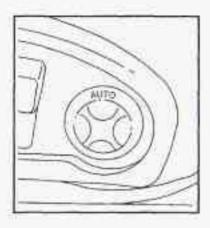
If your vehicle has this feature, the control is located on the outboard sides of the front seats. With the ignition on, briefly press the top of the control where it is marked AUTO to activate the massaging lumbar feature.
