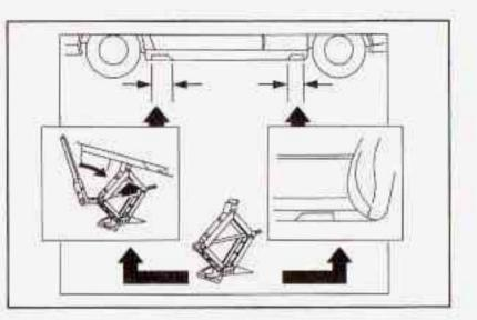
Find the jacking location from the diagrams above and corresponding hoisting notches located in the plastic molding. The front location is 8.5 inches (21 cm) from the rear edge of the front wheel well, and the rear location is 3.5 inches (8.5 cm) from the front edge of the rear wheel well.
