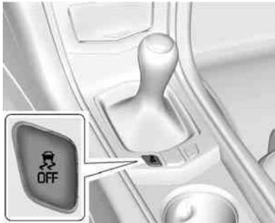
Manual Transmission TCS/ StabiliTrak Button Shown, Automatic Transmission TCS/ StabiliTrak Button Similar
