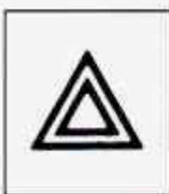
Hazard Warning Flasher
