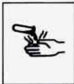
Caustic Battery Acid Could Cause Burns
