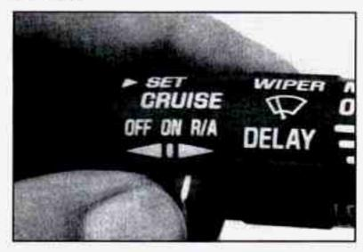
Once you're going about 25 mph (40 km/h) or more, you can move the Cruise Control switch from ON to R/A (Resume/Accelerate) for about half a second.
