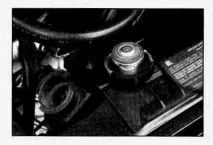
Put the cap back on the coolant recovery tank, but leave the radiator pressure cap off.
