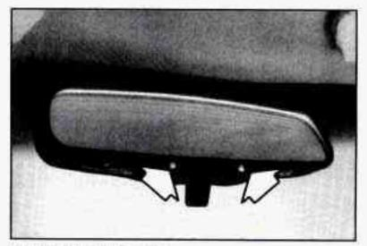
You can also turn the map lamps on and off by pressing the switch near each light.
