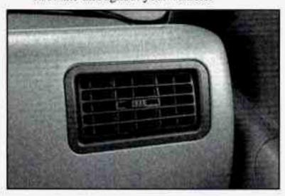
You will find air vents in the center and on the sides of your instrument panel. You can move the vents to direct the flow of air, or close the vents altogether. When you close a vent, it will increase the flow of air coming out of any vents that are open.
