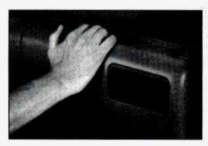
To open your glove box, squeeze the lever at the top of the glovebox and lower the door.
