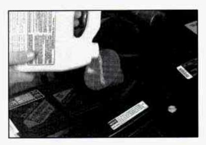
Fill the radiator with the proper mix, up to the base of the filler neck.
