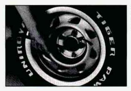
Using the wheel wrench, loosen all the wheel nuts. Don't remove them yet.
