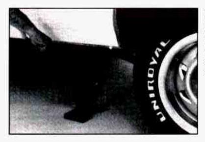
Raise the vehicle by turning the jackhandle clockwise. Raise the vehicle far enough off the ground so there is enough room for the spare tire to fit.
