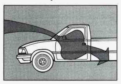
Your vehicle's ventilation system supplies outside air to the inside of your vehicle when it is moving. With the side windows closed, air will flow into the front air inlet grilles, through the vehicle, and out the rear air exhaust valve. Outside air will also enter the vehicle when the heater or the air conditioning fan is running.
