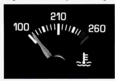
This gage shows the engine coolant temperature. If the gage pointer moves into the red area, your engine is too hot!
