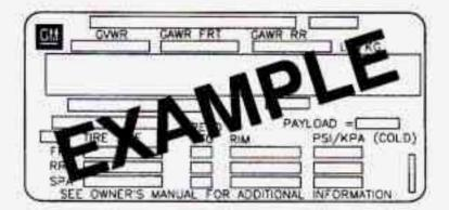
The Certification/Tire label is found on the driver's door lock pillar. The label shows the size of your original tires and the inflation pressures needed to obtain the gross weight capacity of your vehicle. This is called the GVWR (Gross Vehicle Weight Rating). The GVWR includes the weight of the vehicle, all occupants, fuel, cargo and trailer tongue weight, if pulling a trailer.
