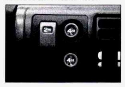
If your four-wheel drive vehicle has the electronic transfer case, the transfer case switches are on the right side of your instrument panel above the radio controls.
