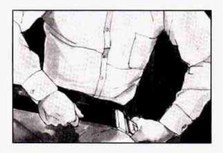
To make it shorter, pull the belt as shown until it is snug. Buckle and position it the same way as the lap part of the driver's safety belt (see "Driver Position" in the Index). Make sure the release button on the buckle is positioned so you would be able to unbuckle the safety belt quickly if you ever had to. To unlatch the belt, just push the button on the buckle.
