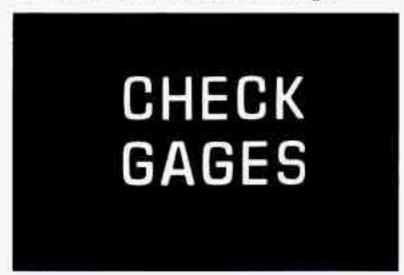
This amber CHECK GAGES indicator light is above the fuel gage on the instrument cluster and will come on briefly when you are starting the engine.
