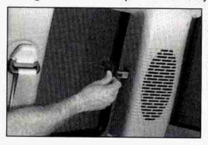
To open a rear swing—out window, pull the latch toward the front of the vehicle and then push the latch out and rearward. When you close the window, be sure the latch catches.
