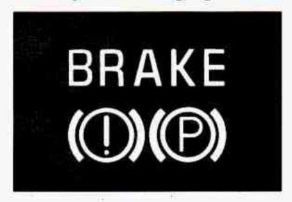
Your vehicle's hydraulic brake system is divided into two parts. If one part isn't working, the other part can still work and stop you. For good braking, though, you need both parts working well.
