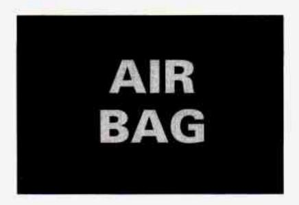
There is an air bag readiness light on the instrument panel, which shows AIR BAG. The system checks the air bag's electrical system for malfunctions. The light tells you if there is an electrical problem. See "Air Bag Readiness Light" in the Index for more information.
