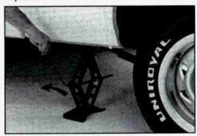
Lower the vehicle by turning the jackhandle counterclockwise. Lower the jack completely.
