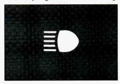
This blue high-beam indicator light is above the engine oil temperature gage on the instrument cluster and is on whenever you use your high beam headlamps. See "Headlamp High-Low Beam Changer" in this section.
