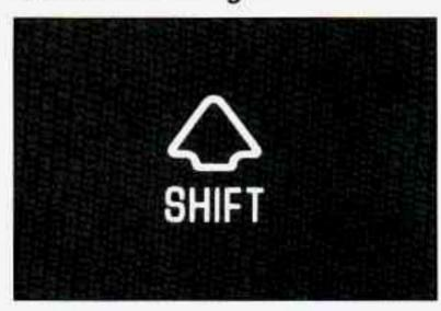
This amber SHIFT indicator light is at the top of the instrument cluster of vehicles with manual transmissions. Shifting when the indicator light is on will help you get the best fuel economy. See "SHIFT Light" in this section.
