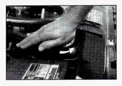
2. Then keep turning the pressure cap, but now push down as you turn it. Remove the pressure cap.
