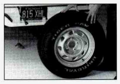
When the tire has been completely lowered, tilt the retainer at the end of the cable and pull it through the wheel opening. Pull the tire out from under the vehicle.
