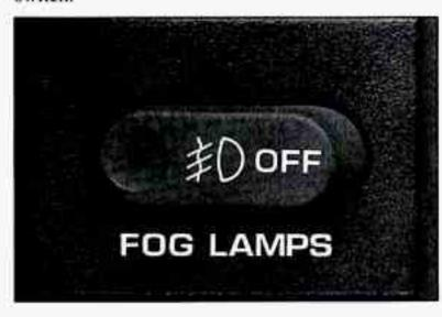
Press the side of the switch with the light to turn the fog lamps on, and OFF to turn them off. A light will glow in the switch when the fog lamps are on.
