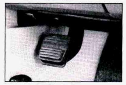
Hold the regular brake pedal down with your right foot. Push down the parking brake pedal with your left foot. If the ignition is on, the brake system warning light will come on.
