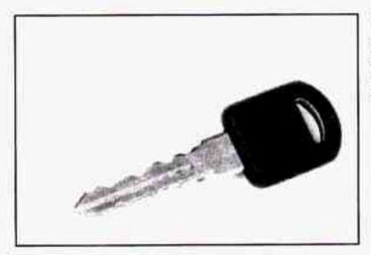
This vehicle has one double-sided key for the ignition and door locks. It will fit with either side up.
