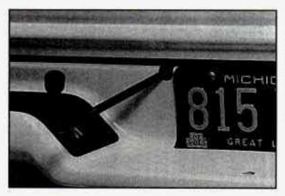
Insert the chisel end of the wheel wrench, on an angle, into the hole in the rear bumper. Be sure the chisel end of the wheel wrench connects into the hoist shaft.
