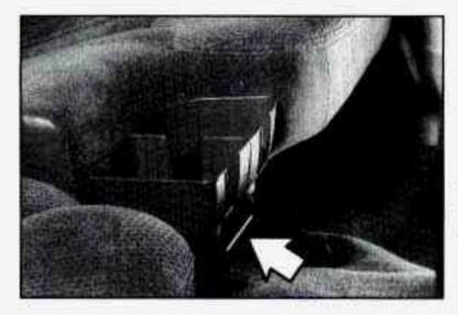
Cupholders are on the front of split-bench seats. Squeeze the latch at the front of the cupholder and pull it straight out. The liner removes for easy cleaning and the cupholder is dishwasher safe.
