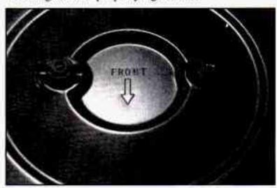
To avoid ingesting dust in the engine, the arrow on the air cleaner lid should point to the front of the engine.
