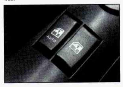
Push the side of the switch with the down arrow to lower the window.
