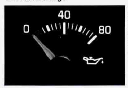
The oil pressure gage shows the engine oil pressure in psi (pounds per square inch) when the engine is running. Canadian vehicles indicate pressure in kPa (kilopascals).
