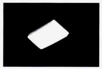
The dome lamp will come on when the side doors are opened. You can also turn the dome lamp on by turning the INT LIGHTS dimmer switch up until it clicks.
