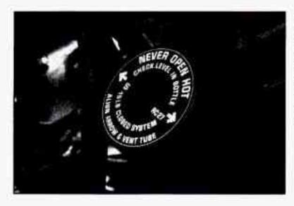
When you replace your radiator pressure cap, a GM cap is recommended. See "Service Replacement Part and Filter Recommendations" in the Index.
