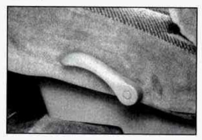
To adjust the seatback, lift the lever on the outer side of the seat. Release the lever to lock the seatback where you want it. Pull up on the lever and the seat will go to an upright position.
