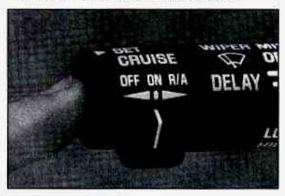
Use the accelerator pedal to get to the higher speed. Push the button at the end of the lever, then release the button and the accelerator pedal. You'll now cruise at the higher speed.
