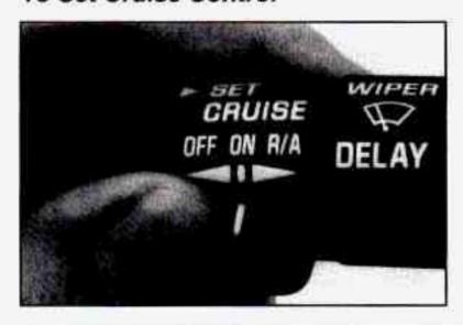
Move the Cruise Control switch to ON.
