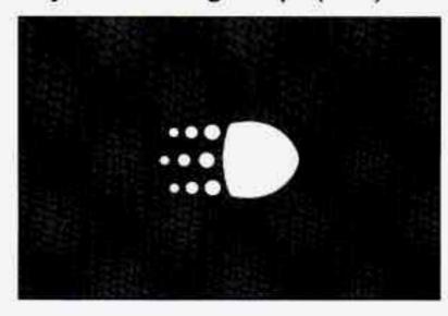
You may have this light on the instrument panel. It goes on whenever the Daytime Running Lamps are on, the ignition is on, the headlamp switch is off, and the parking brake is released.
