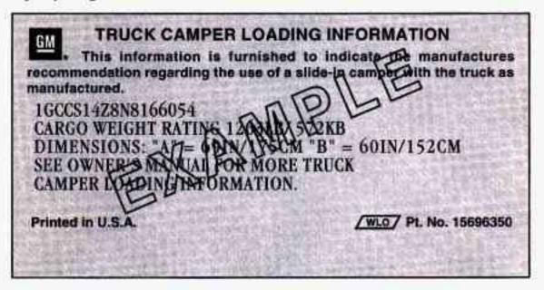
This label will tell you if your vehicle can carry a slide—in camper, how much of a load your vehicle can carry, and how to spread out your load the right way. Also, it will help you match the right slide—in camper to your vehicle.
