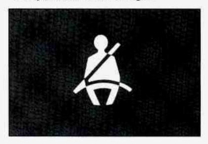
When the key is turned to RUN or START, a tone will come on for about eight seconds to remind people to fasten their safety belts, unless the driver's safety belt is already buckled. The safety belt light will also come on and stay on for about 20 seconds, then it will flash for about 55 seconds. If the driver's belt is already buckled, neither the tone nor the light will come on.
