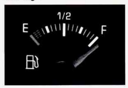
The fuel gage tells you about how much fuel you have remaining when the ignition is on. When the gage first indicates empty, you still have a little fuel left, but you should get more fuel SOOTI.
