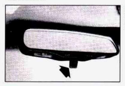
Press the tab under the mirror to reduce glare from headlamps behind you.
