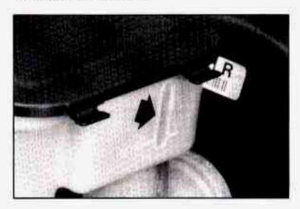
You can check the brake fluid without taking off the cap. Just look at the windows on the brake fluid reservoir. The fluid levels should be above MIN. If they aren't, have your brake system checked to see if there is a leak.
