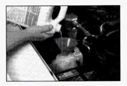
Then fill the coolant recovery tank to the ADD mark.
