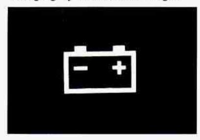
The red charging system indicator light is above your oil temperature gage on your instrument cluster and will come on briefly when you turn on the ignition, but the engine is not running, as a check to show you it is working.
