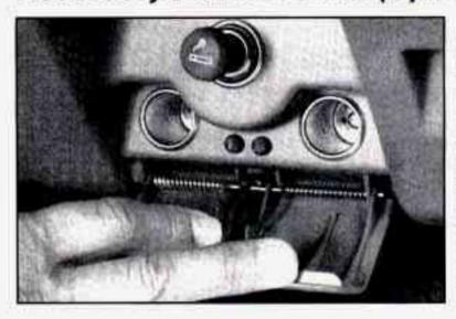
If you have accessory power outlets, you can plug in auxiliary electrical equipment. Just pull down from the top of the door and follow the proper installation instructions that are included with any electrical equipment you install.
