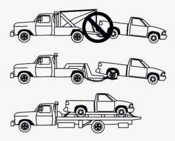
Do not tow with sling-type equipment or the rear bumper system will be damaged.
