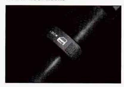
If your vehicle has power door locks, push LOCK on the power door lock switch on the door armrest. This switch will lock all the doors at once.
