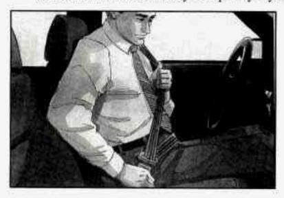
To make the lap part tight, pull down on the buckle end of the belt as you pull up on the shoulder belt.
