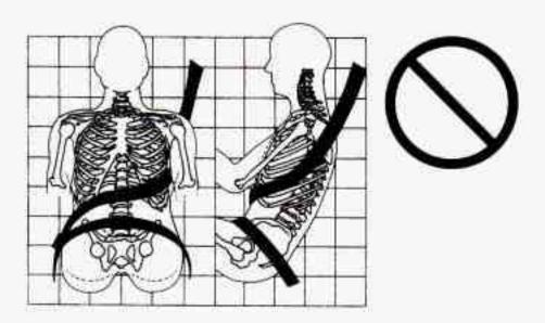
A: The shoulder belt is worn under the arm. It should be worn over the shoulder at all times.
