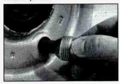
Put the nuts on by hand. Make sure the cone-shaped end is toward the wheel.
