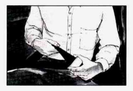
Each jump seat has a lap belt with no retractor. To make the belt longer, tilt the latch plate a little and pull the belt.
