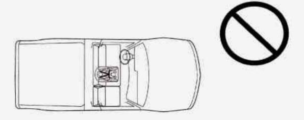
Don't use a child restraint in this position. The restraint won't work properly.
