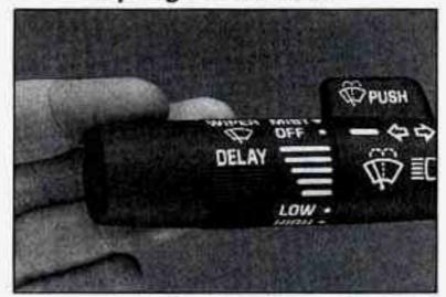
To change the headlamps from low beam to high or high to low, pull the multifunction lever all the way toward you. Then release it.
