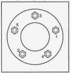
Use the wrench to tighten the wheel nuts firmly in a criss-cross sequence as shown. Remove the wheel blocks.
