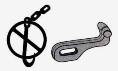
When your vehicle is being towed, have the key off. The steering wheel should be clamped in a straight—ahead position with a clamping device designed for towing service. Do not use the vehicle's steering column lock for this. The transmission (either automatic or manual) should be in NEUTRAL (N) and the transfer case (either manual shift or electronic shift), if you have one, should be in 2HI. The parking brake should be released.
