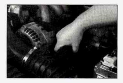
Start the engine and let it run until you can feel the upper radiator hose getting hot. Watch out for the engine fan.
