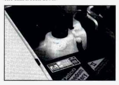
The coolant level should be at the ADD mark, If it isn't, you may have a leak in the radiator hoses, heater hoses, radiator, water pump or somewhere else in the cooling system.
