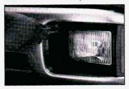
Remove the screws from the headlamp retainer.
