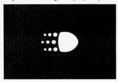
This green DRL indicator light is above the fuel gage on the instrument cluster.
