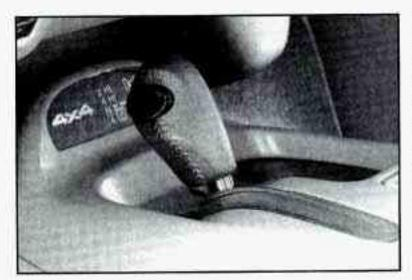
If your four-wheel drive vehicle has the manual transfer case, the transfer case shift lever is on the floor next to the driver. Use this lever to shift into and out of four-wheel drive.
