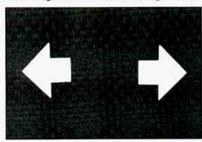
This light with the green arrows is on both sides of the speedometer on the instrument cluster. The turn signal indicator will come on whenever you signal a turn or lane change. See "Turn and Lane Change Signal" in this section.
