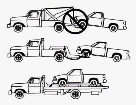
Do not tow with sling-type equipment or the front bumper system will be damaged.
