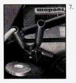
Don't let the other end touch metal. Connect it to the positive (+) terminal of the good battery. Use a remote positive (+) terminal if the vehicle has one.
