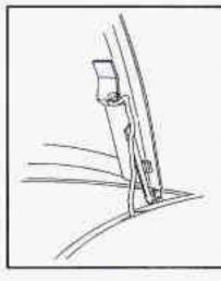
Lift the hood, release the hood prop from its retainer and put the hood prop into the slot in the hood hinge. The underhood lamp will automatically come on and stay on until the hood is closed.
