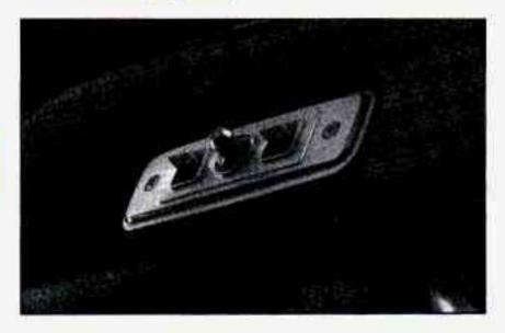
If your vehicle has a power seat on the driver or passenger's side, you can adjust it with this switch at the front center cushion of the seat. You can use these switches to move the seat where you want it. To raise the seat, move the center knob up. To lower the seat, move the center knob down. To move the seat forward, move the center knob toward the right. To move the seat rearward, move the center knob toward the left.
