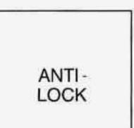
If there's a problem with the anti-lock brake system, this warning light will stay on. See "Anti-Lock Brake System Warning Light" in the Index.
