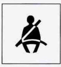
The safety belt light will also come on and stay on for about 20 seconds, then it will flash for about 55 seconds. If the driver's belt is already buckled, neither the tone nor the light will come on.
