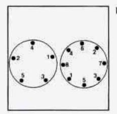
Tighten the nuts firmly in a criss-cross sequence as shown. Rotate the wheel wrench clockwise.
