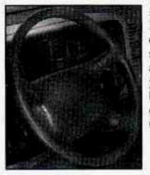
If it says SUPPLEMENTAL INFLATABLE RESTRAINT on the middle part of the steering wheel and there's a right front passenger seat, your vehicle has two air bags -- one air bag for the driver and another air bag for the right front passenger. If it says SUPPLEMENTAL INFLATABLE RESTRAINT on the middle part of the steering wheel but there is no right front passenger seat, your vehicle has an air bag for the driver only.
