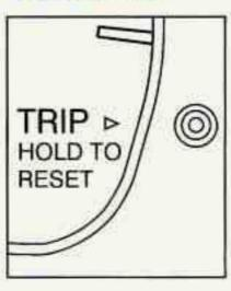
The trip odometer can tell you how far your vehicle has been driven since you last set the trip odometer to zero.
