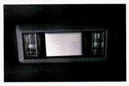
If your vehicle has reading lamps, press the button next to the lamp to turn the lamp on. Press the button again to turn the lamp off.
