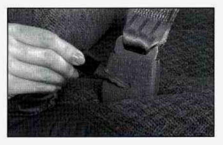
Disconnect the quick release latch plates for the lap shoulder belts on the bench seat to be removed. To do this, press the tip of a key into the release hole of the safety belt buckle while pulling up on the safety belt.
