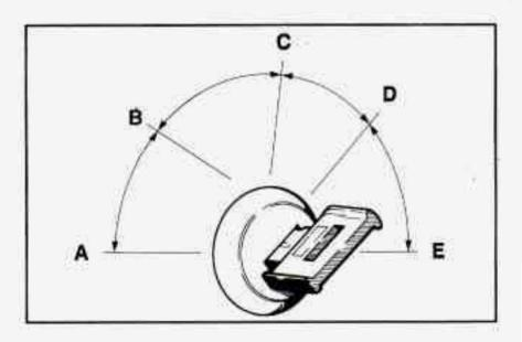
ACCESSORY (A): ACCESSORY lets you use things like the radio, power windows and the windshield wipers when the engine is off. To get into ACCESSORY, push in the key and turn it toward you. Your steering wheel will remain locked, just as it was before you inserted the key. LOCK (B): This position locks your ignition, steering wheel and transmission. It's a theft-deterrent feature. You will only be able to remove your key when the ignition is turned to LOCK.
