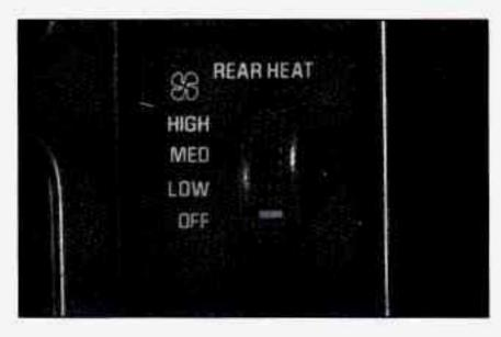
To increase and decrease the flow of heated air to the rear floor vents, move the switch marked REAR HEAT to the blower speed you want.
