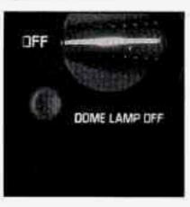
You can use the dome lamp button, located below the headlamp knob, to set the dome lamps to automatically come on when the doors are open, or to remain off.
