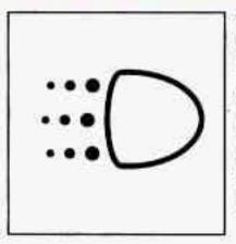
You may have this light on the instrument panel. It will light whenever the DRL are on. It is also a reminder to turn on your headlamps when driving at night. For more details about DRL, see "Headlamps and Vehicle Lighting" in this section.
