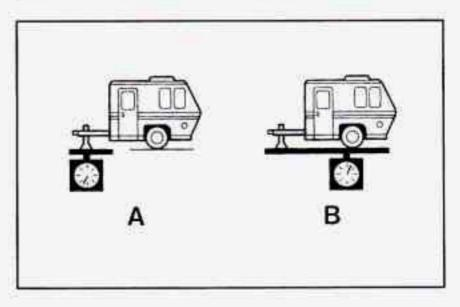
If you're using your platform hitch as a weight-carrying hitch, the trailer tongue (A) should weigh 10 percent of the total loaded trailer weight (B). If you're using your platform hitch as a weight-distributing hitch, the trailer tongue (A) should weigh 12 percent of the total loaded trailer weight (B).
