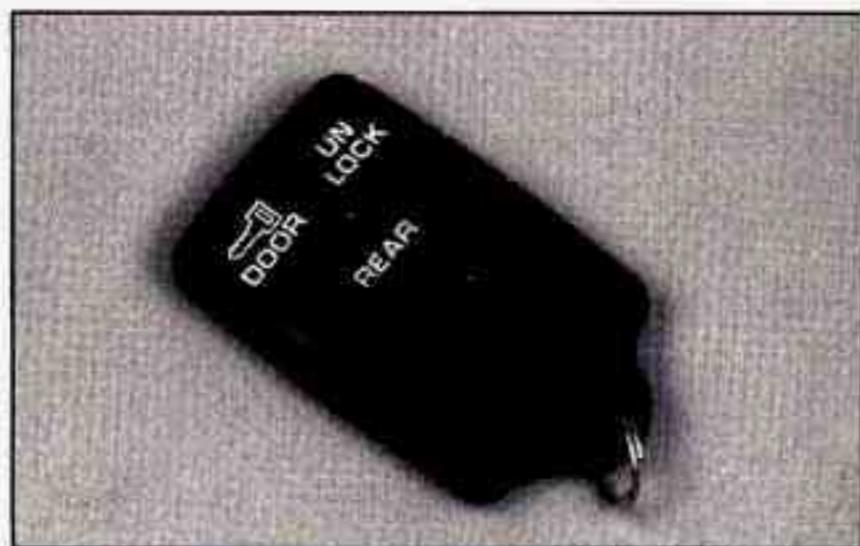
To unlock the driver's door, press the UNLOCK button. If you press this button again within five seconds, all the doors will unlock. Press the REAR button to unlock the rear door only. When the UNLOCK or REAR button is pressed, the interior dome lamps are turned on for 40 seconds or until the ignition switch is activated.
