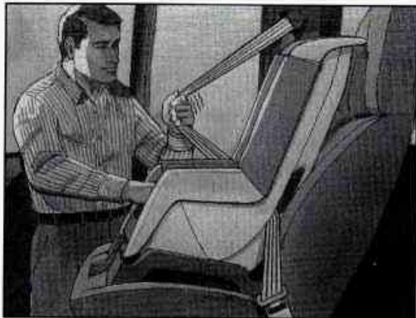
6. Pull the rest of the shoulder belt all the way out of the retractor to set the lock.
