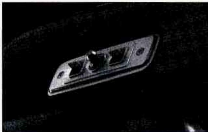
If your vehicle has a power seat on the driver or passenger's side, you can adjust it with this switch at the front center cushion of the seat.
