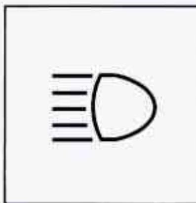
When the high beams are on, this light on the instrument panel also will be on.
