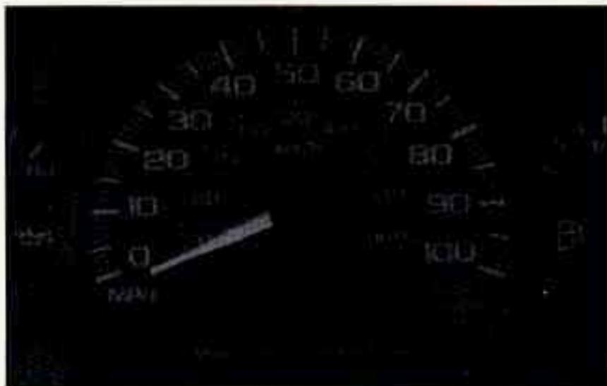
Your speedometer lets you see your speed in both miles per hour (mph) and kilometers per hour (km/h). Your odometer shows how far your vehicle has been driven, in either miles (used in the United States) or kilometers (used in Canada).
