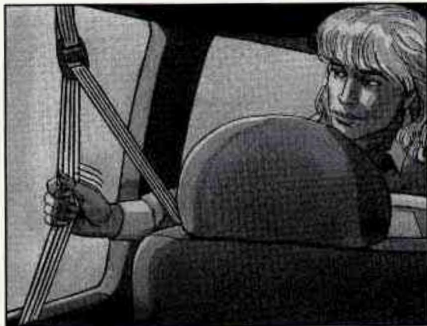
6. To tighten the belt, feed the shoulder belt back into the retractor while you push down on the child restraint.
