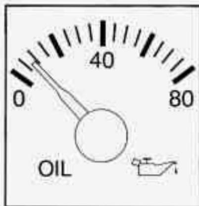
The oil pressure gage shows the engine oil pressure in psi (pounds per square inch) when the engine is running. Canadian vehicles indicate pressure in kPa (kilopascals).
