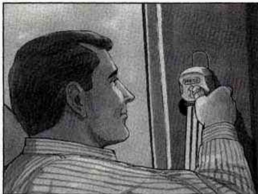
To move it down, push in at the word **PRESS** and move the height adjuster to the desired position. You can move the adjuster up just by pushing up on the shoulder belt guide. After you move the adjuster to where you want it, try to move it down without pushing in to make sure it has locked into position.
