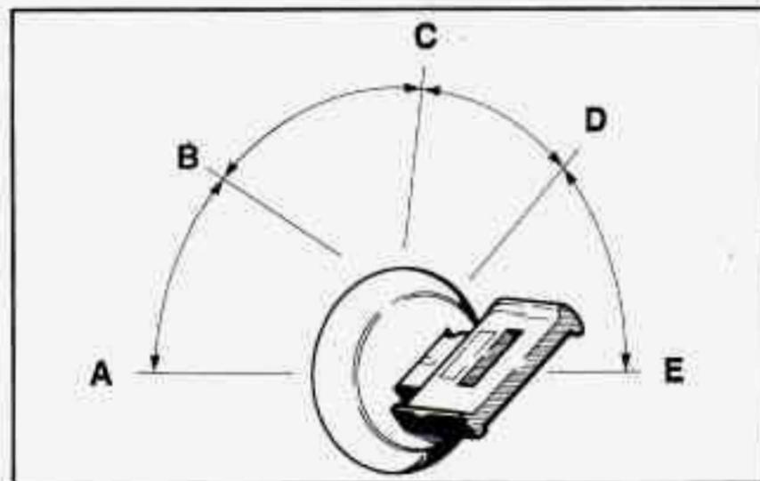
**ACCESSORY (A):** ACCESSORY lets you use things like the radio, power windows and the windshield wipers when the engine is off. To get into ACCESSORY, push in the key and turn it toward you. Your steering wheel will remain locked, just as it was before you inserted the key.
