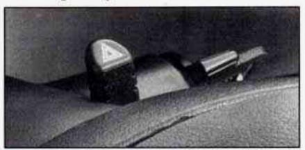
Press the switch to make your front and rear turn signal lamps flash on and off. Your hazard warning flashers work no matter what position your key is in, and even if the key isn't in.
