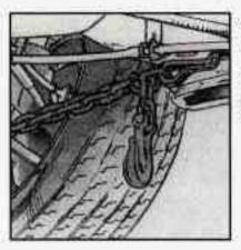
Attach T-hook chains into the slots in the bottom of the floor pan support rails, just ahead of the rear wheels, on both sides.
