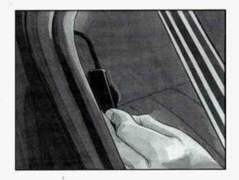
Pull the elastic cord out from between the edge of the scatback and the interior body to remove the guide from its storage clip.
