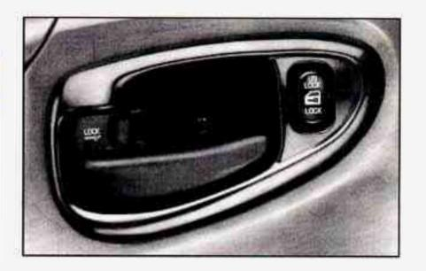
From the inside, push the lever to lock the door. To unlock, pull the lever.
