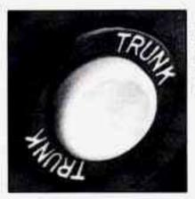
Press the button under the instrument panel on the driver's side. Your transaxle shift lever must be in PARK (P).
