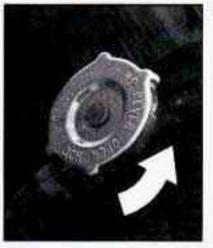
You can remove the radiator pressure cap when the cooling system, including the radiator pressure cap and upper radiator hose, is no longer hot.
