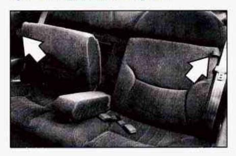
Pull forward on the seat tab to fold the seat down. To return the seat to its original position, push it back up and make sure it latches.
