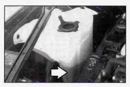
When your engine is cold, the coolant level should be at the COLD mark or a little higher. When your engine is warm, the level should be up to the HOT mark or a little higher.
