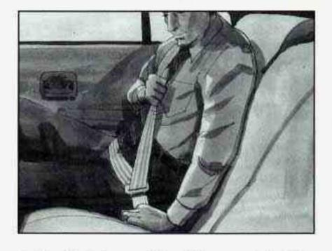
To make the lap part tight, pull down on the buckle end of the belt as you pull up on the shoulder part.
