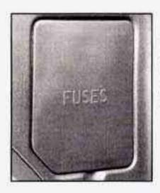
Some fuses are in a fuse block on the passenger's side of the instrument panel. Pull off the cover labeled FUSES to expose the fuses.
