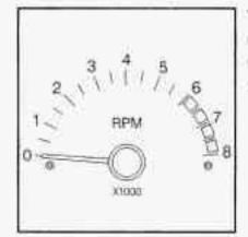
The tachometer displays the engine speed in thousands of revolutions per minute (rpm).
