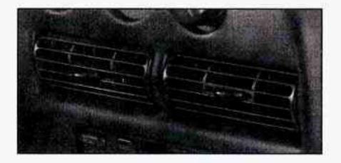
Adjust the direction of airflow by moving the louvered vents.
