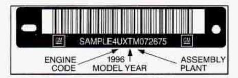
This is the legal identifier for your Chevrolet. It appears on a plate in the front corner of the instrument panel, on the driver's side. You can see it if you look through the windshield from outside your vehicle. The VIN also appears on the Vehicle Certification and Service Parts labels and the certificates of title and registration.
