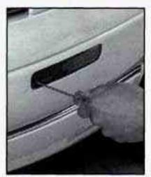
Remove the screw from the sidemarker lens.
