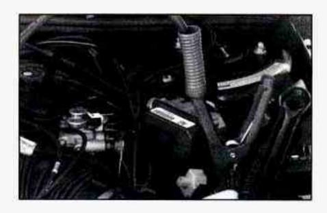
Connect the red positive (+) cable to the positive (+) terminal of the vehicle with the dead battery. Use a remote positive (+) terminal if the vehicle has one.
