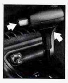
Hold in the button on the lever, and push the lever all the way toward the front of your vehicle.
