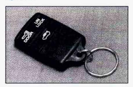
Press UNLOCK once to unlock the driver's door. Press UNLOCK again within five seconds to unlock the passenger's door, too. The interior lamps will come on (see "Sustained Interior Illumination" in the Index for more details).
