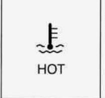
This light tells you that your engine coolant has overheated or your radiator cooling fan is not working.
