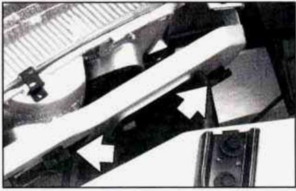
Open the flap by lifting the snap screw.
