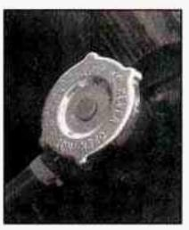
10. Then replace the pressure cap. At any time during this procedure if coolant begins to flow out of the filler neck, reinstall the pressure cap. Be sure the arrows on the pressure cap line up like this.
