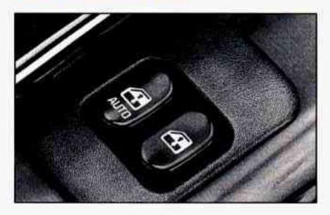
Switches on the driver's door armrest control each of the windows when the ignition is on. In addition, the passenger door has a switch for its own window. The driver's window switch has an auto-down feature. This switch is labeled AUTO. Tap the rear of the switch, and the driver's window will open a small amount. If the rear of the switch is pressed all the way down, the window will go all the way down.
