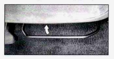
The driver's seat may have a bar and a handle under the front edge of the seat. Lift the bar to unlock the seat and slide it forward and backward.
