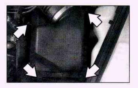
To check or replace the air filter, remove the four screws and pull off the cover.
