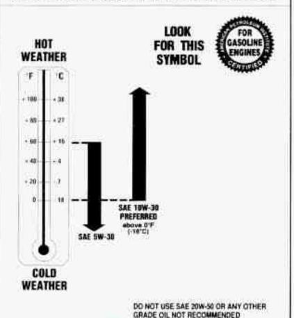
As shown in the chart, if you have the 3.4L engine, SAE 10W-30 is best for your vehicle. However, you can use SAE 5W-30 if it's going to be colder than 60°F (16°C) before your next oil change. When it's very cold, you should use SAE 5W-30. These numbers on an oil container show its viscosity, or thickness. Do not use other viscosity oils, such as SAE 20W-50.
