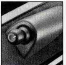
The electric mirror control is on the driver's door. Turn the control to the left to adjust the left mirror or to the right to adjust the right mirror. Then move the control in the direction you want to move the mirror.
