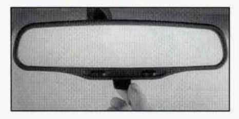
To reduce glare from lamps behind you, push the lever forward (to the night position). To return the mirror to the day position, pull the lever toward you.
