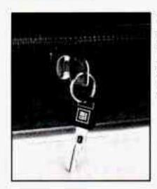
To unlock the trunk from the outside, insert the door key and turn it. You can also use the Remote Lock Control transmitter, if your vehicle has this option.
