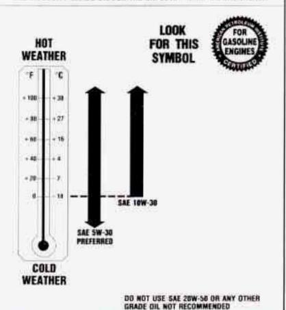
As shown in the chart, unless you have the 3.4L engine, SAE 5W-30 is best for your vehicle. However, you can use SAE 10W-30 if it's going to be 0°F (-18°C) or above. These numbers on an oil container show its viscosity, or thickness. Do not use other viscosity oils, such as SAE 20W-50.
