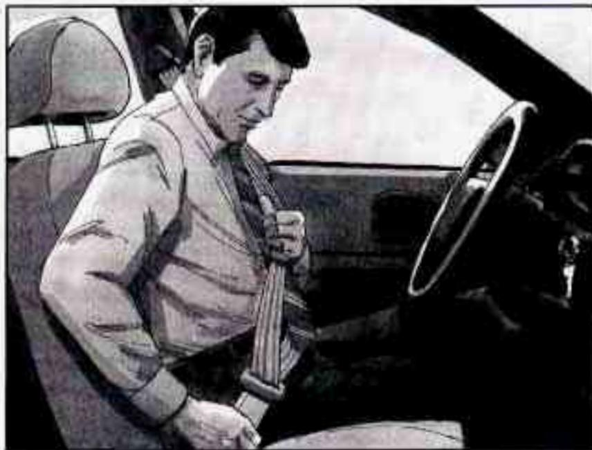
5. To make the lap part tight, pull down on the buckle end of the belt as you pull up on the shoulder belt.
