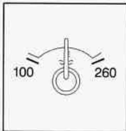
You have a gage that shows the engine coolant temperature. If the gage pointer moves into the red area, your engine is too hot!
