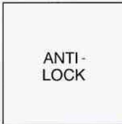
If there's a problem with the anti-lock brake system, this warning light will stay on or flash. See "Anti-Lock Brake System Warning Light" in the Index.
