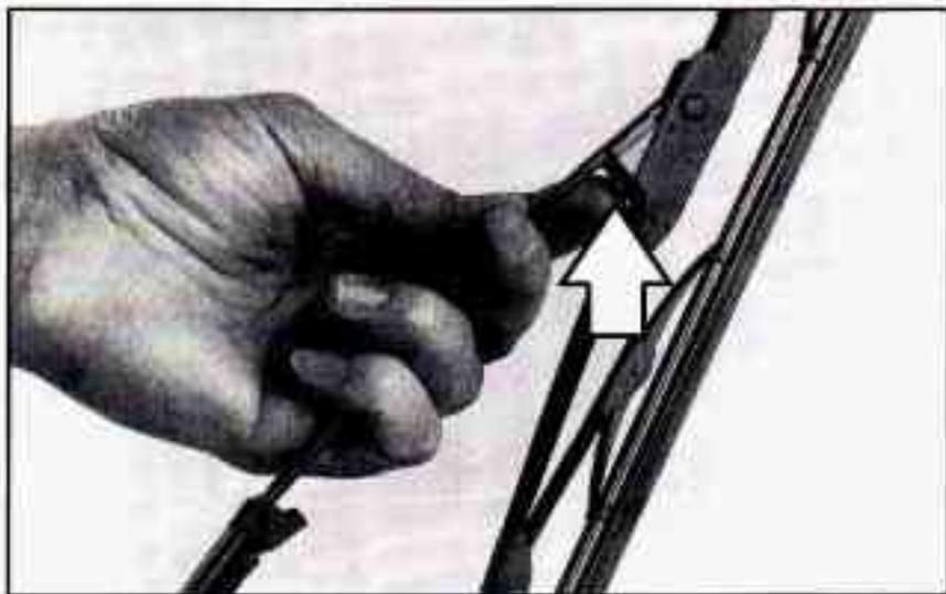
2. Lift the release clip with a screwdriver and pull the blade off the wiper arm.
