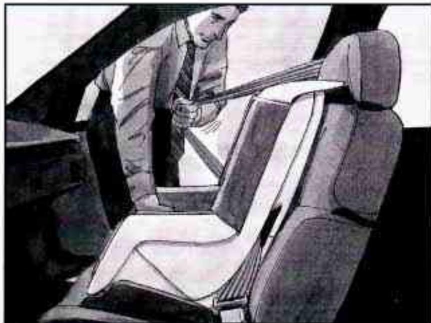
6. Pull the rest of the shoulder belt all the way out of the retractor to set the lock.
