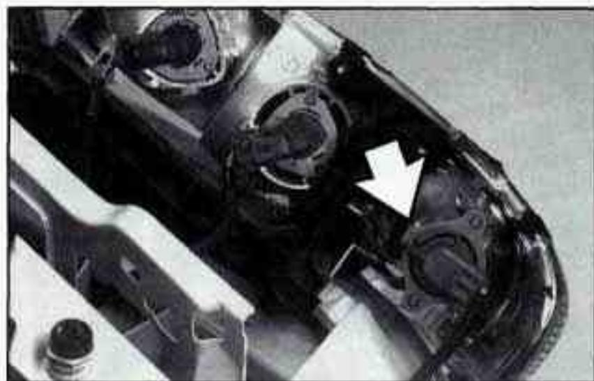
4. Slide the headlamp assembly outboard and gently pull the inside of the assembly away from the vehicle.
