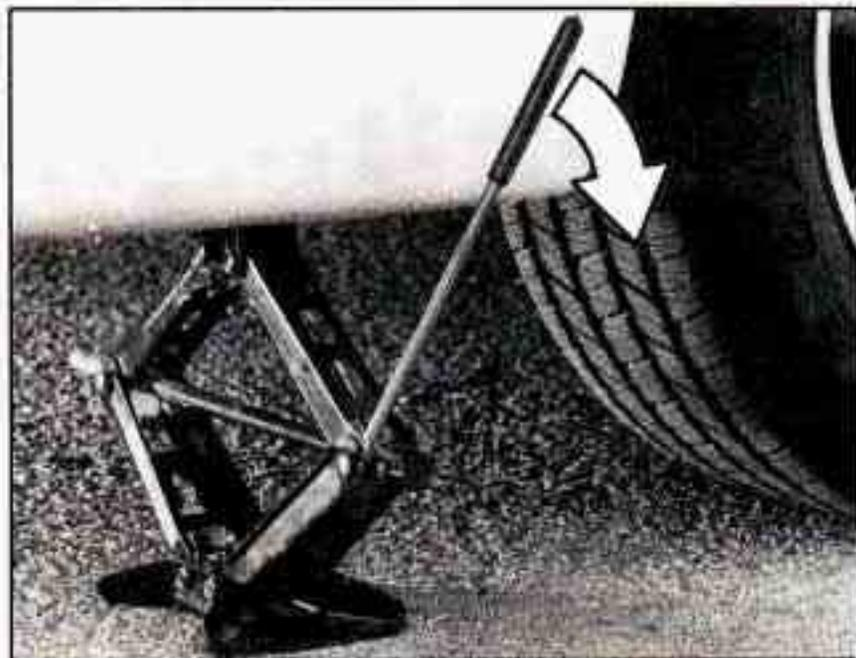
4. Raise the vehicle by turning the jack handle clockwise. Raise the vehicle far enough off the ground for the spare tire to fit under the vehicle.
