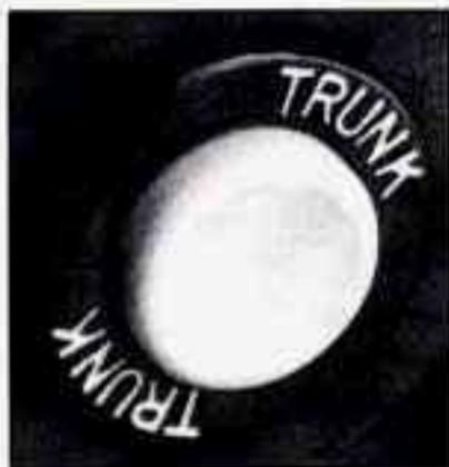
Press the button under the instrument panel on the driver's side. Your transaxle shift lever must be in PARK (P).
