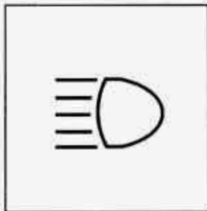
To change your headlamps from low beam to high beam, or high to low, pull the multifunction lever all the way toward you. Then release it. When the high beams are on, a light on the instrument panel also will be on.
