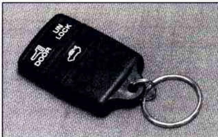
Press UNLOCK once to unlock the driver's door. Press UNLOCK again within five seconds to unlock the passenger's door, too. The interior lamps will come on (see "Sustained Interior Illumination" in the Index for more details).
