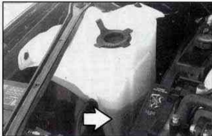
When your engine is cold, the coolant level should be at the COLD mark or a little higher. When your engine is warm, the level should be up to the HOT mark or a little higher.
