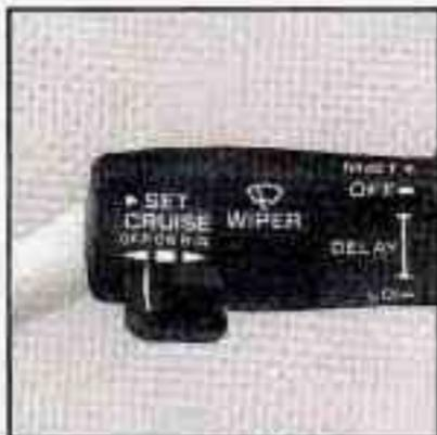
3. Push in the SET button at the end of the lever and release it.
