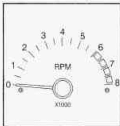
The tachometer displays the engine speed in thousands of revolutions per minute (rpm).
