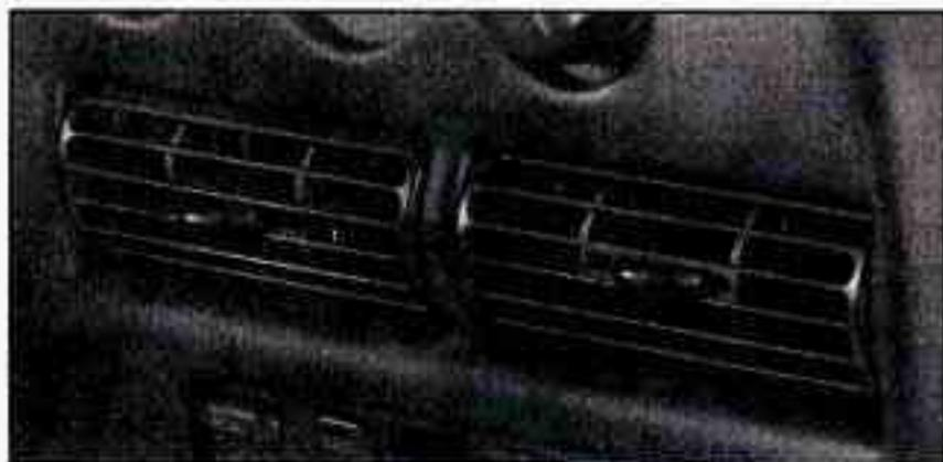
Adjust the direction of airflow by moving the louvered vents.
