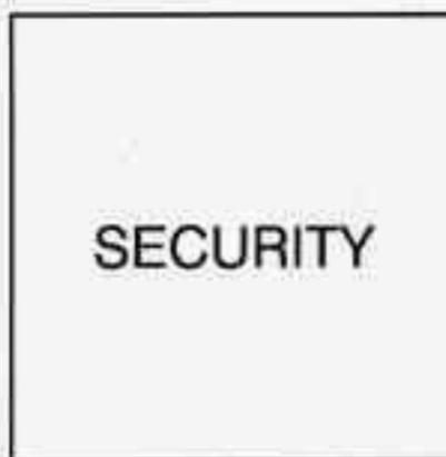
This light will come on when you turn the key to START and stay on until the vehicle starts. It will also come on and stay on if your key is too dirty or wet for the PASS-Key II system to read the resistor pellet.
