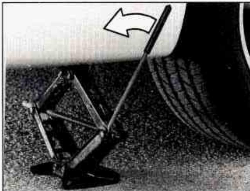
8. Lower the vehicle by turning the jack handle counterclockwise. Lower the jack completely.
