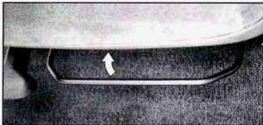
The driver's seat may have a bar and a handle under the front edge of the seat. Lift the bar to unlock the seat and slide it forward and backward.
