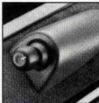
The electric mirror control is on the driver's door. Turn the control to the left to adjust the left mirror or to the right to adjust the right mirror. Then move the control in the direction you want to move the mirror.
