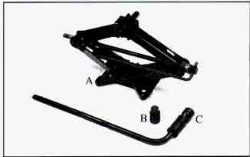
The tools you'll be using include the jack (A), socket (B) and wheel wrench (C).
