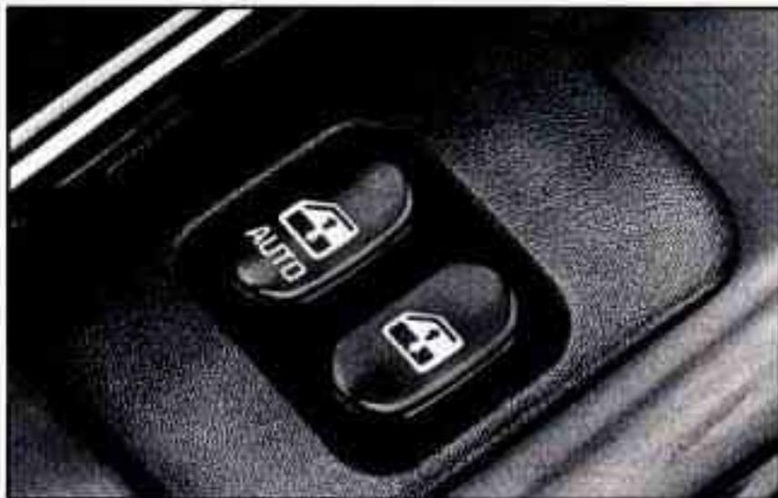
Switches on the driver's door armrest control each of the windows when the ignition is on. In addition, the passenger door has a switch for its own window.
