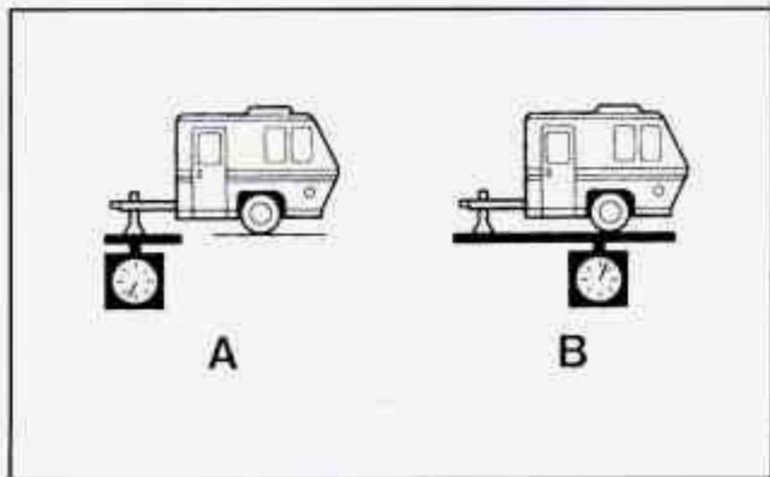
If you're using a weight-carrying hitch, the trailer tongue (A) should weigh 10% of the total loaded trailer weight (B). If you have a weight-distributing hitch, the trailer tongue (A) should weigh 12% of the total loaded trailer weight (B).
