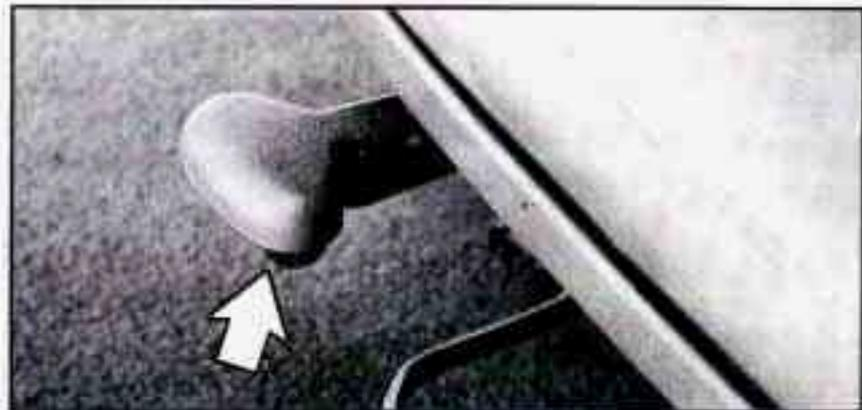
Lift the handle to tilt the seat up or down.
