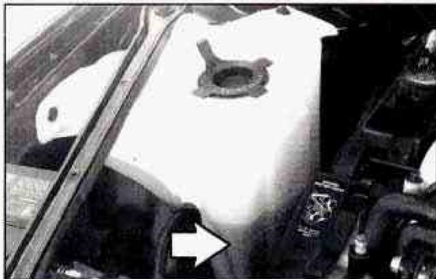
The coolant level should be at or above the COLD mark. If it isn't, you may have a leak in the radiator hoses, heater hoses, radiator, water pump or somewhere else in the cooling system.
