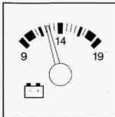
When your engine is not running, but the ignition is in the RUN position, this gage shows your battery's state of charge in DC volts.
