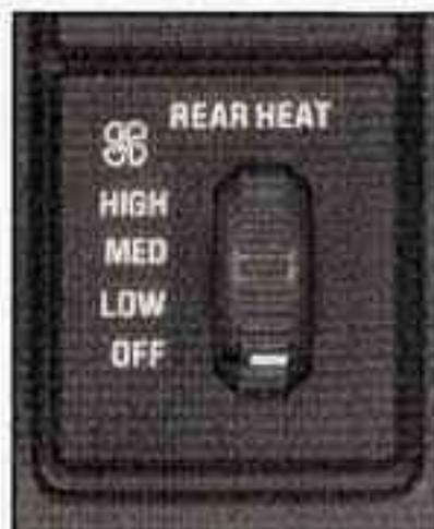
If you have a rear heater (without rear air conditioning), the control switch is located on the instrument panel.
