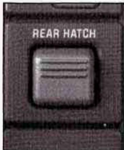
The electric hatch release button lets you release the tailgate glass. To release the glass, press the top of the button.
