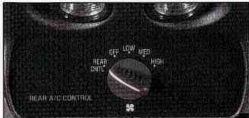
To operate the rear system using the front control, just turn the knob to the blower position you want.
