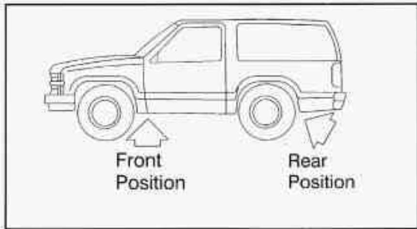
4. With UP on the ratchet facing you, raise the vehicle by rotating the ratchet and wheel wrench clockwise. Raise the vehicle far enough off the ground so there is enough room for the spare tire to fit.
