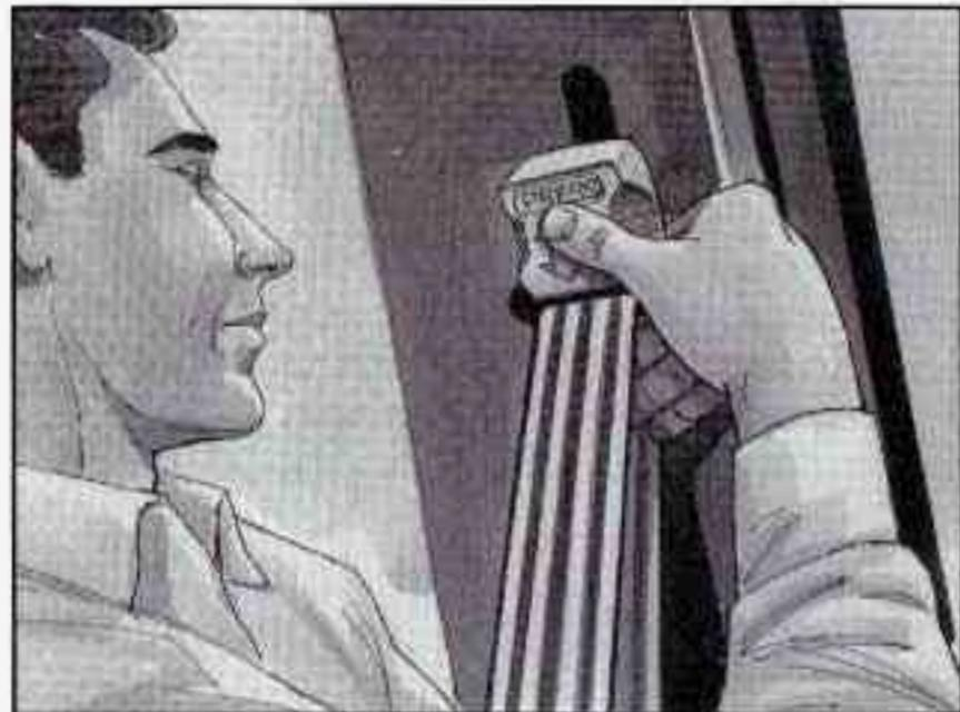
To move the height adjuster down, push in at the word **PRESS** and move the height adjuster to the desired position. You can move the adjuster up just by pushing up on the shoulder belt guide. After you move the adjuster to where you want it, try to move it down without pushing in to make sure it has locked into position.
