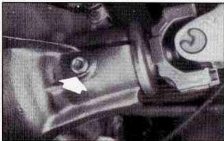
If the level is below the bottom of the filler plug hole, you'll need to add some lubricant. Add enough lubricant to raise the level to the bottom of the filler plug hole.
