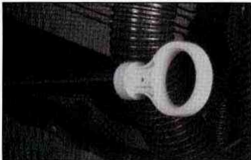
The engine oil dipstick has a yellow ring handle and is located on the passenger side of the engine.
