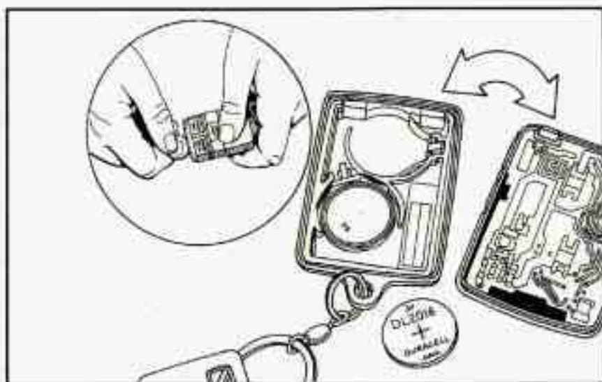
1. Insert a dime in the side seam of the transmitter housing, near the key ring hole.
