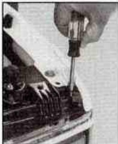
1. Remove the two screws at the top of the radiator support.
