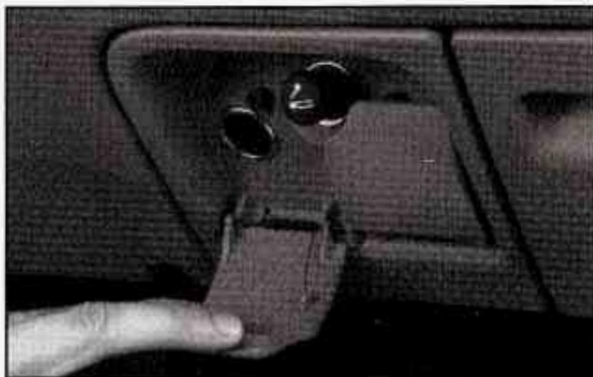
You may have two power outlets near the cigarette lighter. To access these outlets, pull down the covers. Use these outlets to power mobile telephones or other devices designed to operate with vehicle electrical systems.
