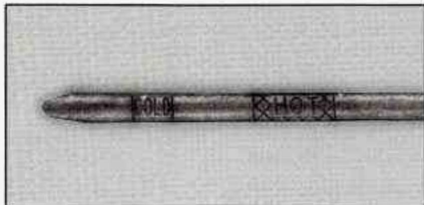
3. Check both sides of the dipstick, and read the lower level. The fluid level must be in the COLD area for a cold check or in the HOT area or cross-hatched area for a hot check.
