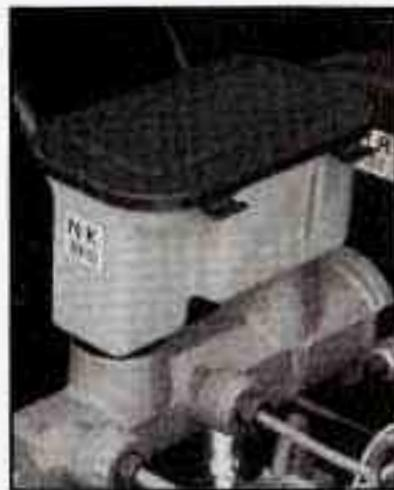
Your brake master cylinder reservoir is here. It is filled with DOT-3 brake fluid.
