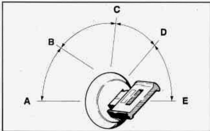
**ACCESSORY (A):** This position lets you use things like the radio and the windshield wipers when the engine is off. Push in the key and turn it toward you. Your steering wheel will remain locked, just as it was before you inserted the key.
