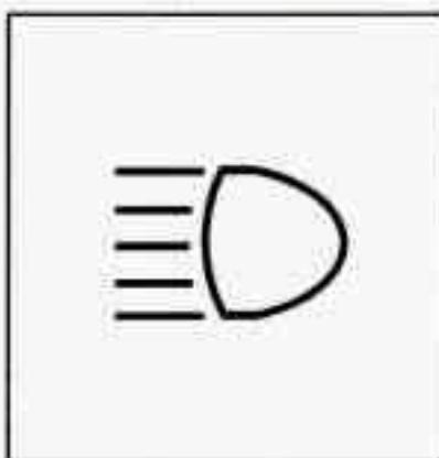
The high-beam indicator is on whenever you use your high-beam headlamps. For more details about high beams, see "Headlamp High/Low Beam Changer" earlier in this section.
