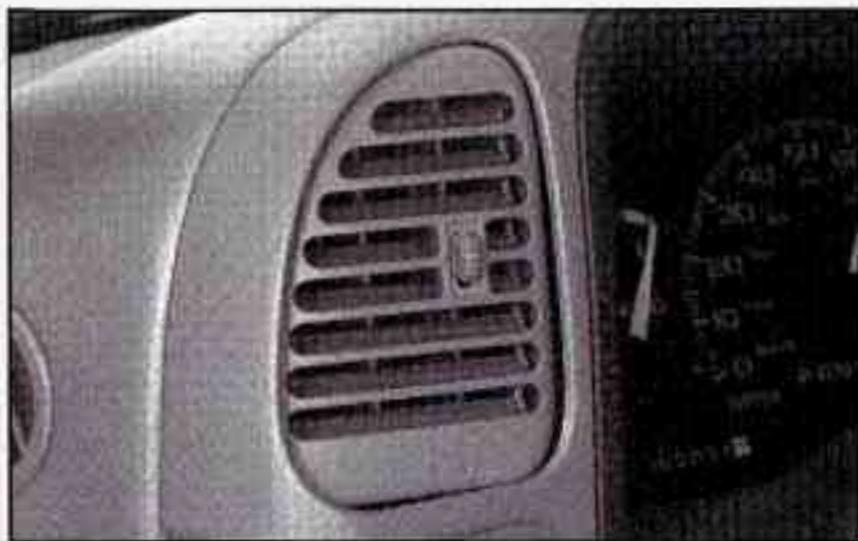
Your vehicle has air outlets in the center and on the sides of your instrument panel. You can move the outlets from side to side or up and down to direct the flow of air, or close the outlets altogether. When you close an outlet, it will increase the flow of air coming out of any outlets that are open. These outlets do not completely shut off airflow when in a closed vent position.
