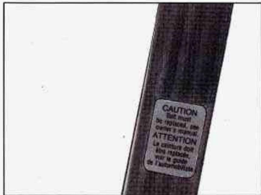
If you ever see a label on a right front safety belt in a two-door Utility model that says to replace the belt, be sure to do so. Then the new belt will be there to help protect you in a collision. You would see this label on the belt near the door opening.
