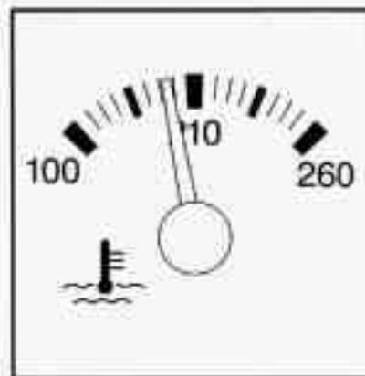
This gage shows the engine coolant temperature.
