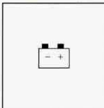
The charging system warning light should come on briefly when you turn on the ignition, before starting the engine, as a check to show you it is working.
