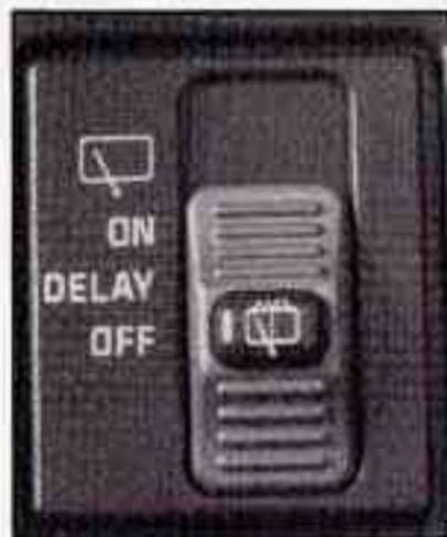
The rear window wiper/washer switch is on your instrument panel, to the right of the gage cluster.
