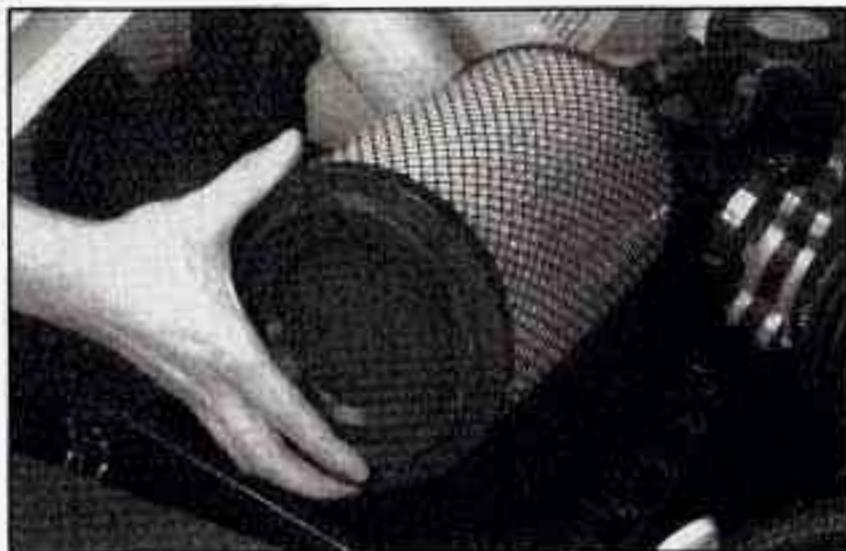
To remove the air filter, unhook the retainer clips and remove the cover. Lift the filter and the connected duct out of the air cleaner housing. Hold the duct and remove the filter by both pulling and twisting the filter away from the duct. Care should be taken to dislodge as little dirt as possible.
