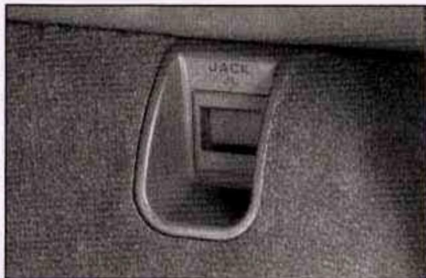
To open the jack cover on four-door utility models, push the cover latches down and remove the cover.
