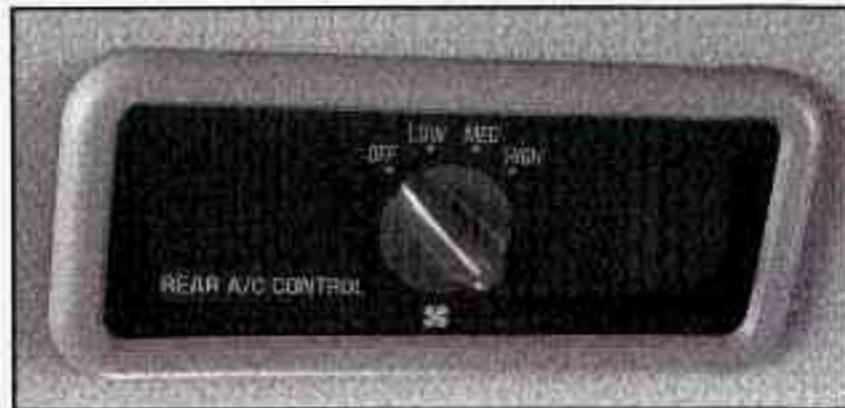
To use the rear control, first turn the front control knob to REAR CNTL. Then, the rear control can be used to increase and decrease the airflow.
