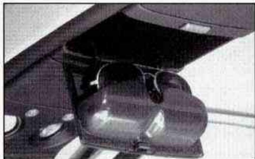
To open the center compartment, press the release button located at the rear of the compartment door.
