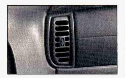
Your vehicle has air vents near the center and on the sides of the instrument panel that allow you to adjust the direction and the amount of airflow inside the vehicle. Push the vent up or down to direct airflow to your preference. Increase or reduce the amount of airflow by opening and closing the louvers. The vents rotate to direct the airflow from side to side.
