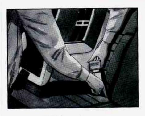
Buckle the belt. Make sure the release button is positioned so you would be able to unbuckle the safety belt quickly if you ever had to.
