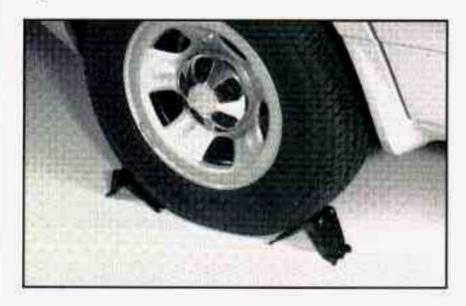
Before you start, block the front and rear of the tire farthest away from the one being changed. Then put your spare tire near the flat tire.
