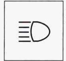
When the high beams are on, this indicator light on the instrument panel also will be on.
