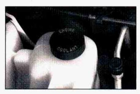
When your engine is cold, the coolant level should be at ADD, or a little higher. When your engine is warm, the level should be up to FULL HOT, or a little higher.
