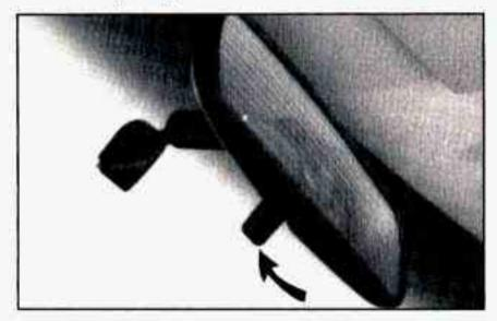
You can adjust the mirror for day or night driving. Press the tab forward (away from you) for day driving. Pull the tab back (toward you) for night driving.
