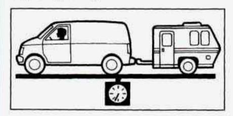
If your vehicle comes with the Trailering Package, there is also a load rating which includes the weight of the vehicle and the trailer it tows. This rating is called the Gross Combination Weight Rating (GCWR).
