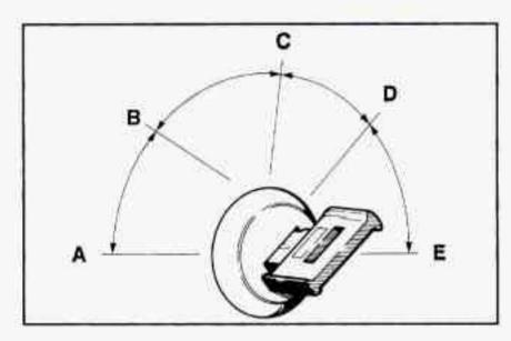
ACCESSORY (A): This position lets you use things like the radio and the windshield wipers when the engine is off. To get into ACCESSORY, push in the key and turn it toward you. Your steering wheel will remain locked, just as it was before you inserted the key.
