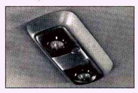
The dome lamps will come on when you open any of the doors. They will remain on for 20 seconds after the last door closes. When the ignition switch is turned on, the dome lamps will go off. You can also turn on the dome lamps by turning the dimmer dial up until the second click.
