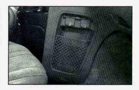
There is also a map/storage pocket on the passenger's side of the engine cover console.
