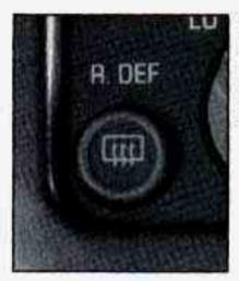
To turn on the rear window defogger, find the button to the left of the heater controls with the defog symbol on it. The rear window defogger will only work when the ignition switch is in the RUN position.
