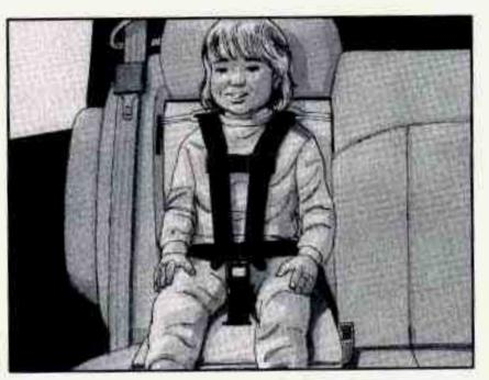
11. Adjust the position of the harness on the child's shoulders by moving the clip up or down along the harness. On each side of the harness, the shoulder part should be centered near the child's shoulder. The harness should be away from the child's face and neck, but not falling from the child's shoulders.
