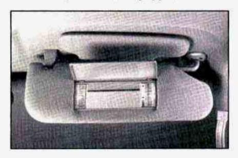
Some visors have mirrors built in, with or without lamps. Just lift the mirror cover on each visor to turn the lamps on, if you have them.
