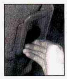
To fold your non-touring seatback forward, pull up on the latch release lever while pulling the seatback toward the rear of the vehicle.
