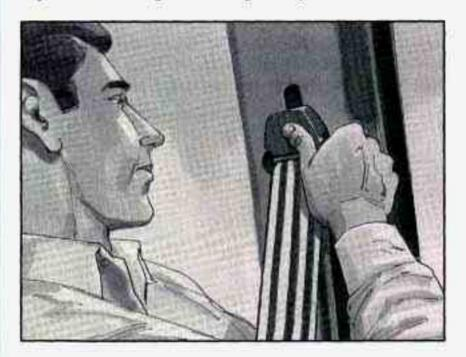
To move it down, push in at the top of the arrows and move the height adjuster to the desired position. You can move the adjuster up just by pushing up on the shoulder belt guide. After you move the adjuster to where you want it, try to move it down without pushing in to make sure it has locked into position.
