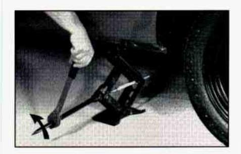
Lower the vehicle by turning the ratchet counterclockwise. Lower the jack completely.
