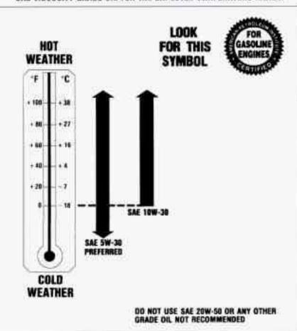
As shown in the chart, SAE 5W-30 is best for your vehicle. However, you can use SAE 10W-30 if it's going to be 0°F (-18°C) or above. These numbers on an oil container show its viscosity, or thickness. Do not use other viscosity oils, such as SAE 20W-50.
