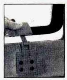
To open your swing-out windows, pull up on the latch and push the window out.
