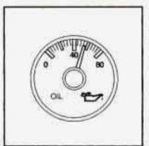
The oil pressure gage shows the engine oil pressure in psi (pounds per square inch) when the engine is running.
