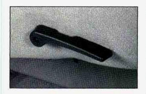
To adjust your seatback, pull up on the lever on the lower outside of the seat.
