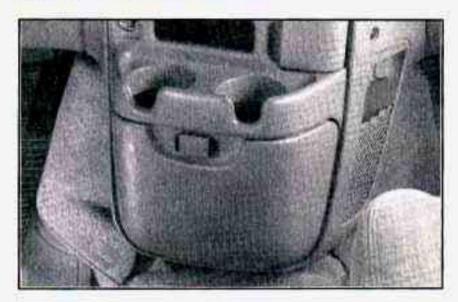
Your front storage compartment/glove box is at the center of the engine cover. To open the compartment, press the two tabs together and pull.
