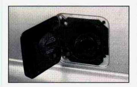
While refueling, place the cap in the holder on the fuel filler door.
