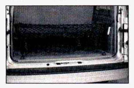
You may have a convenience net in the rear of your vehicle to help keep small loads, like grocery bags, in place during sharp turns or quick stops and starts.
