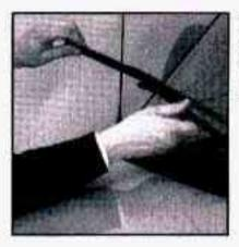
To replace your windshield wiper blade inserts, lift the wiper arm away from the windshield.
