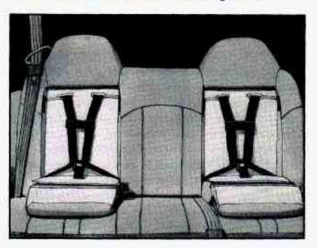
If your vehicle has this option, there's a built-in child restraint at each outboard position of the second row bench seat. This child restraint system conforms to all applicable Federal Motor Vehicle Safety Standards.
