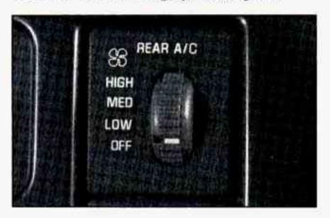
You may have rear air conditioning. The rear air conditioning switch is located to the right of the heater controls. Turn the switch toward HIGH for higher airflow in the rear area. Turn the switch to the OFF position to turn the system off.
