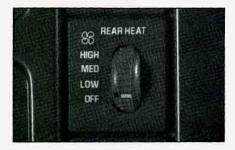
You may have the optional rear heater. The three-speed fan switch is to the right of the radio. Turn the switch toward HIGH for higher airflow in the rear area. Turn the switch to the OFF position to turn the system off.
