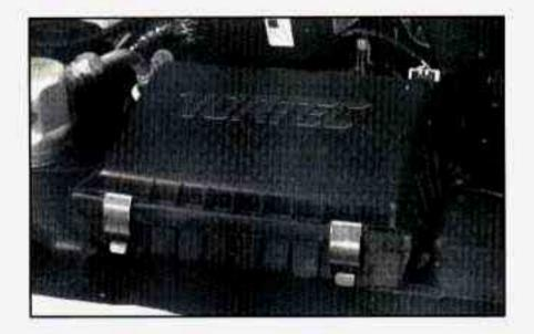
To remove the air filter, lift the hood, unsnap both clips and remove the top. After changing the filter, snap both clips to secure the air cleaner. Be sure the air cleaner lid is correctly positioned to seal out dust and contaminants that are harmful to your engine.
