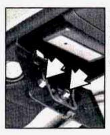
The pegs inside the compartment door are used to make sure the button on the compartment door will contact the control button on the garage door opener.
