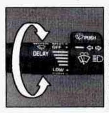
You control the windshield wipers by turning the band with the wiper symbol on it.
