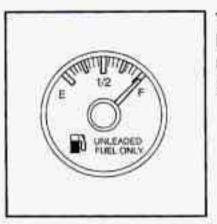
The fuel gage tells you how much fuel you have remaining when the ignition is on.
