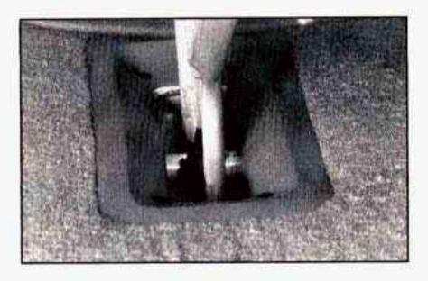
Lower the seat into position. Make sure the front retainers are hooked onto the anchor pins.
