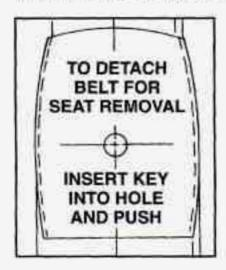
If you are removing the center seat, remove the right lap-shoulder belt.
