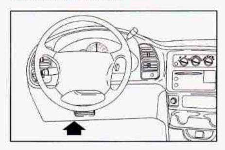
The fuse block is on the lower portion of the instrument panel on the driver's side.
