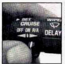
Once you're going about 25 mph (40 km/h) or more, you can move the cruise control switch from ON to R/A for about 1.1/2 seconds.
