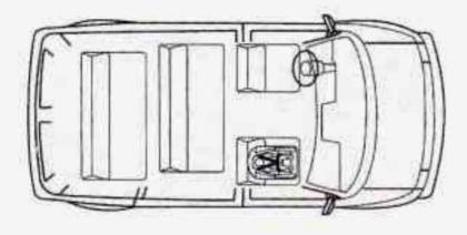
Your vehicle has a front passenger air bag. Never put a rear-facing child restraint in this seat. Here's why:
