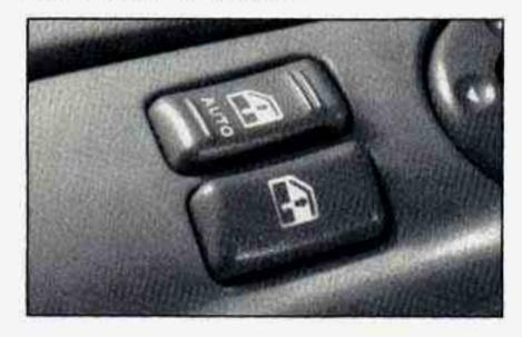
If you have the optional power windows, the controls are on each of the front side doors. The driver's door has a switch for the front passenger window as well. Your power windows will not move unless the ignition has been turned to RUN or ACCESSORY.
