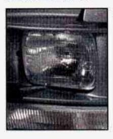
Remove the four retainer screws and the retainer.
