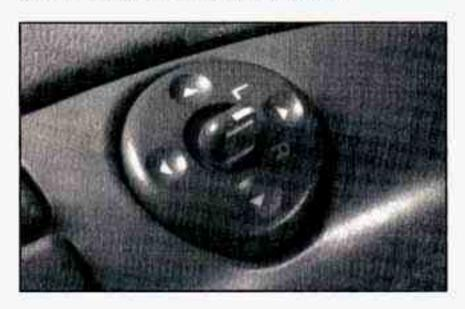
To move a mirror, turn the knob in the middle of the control to L for the driver's side mirror or to R for the passenger's side mirror. Then press the four-way pad to move the mirror in the desired direction.
