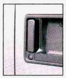
To open the rear doors from the outside, open the passenger's side rear door first. Grasp the handle and pull the door open.
