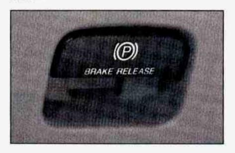
To release the parking brake, hold the regular brake pedal down. Pull the brake release lever located on the lower left side of the steering column.
