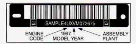
This is the legal identifier for your vehicle. It appears on a plate in the front corner of the instrument panel, on the driver's side. You can see it if you look through the windshield from outside your vehicle. The VIN also appears on the Vehicle Certification and Service Parts labels and the certificates of title and registration.
