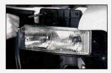
Remove the remaining three screws; the first one from the corner reflector pocket and the two remaining from the composite assembly.
