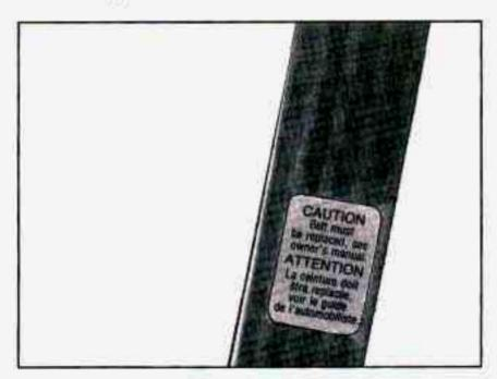
If you ever see a label on a right front safety belt that says to replace the belt, be sure to do so. Then the new belt will be there to help protect you in a collision. You would see this label on the belt near the latch plate.
