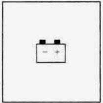
The charging system light will come on briefly when you turn the ignition on, but the engine is not running, as a check to show you the light is working.
