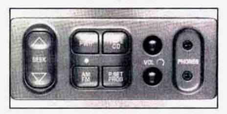
This feature allows rear seat passengers to listen to a different music source than the front seat passengers including AM-FM automatic tone control and cassette tapes. For example, rear seat passengers may listen to a cassette tape through headphones while the driver listens to the radio through the front speakers. The rear seat passengers have control of the volume for each headphone. Be aware that the front seat audio controls always override the rear seat audio controls.
