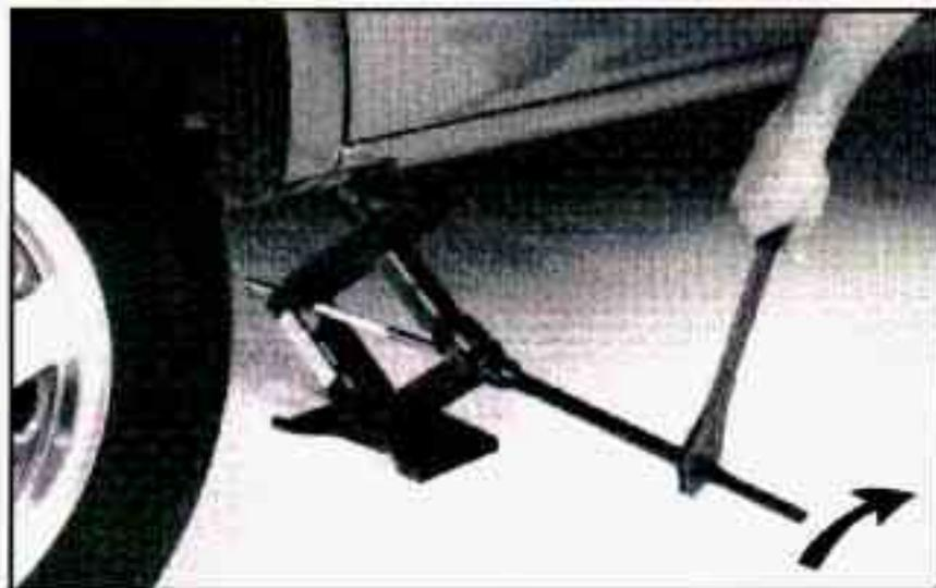
7. Raise the vehicle by rotating the ratchet clockwise. Make sure the UP mark faces you. Raise the vehicle far enough off the ground so there is enough room for the spare tire to fit.
