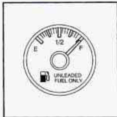
The fuel gage tells you how much fuel you have remaining when the ignition is on.
