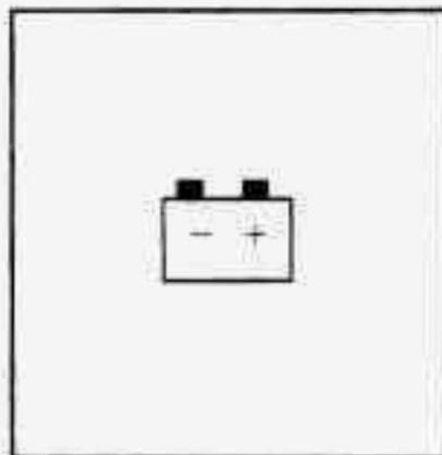
The charging system light will come on briefly when you turn the ignition on, but the engine is not running, as a check to show you the light is working.
