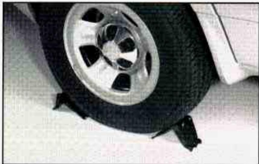
1. Before you start, block the front and rear of the tire farthest away from the one being changed. Then put your spare tire near the flat tire.
