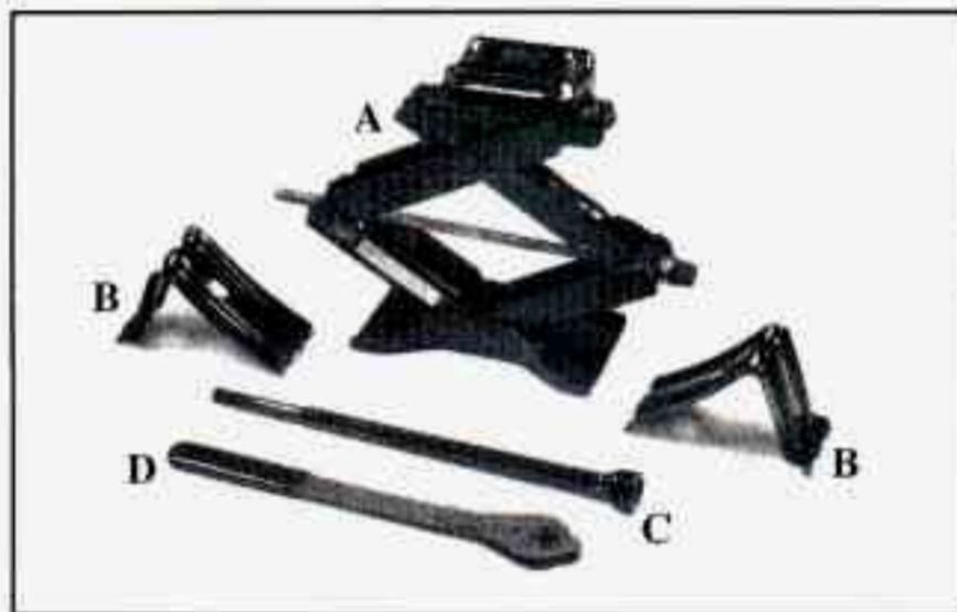
The tools you'll be using include the jack (A), wheel blocks (B), extension (C) and ratchet (D).
