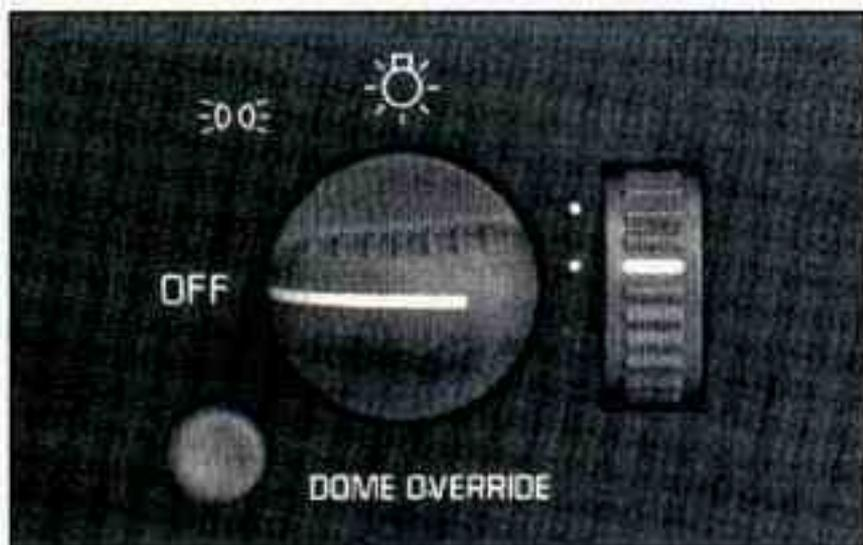
Your lamp switch is on the driver's side of the instrument panel.
