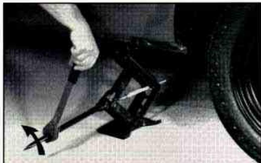
11. Lower the vehicle by turning the ratchet counterclockwise. Lower the jack completely.
