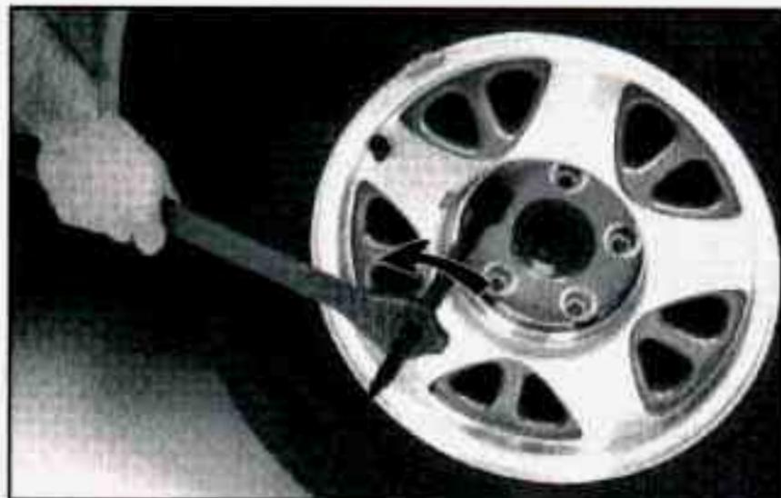
2. With the DOWN side facing you, use the ratchet and socket to loosen all the wheel nuts. Don't remove them yet.
