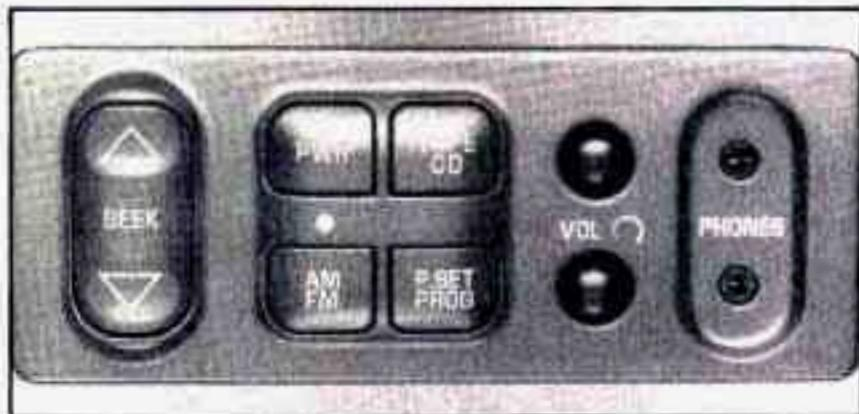
This feature allows rear seat passengers to listen to a different music source than the front seat passengers including AM-FM automatic tone control and cassette tapes. For example, rear seat passengers may listen to a cassette tape through headphones while the driver listens to the radio through the front speakers. The rear seat passengers have control of the volume for each headphone. Be aware that the front seat audio controls always override the rear seat audio controls.
