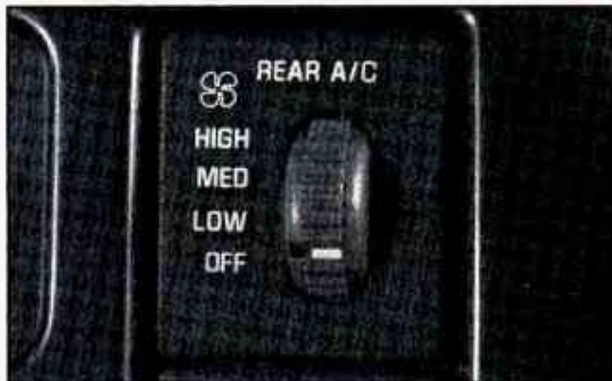
You may have rear air conditioning. The rear air conditioning switch is located to the right of the heater controls. Turn the switch toward HIGH for higher airflow in the rear area. Turn the switch to the OFF position to turn the system off.
