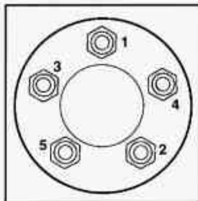
12. Tighten the wheel nuts firmly in a criss-cross sequence as shown. Turn the ratchet clockwise with the UP mark facing you.
