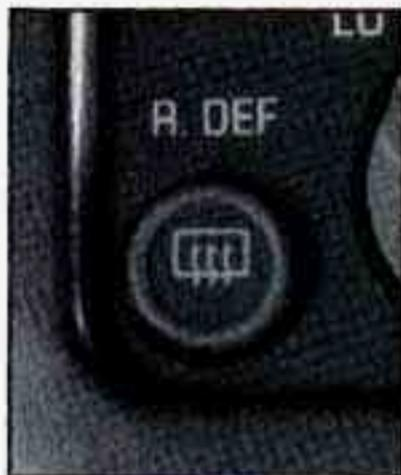
To turn on the rear window defogger, find the button to the left of the heater controls with the defog symbol on it.
