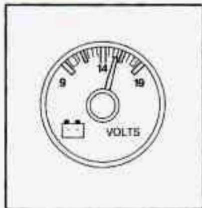
When your engine is not running, but the ignition is on (in the RUN position), the gage shows your battery's state of charge in DC volts.
