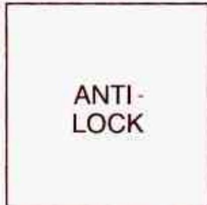
If there's a problem with the anti-lock brake system, this warning light will stay on. See "Anti-Lock Brake System Warning Light" in the Index.
