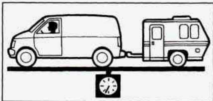
If your vehicle comes with the Trailering Package, there is also a load rating which includes the weight of the vehicle and the trailer it tows. This rating is called the Gross Combination Weight Rating (GCWR).
