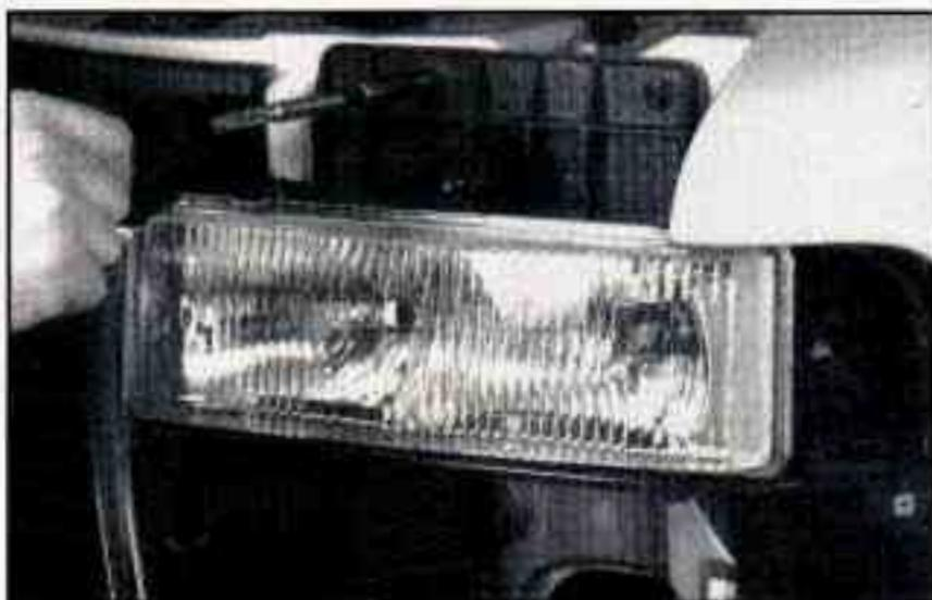
5. Remove the remaining three screws; the first one from the corner reflector pocket and the two remaining from the composite assembly.
