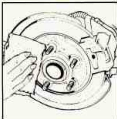
9. Remove any rust or dirt from the wheel bolts, mounting surfaces and spare wheel.
