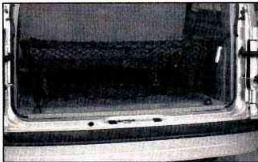
You may have a convenience net in the rear of your vehicle to help keep small loads, like grocery bags, in place during sharp turns or quick stops and starts.
