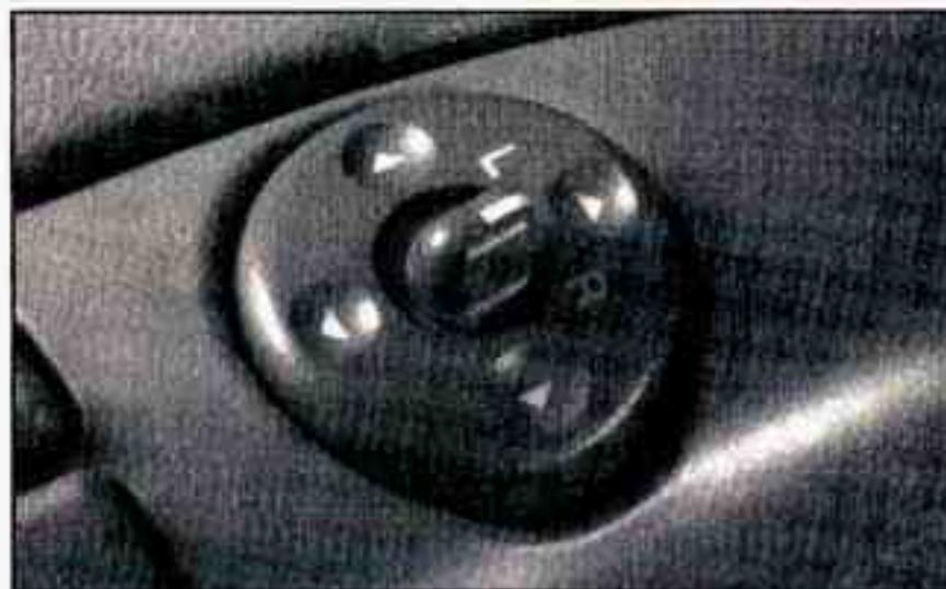
To move a mirror, turn the knob in the middle of the control to L for the driver's side mirror or to R for the passenger's side mirror. Then press the four-way pad to move the mirror in the desired direction.
