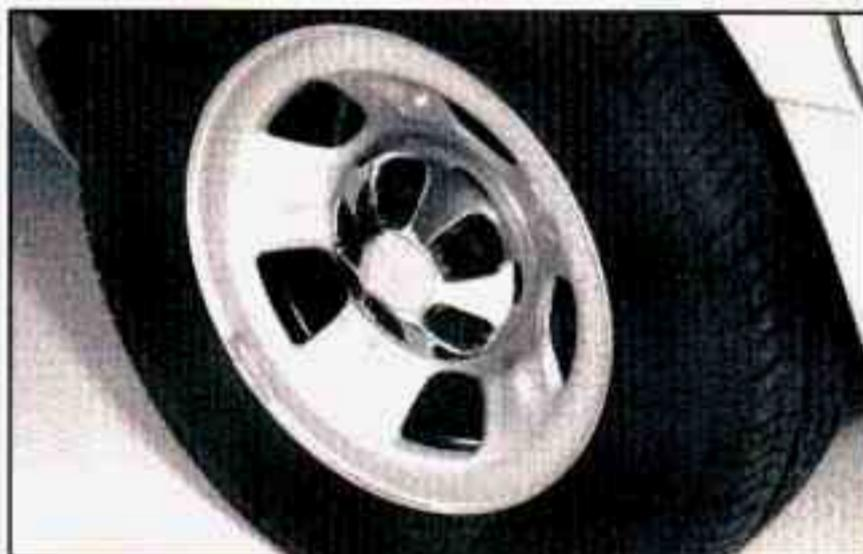
If you have a standard steel wheel, carefully pry along the edge of the hub cap until it comes off. Be careful, the rim edges may be sharp. Don't try to remove the hub cap with your bare hands.
