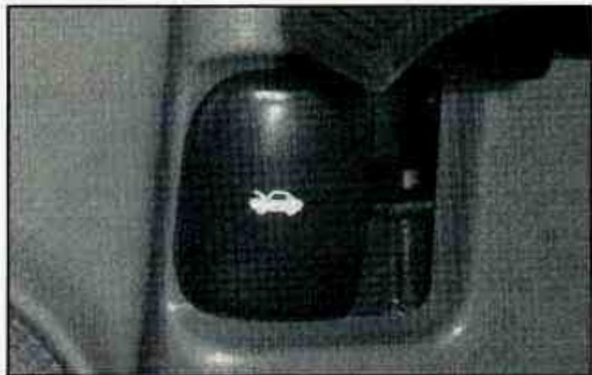
To open the hood, first pull the handle inside the vehicle on the lower driver's side of the kick panel.
