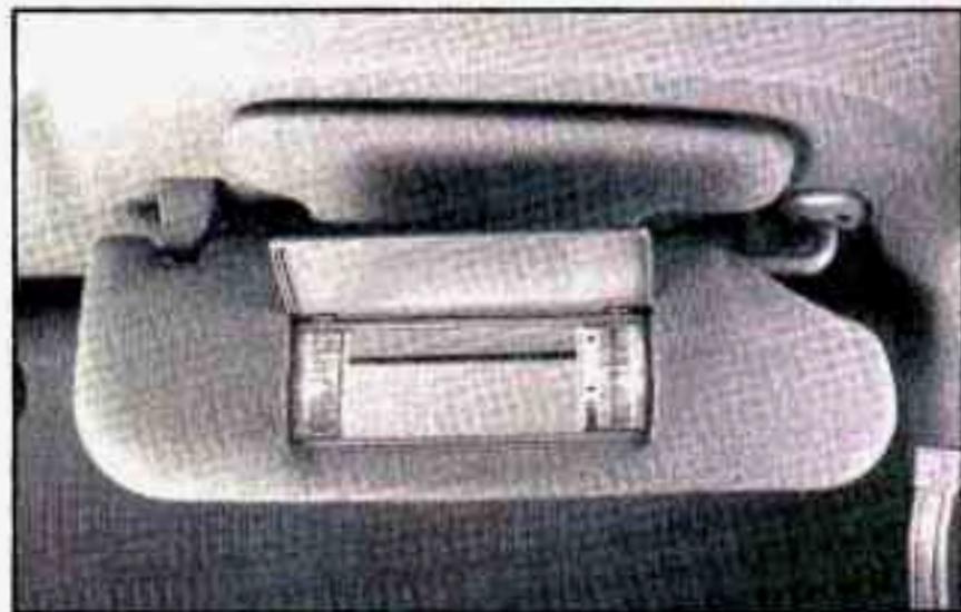
Some visors have mirrors built in, with or without lamps. Just lift the mirror cover on each visor to turn the lamps on, if you have them.
