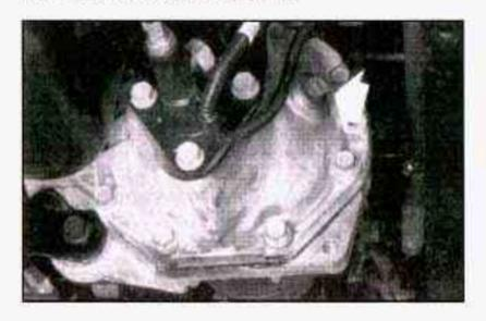
To get an accurate reading, the vehicle should be on a level surface. If the level is below the bottom of the filler plug hole, you may need to add some lubricant.
