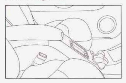
If your vehicle has this console compartment, squeeze the front lever while lifting the top to open it. You can store cassettes and compact discs in the slots in front of the compartment. Some models will have a console with pop-out cupholders located on the front of the storage compartment. If your vehicle has this console push in and release on the cupholder door. The cupholders will pop out for use.
