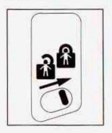
The security lock lever is located on the inside edge of each rear door.
