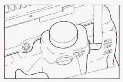
The coolant recovery tank is located in the engine compartment near the passenger side of the vehicle. See Engine Compartment Overview on page 5-12 for more information on location.
