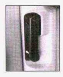
Pull the handle located inside the vehicle on the lower left side of the instrument panel.
