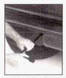
To remove the underbody-mounted spare, insert the chisel end of the wheel wrench, on an angle, into the hoist shaft hole in the rear bumper.
