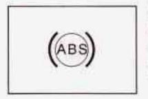
If there's a problem with the anti-lock brake system, this warning light will stay on. See Anti-Lock Brake System Warning Light on page 3-31.
