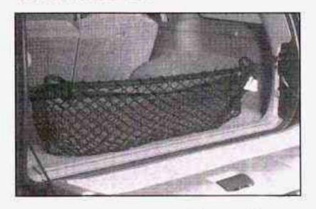
You may have a convenience net in the rear of your vehicle to help keep small items, like gloves and light clothing, in place during sharp turns or quick stops and starts. The net is not designed to retain these items during off-road use. The net is not for larger, heavier items.
