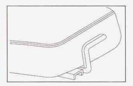
Move the lever located under the front of the manual seat up to unlock it. Slide the seat to where you want it and release the lever. Try to move the seat with your body to make sure the seat is locked into place.
