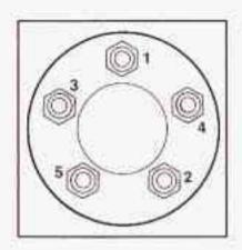
Use the wrench to tighten the wheel nuts firmly in a crisscross sequence as shown. Notice: Improperly tightened wheel nuts can lead to brake pulsation and rotor damage. To avoid expensive brake repairs, evenly tighten the wheel nuts in the proper sequence and to the proper torque specification.
