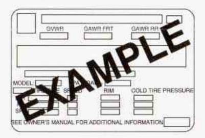
The Certification/Tire tabel is found on the driver's door edge, above the door latch. The label shows the size of your original tires and the inflation pressures needed to obtain the gross weight capacity of your vehicle. This is called the Gross Vehicle Weight Rating (GVWR). The GVWR includes the weight of the vehicle, all occupants, fuel, cargo and trailer tongue weight, if pulling a trailer.
