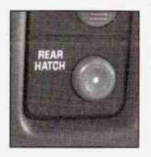
The REAR HATCH button, located to the right of the steering wheel on the instrument panel, allows you to release the rear glass from inside the vehicle.
