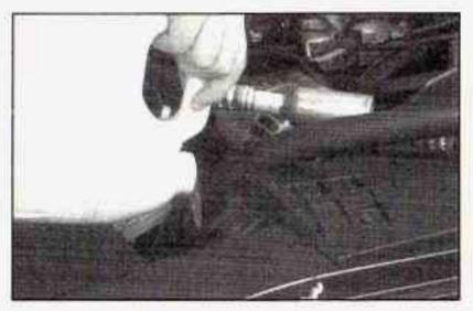
Fill the radiator with the proper DEX-COOL coolant mixture, up to the base of the filler neck. See Engine Coolant on page 5-23 for more information about the proper coolant mixture.
