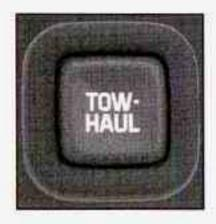
Your vehicle may be equipped with tow/haul mode. The button will be located on the floor console.
