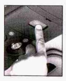
Now, with the compartment door closed, press the button again to make sure the garage door operates properly.
