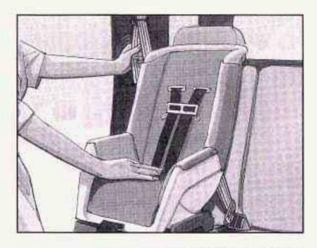
To tighten the belt, feed the shoulder belt back into the retractor while you push down on the child restraint. If you're using a forward-facing child restraint, you may find it helpful to use your knee to push down on the child restraint as you tighten the belt. Push and pull the child restraint in different directions to be sure it is secure.
