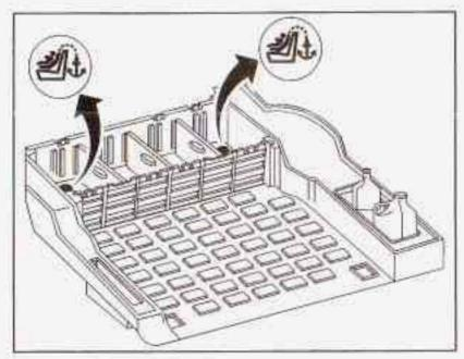
If your vehicle is equipped with the rear convenience system, there will be plugs covering the anchor brackets. To remove the plugs, grasp the edges of the plugs and pull them out. See "Rear Convenience System" in the Index for more information. Don't use the rear set of tie-down brackets near the littgate/endgate or the center tie-down bracket near the rear seats.
