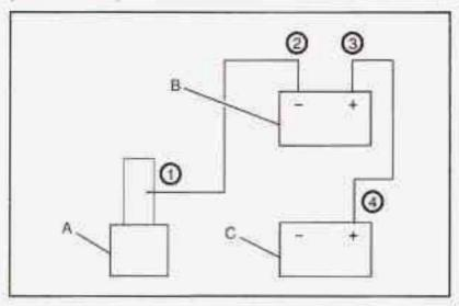
To disconnect the jumper cables from both vehicles, do the following:
