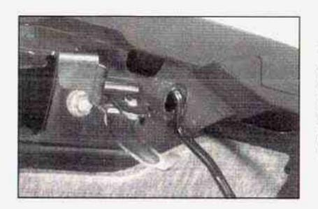
Release the hood prop from its retainer and put the hood prop into the slot in the hood.
