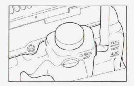
When the engine is cold, the coolant level should be at least up to the ADD mark. If it isn't, you may have a leak at the pressure cap or in the radiator hoses, heater hoses, radiator, water pump or somewhere else in the cooling system.
