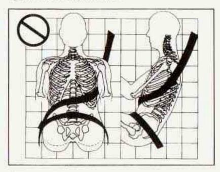
A: The shoulder belt is wern under the arm. It should be worn over the shoulder at all times.
