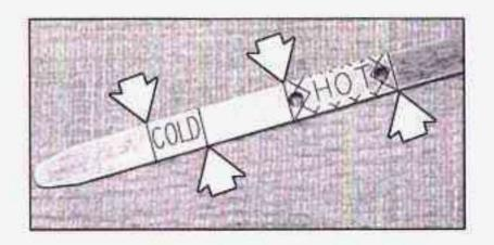
If the fluid level is in the acceptable range, push the dipstick back in all the way; then flip the handle down to lock the dipstick in place.
