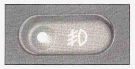
The fog lamp button is located on the instrument panel near the lamp control.
