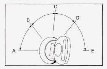
Notice: Don't operate accessories in the ACCESSORY position for long periods of time. Prolonged operation of accessories in the ACCESSORY position could drain your battery and prevent you from starting your vehicle.
