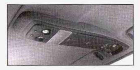
If your vehicle has this feature, the overhead console includes reading lamps, a compartment for a garage door opener, a temperature and compass display and a storage compartment for sunglasses.
