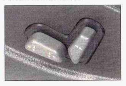
Horizontal Control: Raise or lower the front of the seat by raising or lowering the forward edge of the control. Raise or lower the rear of the seat by raising or lowering the rear edge of the control. Move the seat forward or rearward by moving the whole control toward the front or the rear of the vehicle.
