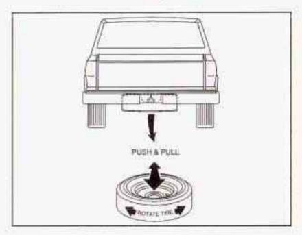
Make sure the tire is stored securely. Push, pull, and then try to rotate or turn the tire. If the tire moves, use the wheel wrench to tighten the cable. Follow this diagram for the inside-mounted spare.
