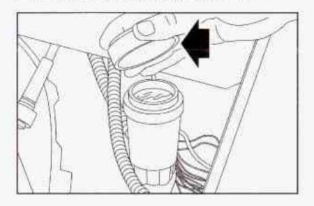
Refer to the Maintenance Schedule to determine how often you should check the fluid level in your clutch master cylinder reservoir and for the proper fluid. See Part B: Owner Checks and Services on page 6-26 and Part D: Recommended Fluids and Lubricants on page 6-33.
