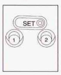
If your vehicle has this feature, the control located on the outboard side of the driver's seat looks like this. Use this memory function to save your seat cushion and seatback settings by using the following procedure:
