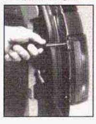
Remove the two screws from the lamp assembly.
