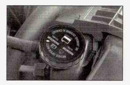
Then replace the pressure cap. At any time during this procedure if coolant begins to flow out of the filler neck, reinstall the pressure cap. Be sure the arrow on the pressure cap lines up like this.
