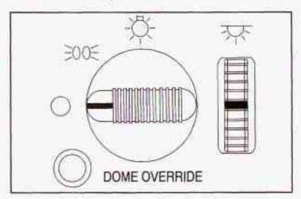
The control on the driver's side of the instrument panel operates the exterior lamps.
