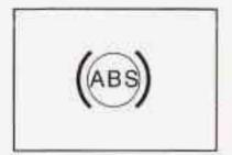
With the anti-lock brake system, this light will come on when you start your engine and may stay on for several seconds. That's normal.
