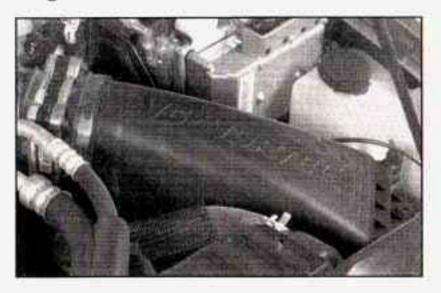
The engine air cleaner/filter is located toward the front of the engine compartment on the driver's side of the vehicle. See Engine Compartment Overview on page 5-12 for more information on the location of the engine air cleaner/filter.
