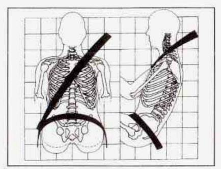
The lap part of the belt should be worn low and snug on the hips, just touching the thighs. In a crash, this applies force to the strong pelvic bones. And you'd be less likely to slide under the lap belt. If you slid under it, the belt would apply force at your abdomen. This could cause serious or even fatal injunes. The shoulder belt should go over the shoulder and across the chest. These parts of the body are best able to take belt restraining forces.
