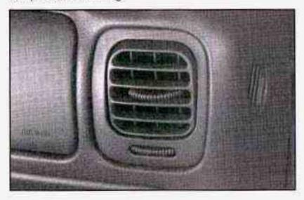
Use the thumbwheels located in the center and on the sides, to change the direction of the air flowing through the outlets.
