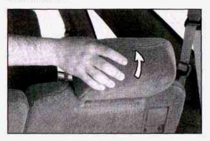
To return the head restraints to the upright position, reach behind the seats and pull the head restraint up until it locks into position. On two-door models with an inside mounted spare tire, the driver's side rear seat head restraint must be lifted and held upright as the seatback is raised. Otherwise, the head restraint will hit the spare tire and prevent the seatback from properly latching.
