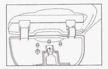
The pegs inside the compartment door are used to make sure the button on the compartment door will contact the control button on the garage door opener.
