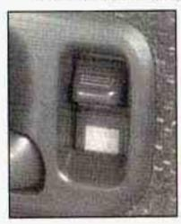
To manually lock a door from the inside, slide the manual lever on your door down. To manually unlock a door from the inside, slide the lever on the door up.
