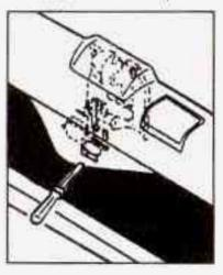
Use a thin object to reach through the access holes in both the trim panel and the hardware cover.
