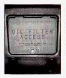
The access door for the remote oil filter is in the steering linkage shield assembly located under the radiator support.
