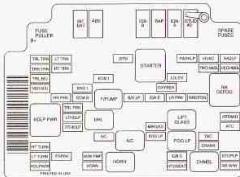
The engine compartment fuse block is located under the hood on the driver's side of the vehicle. See *Engine Compartment Overview* on page 5-12 for more information on location.
