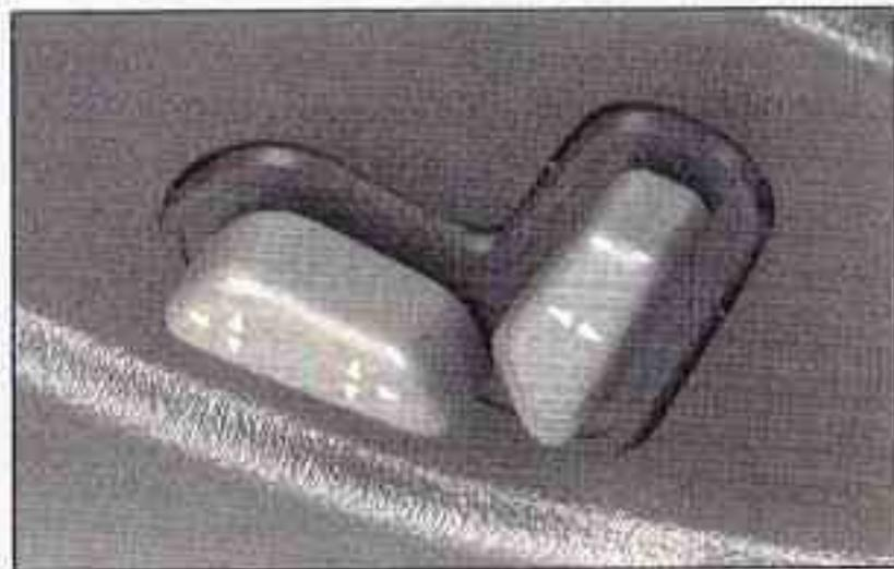
**Horizontal Control:** Raise or lower the front of the seat by raising or lowering the forward edge of the control.
