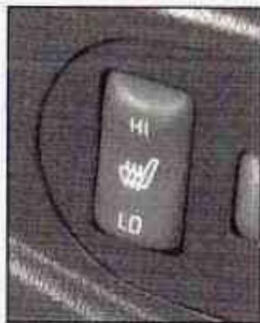
If your vehicle has this feature, the controls are located on the outboard side of the front seats.
