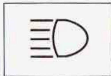
When the high beams are on, this indicator light on the instrument panel cluster will also be on.
