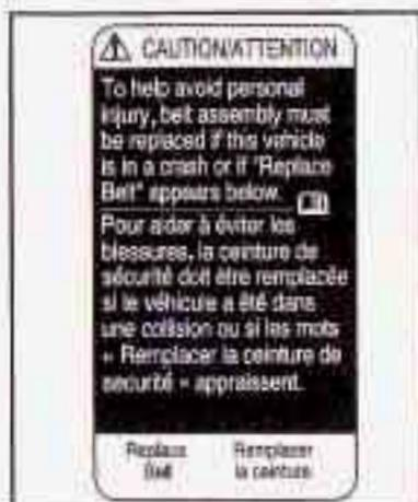
If you ever see a label on the driver's or the right front passenger's safety belt that says to replace the belt, be sure to do so. Then the new belt will be there to help protect you in a collision. You would see this label on the belt near the door opening.
