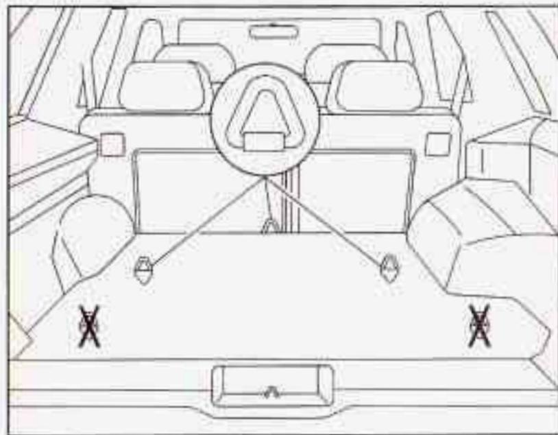
Anchor brackets for the rear outside seat positions are located on the floor in the cargo area of your vehicle.
