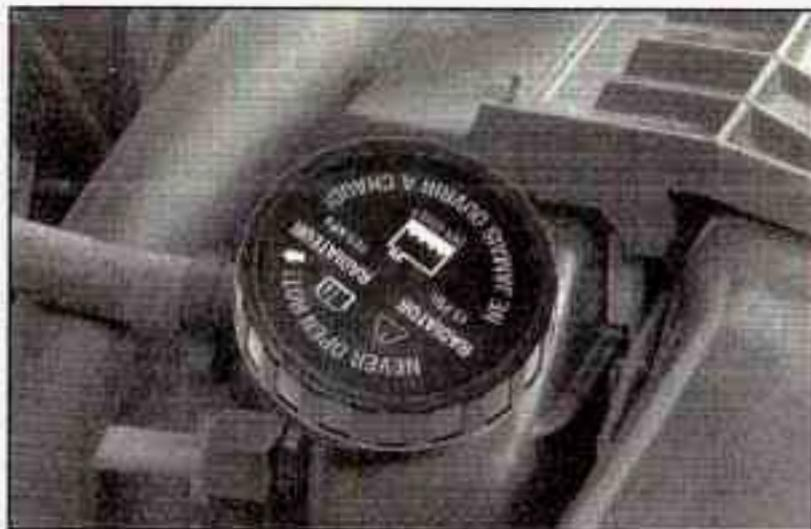
8. Then replace the pressure cap. At any time during this procedure if coolant begins to flow out of the filler neck, reinstall the pressure cap. Be sure the arrow on the pressure cap lines up like this.
