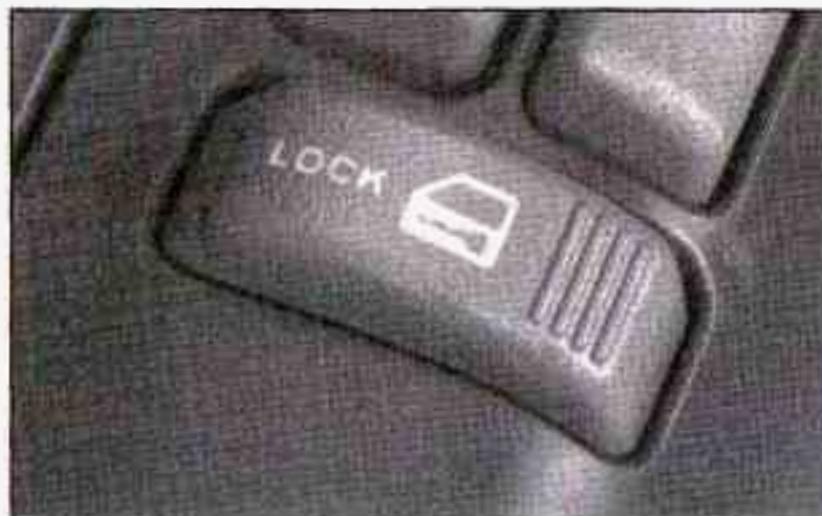
If your vehicle has power door locks, the switches are located on the driver's and the passenger's front armrests. Remove the ignition key and press LOCK to lock all the doors at once. To unlock the doors, press the raised area to the right of the key symbol.
