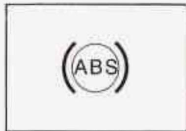
With the anti-lock brake system, this light will come on when you start your engine and may stay on for several seconds. That's normal.
