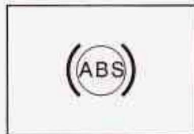
If there's a problem with the anti-lock brake system, this warning light will stay on. See *Anti-Lock Brake System Warning Light* on page 3-31.
