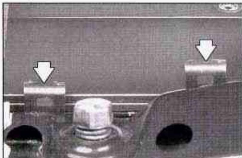
2. Remove the black retainer clips by lifting up.
