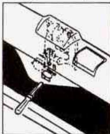
2. Use a thin object to reach through the access holes in both the trim panel and the hardware cover.
