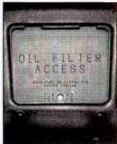
The access door for the remote oil filter is in the steering linkage shield assembly located under the radiator support. Turn the screw to unlock or lock the door. If you open the door, make sure it is securely closed when you are finished.
