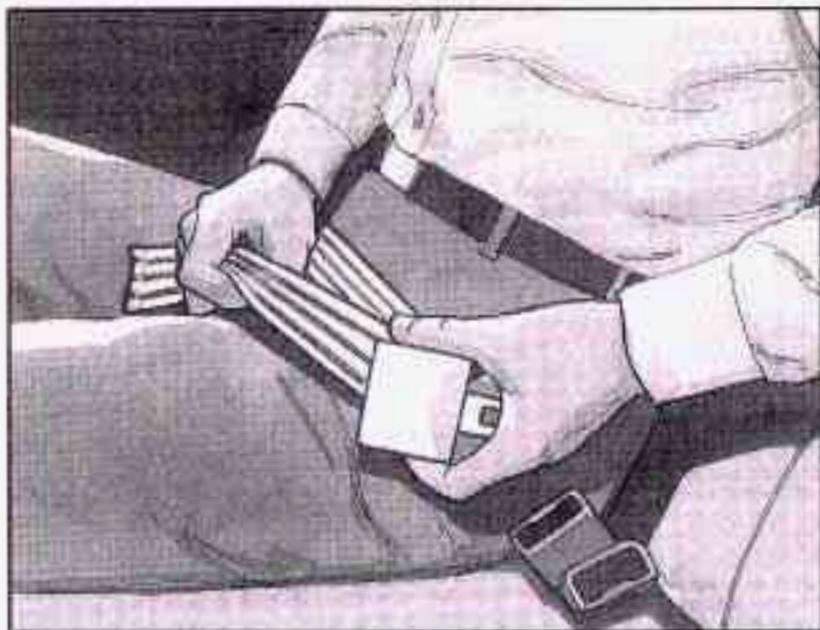
When you sit in the center front seating position, you have a lap safety belt, which has no retractor. To make the belt longer, tilt the latch plate and pull it along the belt.
