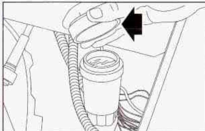
Refer to the Maintenance Schedule to determine how often you should check the fluid level in your clutch master cylinder reservoir and for the proper fluid. See *Part B: Owner Checks and Services* on page 6-26 and *Part D: Recommended Fluids and Lubricants* on page 6-33.
