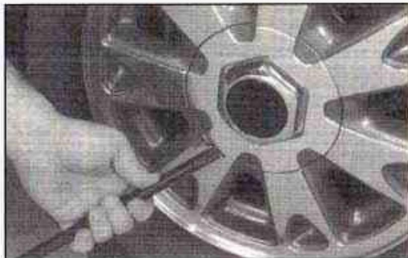
Position the chisel end of your wheel wrench, or the hub cap removal tool (if equipped), in the notch of the hub cap and pry off the hub cap.
