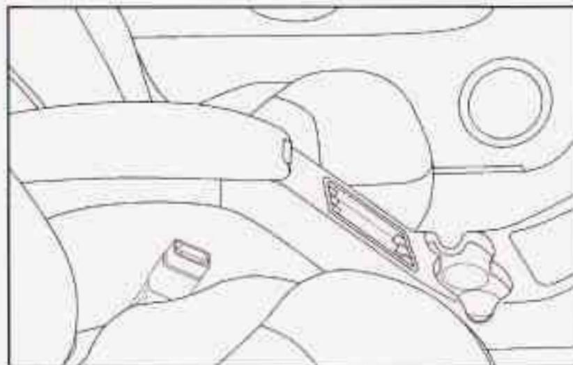
If your vehicle has this console compartment, squeeze the front lever while lifting the top to open it. You can store cassettes and compact discs in the slots in front of the compartment.
