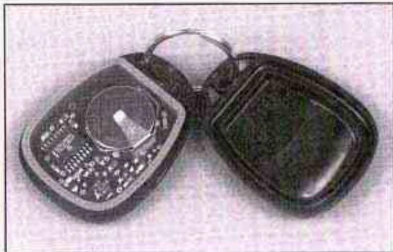
1. Insert an object like a thin coin in the slot between the covers of the transmitter housing near the key ring hole. Remove the bottom by twisting the object.
