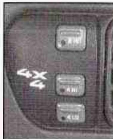
If your four-wheel-drive vehicle has the electronic transfer case, the transfer case buttons are to the right of the steering wheel on the instrument panel.
