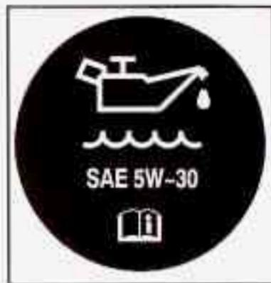
The engine oil fill cap is located in the engine compartment toward the passenger side of the vehicle.
