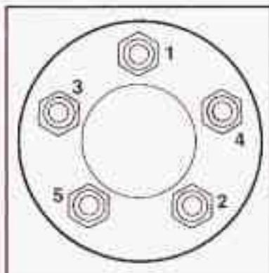
11. Use the wrench to tighten the wheel nuts firmly in a crisscross sequence as shown.
