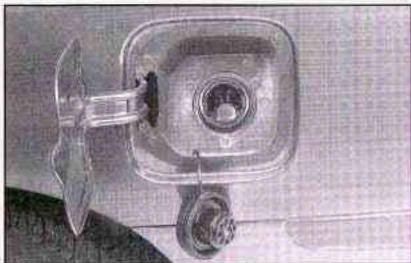
While refueling, hang the cap by the tether from the hook on the fuel filler door.
