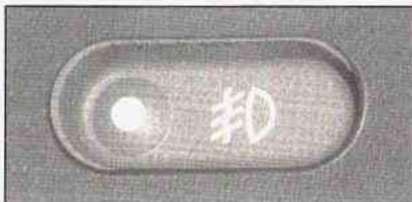
The fog lamp button is located on the instrument panel near the lamp control.
