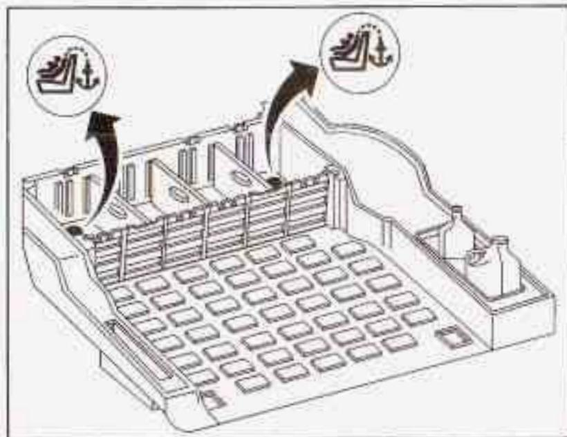
If your vehicle is equipped with the rear convenience system, there will be plugs covering the anchor brackets. To remove the plugs, grasp the edges of the plugs and pull them out. See "Rear Convenience System" in the Index for more information. Don't use the rear set of tie-down brackets near the liftgate/endgate or the center tie-down bracket near the rear seats.
