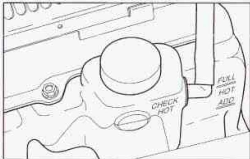
The coolant recovery tank is located in the engine compartment near the passenger side of the vehicle. See *Engine Compartment Overview* on page 5-12 for more information on location.
