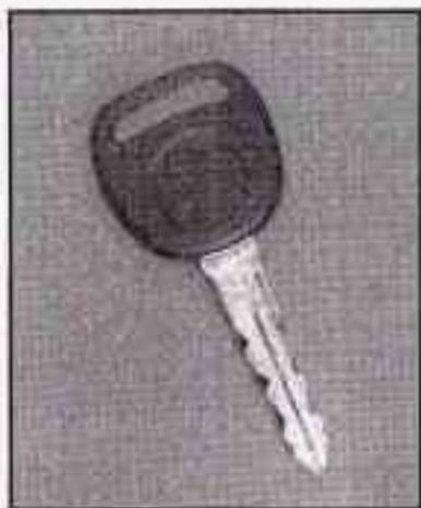
This vehicle has one double-sided key for the ignition, tailgate and door locks. It will fit with either side up.
