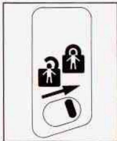
The security lock lever is located on the inside edge of each rear door.
