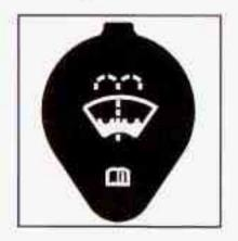
Open the cap with the washer symbol on it. Add washer fluid until the tank is full.
