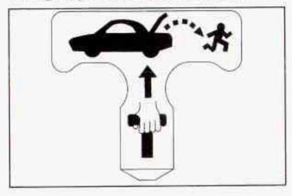
Notice: The emergency trunk release handle is not designed to be used to tie down the trunk lid or as an anchor point when securing items in the trunk. Improper use of the emergency trunk release nandie could damage it. There is a glow-in-the-dark emergency trunk release handle located on the inside of the trunk lid of your vehicle. This handle will glow following exposure to light. Pull the release handle up to open the trunk from the inside.
