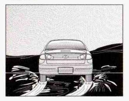
What's the worst time for this? "Wet ice." Very cold snow or ice can be slick and hard to drive on. But wet ice can be even more trouble because it may offer the least traction of all. You can get wet ice when it's about freezing (32"F; 0"C) and freezing rain begins to fall. Try to avoid driving on wet ice until salt and sand crews can get there.
