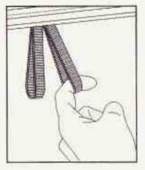
Pull the release straps located in the trunk. The right strap operates the passenger's side rear split seat. The left strap operates the driver's side rear split seat.
