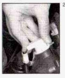
Hold down the tab at the top of the bulb retainer. Twist the retainer one-eighth of a turn counterclockwise and pull the assembly out.
