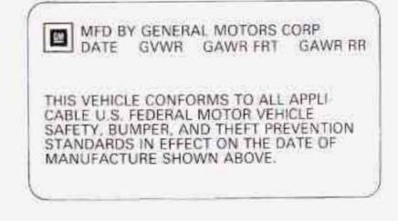
The other label is the Certification label, found on the rear edge of the driver's door. It tells you the gross weight capacity of your vehicle, called the Gross Vehicle Weight Rating (GVWR). The GVWR includes the weight of the vehicle, all occupants, fuel and cargo. Never exceed the GVWR for your vehicle, or the Gross Axle Weight Rating (GAWR) for either the front or rear axle.
