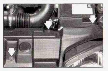
Remove the plastic fasteners from the shield. Use a tool to pry up the center of the fastener. Be careful not to break the fasteners that hold the shield in place.
