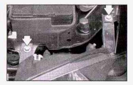
Remove the two bolts from the headlamp assembly. Pull the headlamp assembly up and toward the front of the vehicle to access the bulb assembly.
