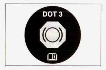
Your brake master cylinder reservoir is on the driver's side of the engine compartment. It is filled with DOT-3 brake fluid. See Engine Compartment Overview on page 5-12.
