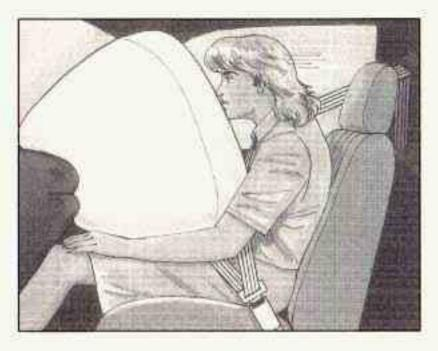
The right front passenger's air bag is in the instrument panel on the passenger's side.
