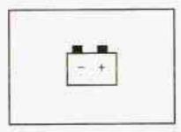
The charging system light will come on briefly when you turn on the ignition, and the engine is not running, as a check to show you it is working,
