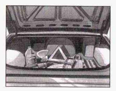
Include an ice scraper, a small brush or broom, a supply of windshield washer fluid, a rag, some winter outer clothing, a small shovel, a flashlight, a red cloth and a couple of reflective warning triangles. And, if you will be driving under severe conditions, include a small bag of sand, a piece of old carpet or a couple of burtap bags to help provide traction. Be sure you properly secure these items in your vehicle.
