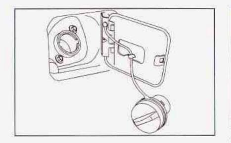
While refueling, hang the fuel cap inside the fuel door by placing the fuel cap tether in the hanger.
