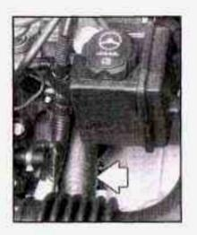
With the coolant surge tank pressure cap off, start the engine and let it run until you can feel the upper radiator hose getting hot. Watch out for the engine cooling fan.
