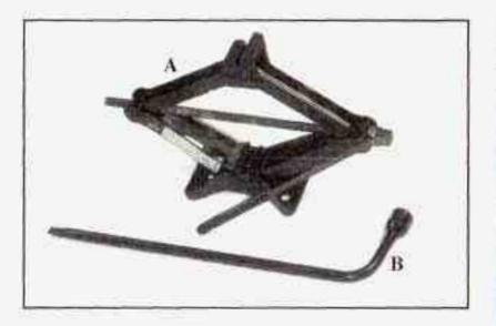
The tools you'll be using include the jack (A) and wheel wrench (B). Removing the Flat Tire and Installing the Spare Tire
