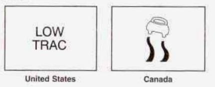
When your Enhanced Traction System is limiting wheel spin, this light will come on. Slippery road conditions may exist if the Enhanced Traction System active light comes on, so adjust your driving accordingly.
