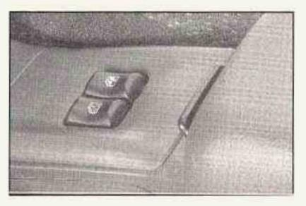
If your vehicle has this feature, the switches on the center console control each of the power windows when the ignition is on. In addition, on four-door models, each rear passenger door has a control switch for its own window. To lower a window, press and hold the rear of the switch. To raise the window, press and hold the switch forward.
