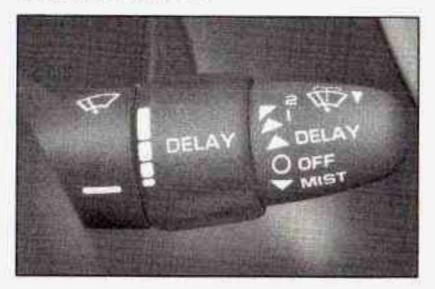
Use this lever located on the right side of the steering wheel to operate the windshield wipers.
