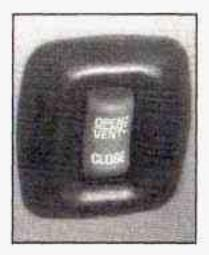
Your vehicle may have a sunroof. With the ignition on, press and hold the rear of the switch and the glass panel will open to the vent position. Open the sunshade by hand when using the vent position.
