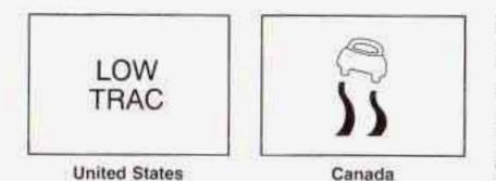
This light will come on when your Enhanced Traction System is limiting wheel spin. See Enhanced Traction System Active Light on page 3-29.
