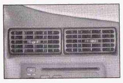
Use the louvers located on the air outlets to change the direction of the airflow.
