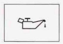
If the oil pressure light appears on the instrument cluster, it means you need to check your engine oil level right away.
