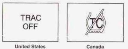
When the transaxle shift lever is in any position other than FIRST (1) or SECOND (2) and the parking brake is fully released, this warning light will come on to let you know if there's a problem with the system. See Enhanced Traction System Warning Light on page 3-28. When this warning light is on, the system will not limit wheel spin. Adjust your driving accordingly.
