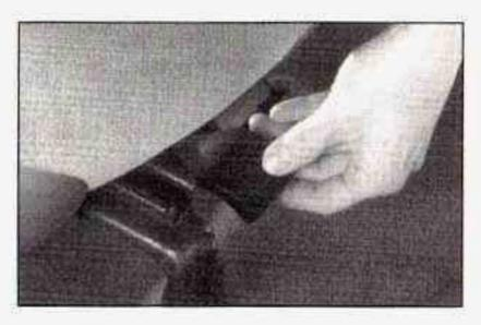
If your vehicle is equipped with easy entry seats, this is your front passenger seat adjuster. Pull up on the lever located at the front of the passenger's seat up to unlock it. Slide the seat to a comfortable position and release the lever. Then try to move the seat with your body, to make sure the seat is locked into place.
