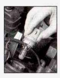
Remove the bulb by pulling it straight out.
