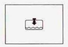
If the low coolant light comes on and stays on, it means you're low on engine coolant. See Low Coolant Warning Light on page 3-30.
