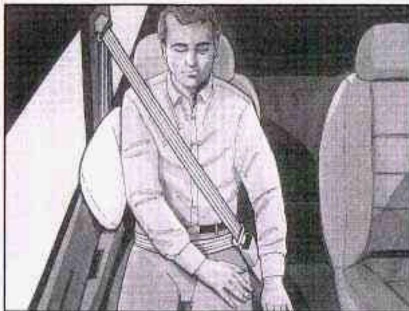
If your vehicle has one, the passenger's side impact air bag is in the side of the passenger's seatback closest to the door.
