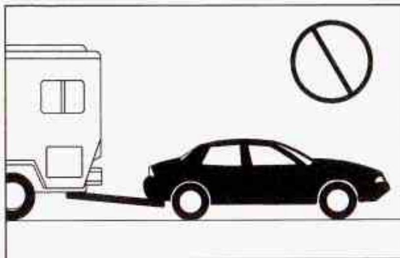
**Notice:** Do not tow your vehicle from the rear. Your vehicle could be badly damaged and the repairs would not be covered by your warranty.
