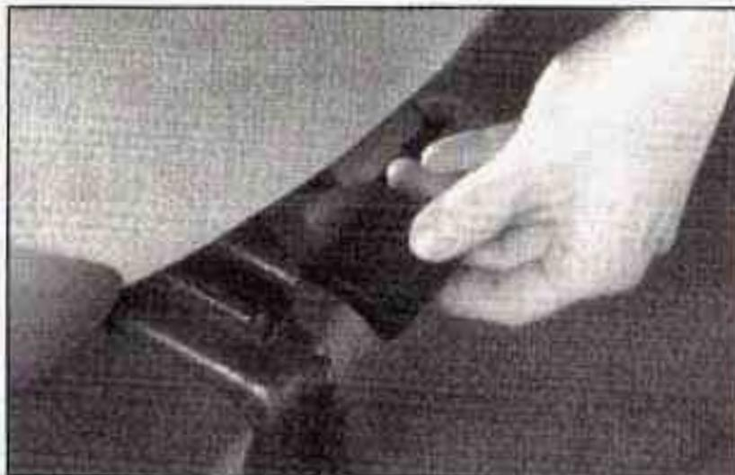
If your vehicle is equipped with easy entry seats, this is your front passenger seat adjuster. Pull up on the lever located at the front of the passenger's seat up to unlock it. Slide the seat to a comfortable position and release the lever. Then try to move the seat with your body, to make sure the seat is locked into place.
