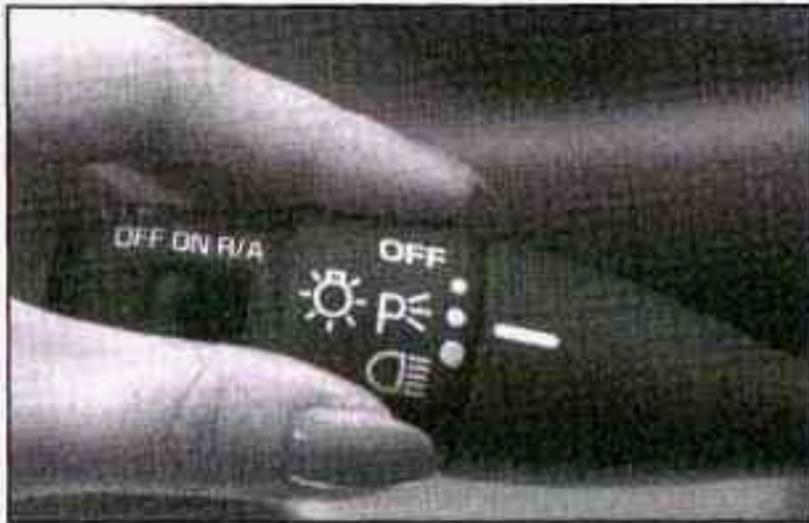
The exterior lamp band on the turn signal/multifunction lever controls the exterior lamps.
