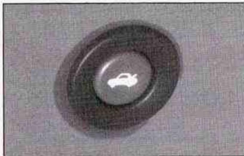
Press the remote trunk release button, located on the lower left side of the instrument panel, to release the trunk lid.
