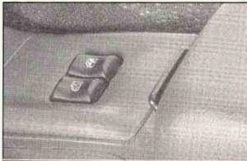
If your vehicle has this feature, the switches on the center console control each of the power windows when the ignition is on. In addition, on four-door models, each rear passenger door has a control switch for its own window.
