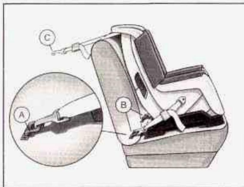
In order to use the system, you need either a forward-facing child restraint that has attaching points (B) at its base and a top tether anchor (C), or a rear-facing child restraint that has attaching points (B), as shown here.
