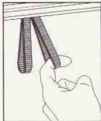
1. Pull the release straps located in the trunk. The right strap operates the passenger's side rear split seat. The left strap operates the driver's side rear split seat.
