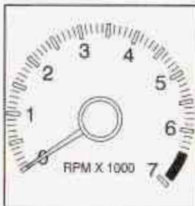
If your vehicle has this feature, the tachometer displays the engine speed in revolutions per minute (rpm).
