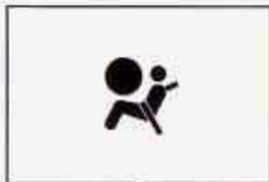
There is an air bag readiness light on the instrument panel, which shows the air bag symbol.
