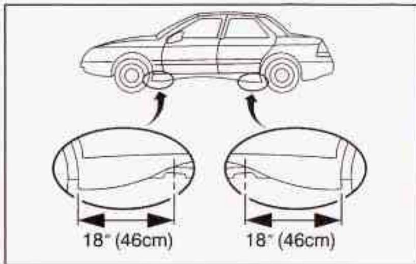
3. Near each wheel well is a notch in the frame which the jack head fits in. The front notch is 9 inches (23 cm) back from the front wheel well. The rear notch is 8 inches (20 cm) forward from the rear wheel well. As is shown in the diagram above, if your vehicle has flared side moldings, both front and rear notches are 18 inches (46 cm) from the wheel wells.
