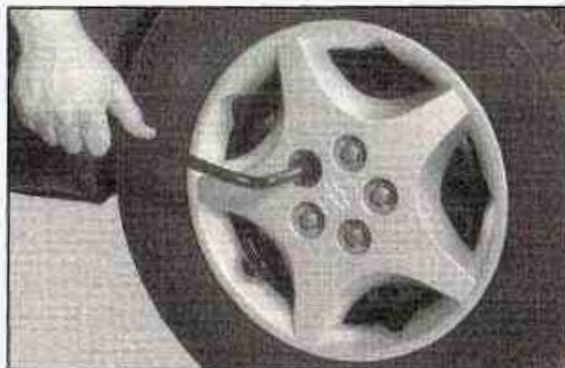
1. If your vehicle is equipped with wheel covers, use the wheel wrench to begin loosening the plastic wheel nut caps. Once you have loosened the plastic wheel nut caps with the wheel wrench you can finish loosening them with your fingers. Using the flat end of the wheel wrench, pry along the edge of the wheel cover until it comes off.
