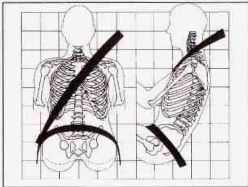
The lap part of the belt should be worn low and snug on the hips, just touching the thighs. In a crash this applies force to the strong pelvic bones. And you'd be less likely to slide under the lap belt. If you slid under it,
