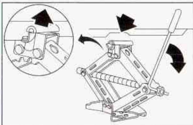
4. Raise the vehicle by turning the jack handle clockwise. Raise the vehicle far enough off the ground so there is enough room for the compact spare tire to fit underneath the wheel well.
