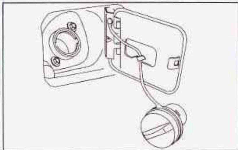
While refueling, hang the fuel cap inside the fuel door by placing the fuel cap tether in the hanger.
