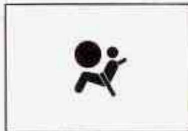
This light will come on when you start your vehicle, and it will flash for a few seconds. Then the light should go out. This means the system is ready.
