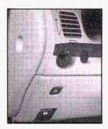
Some fuses are in a fuse block at the end of the instrument panel on the driver's side of the vehicle. Pull off the cover labeled FUSES to expose the fuses.
