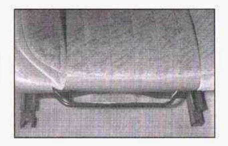
If your vehicle has the manual seat, lift the bar located under the front of the seat to unlock it. Slide the seat to where you want it and release the bar. Try to move the seat back and forth to be sure the seat is locked in place.
