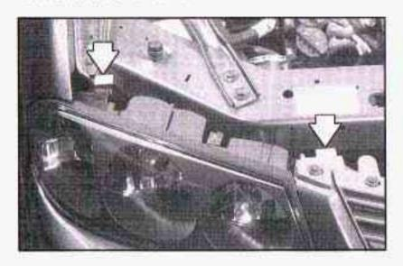
Remove the two headlamp fasteners by pulling up on them.
