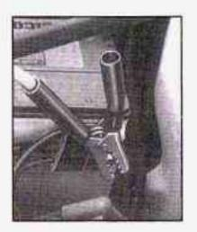
Now connect the black negative (-) cable to the negative (-) terminal location of the vehicle with the good battery. Use a remote negative (-) terminal if the vehicle has one. Don't let the other end touch anything until the next step. The other end of the negative (-) cable doesn't go to the dead battery. It goes to a heavy, unpainted metal part or to a remote negative (-) terminal on the vehicle with the dead battery.
