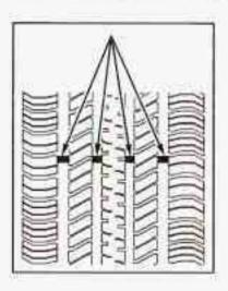
One way to tell when it's time for new tires is to check the treadwear indicators, which will appear when your tires have only 1/16 inch (1.6 mm) or less of tread remaining. You need a new tire if any of the following statements are true:
