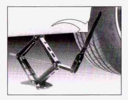
Raise the vehicle by turning the jack handle clockwise. Raise the vehicle far enough off the ground for the compact spare tire to fit underneath the wheel well of the vehicle. Remove all wheel nuts and take off the flat tire.
