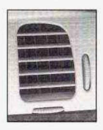
Use the knob located below or to the side of the outlet, to change the direction of the air flow.
