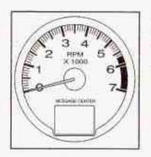
Your vehicle may have a tachometer that displays the engine speed in thousands of revolutions per minute (rpm).
