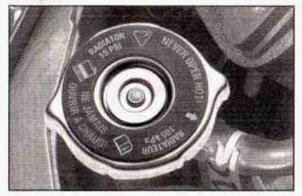
The radiator pressure cap is located in the front of the engine compartment near the diagonal cross brace on the passenger's side of the vehicle. See Engine Compartment Overview on page 5-12 for more information on location. You can remove the radiator pressure cap when the cooling system, including the radiator pressure cap and upper radiator hose, is no longer hot.
