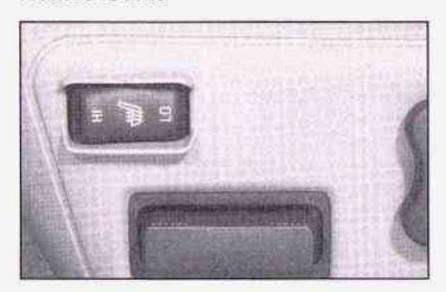
If your vehicle has this option, both the driver's and passenger's heated seat switches are located on the outboard sides of the seats near the front.
