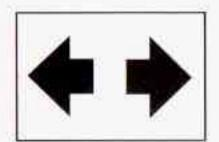
An arrow on the instrument panel cluster will flash in the direction of the turn or lane change.
