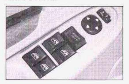
Switches located on the driver's door armrest control each of the windows when the Ignition is in ON, ACC, or when Retained Accessory Power (RAP) is active. See "Retained Accessory Power (RAP)" under Ignition Positions on page 2-18.
