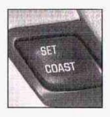
Press the SET button on the steering wheel and release it
