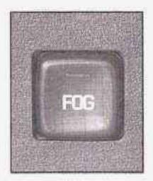
If your vehicle is equipped with fog lamps, the button is located on the instrument panel next to the exterior lamps control wheel to the left of the steering column.
