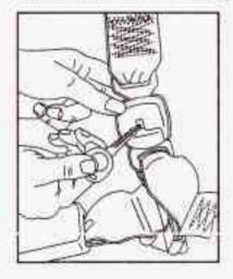
Remove the rear center lap-shoulder belt latch by pressing the release button.
