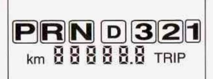
There is also a display, like the graphic above, located on the instrument panel cluster that will indicate the gear the vehicle is in.
