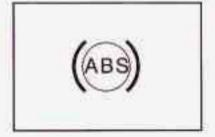
If your vehicle is equipped with anti-lock brakes, the anti-lock brake system warning light should come on for a few seconds when you turn the ignition key to ON.
