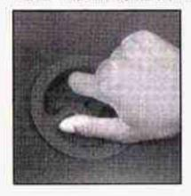
Turn the center nut on the compact spare tire cover counterclockwise to remove it. Then remove the cover.
