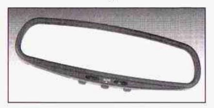
Your vehicle may be equipped with an automatic dimming rearview mirror. Push the button in the center of the mirror to turn this feature on. The mirror will darken gradually to reduce glare from headlamps behind you. This may take a few moments. The mirror will lighten whenever you shift to REVERSE (R).
