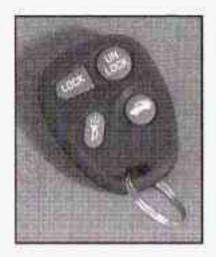
Using the remote keyless entry transmitter, you can lock and unlock your doors or release your trunk from about 3 feet (1 m) up to 30 feet (9 m) away.
