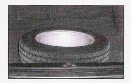
When storing a full-size tire, use the extension and protector guide located in the foam holder to help prevent wheel surface damage. To store a full-size tire do the following:
