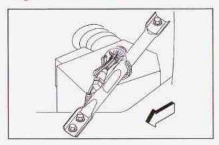
Your vehicle may be equipped with this feature. In very cold weather, 0°F (-18°C) or colder, the engine coolant heater can help. You'll get easier starting and better fuel economy during engine warm-up. Usually, the coolant heater should be plugged in a minimum of four hours prior to starting your vehicle. At temperatures above 32°F (0°C), use of the coolant heater is not required.
