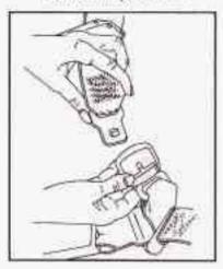
Reconnect the center safety belt latch plate to the buckle.
