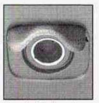
Your vehicle has a 12-volt outlet which can be used to plug in electrical equipment such as a cellular telephone, a compact disc player, etc.
