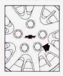
If your vehicle is equipped with wheel covers, loosen the plastic nut caps with the wheel wrench in a counter clockwise direction.
