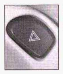
The hazard warning flasher button is located to the right of the steering wheel on the instrument panel cluster.
