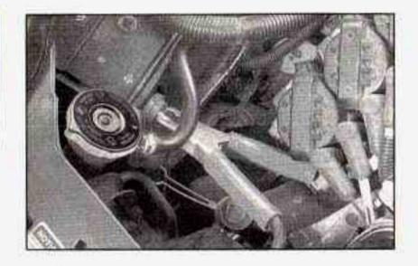
Connect the red positive (+) cable to the positive (+) terminal location of the vehicle with the dead battery. Use a remote positive (+) terminal if the vehicle has one.
