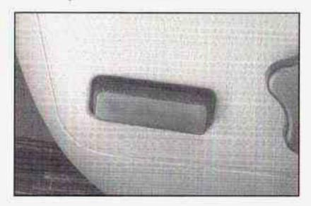
If your vehicle has this feature, the control is located on the outboard side of the front seats toward the front of the seat cushion. To adjust the seat do any of the following:
