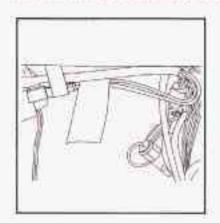
It is located on the passenger's side of the vehicle, under the glove box, and is labeled with a wire function and fuse rating. Notice: Adding some electrical equipment to your vehicle can damage it or keep other things from working as they should. This wouldn't be covered by your warranty. Check with your dealer before adding electrical equipment, and never use anything that exceeds the amperage rating.
