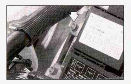
To uncover the remote positive (+) terminal, lift the plastic cap. You should always use the remote positive (+) terminal instead of the positive (+) terminal on the battery.
