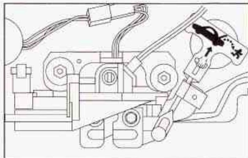
There is a glow-in-the-dark trunk release handle located inside the trunk on the latch. This handle will glow following exposure to light. Pull the release handle up to open the trunk from the inside.
