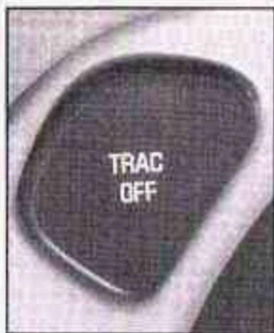
To turn the system on or off, press the TRAC OFF button on the left side of the instrument panel.
