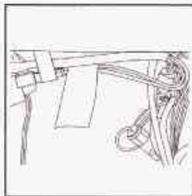
It is located on the passenger's side of the vehicle, under the glove box, and is labeled with a wire function and fuse rating.
