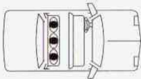
To assist you in locating the lower anchors for this child restraint system, each seating position with the LATCH system will have a dot on the seatback directly above the anchor.
