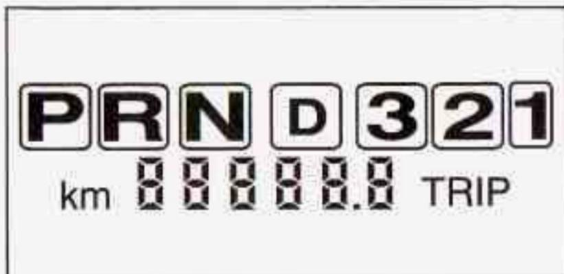
There is also a display, like the graphic above, located on the instrument panel cluster that will indicate the gear the vehicle is in.
