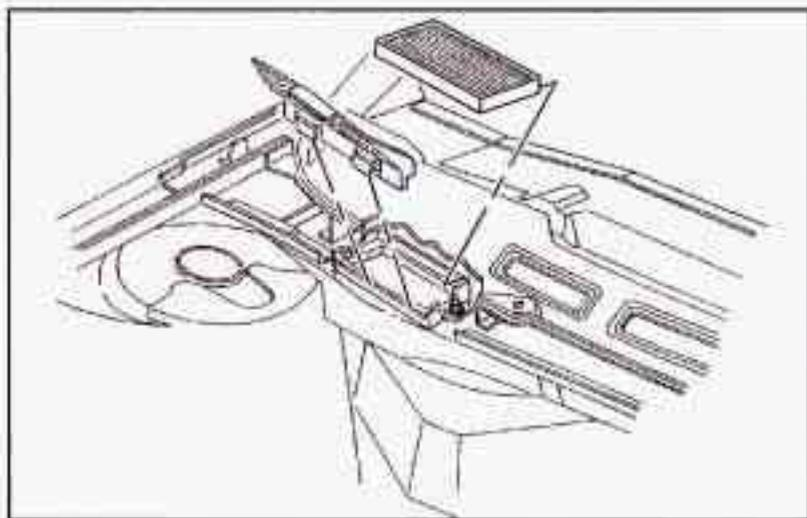
5. Remove the air inlet grille retainers.
