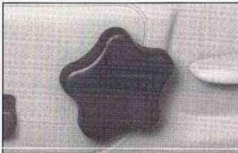
If your vehicle has this feature, the knob is located on the outboard side of the driver's seat. Turn the knob toward the front of the vehicle to increase lumbar support. Turn the knob toward the rear of the vehicle to decrease lumbar support.
