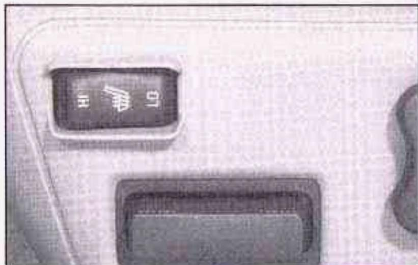
If your vehicle has this option, both the driver's and passenger's heated seat switches are located on the outboard sides of the seats near the front.
