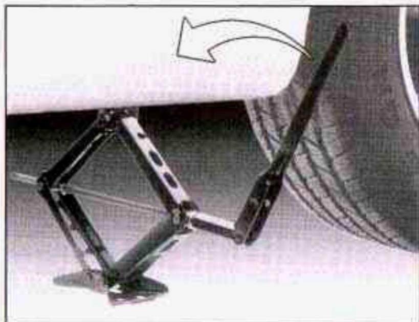
6. Lower the vehicle by turning the jack handle counterclockwise. Lower the jack completely.
