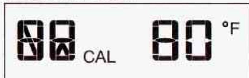
To calibrate the compass, in an area free from large metal objects, make one to two 360° turns. The calibration symbol will turn off and the compass reading will be displayed.
