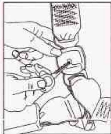
1. Remove the rear center lap-shoulder belt latch by pressing the release button.
