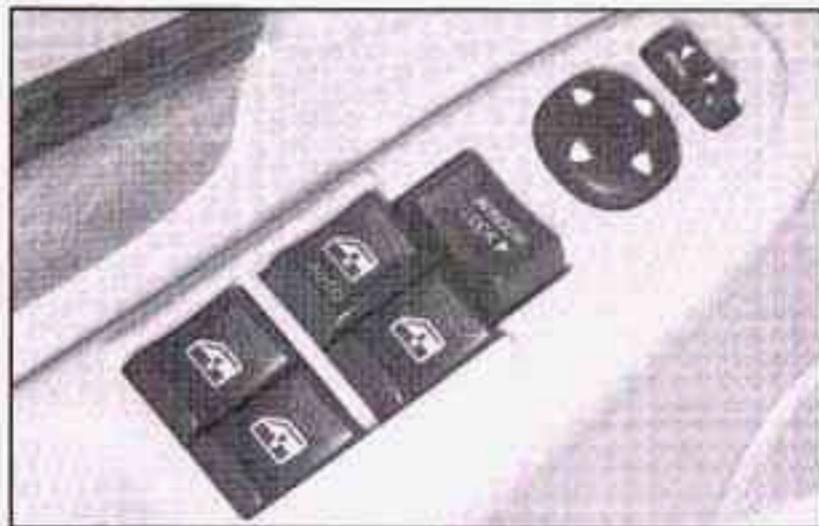
Switches located on the driver's door armrest control each of the windows when the Ignition is in ON, ACC, or when Retained Accessory Power (RAP) is active. See "Retained Accessory Power (RAP)" under *Ignition Positions* on page 2-18.
