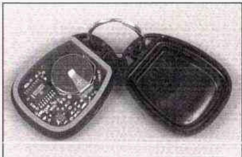
**Notice:** When replacing the battery, use care not to touch any of the circuitry. Static from your body transferred to these surfaces may damage the transmitter.
