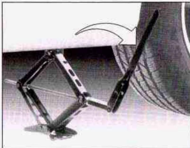
2. Raise the vehicle by turning the jack handle clockwise. Raise the vehicle far enough off the ground for the compact spare tire to fit underneath the wheel well of the vehicle. Remove all wheel nuts and take off the flat tire.
