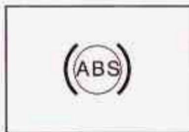
If your vehicle is equipped with anti-lock brakes, the anti-lock brake system warning light should come on for a few seconds when you turn the ignition key to ON.
