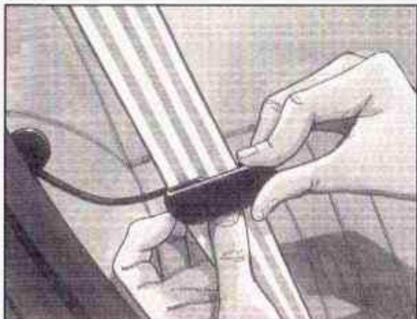
2. Slide the guide under and past the belt. The elastic cord must be under the belt. Then, place the guide over the belt, and insert the two edges of the belt into the slots of the guide.
