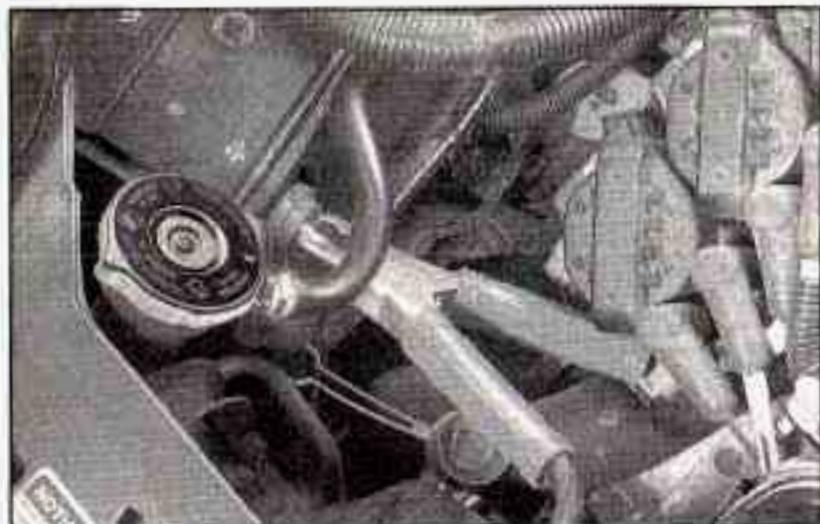
6. Connect the red positive (+) cable to the positive (+) terminal location of the vehicle with the dead battery. Use a remote positive (+) terminal if the vehicle has one.
