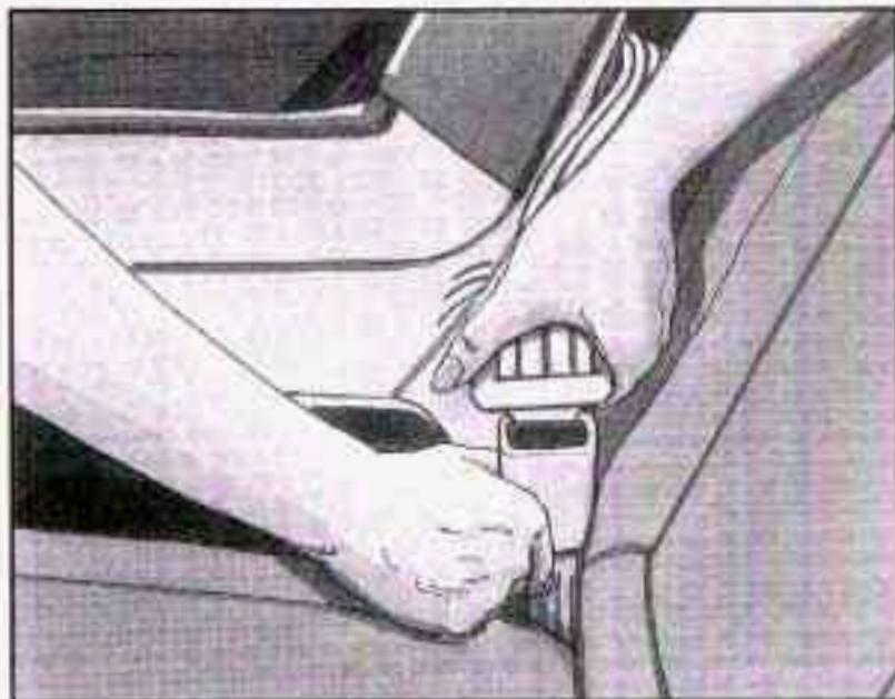
You'll be using the lap-shoulder belt. See *Top Strap on page 1-41* if the child restraint has one. Be sure to follow the instructions that came with the child restraint. Secure the child in the child restraint when and as the instructions say.
