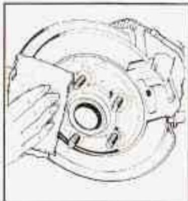
3. Remove any rust or dirt from the wheel bolts, mounting surfaces and spare wheel.
