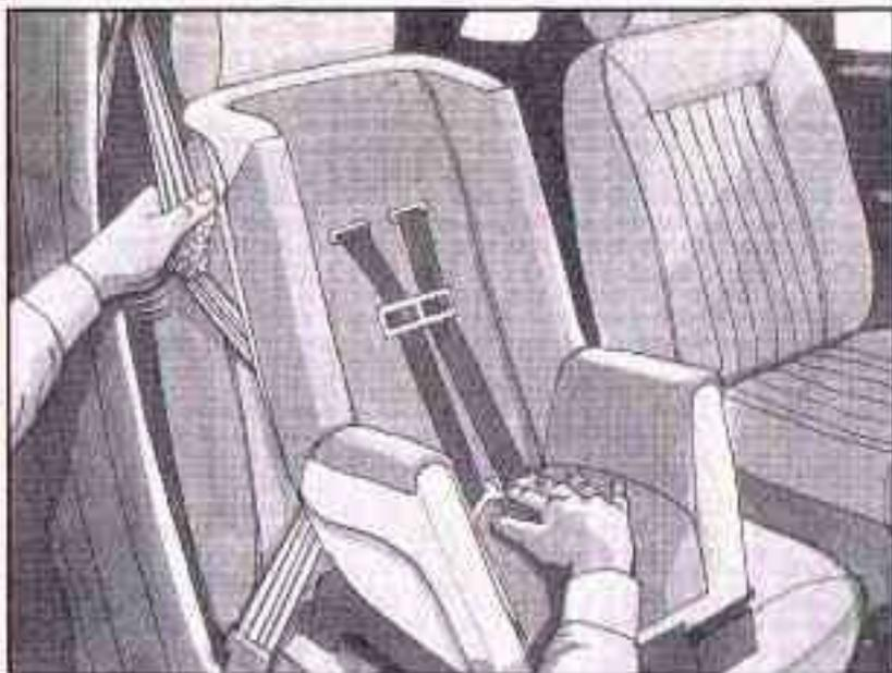
6. To tighten the belt, feed the shoulder belt back into the retractor while you push down on the child restraint. You may find it helpful to use your knee to push down on the child restraint as you tighten the belt.
