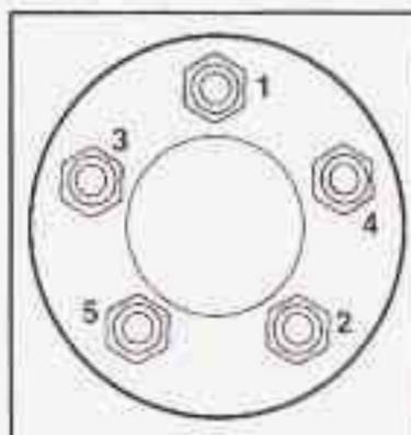
7. Tighten the wheel nuts firmly in a crisscross sequence as shown.
