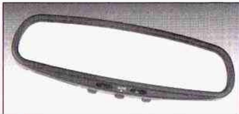
Your vehicle may be equipped with an automatic dimming rearview mirror. Push the button in the center of the mirror to turn this feature on. The mirror will darken gradually to reduce glare from headlamps behind you. This may take a few moments. The mirror will lighten whenever you shift to REVERSE (R).
