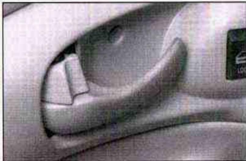
To lock the door from the inside, push the manual lock lever forward. To unlock the door, pull the lever rearward.
