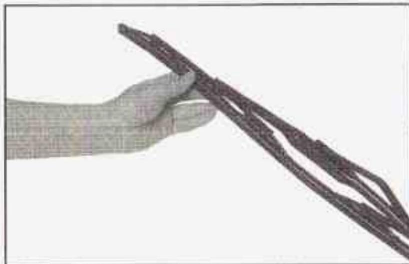
4. While holding the wiper arm away from the glass, push the release clip from under the blade connecting point and pull the old blade assembly down toward the glass to remove it from the wiper arm.
