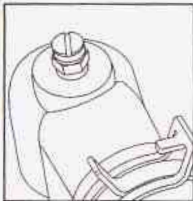
3400 V6 Bleed Valve #1
