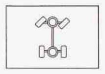
An 4WD indicator light will illuminate when you shift into four-wheel drive and the front axle engages.
