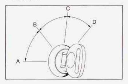
A (LOCK): This position locks your ignition and manual transmission. It's a theft-deterrent feature. You will only be able to remove your key when the ignition is turned to LOCK.
