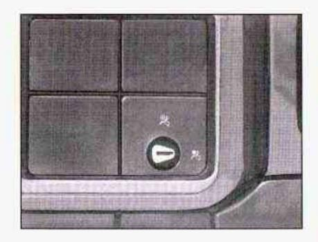
In addition to the AIR BAG OFF switch, your vehicle may have the passenger sensing system. The passenger sensing system is designed to turn off the right front passenger's frontal air bag when a rear facing child restraint is in the right front seat. In addition to the passenger sensing system, you may use the AIR BAG OFF switch located on the instrument panel to turn the air bag off. See Air Bag Off Switch on page 1-68 and Passenger Sensing System on
