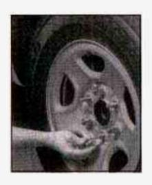
After mounting the spare, reinstall the wheel nuts with the rounded end of the nuts toward the wheel. Tighten each wheel nut by hand using the wheel wrench until the wheel is held against the hub.
