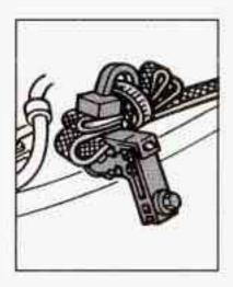
In very cold weather, 0°F (-18°C) or colder, the engine coolant heater can help. You'll get easier starting and better fuel economy during engine warm-up. Usually, the coolant heater should be plugged in a minimum of four hours prior to starting your vehicle.
