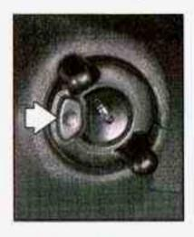
The ignition key cannot be removed from the ignition of manual transmission vehicles unless the key release button is used.
