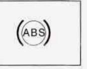
If there's a problem with the anti-lock brake system, this warning light will stay on. See Anti-Lock Brake System Warning Light on page 3-41.
