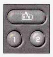
If your vehicle has this feature, then the controls for the memory function are located on the driver's door.
