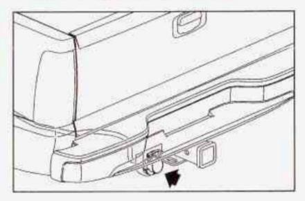
Your pickup may be equipped with the eight-wire trailer towing hamess. This hamess with a seven-pin universal trailer connector is attached to a bracket on the hitch platform.\*
