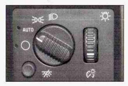
The switch on the driver's side of your instrument panel operates the exterior lamps.
