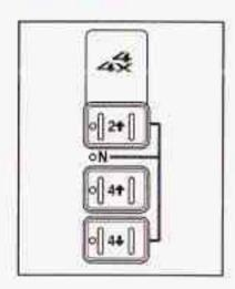
If your four-wheel-drive vehicle has the electronic transfer case, the transfer case switches are located to the left of the instrument panel cluster. Use these switches to shift into and out of four-wheel drive. You can choose among three driving settings:
