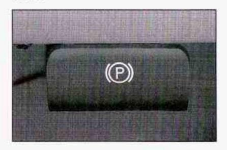
To release the parking brake, hold the regular brake pedal down. Pull the bottom edge of the lever, located above the parking brake pedal, with the parking brake symbol, to release the parking brake. If the ignition is on when the parking brake is released, the brake system warning light will go off.
