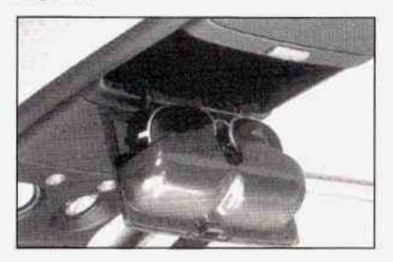
To open the center compartment, press the release button located at the rear of the compartment door. Place your sunglasses in the compartment door with the lenses facing out.
