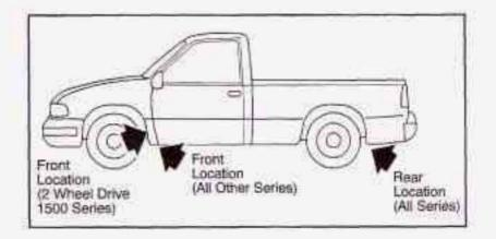
Position the jack under the vehicle. If the flat tire is
