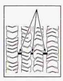
One way to tell when it's time for new tires is to check the treadwear indicators, which will appear when your tires have only 1/16 inch (1.6 mm) or less of tread remaining. Some commercial truck tires may not have treadwear indicators.
