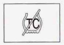
When the traction off light is on, the TAS is off and will not limit wheel spin. Adjust your driving accordingly. The traction off light will come on under the following conditions:
