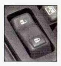
If your vehicle has this power door lock switch, press the raised side of the switch, with the lock symbol, on either front door to lock all the doors at once.
