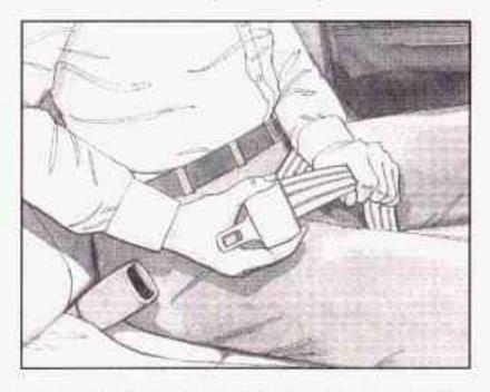
Your lap safety belt has no retractor. To make the belt longer, tilt the latch plate and pull it along the belt.
