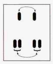
If your vehicle has dual rear wheels and the tread design for the front tires is different from the dual rear tires, always use the correct rotation pattern shown here when rotating your tires. The dual tires are rotated as a pair, and the inside rear tires became the outside rear tires.
