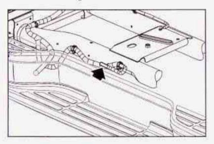
The six-wire harness is located at the rear of the vehicle and is tied to the vehicle's frame. The harness requires the installation of a trailer-wiring harness connector, which is available through your dealer. The six-wire harness contains the following trailer circuits:
