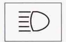
When the high beams are on, this light on the instrument panel cluster also will be on.
