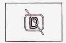
This light will illuminate when the overdrive disable feature is activated. The overdrive disable feature will prevent your vehicle from shifting into fifth (5) gear.
