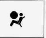
This light will come on when you start your vehicle, and it will flash for a few seconds. Then the light should go out. This means the system is ready.
