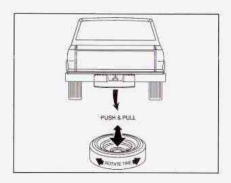
Make sure the tire is stored securely. Push, pull, and then try to rotate or turn the tire. If the tire moves, use the wheel wrench/hoist shaft to tighten the cable.
