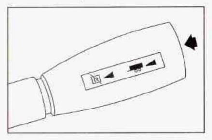
If your vehicle has an Allison Transmission you may have the overdrive disable feature. The overdrive disable feature prevents the transmission from shifting into fifth (5) gear. The selector button is located on the end of the column shift lever. You can turn overdrive disable on and off by pressing and holding the button at the end of the column shift lever until the indicator light, on the instrument panel, illuminates.
