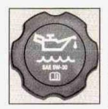
The engine oil fill cap for the VORTEC 4800, 5300 and 6000 V8 engines is located on the engine valve cover on the passenger's side of the vehicle. On the 8100 engine, the oil fill cap is located on the front of the engine. See Engine Compartment Overview on page 5-12 for more information on location.
