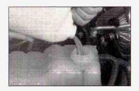
Then fill the coolant surge tank with the proper mixture, to the FULL COLD mark.
