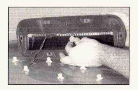
Reinstall the lens and tighten the screws.
