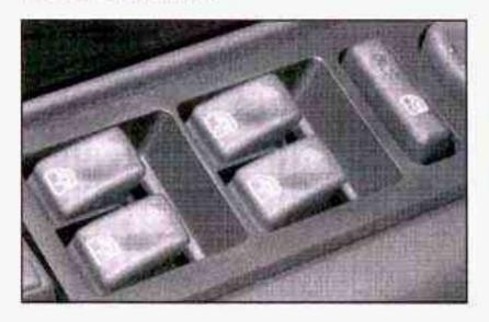
If your vehicle is equipped with power windows, the controls are located on each of the side doors in the front and rear. The driver's door has a switch for the passenger window as well. Your power windows will work when the ignition has been turned to ACCESSORY or RUN or when Retained Accessory Power (RAP) is active. See "Retained Accessory Power" under Ignition Positions on page 2-21.
