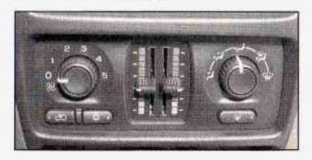
(Fan): Turn the left knob clockwise or counterclockwise to increase or decrease the fan speed. Turn the knob to the off position to turn off the fan. If the knob is in off outside air will still enter the vehicle, and will be directed based on the position of the mode knob. The temperature can also be adjusted using the temperature levers.
