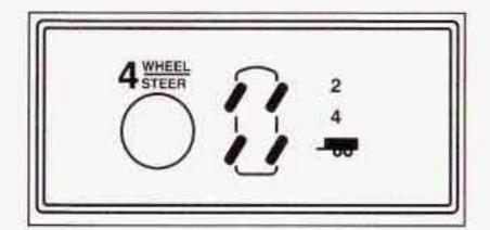
The switch is located on the instrument panel.
