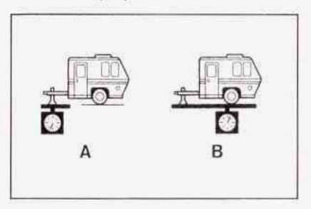
If you're using a weight-carrying or a weight-distributing hitch, the trailer tongue weight (A) should be 10 percent to 15 percent of the total loaded trailer weight (B). Do not exceed the maximum allowable tongue weight for your vehicle.
