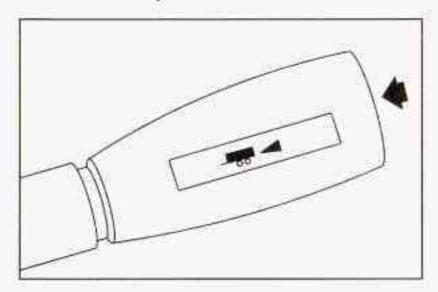
Your vehicle may be equipped with a tow/haul mode. The selector button is located on the end of the column shift lever. You can use this feature to assist when towing or hauling a heavy load. Turn tow/haul on and off by pressing the button until the tow/haul indicator light illuminates on the instrument panel. See "Tow/Haul Mode" under Towing a Trailer on page 4-66 for more information.
