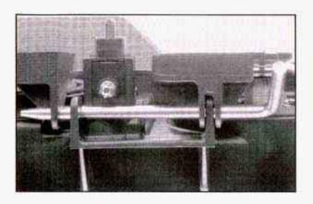
If your vehicle has one pin on the headlamp assembly, remove the pin. To remove the pin, turn the pin up and pull it out straight out.
