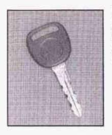
Your vehicle has one double-sided key for the ignition and all door locks as well as the spare tire hoist lock (if equipped).
