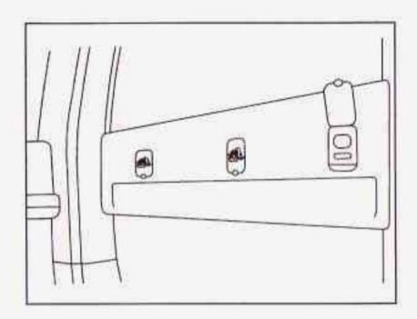
If your vehicle is a regular cab model, there is also a top strap anchor for the right front passenger position located on the back panel of your vehicle, behind the right front passenger seat. In order to get to the anchor, you'll have to remove the trim plug covering it.
