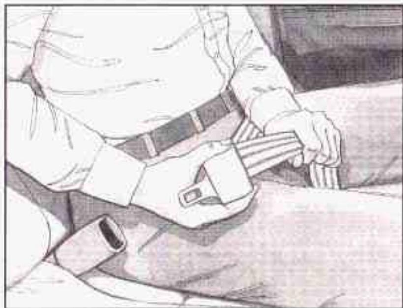
Your lap safety belt has no retractor. To make the belt longer, tilt the latch plate and pull it along the belt.
