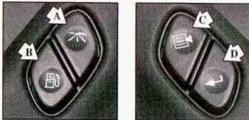
**A (Trip Information):** This button will display the odometer, personal trip odometer, business trip odometer, hourmeter, annual log and the timer.
