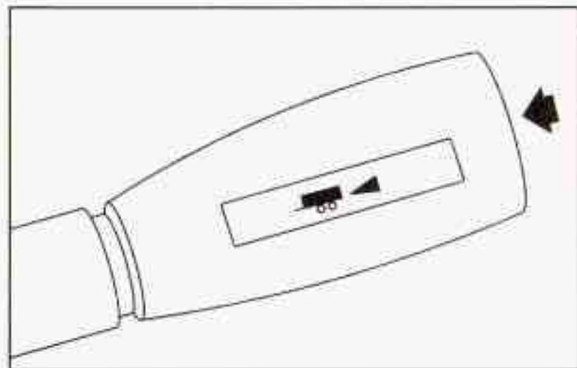
Your vehicle may be equipped with a tow/haul mode. The selector button is located on the end of the column shift lever. You can use this feature to assist when towing or hauling a heavy load. Turn tow/haul on and off by pressing the button until the tow/haul indicator light illuminates on the instrument panel. See "Tow/Haul Mode" under *Towing a Trailer* on page 4-66 for more information.
