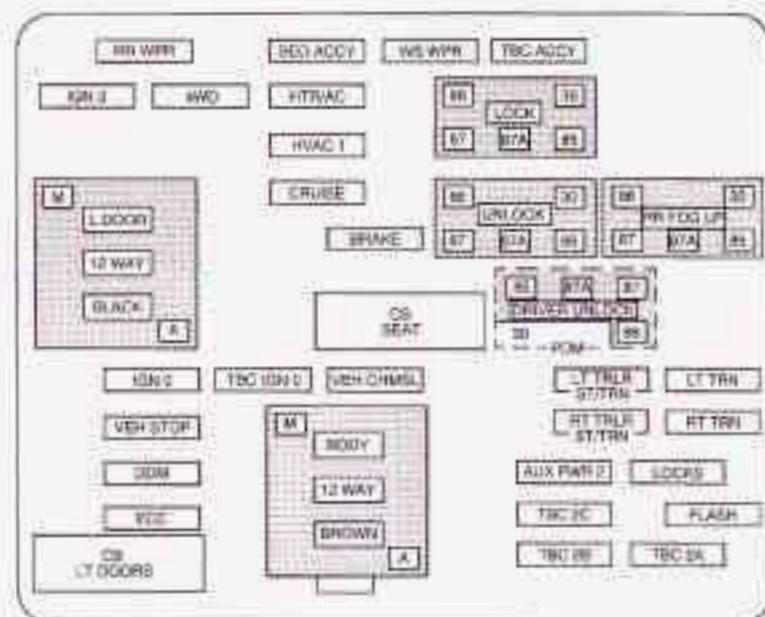
You can remove fuses with a fuse extractor which is mounted to the fuse block access door. To remove fuses, if you don't have a fuse extractor, hold the end of the fuse between your thumb and index finger and pull straight out.
