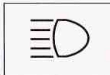
When the high beams are on, this light on the instrument panel cluster also will be on.
