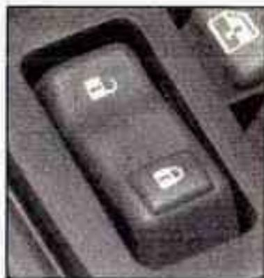
If your vehicle has this power door lock switch, press the raised side of the switch, with the lock symbol, on either front door to lock all the doors at once.
