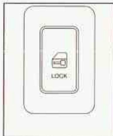
If your vehicle has this power door lock switch, press the bottom of the switch on either front door to lock all the doors at once.
