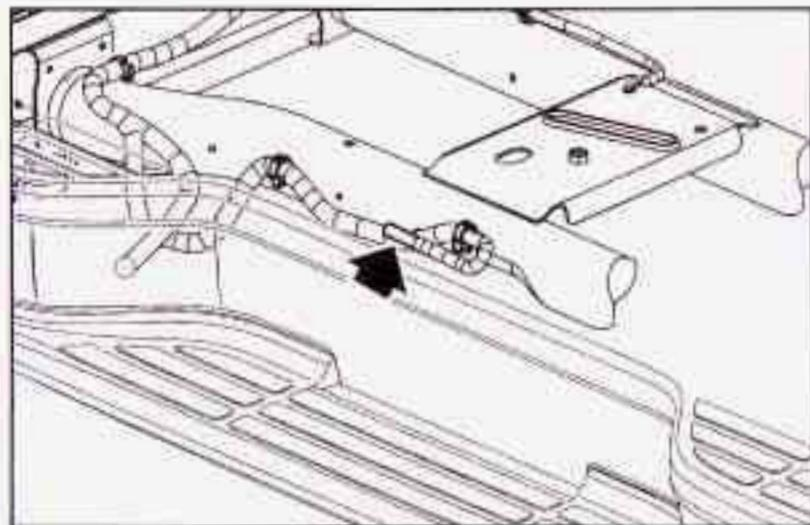
The six-wire harness is located at the rear of the vehicle and is tied to the vehicle's frame. The harness requires the installation of a trailer-wiring harness connector, which is available through your dealer.
