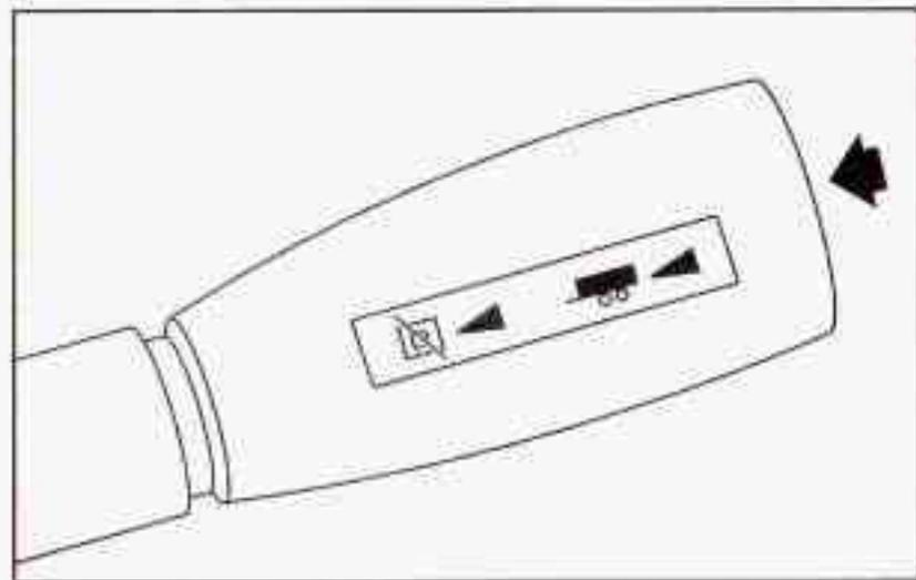
If your vehicle has an Allison Transmission you may have the overdrive disable feature. The overdrive disable feature prevents the transmission from shifting into fifth (5) gear. The selector button is located on the end of the column shift lever. You can turn overdrive disable on and off by pressing and holding the button at the end of the column shift lever until the indicator light, on the instrument panel, illuminates.
