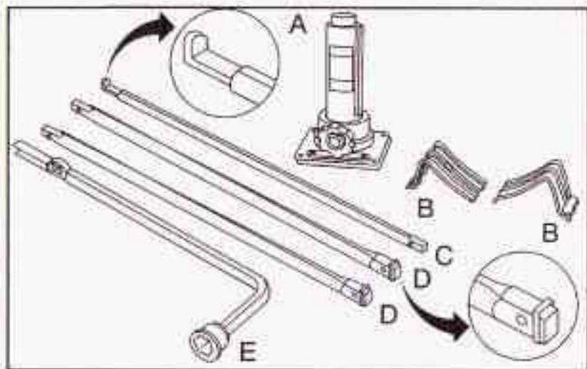
The tools you'll be using include the bottle jack (A), the wheel blocks (B), the jack handle (C), the jack handle extensions (D), and the wheel wrench (E).
