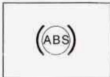
If there's a problem with the anti-lock brake system, this warning light will stay on. See *Anti-Lock Brake System Warning Light* on page 3-41.
