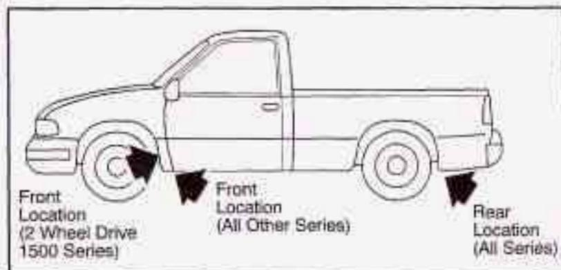
2. Position the jack under the vehicle. If the flat tire is on the front of the vehicle (Two-Wheel Drive 1500 Series vehicles), position the jack under the bracket attached to the vehicle's frame, behind the flat tire. If the flat tire is on the front of the vehicle (all other models), position the jack on the frame behind the flat tire.
