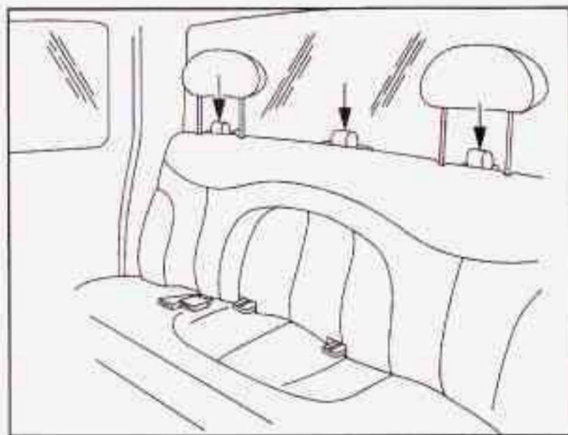
If your vehicle is an extended cab model, you'll find the top strap anchors for the rear seating positions near the top of the seatback. In addition to the top strap anchors, each seating position has a fabric loop at the top of the seatback that you'll use to route a top strap through.
