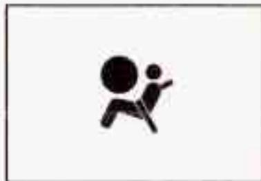
There is an air bag readiness light on the instrument panel cluster, which shows the air bag symbol.
