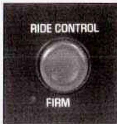
This button is located on the center of the instrument panel near the radio. Press it to activate the selectable ride setting as desired. An indicator light near the button will illuminate whenever the system is active.
