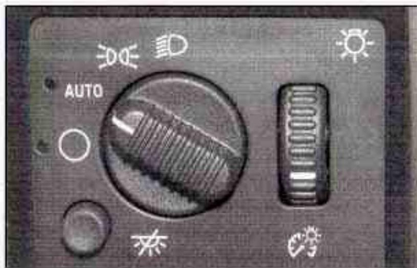
The switch on the driver's side of your instrument panel operates the exterior lamps.
