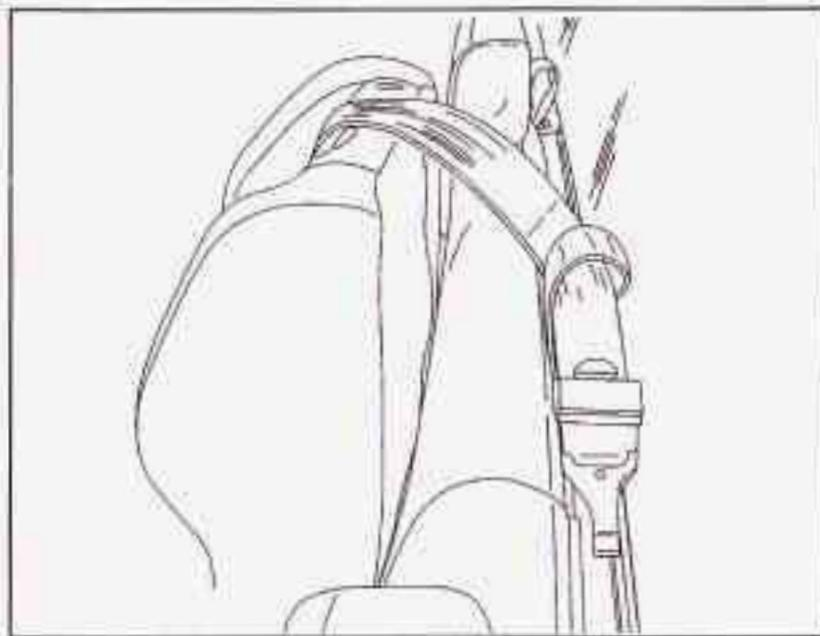
When using a child restraint with a top strap in the center rear position, route the top strap through the fabric loop on the seatback. Then, raise the head restraint and attach the top strap to the anchor point located at the closest outboard position.
