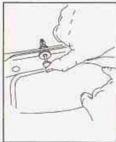
2. Push the flat end of the push-pin toward the retainer until it locks into place, making sure each is secure.
