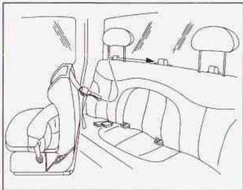
When using a child restraint with a top strap in either rear outboard position, raise the head restraint and route the top strap through the fabric loop on the seatback. Then, attach the top strap to the anchor point at the center rear seating position.
