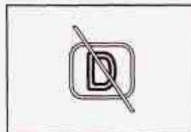
This light will illuminate when the overdrive disable feature is activated. The overdrive disable feature will prevent your vehicle from shifting into fifth (5) gear.
