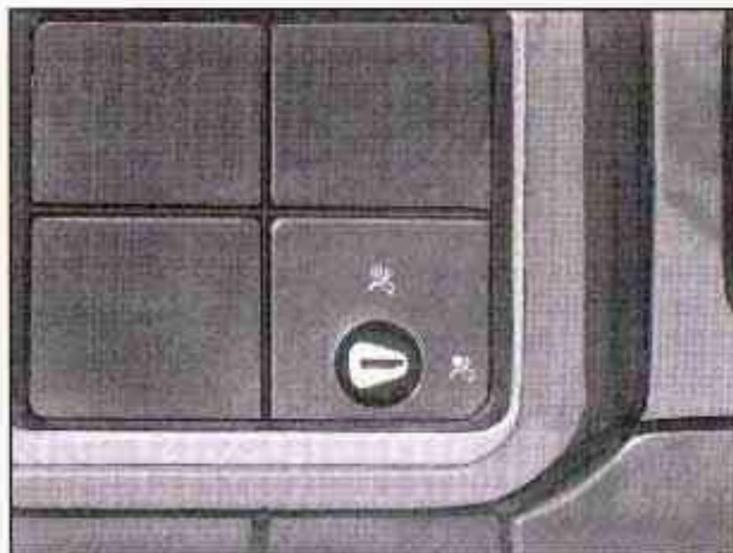
In addition to the AIR BAG OFF switch, your vehicle may have the passenger sensing system. The passenger sensing system is designed to turn off the right front passenger's frontal air bag when a rear facing child restraint is in the right front seat. In addition to the passenger sensing system, you may use the AIR BAG OFF switch located on the instrument panel to turn the air bag off. See *Air Bag Off Switch* on page 1-68 and *Passenger Sensing System* on
