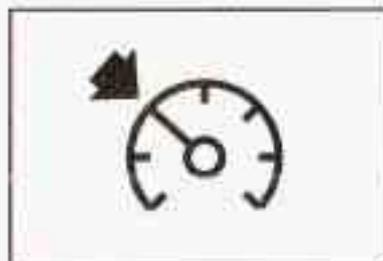
The cruise light on the instrument panel will illuminate when the cruise control is engaged.
