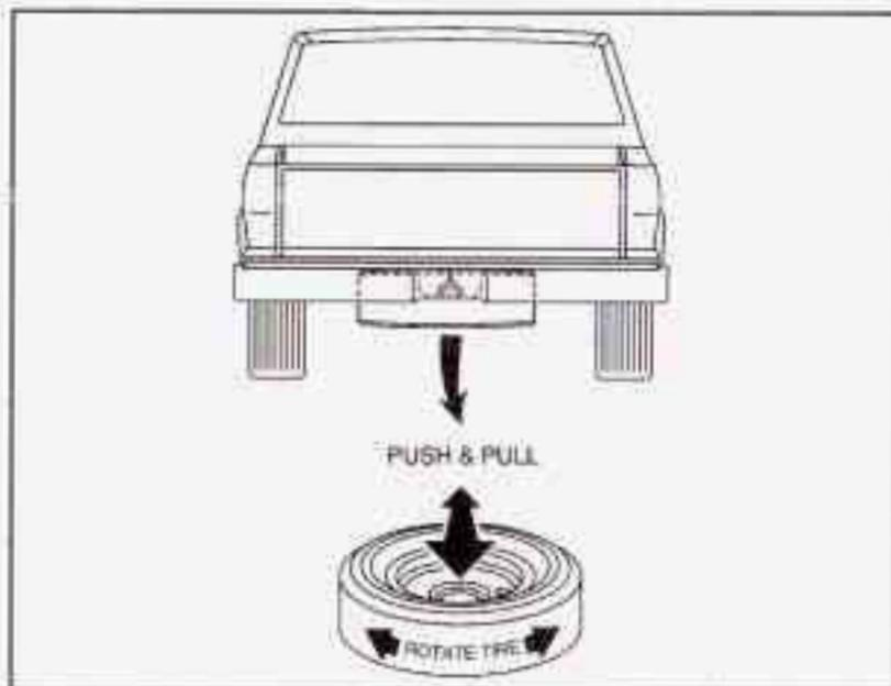
6. Make sure the tire is stored securely. Push, pull, and then try to rotate or turn the tire. If the tire moves, use the wheel wrench/hoist shaft to tighten the cable.
