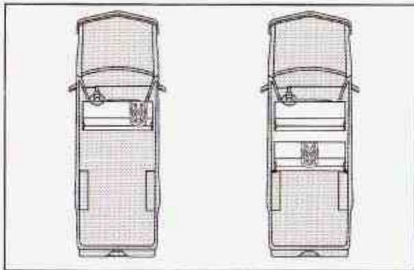
In order to use the system, you need either a forward-facing child restraint that has attaching points (B) at its base and a top tether anchor (C), or a rear-facing child restraint that has attaching points (B), as shown here.
