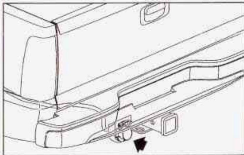
Your pickup may be equipped with the eight-wire trailer towing harness. This harness with a seven-pin universal trailer connector is attached to a bracket on the hitch platform.\*
