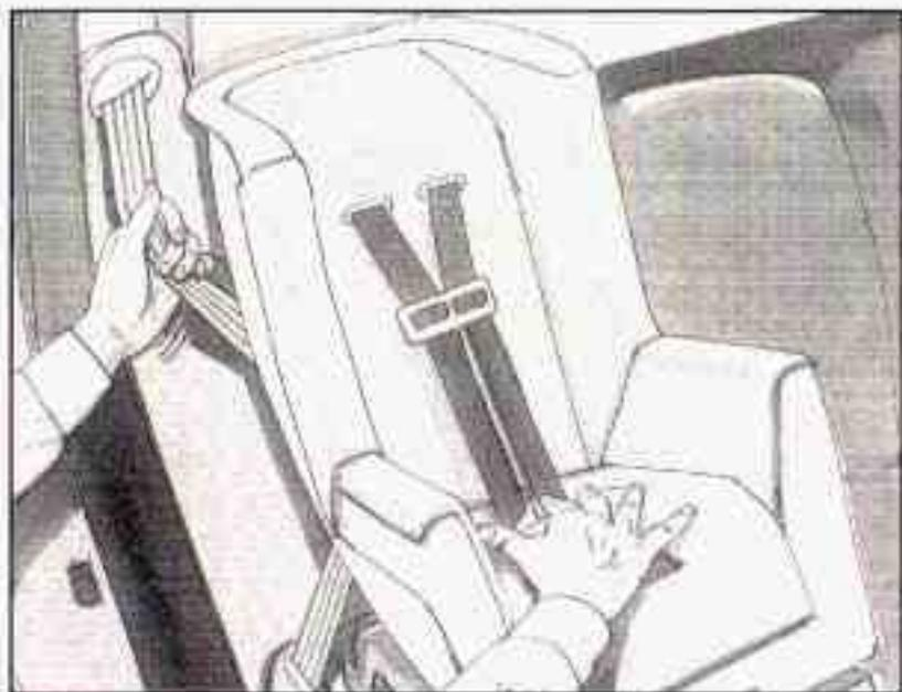
6. To tighten the belt, feed the shoulder belt back into the retractor while you push down on the child restraint. If you're using a forward-facing child restraint, you may find it helpful to use your knee to push down on the child restraint as you tighten the belt. You should not be able to pull more of the belt out of the retractor once the lock has been set.
