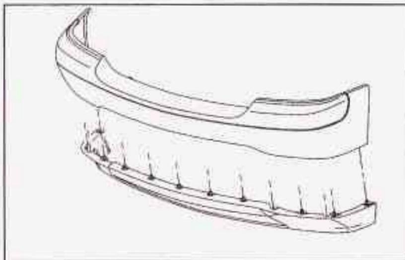
The front bumper lower air dam is held in place by a series of push-pins located around the lower edge of the front bumper. The push-pins are accessible from underneath the front bumper. The following steps must be performed on each of the push-pins to remove the air dam:
