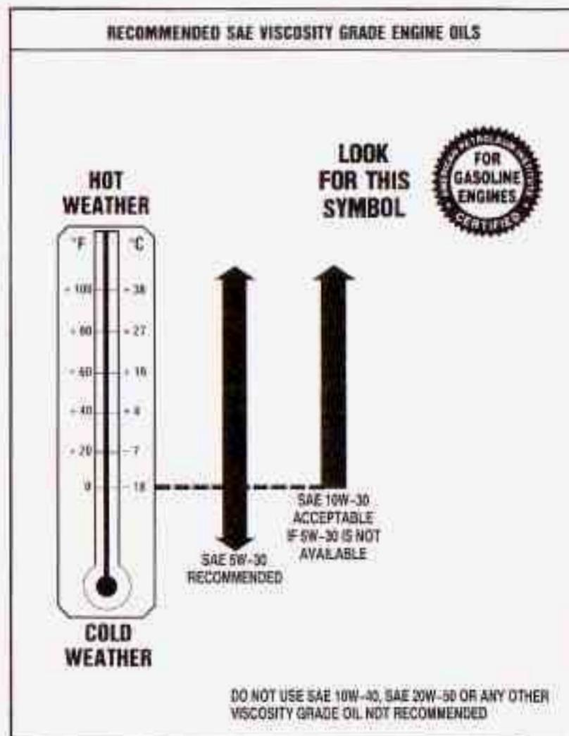
As in the chart shown previously, SAE 5W-30 is the only viscosity grade recommended for your vehicle. You should look for and use only oils which have the API Starburst symbol and which are also identified as SAE 5W-30. If you cannot find such SAE 5W-30 oils, you can use an SAE 10W-30 oil which has the API Starburst symbol, if it's going to be 0°F (-18°C) or above. Do not use other viscosity grade oils, such as SAE 10W-40 or SAE 20W-50 under any conditions.
