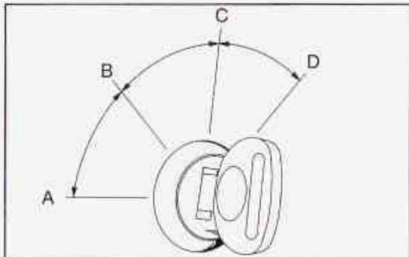
**A (LOCK):** This position locks your ignition and manual transmission. It's a theft-deterrent feature. You will only be able to remove your key when the ignition is turned to LOCK.
