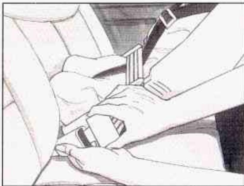
3. Run the vehicle's safety belt through or around the restraint. The child restraint instructions will show you how.
