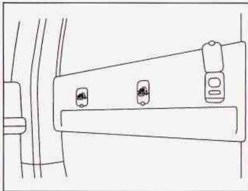
If your vehicle is a Crew Cab model, you'll find top strap anchors for the rear seating positions located on the back panel of your vehicle, behind the rear seat.
