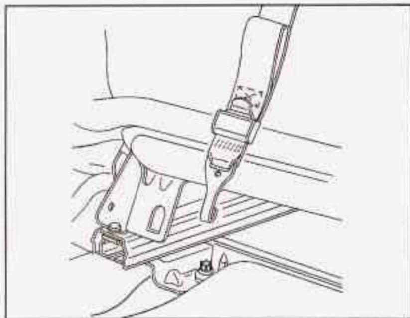
You'll find the top strap anchor for the right front passenger seat behind the seat, near the floor.
