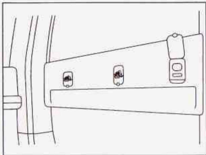
If your vehicle is a regular cab model, there is also a top strap anchor for the right front passenger position located on the back panel of your vehicle, behind the right front passenger seat. In order to get to the anchor, you'll have to remove the trim plug covering it.
