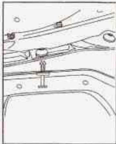
3. Pull the push-pins and lower dam assembly away from the retainers until the lower dam is free.
