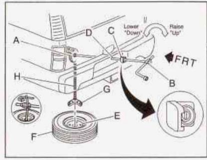
Make sure the tire is stored securely. Push, pull, and then try to rotate or turn the tire. If the tire moves, use the wheel wrench to tighten the cable.
