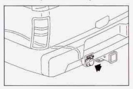
Your vehicle is equipped with the seven-wire trailer towing harness. This harness with a seven-pin universal trailer connector is attached to a bracket on the hitch platform. The seven-wire harness contains the following trailer circuits:
