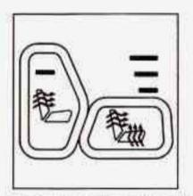
If your vehicle has this feature, the button used to control the driver's heated seat is located on the driver's door panel. The button used to control the passenger's heated seat is located on the passenger's door panel.
