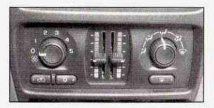
★ (Fan): Turn the left knob clockwise or counterclockwise to increase or decrease the fan speed. Turn the knob to the off position to turn off the fan. If the knob is in off outside air will still enter the vehicle, and will be directed based on the position of the mode knob. The temperature can also be adjusted using the temperature levers.
