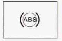
If there's a problem with the anti-lock brake system, this warning light will stay on. See Anti-Lock Brake System Warning Light on page 3-42.
