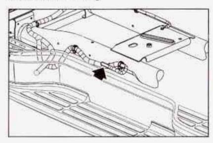
The trailer wiring harness, with a seven-pin connector, is located at the rear of the vehicle and is tied to the vehicle's frame. The harness connector can be plugged into a seven-pin universal heavy-duty trailer connector available through your dealer.
