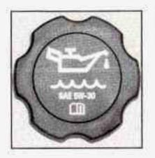
The engine oil fill cap for the VORTEC 4800, 5300, 6000 and 8100 V8 engine is located on the engine valve cover, on the passenger's side of the vehicle.
