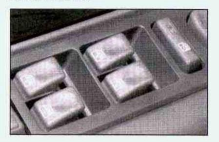
The driver's door has a switch for the passenger's windows as well. Your power windows will work when the ignition has been turned to ACCESSORY or RUN or when Retained Accessory Power (RAP) is active. See Ignition Positions on page 2-21.
