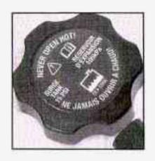
Then replace the pressure cap. Be sure the pressure cap is hand-tight and fully seated. You may also hear this fan noise when you start the engine. It will go away as the fan clutch partially disengages.
