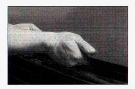
Then go to the front of the vehicle and pull up on the secondary hood release located near the center of the grill. 3. Lift the hood.
