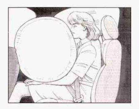
The right front passemger's frontal air bag is in the instrument panel on the passenger's side.
