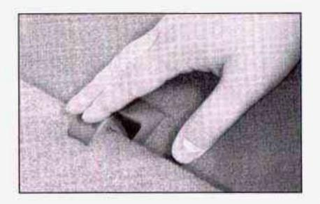
To create a load floor release the panels from the seatback by pushing forward on the latch. Then fold the panels back to cover the rear seat footwell area.
