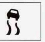
The Stabilitrak® mode button is located on the instrument panel. Stabilitrak<sup>®</sup> and part of the traction control system can be turned off or back on by pressing the Stabilitrak<sup>®</sup> button. All-wheel drive vehicles must be in all-wheel drive mode to turn the system on or off.
