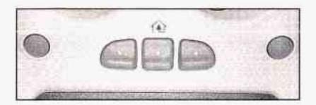
HomeLink® a combined universal transmitter and receiver, provides a way to replace up to three hand-held transmitters used to activate devices such as gate operators, garage door openers, entry door locks, security systems and home lighting. Additional HomeLink® information can be found on the internet at www.homelink.com or by calling 1-800-355-3515.
