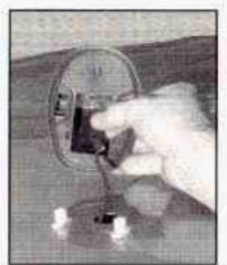
Put a new bulb into the socket and turn clockwise until it locks in place.
