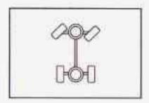
The four-wheel drive indicator will light up when you shift a manual transfer case into four-wheel drive and the front axle engages.
