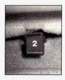
To unlatch the seat from the floor, pull up on the release lever labeled 2, located at the rear of the seat, and lift the rear of the seat up off the floor.
