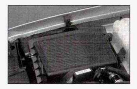
The air cleaner/filter assembly is located on the front corner of the engine compartment on the passenger's side of the vehicle. See Engine Compartment Overview on page 5-14 for more information on location.
