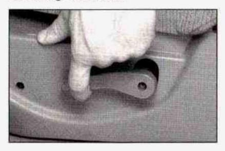
To adjust the front seatback, lift the manual lever located on the outboard side of the seat. Release the lever to lock the seatback where you want it. Lift the lever again without pushing on the seatback and the seatback will go to an upright position. If your vehicle has power seats with a power recliner, see Power Seats on page 1-4 for further information on how to operate the reclining seatback feature.
