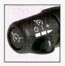
With cruise control, you can maintain a speed of about 25 mph (40 km/h) or more without keeping your foot on the accelerator. This can really help on long trips. Cruise control does not work at speeds below about 25 mph (40 km/h).
