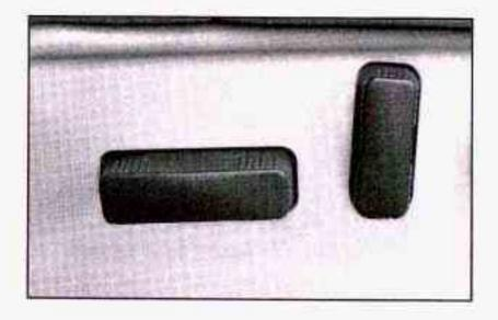
If your vehicle has a power seat, you can adjust it with these controls located on the outboard sides of the seats.
