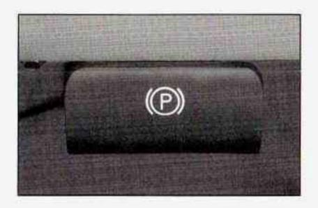
To release the parking brake, hold the regular brake pedal down. Pull the bottom edge of the lever, located above the parking brake pedal, with the parking brake symbol, to release the parking brake.
