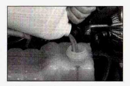
Then fill the coolant surge tank with the proper mixture, to the FULL COLD mark.
