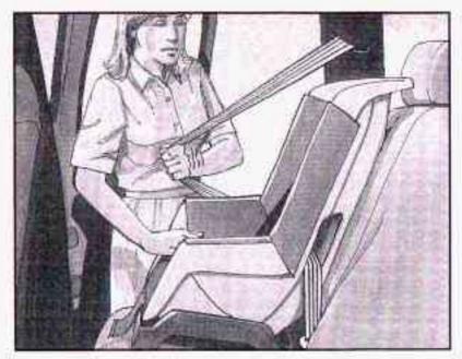
Pull the rest of the shoulder belt all the way out of the retractor to set the lock.
