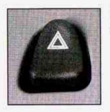
The hazard warning flasher is located at the top of the steering column.
