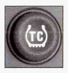
To turn the system on or off, press the TAS on/off button located on the instrument panel.
