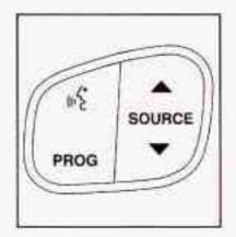
equipped with the steering wheel control buttons you can use them to interact with the OnStar® system.
