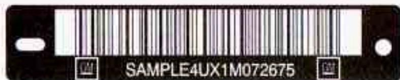
This is the legal identifier for your vehicle. It appears on a plate in the front corner of the instrument panel, on the driver's side. You can see it if you look through the windshield from outside your vehicle. The VIN also appears on the Vehicle Certification and Service Parts labels and the certificates of title and registration.
