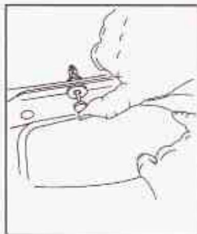
2. Push the flat end of the push-pin towards the retainer until it locks into place, making sure each is secure.
