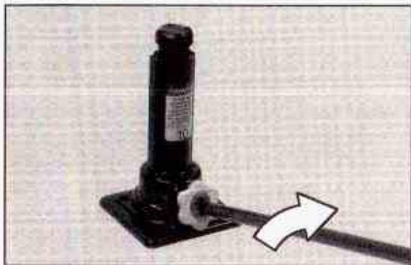
Turn the wheel wrench clockwise to raise the jack lift head to the lifting point.
