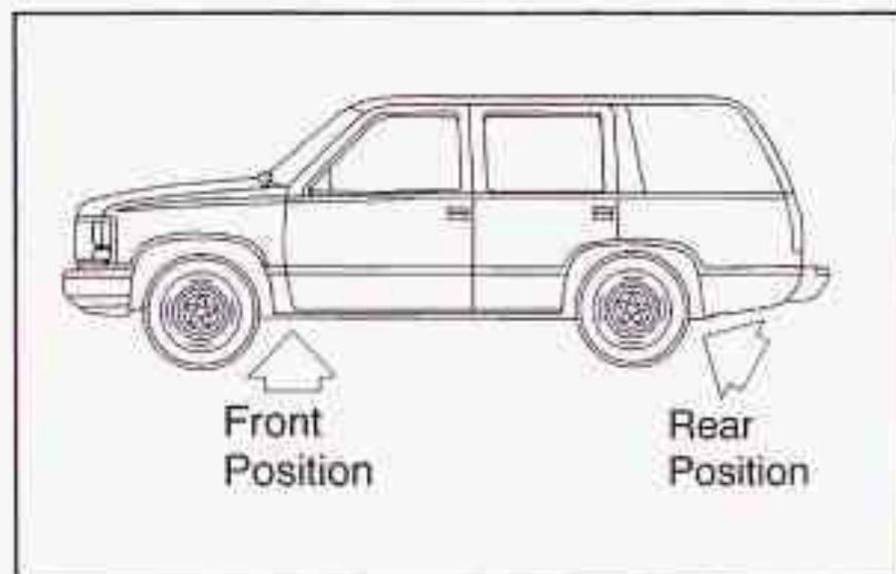
**Notice:** If your vehicle is equipped with **QUADRASTEER™** avoid contact with tie rods and tie rod boots when jacking the vehicle.
