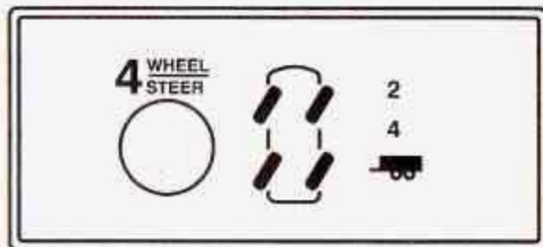
The switch is located on the instrument panel.
