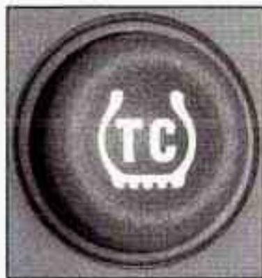
To turn the system on or off, press the TAS on/off button located on the instrument panel.
