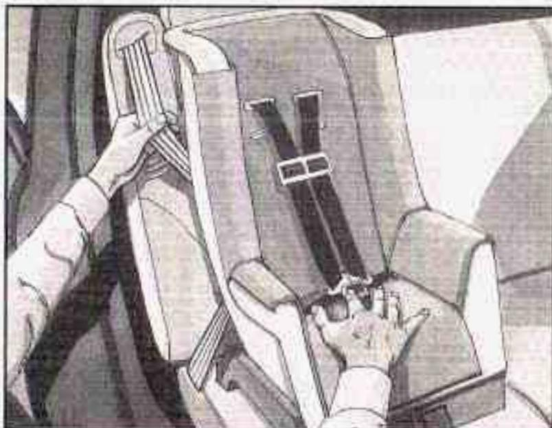
6. To tighten the belt, feed the shoulder belt back into the retractor while you push down on the child restraint. You may find it helpful to use your knee to push down on the child restraint as you tighten the belt. You should not be able to pull more of the belt out of the retractor once the lock has been set.
