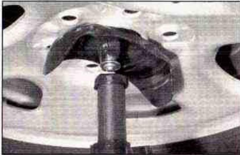
9. Turn the wrench clockwise to raise the jack until it lifts the end fitting
