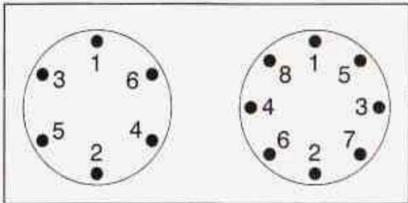
8. Tighten the nuts firmly in a crisscross sequence as shown by turning the wheel wrench clockwise.
