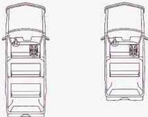
Your vehicle has a right front passenger air bag. A rear seat is a safer place to secure a forward-facing child restraint. Unless your vehicle has the passenger sensing system, *Never* put a rear-facing child restraint in this seat.
