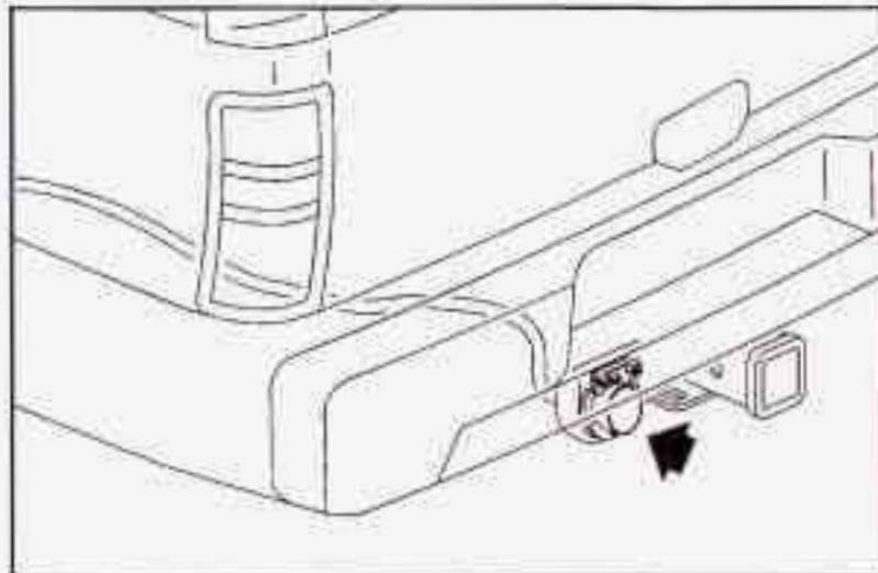
Your vehicle is equipped with the seven-wire trailer towing harness. This harness with a seven-pin universal trailer connector is attached to a bracket on the hitch platform.
