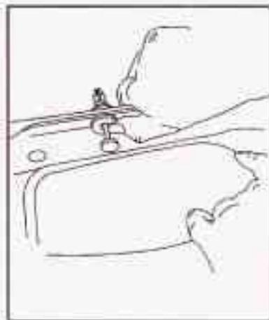
1. Line up each push-pin with its intended retainer and push the washer portion of the push-pin towards the retainer until it locks into place.
