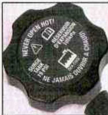
1. Park the vehicle on a level surface. You can remove the coolant surge tank pressure cap when the cooling system, including the coolant surge tank pressure cap and upper radiator hose, is no longer hot.
