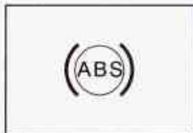
If there's a problem with the anti-lock brake system, this warning light will stay on. See *Anti-Lock Brake System Warning Light* on page 3-42.
