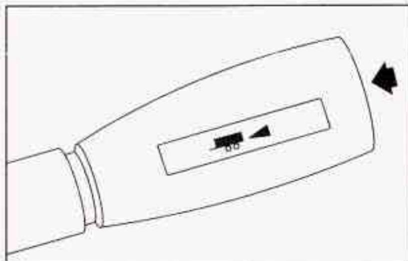
Your vehicle may be equipped with a tow/haul mode. If so, the selector button is located on the end of the column shift lever. You can use this feature to assist when towing or hauling a heavy load. See *Towing a Trailer* on page 4-59 for more information.
