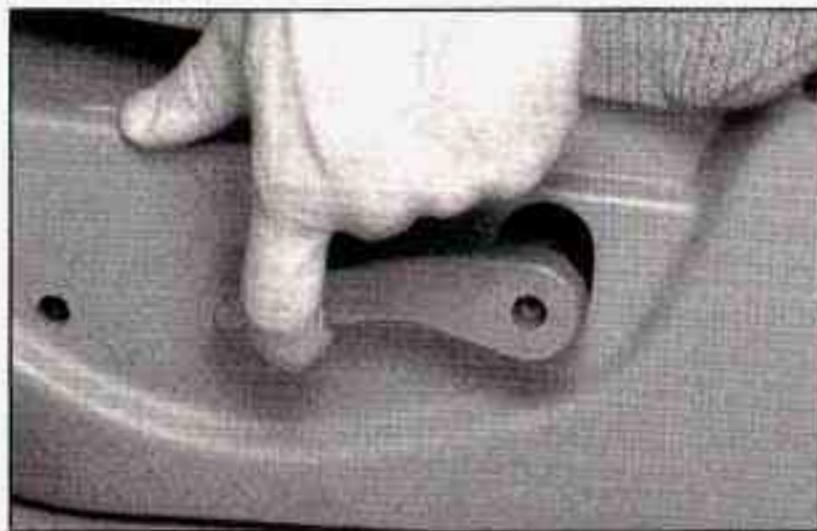
To adjust the front seatback, lift the manual lever located on the outboard side of the seat. Release the lever to lock the seatback where you want it. Lift the lever again without pushing on the seatback and the seatback will go to an upright position.
