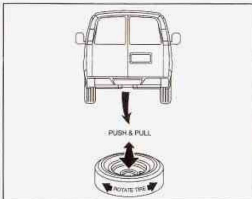
6. Make sure the tire is stored securely. Push, pull, and then try to rotate or turn the tire. If the tire moves, use the wheel wrench to tighten the cable. Put back the jack, tools and spare tire lock (if equipped).
