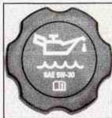
The engine oil fill cap for the VORTEC 4800, 5300, 6000 and 8100 V8 engine is located on the engine valve cover, on the passenger's side of the vehicle.
