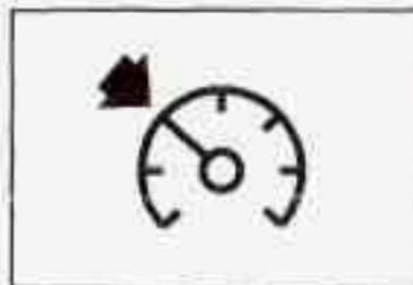
The cruise light on the instrument panel will illuminate when the cruise control is engaged.
