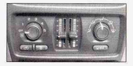
(Fan): Turn the left knob clockwise or counterclockwise to increase or decrease the fan speed. If the knob is in off outside air will still enter the vehicle, and will be directed based on the position of the mode knob. The temperature can still be adjusted using the temperature knob.
