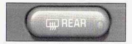
Press this button to turn the rear window defogger on or off. An indicator light in the button will come on to let you know that the rear window defogger is active. The rear window defogger will automatically turn off approximately ten minutes after the button is pressed.
