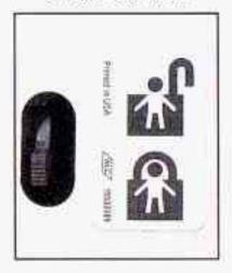
Move the lever down to engage the safety lock. Move the lever up to disengage the safety lock. The rear doors of your vehicle cannot be opened from the inside when this feature is in use. If you want to open the rear door when the security lock is on, unlock the door and open the door from the outside.
