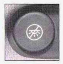
The dome override button is located below the exterior lamps knob.
