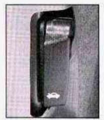
To open the hood, first pull the handle located inside the vehicle on the lower driver's side of the instrument panel.
