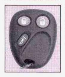
press unlock, the driver's door will unlock automatically, the parking lamps may flash and the interior lights will go on.
