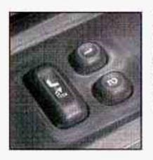
Your vehicle may have this feature. The controls are located on the driver's door, and are used to program and recall memory settings for the driver's seating and outside mirror positions.
