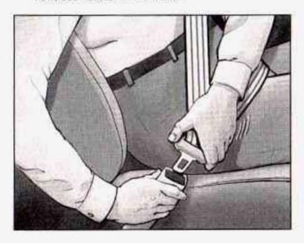
Pick up the latch plate and pull the belt across you. Don't let it get twisted. Push the latch plate into the buckle until it clicks.
