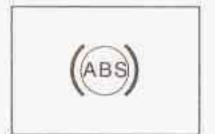
If there's a problem with the anti-lock brake system, this warning light will stay on. See Anti-Lock Brake System Warning Light on page 3-38. Along with ABS, your vehicle has a Dynamic Rear Proportioning (DRP) system. If there's a DRP problem, both the brake and ABS warning lights will come on accompanied by a 10-second chime. The lights and chime will come on each time the ignition is turned on until the problem is repaired. See your dealer for service.
