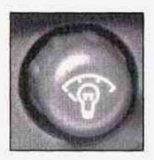
Press the knob located next to the exterior lamps knob to extend it. Adjust the instrument panel lights. Turn the knob all the way up to turn on the interior lamps. Press the knob back into its stored position when you're not using it.
