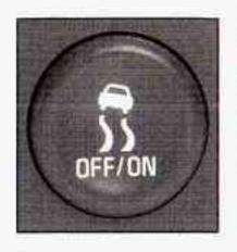
To turn the system on or off, press the TAS OFF/ON button located near the shift lever. If you used the button to turn the system off, the TRAC OFF light on the button will come on and stay on.
