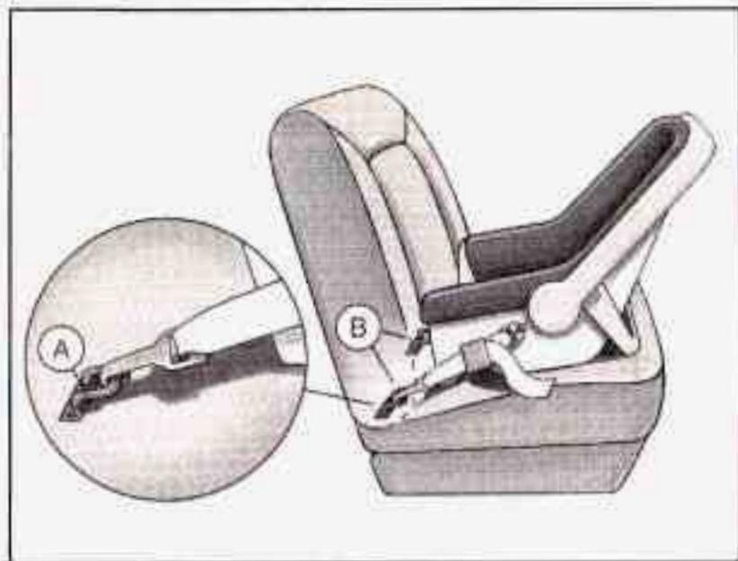
With this system, use the LATCH system instead of the vehicle's safety belts to secure a child restraint. See *Securing a Child Restraint in a Rear Outside Seat Position* on page 1-43.
