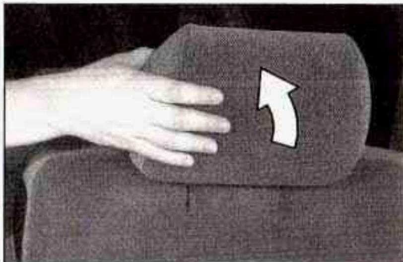
To return the head restraint to the upright position, reach behind the seat and pull the restraint up until it locks into place. Push and pull on the head restraint to make sure that it is latched securely.
