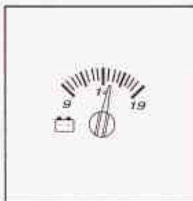
When your engine is not running, but the ignition is on (in RUN), this gage shows your battery's state of charge in DC volts.
