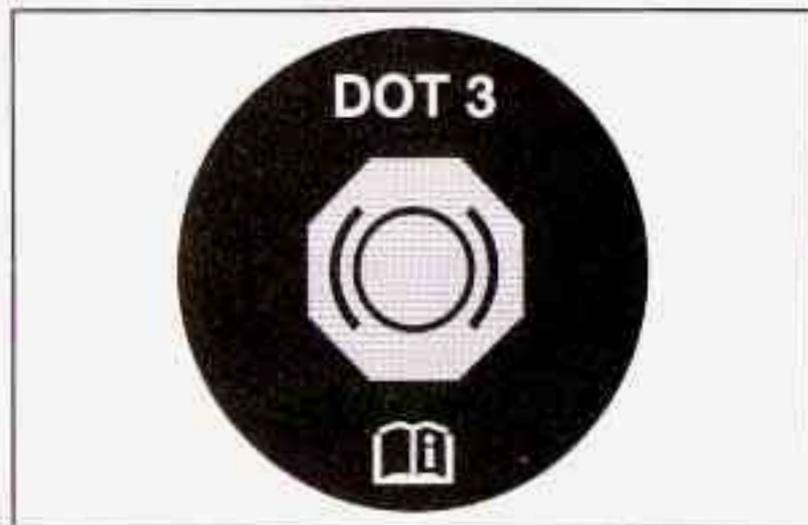
Your brake master cylinder reservoir is filled with DOT-3 brake fluid. See *Engine Compartment Overview* on page 5-12 for the location of the reservoir.
