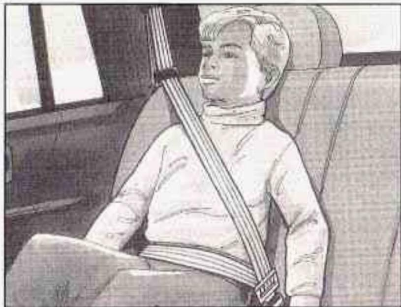
4. Buckle, position and release the safety belt as described in *Rear Seat Passengers* on page 1-22. Make sure that the shoulder belt crosses the shoulder.
