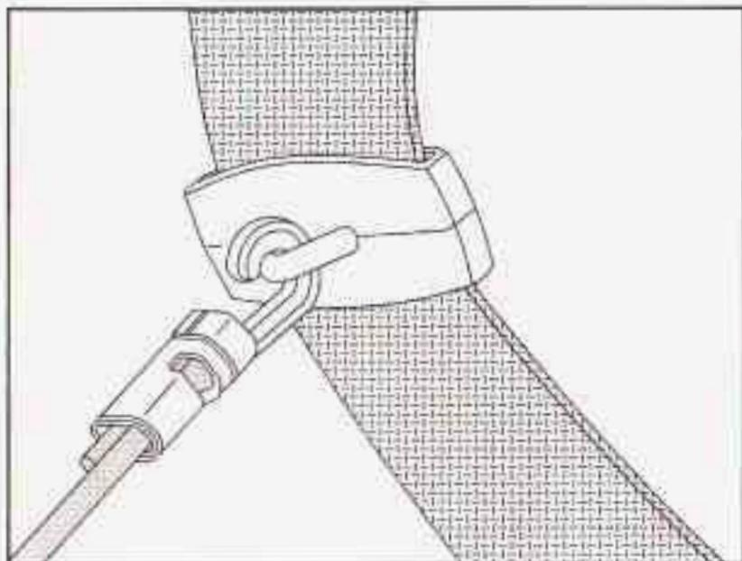
2. Align the sliding comfort guide, located on the shoulder belt, with the hook. Attach the hook to the loop on the sliding comfort guide.
