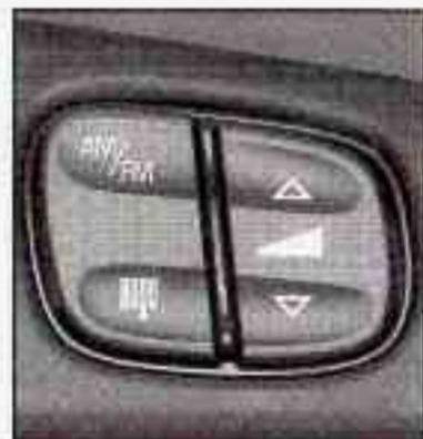
If your vehicle has this feature, certain radio functions can be operated by using the controls on your steering wheel.
