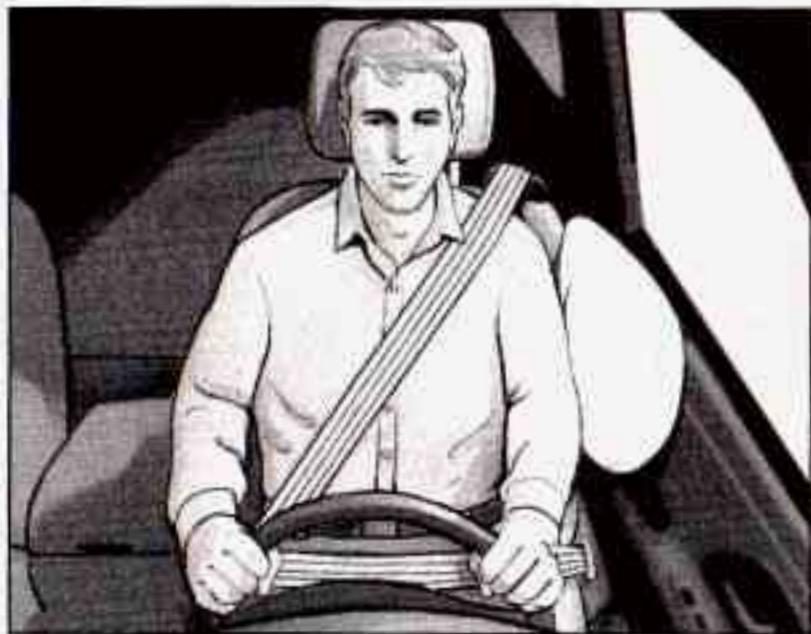
If your vehicle has one, the driver's side impact air bag is in the side of the driver's seatback closest to the door.
