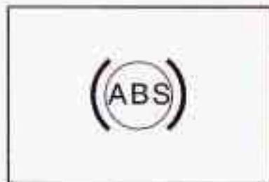
With the anti-lock brake system, this light will come on when you start your engine and may stay on for several seconds. That's normal. A chime may also sound when the light comes on.
