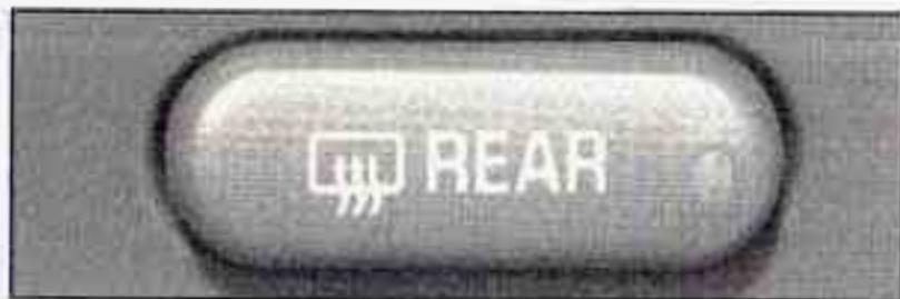
Press this button to turn the rear window defogger on or off. An indicator light in the button will come on to let you know that the rear window defogger is active.
