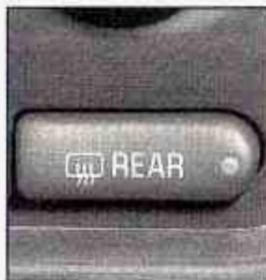
Press this button to turn the rear window defogger on or off.
