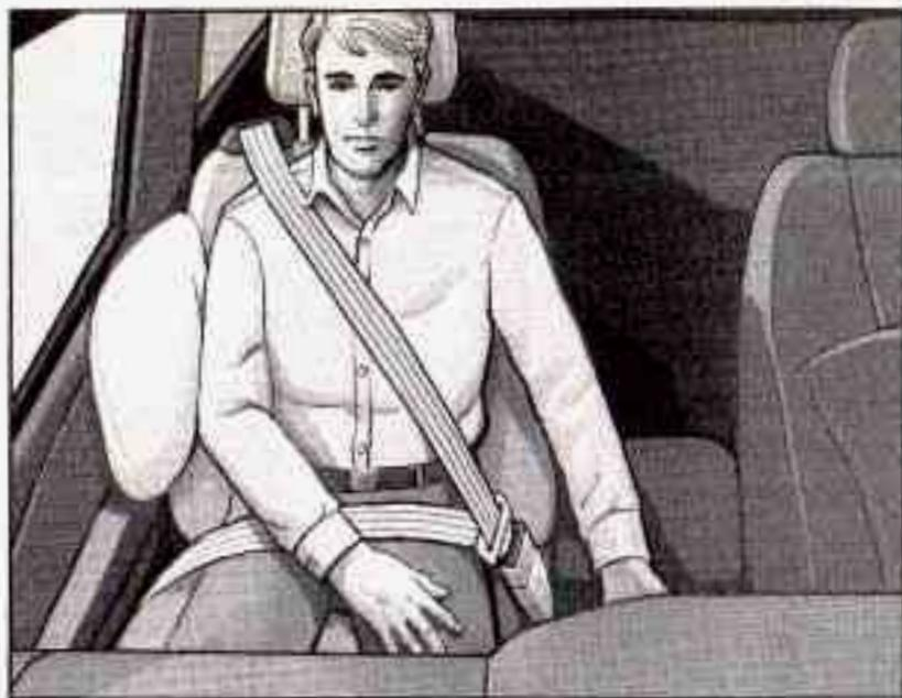
If your vehicle has one, the right front passenger's side impact air bag is in the side of the passenger's seatback closest to the door.
