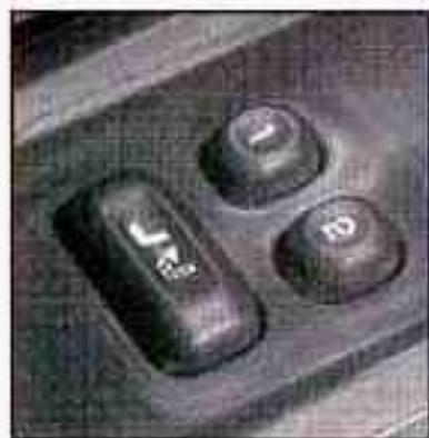
Your vehicle may have this feature. The controls are located on the driver's door, and are used to program and recall memory settings for the driver's seating and outside mirror positions.
