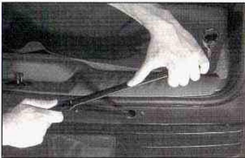
If the spare tire is hanging from the cable, insert the jack handle, extension and wheel wrench into the hoist shaft hole in the bumper, on an angle, and turn the wheel wrench counterclockwise to lower the spare the rest of the way.
