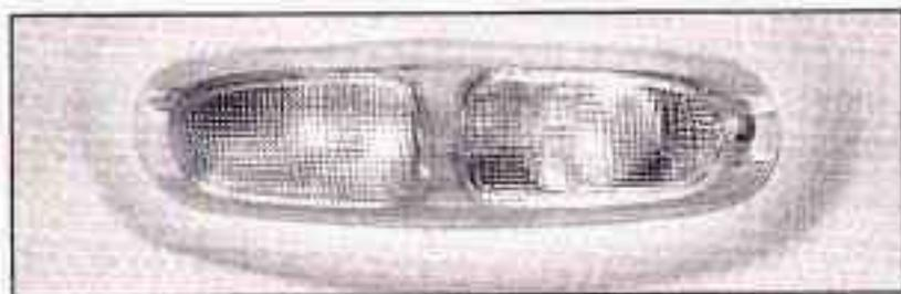
Press the lens on the lamp located above the doors to turn the reading lamps on and off.
