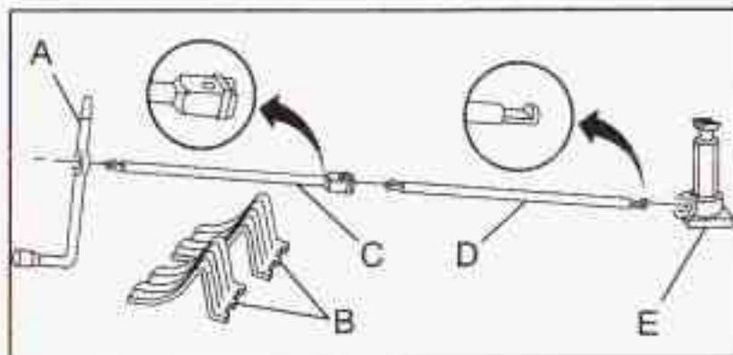
The tools you'll be using include the wheel wrench (A), tire blocks (B), extension(s) (socket end) (C), handle (jack end) (D), and jack (E). The Trailblazer EXT will include an additional extension.
