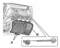
Twist the compartment retainers (A) and pull outward to remove.
