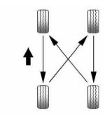
When rotating the vehicle's tires, always use the correct rotation pattern shown here.
