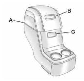
For vehicles with a second row center console, press the buttons (B) or (C) to access storage areas.
