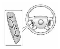
(\*): Press to turn cruise control on and off. The indicator comes on when cruise control is on.
