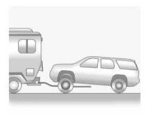
To tow a front-wheel-drive vehicle from the front with two wheels on the ground:
