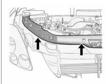
Detach fasteners and lift off the panel that covers the radiator cap.
