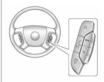
△ / ➢ ▽: Press to change favorite radio stations, select tracks on a CD/DVD, or to navigate tracks or folders on an iPod® or USB device.
