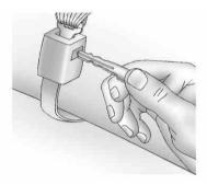
Disconnect the rear safety belt mini-latch using a key in the slot on the mini-buckle, and let the belt retract into the headliner. Stow the mini-latch in the holder in the headliner.
