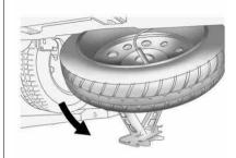
Lower the jack by turning the lug wrench counterclockwise. Keep lowering the jack until the spare tire slides off the jack.
