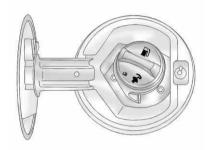
To remove the fuel cap, turn it slowly counterclockwise. The fuel cap has a spring in it; if the cap is released too soon, it will spring back to the right.
