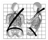
Sit up straight and always keep your feet on the floor in front of you. The lap part of the belt should be worn low and snug on the hips, just touching the thighs. In a crash, this applies force to the strong pelvic
