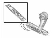
**P (Park):** This position locks the front wheels. It is the best position to use when starting the engine because the vehicle cannot move easily.
