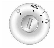
The ignition switch has four different positions.
