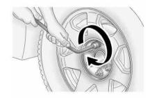
Loosen the wheel nuts — but do not remove them — using the lug wrench. For wheels with a wheel lock key, use the wheel lock key between the lock nut and lug wrench. The key is supplied in the front passenger door pocket. Notice: If this vehicle has wheel locks and an impact wrench is used to remove the wheel nuts, the lock nut or wheel lock key could be damaged. Do not use an impact wrench to remove the wheel nuts if this vehicle has wheel locks.
