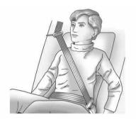
Buckle, position, and release the safety belt as described previously in this section. Make sure the shoulder portion of the belt is on the shoulder and not falling off of it. The belt should be close to, but not contacting, the neck
