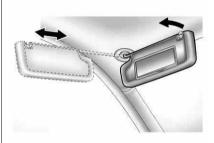
Pull the sun visor down to block glare. Detach the sun visor from the center mount to pivot to the side window, or to extend along the rod, if available
