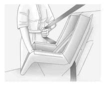
Pull the shoulder belt all the way out of the retractor to set the lock. When the retractor lock is set, the shoulder belt can be tightened but not pulled out of the retractor.
