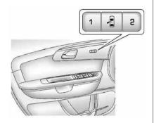
On vehicles with the memory feature, the controls on the driver door are used to program and recall memory settings for the driver seat and outside mirrors.
