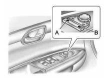
The controls for power foldaway mirrors are located on the driver door.
