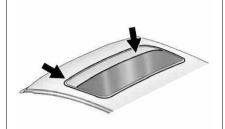
Do not keep the sunroof open for long periods of time while the vehicle is not in use. Dirt and debris may collect on the sunroof seal or in the tracks that could cause an issue with sunroof operation, noise or plug the water drainage system. Periodically open the sunroof and remove any obstacles or loose debris. Wipe the sunroof seal and roof sealing area using a clean cloth, mild soap, and water. Do not remove grease from sunroof.
