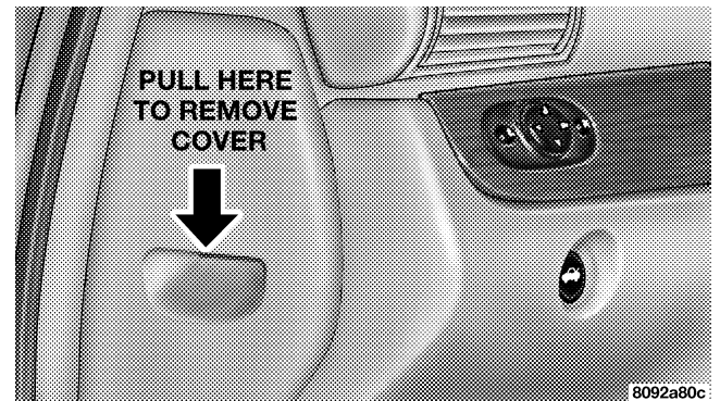
Fuse Panel Cover
